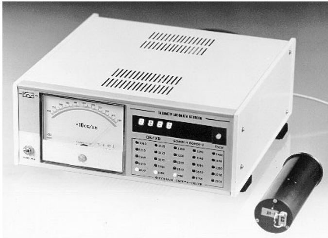
Figure 8.21 Conventional tachometer and firing-pins sensor
