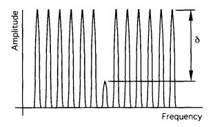
**Figure 1.19** Composite triple-beat  $(=\delta)$  measurement.
