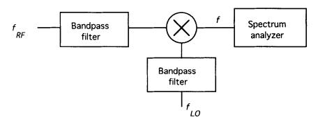
Figure 3.11 Mixer IP2 measurement.
