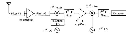
Figure 1.6 Typical dual-conversion receiver.
