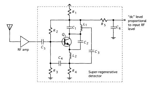
Figure 2.121 Self-quenched superregenerative receiver.
