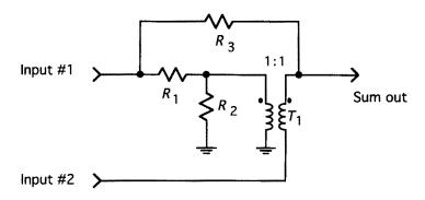
Figure 2.107 A 6-dB power splitter/combiner.
