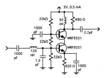
Figure 2.5 Low-current cascode amplifier.
