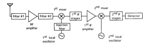
Figure 1.1 Typical dual-conversion receiver.
