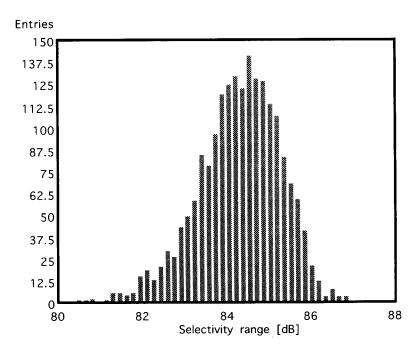
Figure 4.21 Histogram of simulated selectivity distribution.
