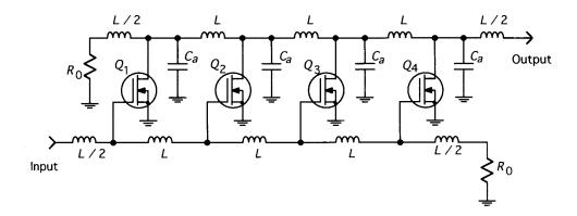
Figure 2.4 Four-stage distributed amplifier.
