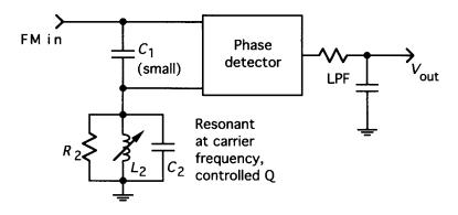
Figure 2.42 Quadrature detector.
