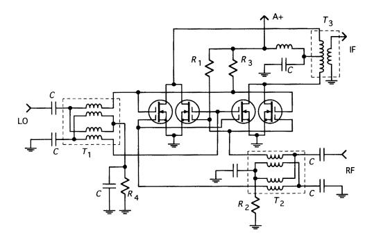
Figure 2.86 Dual-gate FET double-balanced mixer.
