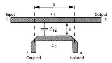
Figure 2.59 Printed directional coupler much shorter than  $\lambda/4$ .
