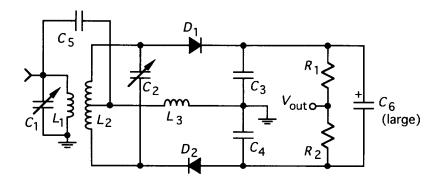
Figure 2.43 Ratio FM detector.
