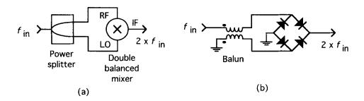
Figure 2.75 Passive frequency doublers.
