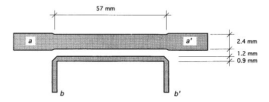
Figure 2.60 A 30-dB 125-MHz microstrip directional coupler.
