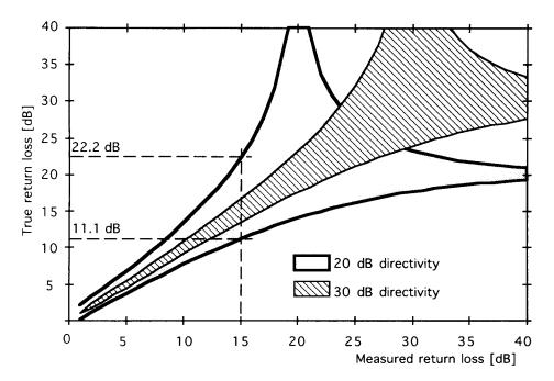
Figure 3.7 Relationship between return loss and directivity.
