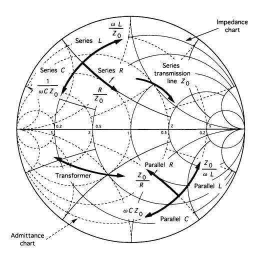
Figure 2.77 Impedance matching guide.
