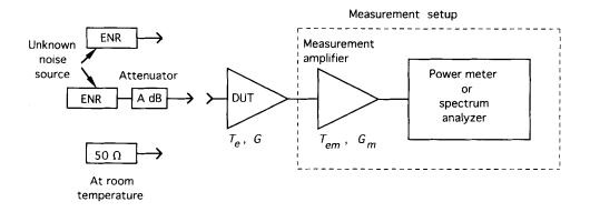
Figure 3.24 Approximate determination of unknown noise source ENR.
