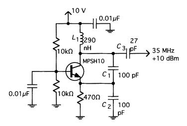
Figure 2.92 Colpitts 35-MHz oscillator.
