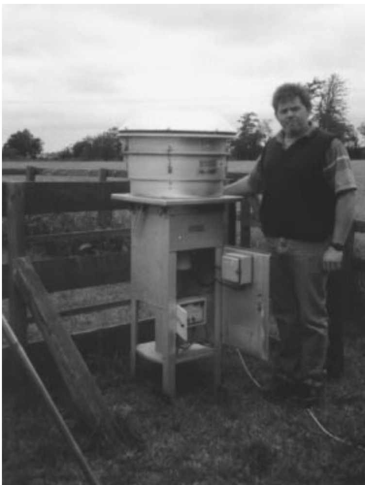
FIGURE 73.8 Cascade impactor with a 10 \mu\text{m} inlet head operating at a rural site in eastern England.
