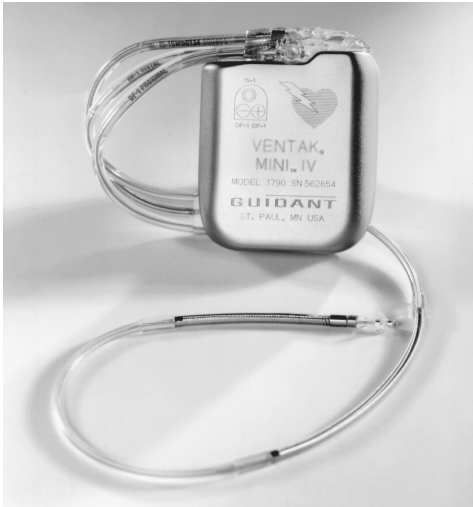
Figure 115.14 The Guidant/CPI Ventak Mini IV ICD with the Endotak lead system attached (a single-pass lead). The Mini IV is a single chamber defibrillator. (Courtesy of Guidant/CPI, St. Paul, MN.)
