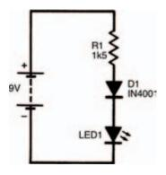
Figure 6.3 Our first simple circuit using a diode
