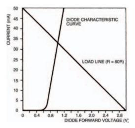
Figure 7.5 Load line from Table 1 results
