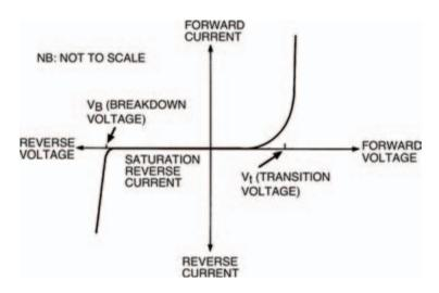
Figure 6.14 Plotting the reverse bias characteristics for an ordinary diode is not practical, so we give you the characteristic curve here
