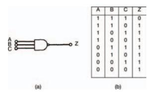
Figure 10.30 A three input NAND gate (a) symbol, (b) truth table
