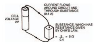
Figure 1.5 Cell's voltage is 2 V, and a current of 0.4 A flows
