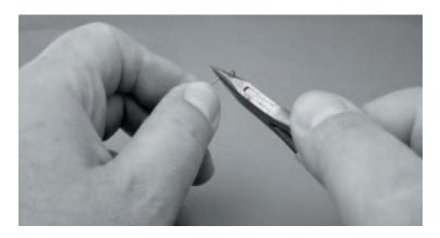
Photo 5.2 ... and bend it carefully into two right angles, judging the length
