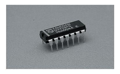
Photo 2.3 A DIL (dual-in-line) IC package
