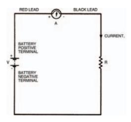
Figure 3.6 A diagram showing a meter connected in circuit, with the red lead at the point of higher potential
