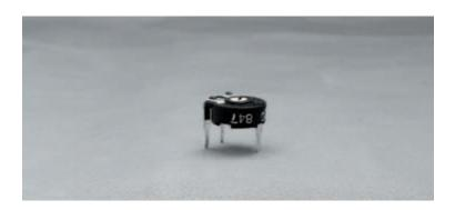
Photo 6.1 A horizontal preset resistor
