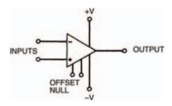
Figure 9.2 The circuit symbol for a 741
