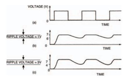
Figure 7.17(a) The squarewave output from the circuit in Figure 7.16 experimentally modified by a 100  $k\Omega$  resistor (b) and a 10  $k\Omega$  resistor (c)
