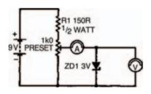
Figure 6.16 A circuit with the zener diode forward biased
