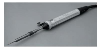
Photo 1.3 Low wattage soldering iron intended for electronics
