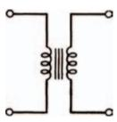
Figure 7.7 The circuit symbol for a transformer
