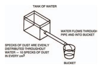
Figure 1.1 Water flowing in a pipe is like electricity in a wire
