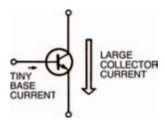
Figure 8.9 Important: a very small base current can control a large collector current
