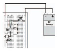
Figure 10.7 Possible breadboard layout of the circuit in Figure 10.6
