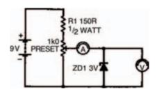
Figure 6.17 The circuit, with the zener diode reverse biased
