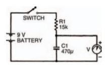
Figure 4.4 A simple resistor and capacitor circuit
