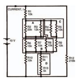
Figure 3.1 A resistor network in which the total resistance can only be calculated by breaking it down into blocks
