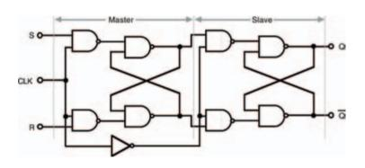
Figure 11.10 An edge-triggered SR-type NAND bistable
