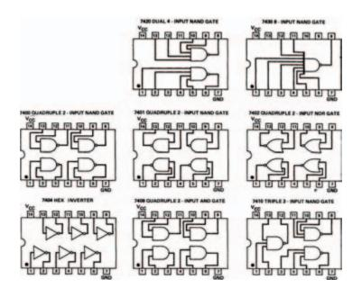
Figure 11.7 Some integrated circuits from the 74 series of transistor—transistor logic (TTL) digital devices
