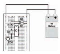
Figure 10.27 Breadboard layout to build the circuit of Figure 10.26
