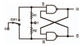
Figure 11.7 Simple circuit to prevent contact bounce
