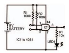
Figure 10.16 Circuit to investigate AND gate Boolean operation
