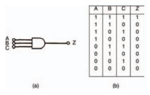
Figure 10.20 (a) a three input AND gate; (b) its truth table
