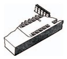
Figure 2.1 The interior of a breadboard, showing the contacts
