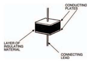
Figure 4.1 A simple diagrammatic representation of a capacitor
