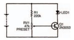
Figure 8.12 A circuit to test a transistor with a varible base current
