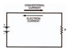
Figure 3.8 Conventional current travels from positive to negative; electron current travels in the opposite direction
