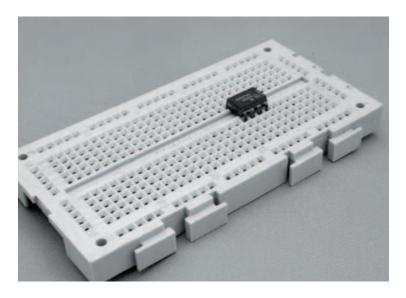
Photo 5.6 The IC mounted across the central divide in the breadboard, which is designed to be the exact size
