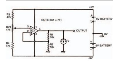
Figure 9.5 Our first experimental circuit: a non-inverting amplifier with a three-rail power supply
