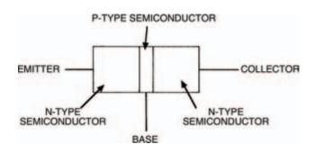
Figure 8.3 A narrow P-area gives two PN junctions very close together
