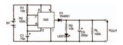
Figure 7.19 The same circuit with a smoothing capacitor added
