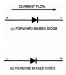
Figure 6.6 Circuit diagrams for forward and reverse biased diodes
