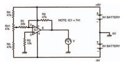
Figure 9.7 Our next experimental circuit: an inverting amplifier
