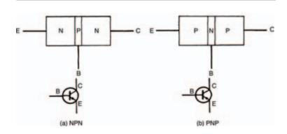
Figure 8.10 The internal construction and circuit symbols for NPN and PNP transistors
