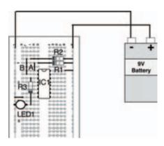
Figure 10.17 Possible breadboard layout to investigate the circuit of Figure 10.16
