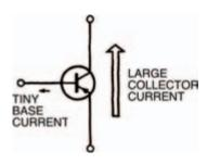
Figure 8.11 An NPN has the same effect as a PNP transistor, but in the opposite direction
