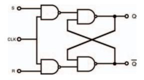
Figure 11.8 A clocked SR-type NAND bistable
