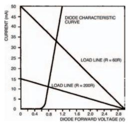
Figure 7.6 This shows the new load line for a resistor of 200  $\Omega$
