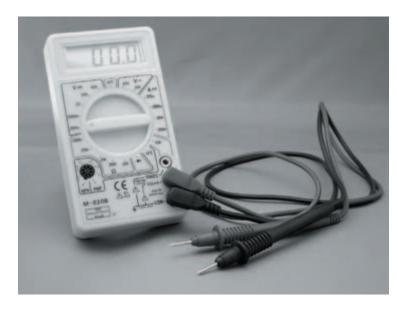
Photo 2.5 A multi-meter — the one used throughout this book — although any multi-meter with at least the specification given will do
