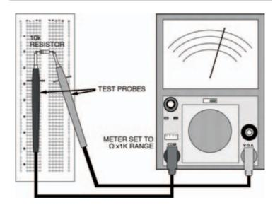
Figure 2.3 About the simplest circuit you could have: a single resistor and a multi-meter. The multi-meter takes the place of a power supply, and the circuit's iob is to test the resistor!
