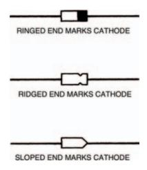
Figure 6.2 Some typical diode body shapes
