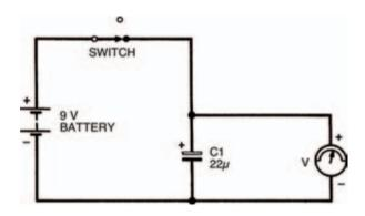
Figure 4.11 An experimental circuit to demonstrate how a capacitor stores voltage (or charge)
