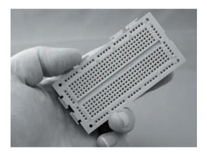
Photo 2.1 A typical breadboard
