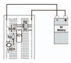
Figure 10.12 Possible breadboard layout for the experimental circuit showing OR gate operation in Figure 10.11
