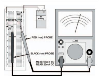
Figure 6.10 The same circuit, set up to measure the current through the diode
