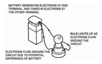
Figure 1.3 A battery forces electrons around a circuit, only when the circuit is complete. If it's not connected (see Figure 1.4 over), no electrons flow — but it still has the potential to make them flow
