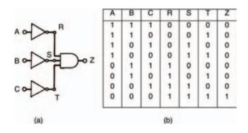
Figure 10.47 A three input AND gate converted to a NOR gate with NOT gates
