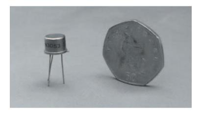
Photo 8.1 A transistor next to a UK fifty pence piece
