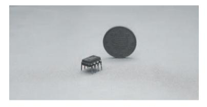
Photo 5.5 The 555, an 8 pin DIL timer IC, beside a UK one penny piece
