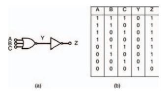
Figure 10.37 (a) using an inverter and a NOR gate to create an OR gate; (b) its truth table to prove this
