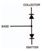
Figure 8.2 A symbol for a transistor considered as two diodes, back to back
