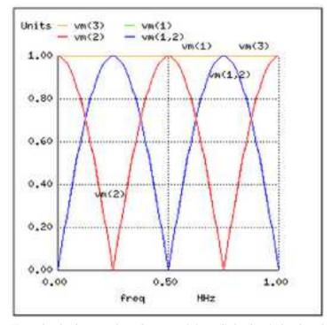
Here, both the supply voltage vm(1) and the line's load-end voltage vm(3) remain steady at 1 volt. The other voltages dip and peak at different frequencies along the sweep range of 1 mHz to 1 MHz. There are five points of interest along the horizontal axis of the analysis: 0 Hz, 250 kHz, 500 kHz, 750 kHz, and 1 MHz. We will investigate each one with regard to voltage and current at different points of the circuit.
