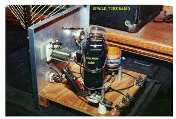
The variable capacitor and air-core inductor shown in the above photograph of a simple radio comprise the main elements in the tank circuit filter used to discriminate one radio station's signal from another.
