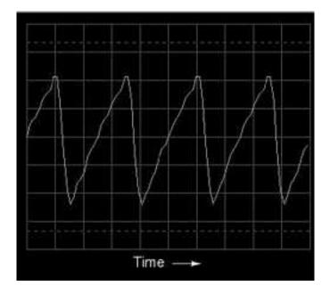
When the spectrum analysis of this waveform is plotted, we see a result that is quite different from that of the regular triangle wave, for this analysis shows the strong presence of even-numbered harmonics (second and fourth):
