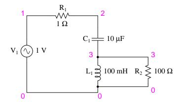
resonant circuit v1 1 0 ac 1 sin r1 1 2 1 c1 2 3 10u l1 3 0 100m r2 3 0 100 .ac lin 20 100 400 .plot ac i(v1) .end
