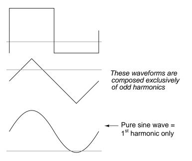
Again, the amount of DC voltage present in a waveform has nothing to do with that waveform's harmonic frequency content.
