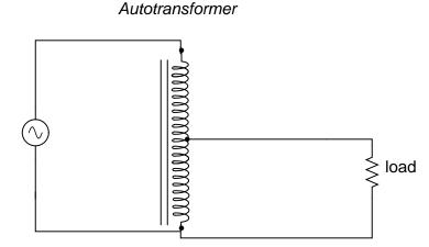
Autotransformers find popular use in applications requiring a slight boost or reduction in voltage to a load. The alternative with a normal (isolated) transformer would be to either have just the right primary/secondary winding ratio made for the job or use a step-down configuration with the secondary winding connected in series-aiding ("boosting") or series-opposing ("bucking") fashion. Primary, secondary, and load voltages are given to illustrate how this would work.
