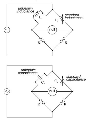
Simple "symmetrical" bridges such as these are so named because they exhibit symmetry (mirrorimage similarity) from left to right. The two bridge circuits shown above are balanced by adjusting the calibrated reactive component ( $L_s$  or  $C_s$ ). They are a bit simplified from their real-life counterparts, as practical symmetrical bridge circuits often have a calibrated, variable resistor in series
