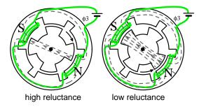
Sequential switching of the stator phases moves the rotor from one position to the next. The mangetic flux seeks the path of least reluctance, the magnetic analog of electric resistance.
