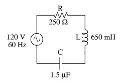
The first step is to determine the reactances (in ohms) for the inductor and the capacitor.
