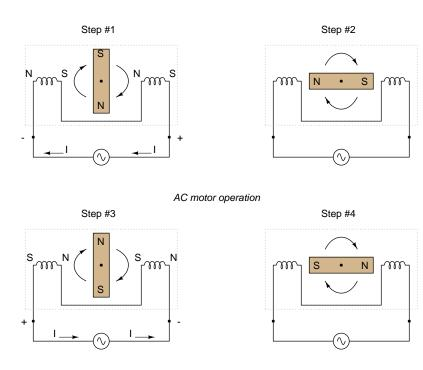
If the rotating magnet is able to keep up with the frequency of the alternating current energizing the electromagnet windings (coils), it will continue to be pulled around clockwise. However, clockwise is not the only valid direction for this motor's shaft to spin. It could just as easily be powered in a counter-clockwise direction by the same AC voltage waveform:
