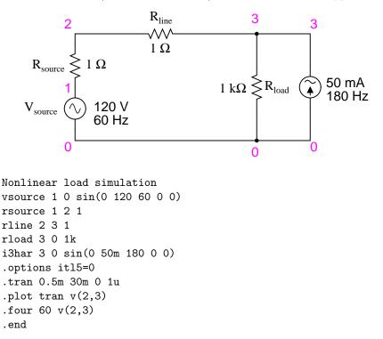
In this circuit, we have a current source of 50 mA magnitude and a frequency of 180 Hz, which is three times the source frequency of 60 Hz. Connected in parallel with the 1 k $\Omega$  load resistor, its current will add with the resistor's to make a nonsinusoidal total line current. I'll show the waveform plot here just so you can see the effects of this 3rd-harmonic current on the total current, which would ordinarily be a plain sine wave:
