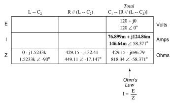
At this point we ask ourselves the question: are there any components or component combinations which share either the total voltage or the total current? In this case, both  $C_1$  and the parallel combination  $R//(L--C_2)$  share the same (total) current, since the total impedance is composed of the two sets of impedances in series. Thus, we can transfer the figure for total current into both columns:
