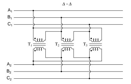
When there is no need for a neutral conductor in the secondary power system,  $\Delta$ - $\Delta$  connection schemes are preferred because of the inherent reliability of the  $\Delta$  configuration.
