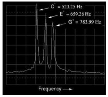
The spectrum display (frequency-domain) is much easier to interpret: each pitch is represented
