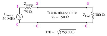
We can specify the cable length in SPICE in terms of time delay from beginning to end. Since the frequency is 50 MHz, the signal period will be the reciprocal of that, or 20 nano-seconds (20 ns). One-quarter of that time (5 ns) will be the time delay of a transmission line one-quarter wavelength long:
