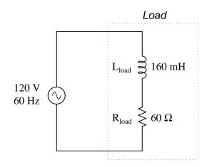
$$\begin{split} X_L &= 60.319 \ \Omega \\ Z_L &= 0 + j60.319 \ \Omega \quad \text{or} \quad 60.319 \ \Omega \not \leq 90^\circ \\ Z_R &= 60 + j0 \ \Omega \quad \text{or} \quad 60 \ \Omega \not \leq 0^\circ \\ Z_{total} &= 60 + j60.319 \ \Omega \quad \text{or} \quad 85.078 \ \Omega \not \leq 45.152^\circ \\ I &= \frac{E}{Z} \\ I &= \frac{120 \ V}{85.078 \ \Omega} \end{split}$$
