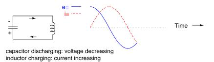
Eventually the capacitor will discharge to zero volts, leaving the inductor fully charged with full current through it:
