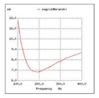
Switching our attention to series LC circuits, we experiment with placing significant resistances in parallel with either L or C. In the following series circuit examples, a 1  $\Omega$  resistor (R<sub>1</sub>) is placed in series with the inductor and capacitor to limit total current at resonance. The "extra" resistance inserted to influence resonant frequency effects is the 100  $\Omega$  resistor, R<sub>2</sub>: Series LC with resistance in parallel with L
