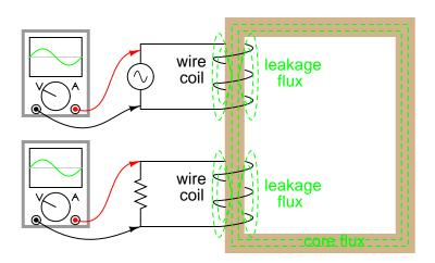
Consequently, this "leakage" flux merely stores and returns energy to the source circuit via selfinductance, effectively acting as a series impedance in both primary and secondary circuits. Voltage gets dropped across this series impedance, resulting in a reduced load voltage: voltage across the load "sags" as load current increases.
