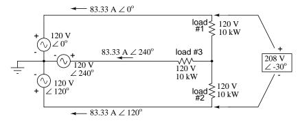
A full mathematical analysis of all the voltages and currents in this circuit would necessitate the use of a network theorem, the easiest being the Superposition Theorem. I'll spare you the long, drawn-out calculations because you should be able to intuitively understand that the three voltage sources at three different phase angles will deliver 120 volts each to a balanced triad of load resistors. For proof of this, we can use SPICE to do the math for us:
