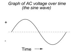
In the voltage plot from an electromechanical alternator, the change from one polarity to the other is a smooth one, the voltage level changing most rapidly at the zero ("crossover") point and most slowly at its peak. If we were to graph the trigonometric function of "sine" over a horizontal range of 0 to 360 degrees, we would find the exact same pattern:
