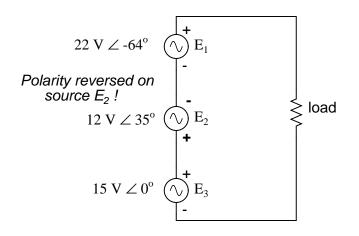
Note how the 12 volt supply's phase angle is still referred to as  $35^{\circ}$ , even though the leads have been reversed. Remember that the phase angle of any voltage drop is stated in reference to its noted polarity. Even though the angle is still written as  $35^{\circ}$ , the vector will be drawn  $180^{\circ}$  opposite of what it was before:
