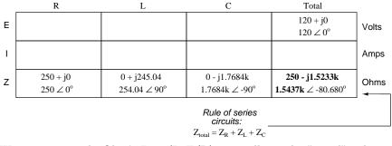
We can now apply Ohm's Law (I=E/R) vertically in the "Total" column to find total current for this series circuit:
