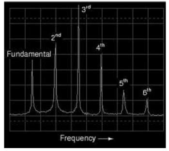
Indeed we do! The fundamental frequency component of 523.25 Hz is represented by the left-most peak, with each successive harmonic represented as its own peak along the width of the analyzer screen. The second harmonic is twice the frequency of the fundamental (1046.5 Hz), the third harmonic three times the fundamental (1569.75 Hz), and so on. This display only shows the first six harmonics, but there are many more comprising this complex tone.
