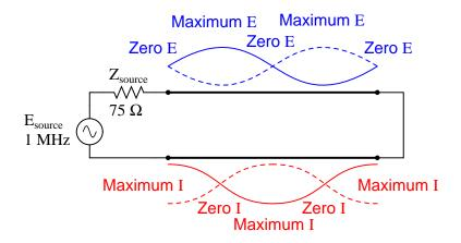
In both these circuit examples, an open-circuited line and a short-circuited line, the energy reflection is total: 100% of the incident wave reaching the line's end gets reflected back toward the source. If, however, the transmission line is terminated in some impedance other than an open or a short, the reflections will be less intense, as will be the difference between minimum and maximum values of voltage and current along the line.
