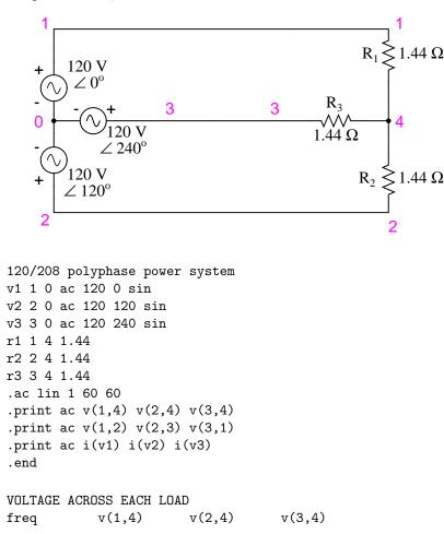
6.000E+01 1.200E+02 1.200E+02 1.200E+02 VOLTAGE BETWEEN "HOT" CONDUCTORS freq v(1,2)v(2,3) v(3,1)6.000E+01 2.078E+02 2.078E+02 2.078E+02 CURRENT THROUGH EACH VOLTAGE SOURCE freq i(v1) i(v2) i(v3) 6.000E+01 8.333E+01 8.333E+01 8.333E+01
