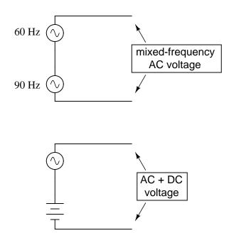
Some computer communications networks operate on the principle of superimposing high-frequency voltage signals along 60 Hz power-line conductors, so as to convey computer data along existing lengths of power cabling. This technique has been used for years in electric power distribution networks to communicate load data along high-voltage power lines. Certainly these are examples of mixed-frequency AC voltages, under conditions that are deliberately established.
