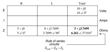
Now that we know total voltage and total impedance, we can apply Ohm's Law (I=E/Z) to determine total current:
