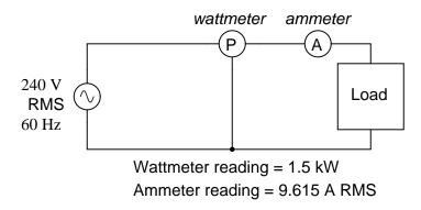
First, we need to calculate the apparent power in kVA. We can do this by multiplying load voltage by load current:
