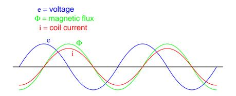
Let us suppose that the primary winding of a transformer is suddenly connected to an AC voltage source at the exact moment in time when the instantaneous voltage is at its positive peak value. In order for the transformer to create an opposing voltage drop to balance against this applied source voltage, a magnetic flux of rapidly increasing value must be generated. The result is that winding current increases rapidly, but actually no more rapidly than under normal conditions:
