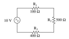
$R_{total} = R_1 + R_2 + R_3$  $R_{total} = 1 k\Omega$  $I_{total} = \frac{E_{total}}{R_{total}}$  $I_{total} = \frac{10 V}{1 k\Omega}$  $I_{total} = 10 mA$
