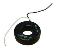
Some CTs are made to hinge open, allowing insertion around a power conductor without disturbing the conductor at all. The industry standard secondary current for a CT is a range of 0 to 5 amps AC. Like PTs, CTs can be made with custom winding ratios to fit almost any application. Because their "full load" secondary current is 5 amps, CT ratios are usually described in terms of full-load primary amps to 5 amps, like this:
