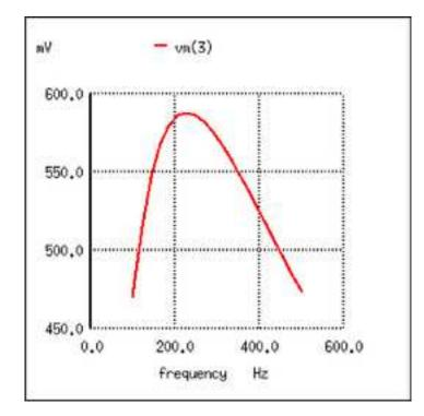
capacitive bandpass filter Load voltage peaks within narrow frequency range
