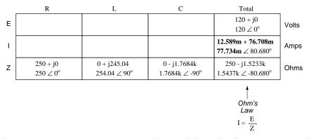
Being a series circuit, current must be equal through all components. Thus, we can take the figure obtained for total current and distribute it to each of the other columns:
