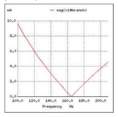
Incidentally, the graph output produced by this SPICE computer analysis is more generally known as a *Bode plot*. Such graphs plot amplitude or phase shift on one axis and frequency on the other. The steepness of a Bode plot curve characterizes a circuit's "frequency response," or how sensitive it is to changes in frequency.
