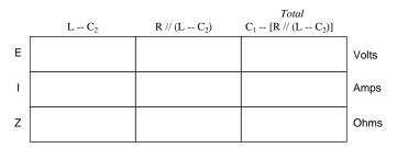
Calculating these new (combination) impedances will require complex addition for series combinations, and the "reciprocal" formula for complex impedances in parallel. This time, there is no avoidance of the reciprocal formula: the required figures can be arrived at no other way!
