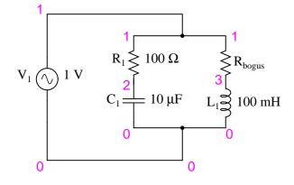
Here, an extra resistor  $(R_{bogus})$  is necessary to prevent SPICE from encountering trouble in analysis. SPICE can't handle an inductor connected directly in parallel with any voltage source or any other inductor, so the addition of a series resistor is necessary to "break up" the voltage
