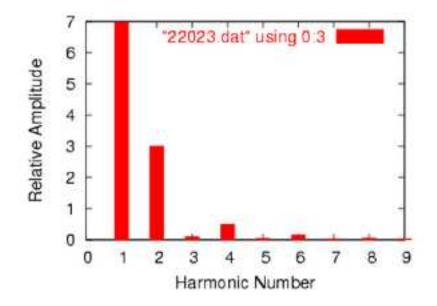
Notice the relatively large even-multiple harmonics in this analysis. By cutting out half of our AC wave, we've introduced the equivalent of several higher-frequency sinusoidal (actually, cosine) waveforms into our circuit from the original, pure sine-wave. Also take note of the large DC component: 4.456 volts. Because our AC voltage waveform has been "rectified" (only allowed to push in one direction across the load rather than back-and-forth), it behaves a lot more like DC.
