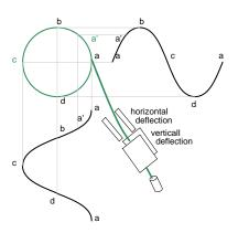
Above we illustrate that the two  $90^{\circ}$  phase shifted sine waves are applied to oscilloscope deflection plates which are at right angles in space. If this were not the case, a one dimensional line would display. The combination of  $90^{\circ}$  phased sine waves and right angle deflection, results in a two dimensional pattern– a circle. This circle is traced out by a counterclockwise rotating spot.
