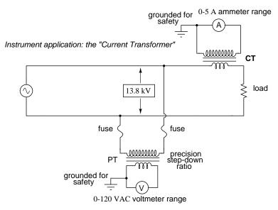
Note that while the PT is a step-down device, the *Current Transformer* (or CT) is a step-up device (with respect to voltage), which is what is needed to step *down* the power line current. Quite often, CTs are built as donut-shaped devices through which the power line conductor is run, the power line itself acting as a single-turn primary winding:
