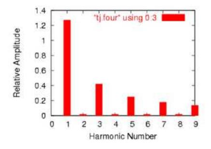
Notice how this analysis shows less of a DC component voltage and lower amplitudes for each of the even harmonic frequency sine waves, all because we let the computer sample more cycles of the wave. Again, the imprecision of the first analysis is not so much a flaw in SPICE as it is a fundamental property of waves and of signal analysis.
