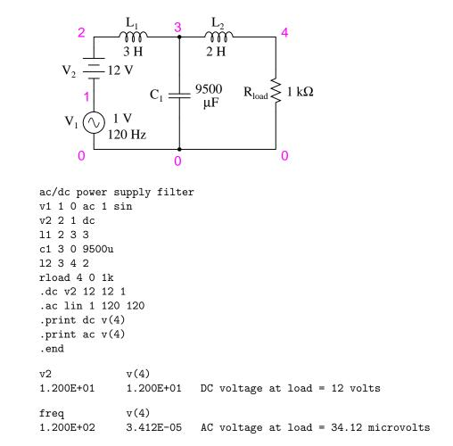
With a full 12 volts DC at the load and only 34.12  $\mu$ V of AC left from the 1 volt AC source imposed across the load, this circuit design proves itself to be a very effective power supply filter.
