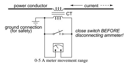
Though it may seem strange to *intentionally* short-circuit a power system component, it is perfectly proper and quite necessary when working with current transformers.
