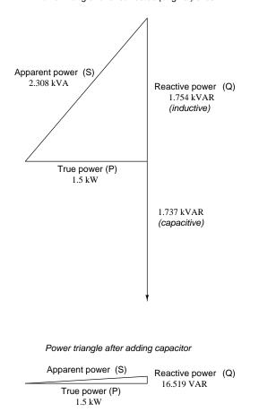
Power triangle for uncorrected (original) circuit
