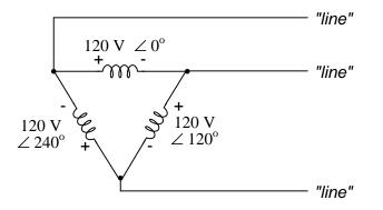
At first glance it seems as though three voltage sources like this would create a short-circuit, electrons flowing around the triangle with nothing but the internal impedance of the windings to hold them back. Due to the phase angles of these three voltage sources, however, this is not the case.
