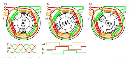
While the variable reluctance motor is simple, even more so than an induction motor, it is difficult to control. Electronic control solves this problem and makes it practical to drive the motor well above and below the power line frequency. A variable reluctance motor driven by a *servo*, an electronic feedback system, controls torque and speed, minimizing ripple torque.
