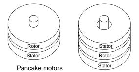
High torque pancake motors may have stator coils on both sides of the rotor as above right. Lower torque applications like floppy disk drive motors suffice with a stator coils on one side of the rotor, above left. The direction of the magnetic flux is axial, that is, parallel to the axis of rotation.
