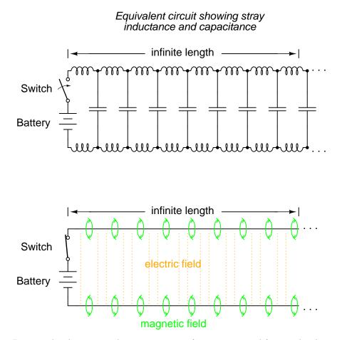
Because the electrons in the two wires transfer motion to and from each other at nearly the speed of light, the "wave front" of voltage and current change will propagate down the length of the wires at that same velocity, resulting in the distributed capacitance and inductance progressively charging to full voltage and current, respectively, like this:
