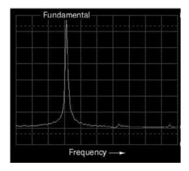
As you can see, the horizontal axis of the display is marked with the word "Frequency," denoting the domain of this measurement. The single peak on the curve represents the predominance of a single frequency within the range of frequencies covered by the width of the display. If the scale of this analyzer instrument were marked with numbers, you would see that this peak occurs at 523.25 Hz. The height of the peak represents the signal amplitude (voltage).
