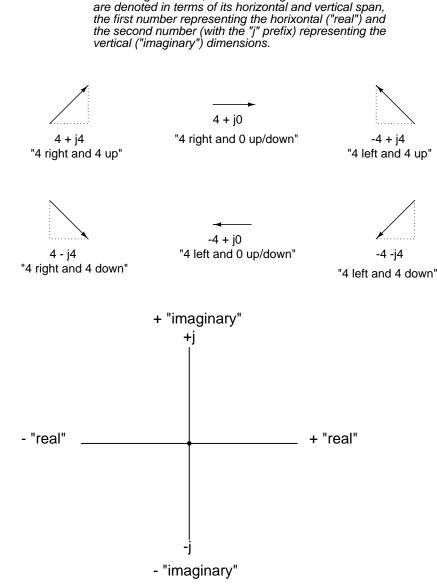
The horizontal component is referred to as the *real* component, since that dimension is compatible with normal, scalar ("real") numbers. The vertical component is referred to as the *imaginary* component, since that dimension lies in a different direction, totally alien to the scale of the real
