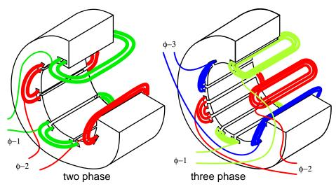
Above, the windings for both a two-phase motor and a three-phase motor have been installed in the stator slots. The coils are wound on an external fixture, then worked into the slots. Insulation wedged between the coil periphery and the slot protects against abrasion.
