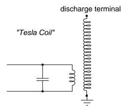
The capacitor, in conjunction with the transformer's primary winding, forms a tank circuit. The secondary winding is wound in close proximity to the primary, usually around the same nonmagnetic form. Several options exist for "exciting" the primary circuit, the simplest being a high-voltage, low-frequency AC source and spark gap:
