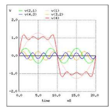
Here we can see the wave becoming flatter at each peak. Finally, adding the 9th harmonic, the fifth sine wave voltage source in our circuit, we obtain this result:
