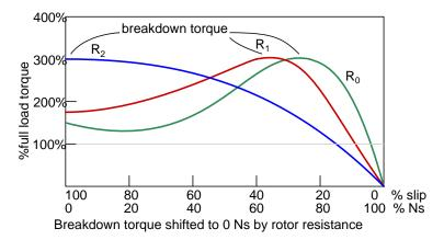
The resistance decreases the torque available at full running speed. But that resistance is shorted out by the time the rotor is started. A shorted rotor operates like a squirrel cage rotor. Heat generated during starting is mostly dissipated external to the motor in the starting resistance. The complication and maintenance associated with brushes and slip rings is a disadvantage of the wound rotor as compared to the simple squirrel cage rotor.
