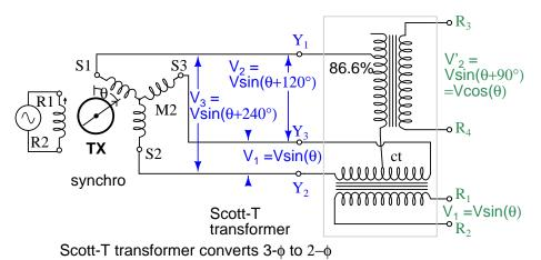
It is possible to derive resolver-like quadrature angular components from a synchro transmitter
