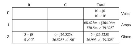
Current in a series circuit is shared equally by all components, so the figures placed in the "Total" column for current can be distributed to all other columns as well:
