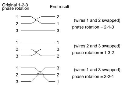
No matter which pair of "hot" wires out of the three we choose to swap, the phase rotation ends up being reversed (1-2-3 gets changed to 2-1-3, 1-3-2 or 3-2-1, all equivalent).
