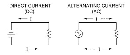
Whereas the familiar battery symbol is used as a generic symbol for any DC voltage source, the circle with the wavy line inside is the generic symbol for any AC voltage source.
