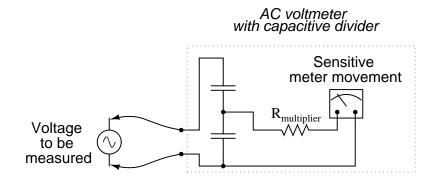
If the meter movement is electrostatic, and thus inherently capacitive in nature, a single "multiplier" capacitor may be connected in series to give it a greater voltage measuring range, just as a series-connected multiplier resistor gives a moving-coil (inherently resistive) meter movement a greater voltage range:
