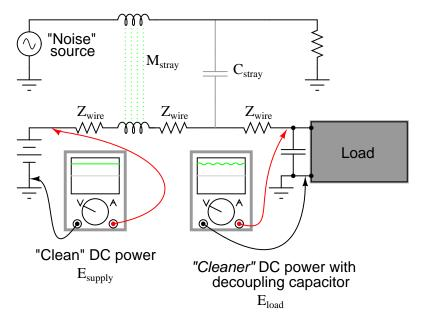
A cursory glance at a crowded printed-circuit board (PCB) will typically reveal decoupling capacitors scattered throughout, usually located as close as possible to the sensitive DC loads. Capacitor size is usually 0.1  $\mu$ F or more, a minimum amount of capacitance needed to produce a low enough impedance to short out any noise. Greater capacitance will do a better job at filtering noise, but size and economics limit decoupling capacitors to meager values.
