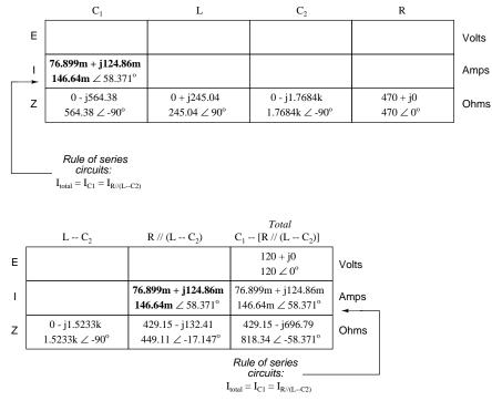
Now, we can calculate voltage drops across  $C_1$  and the series-parallel combination of  $R//(L--C_2)$  using Ohm's Law (E=IZ) vertically in those table columns:
