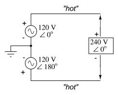
To mathematically calculate voltage between "hot" wires, we must *subtract* voltages, because their polarity marks show them to be opposed to each other:
