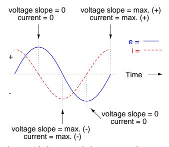
As you might have guessed, the same unusual power wave that we saw with the simple inductor circuit is present in the simple capacitor circuit, too:
