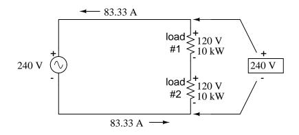
Notice the polarity markings (+ and -) for each voltage shown, as well as the unidirectional arrows for current. For the most part, I've avoided labeling "polarities" in the AC circuits we've been analyzing, even though the notation is valid to provide a frame of reference for phase. In later sections of this chapter, phase relationships will become very important, so I'm introducing this notation early on in the chapter for your familiarity.
