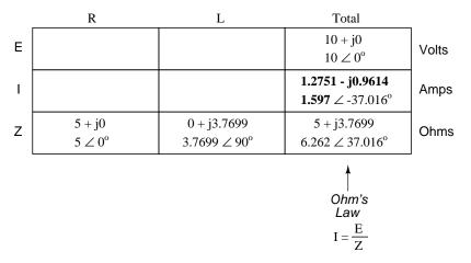
Just as with DC, the total current in a series AC circuit is shared equally by all components. This is still true because in a series circuit there is only a single path for electrons to flow, therefore the rate of their flow must uniform throughout. Consequently, we can transfer the figures for current into the columns for the resistor and inductor alike:
