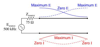
At 750 kHz, the plot looks a lot like it was at 250 kHz: zero source-end voltage (vm(2)) and maximum current (vm(1,2)). This is due to 3/4 of a wave poised along the transmission line, resulting in the source "seeing" a short-circuit where it connects to the transmission line, even though the other end of the line is open-circuited:
