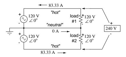
$$E_{total} = (120 \text{ V} \angle 0^{\circ}) + (120 \text{ V} \angle 0^{\circ})$$
