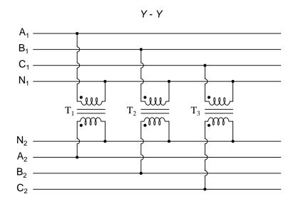
Note how all the winding ends marked with dots are connected to their respective phases A, B, and C, while the non-dot ends are connected together to form the centers of each "Y". Having both primary and secondary winding sets connected in "Y" formations allows for the use of neutral conductors  $(N_1 \text{ and } N_2)$  in each power system.
