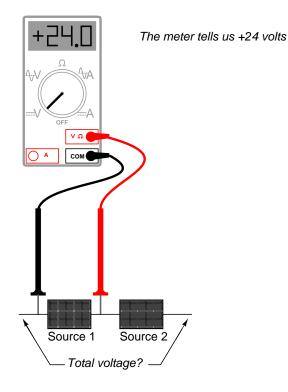
This first measurement of +24 across the left-hand voltage source tells us that the black lead of the meter really is touching the negative side of voltage source #1, and the red lead of the meter really is touching the positive. Thus, we know source #1 is a battery facing in this orientation:
