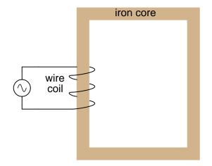
As an inductor, we would expect this iron-core coil to oppose the applied voltage with its inductive reactance, limiting current through the coil as predicted by the equations  $X_L = 2\pi fL$  and I=E/X (or I=E/Z). For the purposes of this example, though, we need to take a more detailed look at the interactions of voltage, current, and magnetic flux in the device.
