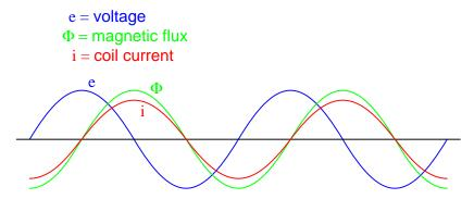
This is why alternating current through an inductor lags the applied voltage waveform by 90°: because that is what is required to produce a changing magnetic flux whose rate-of-change produces an opposing voltage in-phase with the applied voltage. Due to its function in providing magnetizing force (mmf) for the core, this current is sometimes referred to as the magnetizing current.
