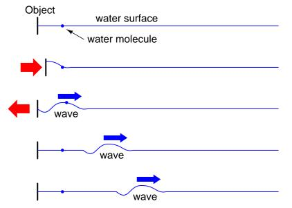
Likewise, electron motion "coupling" travels approximately at the speed of light, although the electrons themselves don't move that quickly. In a very long circuit, this "coupling" speed would
