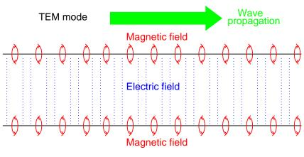
Both field planes perpendicular (transverse) to direction of signal propagation.
