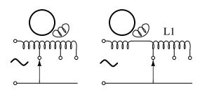
Speed control of shaded pole motor
