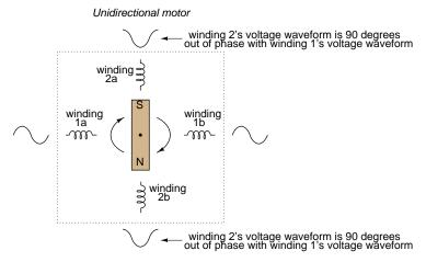
These supplementary coils are typically connected in series with a capacitor to introduce a phase shift in current between the two sets of windings:
