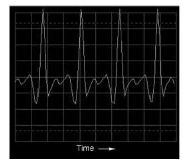
The fundamental frequency of this tone is the same as in the first panflute example: 523.25 Hz, one octave above "middle C." The waveform itself is far from a pure and simple sine-wave form. Knowing that any repeating, non-sinusoidal waveform is equivalent to a series of sinusoidal waveforms at different amplitudes and frequencies, we should expect to see multiple peaks on the spectrum analyzer display:
