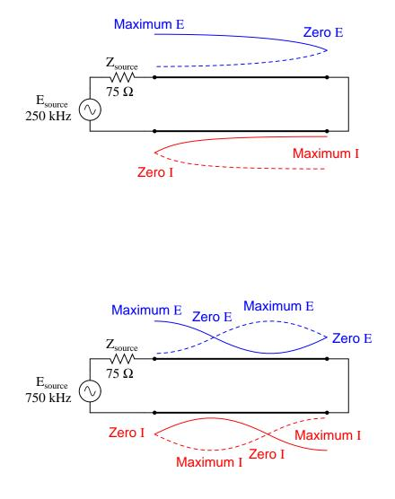
At these frequencies, the transmission line is actually functioning as an *impedance transformer*, transforming an infinite impedance into zero impedance, or vice versa. Of course, this only occurs at resonant points resulting in a standing wave of 1/4 cycle (the line's fundamental, resonant frequency) or some odd multiple  $(3/4, 5/4, 7/4, 9/4 \dots)$ , but if the signal frequency is known and unchanging, this phenomenon may be used to match otherwise unmatched impedances to each other.
