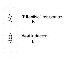
It is worthy to note that the skin effect and radiation losses apply just as well to straight lengths of wire in an AC circuit as they do a coiled wire. Usually their combined effect is too small to notice, but at radio frequencies they can be quite large. A radio transmitter antenna, for example, is designed with the express purpose of dissipating the greatest amount of energy in the form of electromagnetic radiation.
