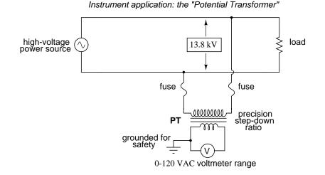
Now the voltmeter reads a precise fraction, or ratio, of the actual system voltage, its scale set to read as though it were measuring the voltage directly. The transformer keeps the instrument voltage at a safe level and electrically isolates it from the power system, so there is no direct connection between the power lines and the instrument or instrument wiring. When used in this capacity, the transformer is called a *Potential Transformer*, or simply *PT*.
