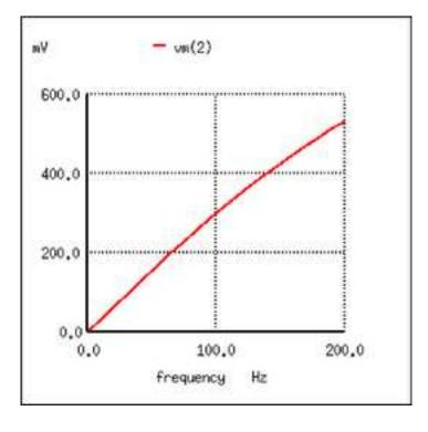
capacitive highpass filter Load voltage increases with increasing frequency
