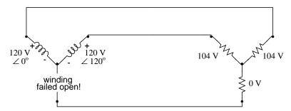
In this case, two load resistances suffer reduced voltage while the third loses supply voltage completely! For this reason,  $\Delta$ -connected sources are preferred for reliability. However, if dual voltages are needed (e.g. 120/208) or preferred for lower line currents, Y-connected systems are the configuration of choice.
