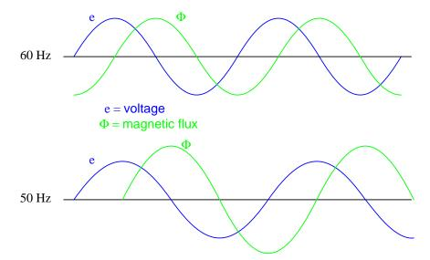
Since instantaneous winding voltage is proportional to the instantaneous magnetic flux's *rate* of change in a transformer, a voltage waveform reaching the same peak value, but taking a longer amount of time to complete each half-cycle, demands that the flux maintain the same rate of change as before, but for longer periods of time. Thus, if the flux has to climb at the same rate as before, but for longer periods of time, it will climb to a greater peak value.
