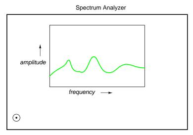
Like an oscilloscope, the spectrum analyzer uses a CRT (or a computer display mimicking a CRT) to display a plot of the signal. Unlike an oscilloscope, this plot is amplitude over *frequency* rather than amplitude over *time*. In essence, a frequency analyzer gives the operator a Bode plot of the signal: something an engineer might call a *frequency-domain* rather than a *time-domain* analysis.
