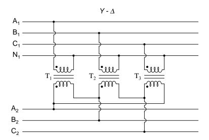
Note how the secondary windings (bottom set) are connected in a chain, the "dot" side of one winding connected to the "non-dot" side of the next, forming the  $\Delta$  loop. At every connection point between pairs of windings, a connection is made to a line of the second power system (A, B, and C).
