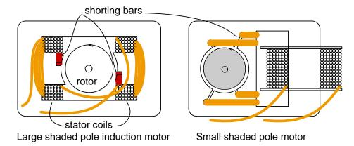
Starting torque is so low that shaded pole motors are only manufactured in smaller sizes, below 50 watts. Low cost and simplicity suit this motor to small fans, air circulators, and other low torque applications. Motor speed can be lowered by switching reactance in series to limit current and torque, or by switching motor coil taps as below
