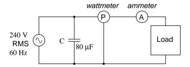
An 80  $\mu$ F capacitor will have a capacitive reactance of 33.157  $\Omega$ , giving a current of 7.238 amps, and a corresponding reactive power of 1.737 kVAR (for the capacitor *only*). Since the capacitor's current is 180° out of phase from the the load's inductive contribution to current draw, the capacitor's reactive power will directly subtract from the load's reactive power, resulting in:
