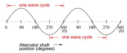
Since the horizontal axis of this graph can mark the passage of time as well as shaft position in degrees, the dimension marked for one cycle is often measured in a unit of time, most often seconds or fractions of a second. When expressed as a measurement, this is often called the *period* of a wave. The period of a wave in degrees is *always* 360, but the amount of time one period occupies depends on the rate voltage oscillates back and forth.
