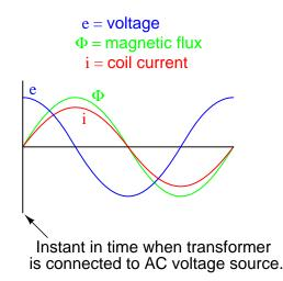
Both core flux and coil current start from zero and build up to the same peak values experienced during continuous operation. Thus, there is no "surge" or "inrush" or current in this scenario.
