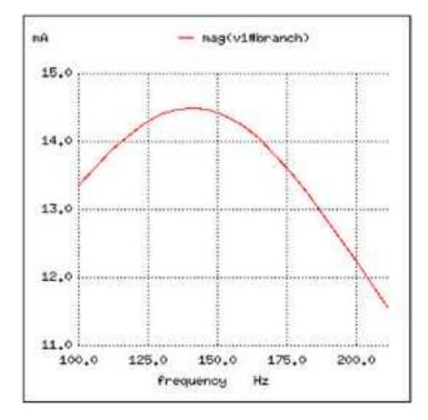
The tendency for added resistance to skew the point at which impedance reaches a maximum or minimum in an LC circuit is called *antiresonance*. The astute observer will notice a pattern between the four SPICE examples given above, in terms of how resistance affects the resonant peak of a circuit:
