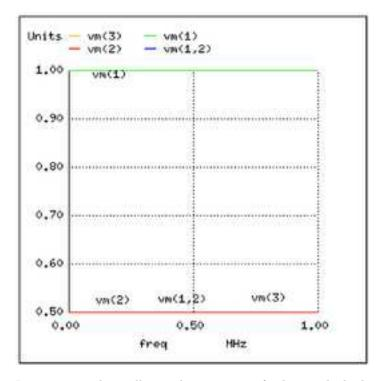
In a system where all impedances are perfectly matched, there can be no standing waves, and therefore no resonant "peaks" or "valleys" in the Bode plot.
