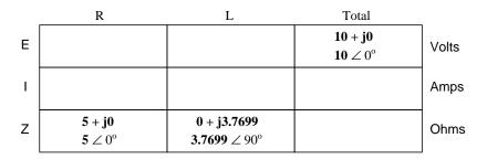
The only difference in our analysis technique this time is that we will apply the rules of parallel circuits instead of the rules for series circuits. The approach is fundamentally the same as for DC. We know that voltage is shared uniformly by all components in a parallel circuit, so we can transfer the figure of total voltage (10 volts  $\angle 0^{\circ}$ ) to all components columns:
