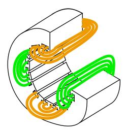
This type of motor may have coils embedded into the stator as shown above for larger size motors. The smaller sizes may use the less complex to build salient pole design.
