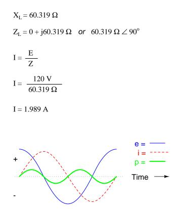
Note that the power alternates equally between cycles of positive and negative. This means that power is being alternately absorbed from and returned to the source. If the source were a mechanical generator, it would take (practically) no net mechanical energy to turn the shaft, because no power would be used by the load. The generator shaft would be easy to spin, and the inductor would not become warm as a resistor would.
