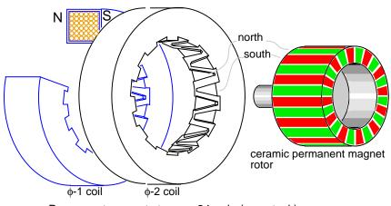
Permanent magnet stepper, 24-pole (can-stack)
