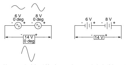
Please note the (+) and (-) polarity marks next to the leads of the two AC sources. Even though we know AC doesn't have "polarity" in the same sense that DC does, these marks are essential to knowing how to reference the given phase angles of the voltages. This will become more apparent in the next example.
