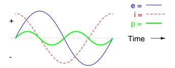
As with the simple inductor circuit, the 90 degree phase shift between voltage and current results in a power wave that alternates equally between positive and negative. This means that a capacitor does not dissipate power as it reacts against changes in voltage; it merely absorbs and releases power, alternately.
