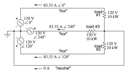
So long as the loads remain balanced (equal resistance, equal currents), the neutral wire will not have to carry any current at all. It is there just in case one or more load resistors should fail open (or be shut off through a disconnecting switch).
