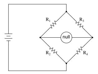
Any one of the four resistors in the above bridge can be the resistor of unknown value, and its value can be determined by a ratio of the other three, which are "calibrated," or whose resistances are known to a precise degree. When the bridge is in a balanced condition (zero voltage as indicated by the null detector), the ratio works out to be this:
