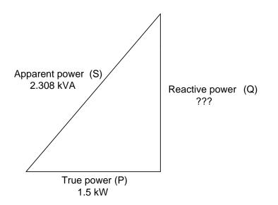
To determine the unknown (reactive power) triangle quantity, we use the Pythagorean Theorem "backwards," given the length of the hypotenuse (apparent power) and the length of the adjacent side (true power):
