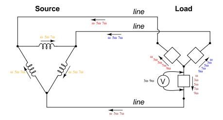
Triplen voltages appear across load phases. Non-triplen currents appear in line conductors and in source phase windings.
