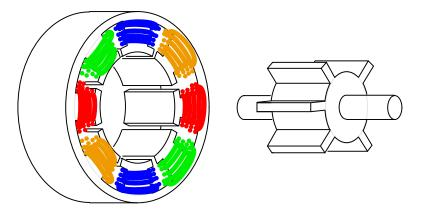
Above, we show the internal construction of a variable reluctance stepper motor. The rotor has protruding poles so that they may be attracted to the rotating stator field as it is switched. An actual motor, is much longer than our simplified illustration. The shaft is frequently fitted with a drive screw, below.
