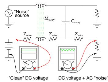
When stray AC voltages from a "noise" source mix with DC signals conducted along signal wiring, the results are usually undesirable. For this reason, power wiring and low-level signal wiring should *always* be routed through separated, dedicated metal conduit, and signals should be conducted via 2-conductor "twisted pair" cable rather than through a single wire and ground connection:
