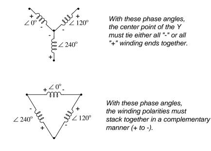
Getting this phasing correct when the windings aren't shown in regular Y or  $\Delta$  configuration can be tricky. Let me illustrate:
