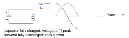
Now we're at a condition very similar to where we started: the capacitor at full charge and zero current in the circuit. The capacitor, as before, will begin to discharge through the inductor, causing an increase in current (in the opposite direction as before) and a decrease in voltage as it depletes its own energy reserve:
