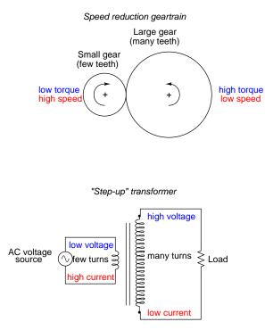
The transformer's ability to step AC voltage up or down with ease gives AC an advantage unmatched by DC in the realm of power distribution. When transmitting electrical power over long distances, it is far more efficient to do so with stepped-up voltages and stepped-down currents (smaller-diameter wire with less resistive power losses), then step the voltage back down and the current back up for industry, business, or consumer use use.
