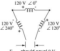
E<sub>break</sub> should equal 0 V
