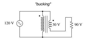
The prime advantage of an autotransformer is that the same boosting or bucking function is obtained with only a single winding, making it cheaper and lighter to manufacture than a regular (isolating) transformer having both primary and secondary windings.
