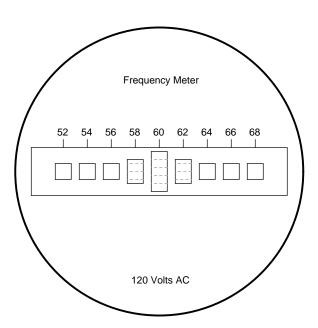
Vibrating reed meters, obviously, are not precision instruments, but they are very simple and therefore easy to manufacture to be rugged. They are often found on small engine-driven generator sets for the purpose of setting engine speed so that the frequency is somewhat close to 60 (50 in Europe) Hertz.
