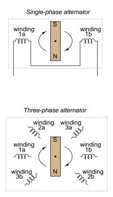
Together, the six "pole" windings of a three-phase alternator are connected to comprise three winding pairs, each pair producing AC voltage with a phase angle  $120^{\circ}$  shifted from either of the other two winding pairs. The interconnections between pairs of windings (as shown for the single-phase alternator: the jumper wire between windings 1a and 1b) have been omitted from the three-phase alternator drawing for simplicity.
