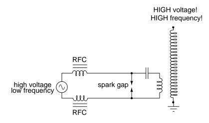
The purpose of the high-voltage, low-frequency AC power source is to "charge" the primary tank circuit. When the spark gap fires, its low impedance acts to complete the capacitor/primary coil tank circuit, allowing it to oscillate at its resonant frequency. The "RFC" inductors are "Radio Frequency Chokes," which act as high impedances to prevent the AC source from interfering with the oscillating tank circuit.
