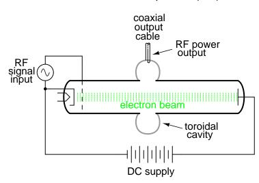
Just as transmission lines are able to function as resonant elements in a circuit, especially when terminated by a short-circuit or an open-circuit, a dead-ended waveguide may also resonate at particular frequencies. When used as such, the device is called a *cavity resonator*. Inductive output tubes use toroid-shaped cavity resonators to maximize the power transfer efficiency between the electron beam and the output cable.
