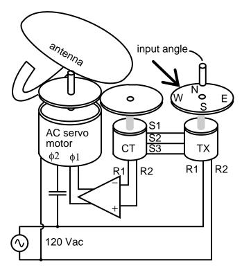
The shaft of the TX is set to the desired position of the radar antenna. The servo system will cause the servo motor to drive the antenna to the commanded position. The CT compares the commanded to actual position and signals the servo amplifier to drive the motor until that commanded angle is achieved.
