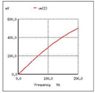
inductive highpass filter Load voltage increases with increasing frequency
