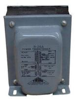
This particular transformer is intended to provide both high and low voltages necessary in an electronic system using vacuum tubes. Low voltage is required to power the filaments of vacuum tubes, while high voltage is required to create the potential difference between the plate and cathode elements of each tube. One transformer with multiple windings suffices elegantly to provide all the
