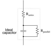
Fortunately, these stray resistances are usually of modest impact (low series resistance and high parallel resistance), much less significant than the stray resistances present in an average inductor.
