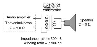
To obtain an impedance transformation ratio of 500:8, we would need a winding ratio equal to the square root of 500:8 (the square root of 62.5:1, or 7.906:1). With such a transformer in place, the speaker will load the amplifier to just the right degree, drawing power at the correct voltage and current levels to satisfy the Maximum Power Transfer Theorem and make for the most efficient power delivery to the load. The use of a transformer in this capacity is called *impedance matching*.
