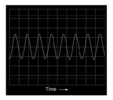
Viewed with an oscilloscope, a sine wave looks like a wavy curve traced horizontally on the screen. The horizontal axis of this oscilloscope display is marked with the word "Time" and an arrow pointing in the direction of time's progression. The curve itself, of course, represents the cyclic increase and decrease of voltage over time.
