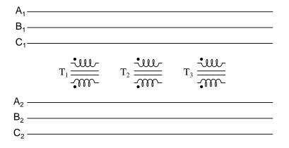
Three individual transformers are to be connected together to transform power from one threephase system to another. First, I'll show the wiring connections for a Y-Y configuration:
