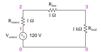
The  $R_{source}$  and  $R_{line}$  resistances in this circuit do more than just mimic the real world: they also provide convenient shunt resistances for measuring currents in the SPICE simulation: by reading voltage across a 1  $\Omega$  resistance, you obtain a direct indication of current through it, since E = IR.
