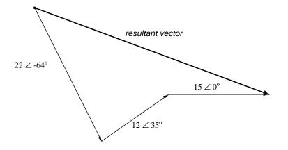
In order to determine what the resultant vector's magnitude and angle are without resorting to graphic images, we can convert each one of these polar-form complex numbers into rectangular form and add. Remember, we're *adding* these figures together because the polarity marks for the three voltage sources are oriented in an additive manner:
