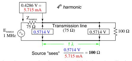
A simple equation relates line impedance  $(Z_0)$ , load impedance  $(Z_{load})$ , and input impedance  $(Z_{input})$  for an unmatched transmission line operating at an odd harmonic of its fundamental frequency:
