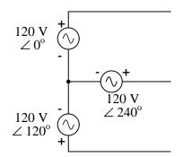
If we draw a circuit showing each voltage source to be a coil of wire (alternator or transformer winding) and do some slight rearranging, the "Y" configuration becomes more obvious:
