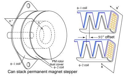
Above is the external package of a can-stack permanent magnet stepper motor.
