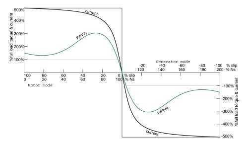
Such an *induction generator* must be excited by a "live" source of 50 or 60 Hz power. No power can be generated in the event of a power company power failure. This type of alternator appears to be unsuited as a standby power source. As an auxiliary power wind turbine generator, it has the advantage of not requiring an automatic power failure disconnect switch to protect repair crews.
