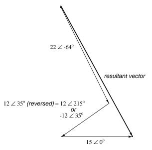
The connection reversal on the 12 volt supply can be represented in two different ways in polar form: by an addition of 180° to its vector angle (making it 12 volts  $\angle 215^{\circ}$ ), or a reversal of sign on the magnitude (making it -12 volts  $\angle 35^{\circ}$ ). Either way, conversion to rectangular form yields the same result:
