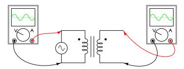
Typically, the transformer will come with some kind of schematic diagram labeling the wire leads for primary and secondary windings. On the diagram will be a pair of dots similar to what is seen above. Sometimes dots will be omitted, but when "H" and "X" labels are used to label transformer winding wires, the subscript numbers are supposed to represent winding polarity. The "1" wires (H<sub>1</sub> and X<sub>1</sub>) represent where the polarity-marking dots would normally be placed.
