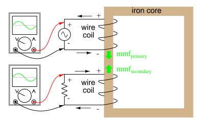
If you find this process a bit confusing, do not worry. Transformer dynamics is a complex subject. What is important to understand is this: when an AC voltage is applied to the primary coil, it creates a magnetic flux in the core, which induces AC voltage in the secondary coil in-phase with the source voltage. Any current drawn through the secondary coil to power a load induces a corresponding current in the primary coil, drawing current from the source.
