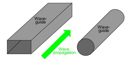
Waveguides are practical only for signals of extremely high frequency, where the wavelength approaches the cross-sectional dimensions of the waveguide. Below such frequencies, waveguides are useless as electrical transmission lines.
