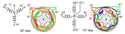
The required stepper drive waveforms for the  $3-\phi$  stepper, above left, can be seen in the "Reluctance motor" section. The drive for a  $4-\phi$  stepper are shown below. Sequentially switching the stator phases produces a rotating magnetic field which the rotor follows. However, due to the lesser number of rotor poles, the rotor moves less than the stator angle for each step. For a variable reluctance stepper motor, the step angle is given by:
