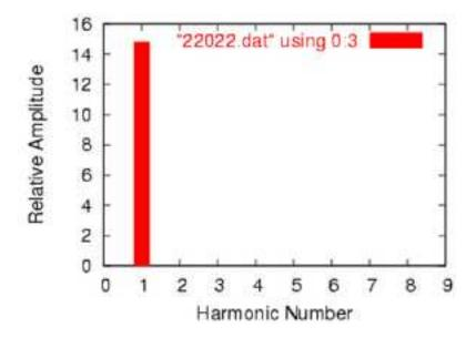
Notice the extremely small harmonic and DC components of this sinusoidal waveform in the table above, though, too small to show on the harmonic plot above. Ideally, there would be nothing but the fundamental frequency showing (being a perfect sine wave), but our Fourier analysis figures aren't perfect because SPICE doesn't have the luxury of sampling a waveform of infinite duration. Next, we'll compare this with the Fourier analysis of the half-wave "rectified" voltage across the load resistor:
