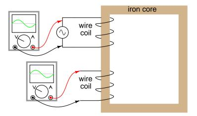
If this secondary coil experiences the same magnetic flux change as the primary (which it should, assuming perfect containment of the magnetic flux through the common core), and has the same number of turns around the core, a voltage of equal magnitude and phase to the applied voltage will be induced along its length. In the following graph, the induced voltage waveform is drawn slightly smaller than the source voltage waveform simply to distinguish one from the other:
