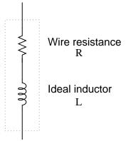
Consequently, the impedance of any real inductor will always be a complex combination of resistance and inductive reactance.
