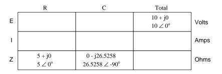
This being a parallel circuit now, we know that voltage is shared equally by all components, so we can place the figure for total voltage (10 volts  $\angle 0^{\circ}$ ) in all the columns:
