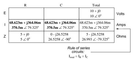
Continuing with our analysis, we can apply Ohm's Law (E=IR) vertically to determine voltage across the resistor and capacitor:
