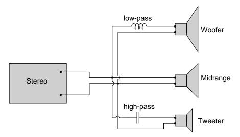
on this stereo system. A real stereo would have six speakers: 2 woofers, 2 midranges, and 2 tweeters.
