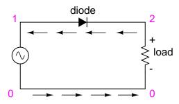
The diode only allows electron flow in a counter-clockwise direction.
