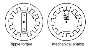
Ripple torque, or cogging caused by the steel pole pieces is illustrated above. Note that there are no stator coils, not even a motor. The PM rotor may be rotated by hand but will encounter
