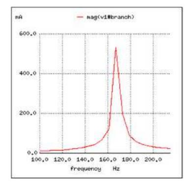
As before, circuit current amplitude increases from left to right, while frequency increases from top to bottom. The peak is still seen to be at the plotted frequency point of 157.9 Hz, the closest analyzed point to our predicted resonance point of 159.155 Hz. This would suggest that our resonant frequency formula holds as true for simple series LC circuits as it does for simple parallel LC circuits, which is the case:
