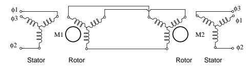
Instrumentation selsyns have no use for starting resistors. They are not intended to be self rotating. Since the rotors are not shorted out nor resistor loaded, no starting torque is developed. However, manual rotation of one shaft will produce an unbalance in the rotor currents until the parallel unit's shaft follows. Though we show three phase rotors above, a single phase rotor is sufficient as shown below. Note that a common source of three phase power is applied to both stators above.
