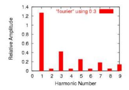
Here, SPICE has broken the waveform down into a spectrum of sinusoidal frequencies up to the ninth harmonic, plus a small DC voltage labelled DC component. I had to inform SPICE of the fundamental frequency (for a square wave with a 20 millisecond period, this frequency is 50 Hz), so it knew how to classify the harmonics. Note how small the figures are for all the even harmonics (2nd, 4th, 6th, 8th), and how the amplitudes of the odd harmonics diminish (1st is largest, 9th is smallest).
