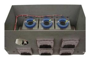
Because of the expense (and often large size) of instrument transformers, they are not used to scale AC meters for any applications other than high voltage and high current. For scaling a milliamp or microamp movement to a range of 120 volts or 5 amps, normal precision resistors (multipliers and shunts) are used, just as with DC.
