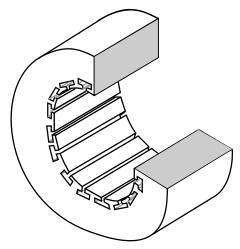
The stator laminations are thin insulated rings with slots punched from sheets of electrical grase steel. A stack of these is secured by end screws, which may also hold the end housings.
