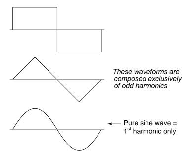
Square waves, triangle waves, and pure sine waves all exhibit this symmetry, and all are devoid of even harmonics. Waveforms like the trumpet tone, the accordion tone, and the sawtooth wave
