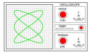
Lissajous figure: Horizontal/Vertical frequency ratio is 3:2
