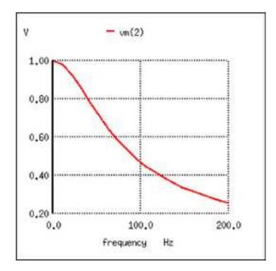
inductive lowpass filter Load voltage decreases with increasing frequency
