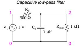
The capacitor's impedance decreases with increasing frequency. This low impedance in parallel with the load resistance tends to short out high-frequency signals, dropping most of the voltage across series resistor  $R_1$ .
