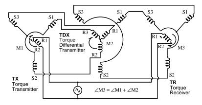
A shipboard radar antenna coupled to a synchro transmitter encodes the antenna angle with respect to ship's bow. It is desired to display the antenna position with respect to true north. We need to add the ships heading from a gyrocompass to the bow-relative antenna position to display antenna angle with respect to true north.  $\angle$  antenna +  $\angle$ gyro
