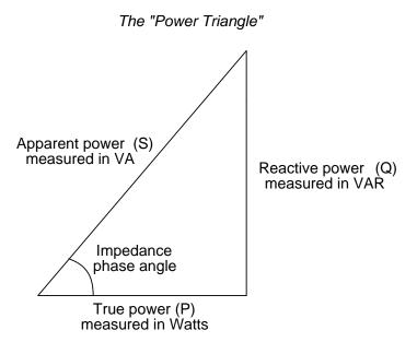
Using the laws of trigonometry, we can solve for the length of any side (amount of any type of power), given the lengths of the other two sides, or the length of one side and an angle.
