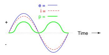
Note that the waveform for power is always positive, never negative for this resistive circuit. This means that power is always being dissipated by the resistive load, and never returned to the source as it is with reactive loads. If the source were a mechanical generator, it would take 240 watts worth of mechanical energy (about 1/3 horsepower) to turn the shaft.
