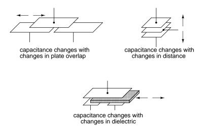
As you can see, all of the differential devices shown in the above illustration have *three* wire connections rather than two: one wire for each of the "end" plates and one for the "common" plate. As the capacitance between one of the "end" plates and the "common" plate changes, the capacitance between the other "end" plate and the "common" plate is such to change in the opposite direction. This kind of transducer lends itself very well to implementation in a bridge circuit:
