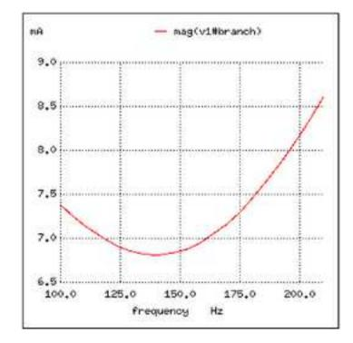
Minimum current at 136.8 Hz instead of 159.2 Hz!
