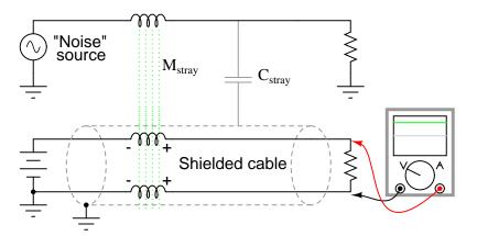
The grounded cable shield – a wire braid or metal foil wrapped around the two insulated conductors – isolates both conductors from electrostatic (capacitive) coupling by blocking any external
