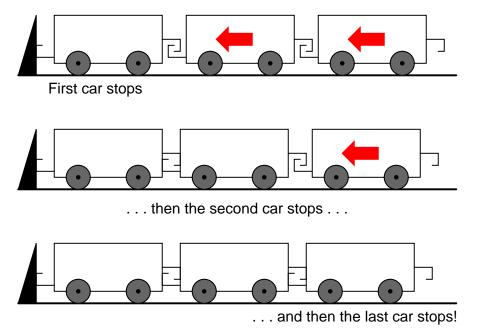
A signal propagating from the source-end of a transmission line to the load-end is called an *incident wave*. The propagation of a signal from load-end to source-end (such as what happened in
