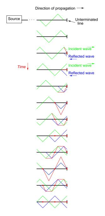
This third, "standing" wave, in fact, represents the only voltage along the line, being the representative sum of incident and reflected voltage waves. It oscillates in instantaneous magnitude, but does not propagate down the cable's length like the incident or reflected waveforms causing it. Note the dots along the line length marking the "zero" points of the standing wave (where the incident
