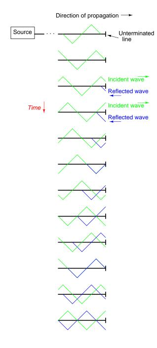
If we add the two waveforms together, we find that a third, stationary waveform is created along the line's length:
