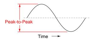
Unfortunately, either one of these expressions of waveform amplitude can be misleading when comparing two different types of waves. For example, a square wave peaking at 10 volts is obviously a greater amount of voltage for a greater amount of time than a triangle wave peaking at 10 volts. The effects of these two AC voltages powering a load would be quite different:
