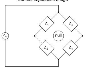
A box with a "Z" written inside is the symbol for any nonspecific impedance.
