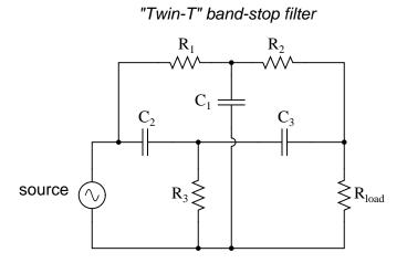
The low-pass filter section is comprised of  $R_1$ ,  $R_2$ , and  $C_1$  in a "T" configuration. The highpass filter section is comprised of  $C_2$ ,  $C_3$ , and  $R_3$  in a "T' configuration as well. Together, this arrangement is commonly known as a "Twin-T" filter, giving sharp response when the component values are chosen in the following ratios:
