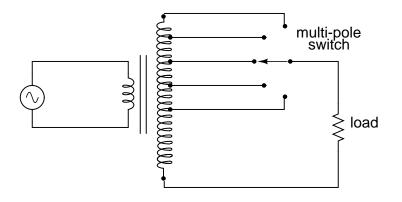
Carrying the concept of winding taps further, we end up with a "variable transformer," where a sliding contact is moved along the length of an exposed secondary winding, able to connect with it at any point along its length. The effect is equivalent to having a winding tap at every turn of the winding, and a switch with poles at every tap position:
