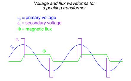
Another cause of abnormal transformer core saturation is operation at frequencies lower than normal. For example, if a power transformer designed to operate at 60 Hz is forced to operate at 50 Hz instead, the flux must reach greater peak levels than before in order to produce the same opposing voltage needed to balance against the source voltage. This is true even if the source voltage is the same as before.
