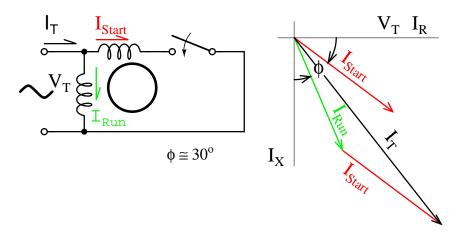
This motor has more starting torque than a shaded pole motor (next section), but not as much as a two phase motor built from the same parts. The current density in the auxiliary winding is so high during starting that the consequent rapid temperature rise precludes frequent restarting or slow starting loads.
