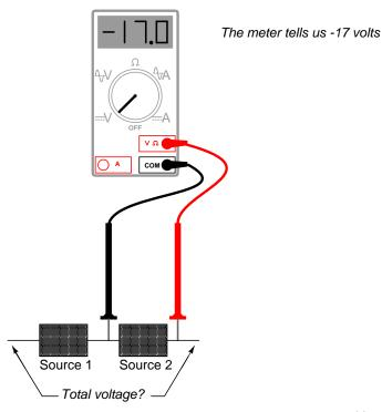
This second voltmeter reading, however, is a *negative* (-) 17 volts, which tells us that the black test lead is actually touching the positive side of voltage source #2, while the red test lead is actually touching the negative. Thus, we know that source #2 is a battery facing in the *opposite* direction:
