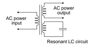
In addition to blocking harmonics created by the saturated core, this resonant circuit also "filters out" harmonic frequencies generated by nonlinear (switching) loads in the secondary winding circuit and any harmonics present in the source voltage, providing "clean" power to the load.
