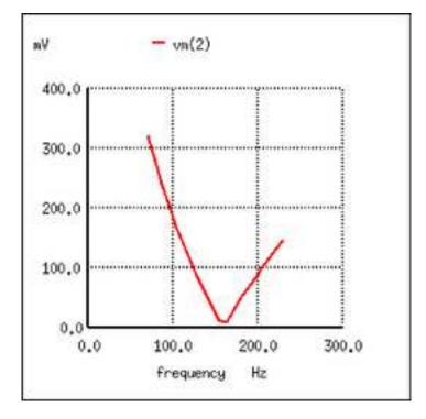
series resonant bandstop filter
