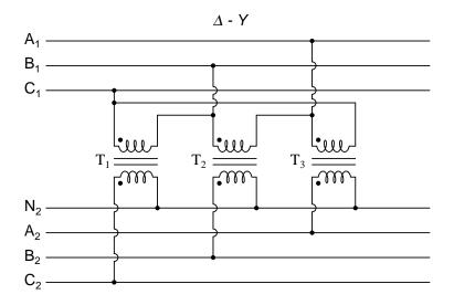
Such a configuration would allow for the provision of multiple voltages (line-to-line or line-toneutral) in the second power system, from a source power system having no neutral.
