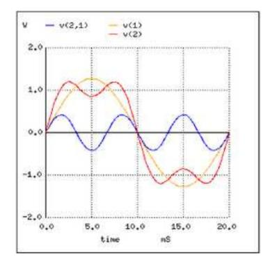
The rise and fall times between positive and negative cycles are much steeper now, and the crests of the wave are closer to becoming flat like a squarewave. Watch what happens as we add the next odd harmonic frequency:
