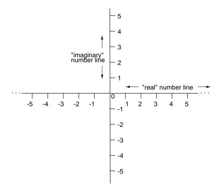
Either method of notation is valid for complex numbers. The primary reason for having two methods of notation is for ease of longhand calculation, rectangular form lending itself to addition and subtraction, and polar form lending itself to multiplication and division.
