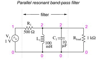
The tank circuit will have a lot of impedance at resonance, allowing the signal to get to the load with minimal attenuation. Under or over resonant frequency, however, the tank circuit will have a low impedance, shorting out the signal and dropping most of it across series resistor  $R_1$ .
