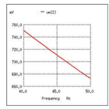
capacitive lowpass filter At 45.26 Hz, the output voltage is above 70.7 percent; At 45.79 Hz, the output voltage is below 70.7 percent; It should be exactly 70.7% at 45.473 Hz!
