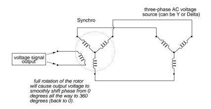
As the synchro's rotor is turned, the rotor coil will progressively align with each stator coil, their respective magnetic fields being  $120^{\circ}$  phase-shifted from one another. In between those positions, these phase-shifted fields will mix to produce a rotor voltage somewhere between  $0^{\circ}$ ,  $120^{\circ}$ , or  $240^{\circ}$  shift. The practical result is a device capable of providing an infinitely variable-phase AC voltage with the twist of a knob (attached to the rotor shaft).
