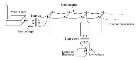
Transformer technology has made long-range electric power distribution practical. Without the ability to efficiently step voltage up and down, it would be cost-prohibitive to construct power systems for anything but close-range (within a few miles at most) use.
