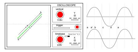
If a pair of  $90^{\circ}$  out of phase sine waves produces a circular Lissajous, a similar pair of currents should be able to produce a circular rotating magnetic field. Such is the case of a 2-phase motor. By analogy three windings placed  $120^{\circ}$  apart in space, and fed with corresponding  $120^{\circ}$  phased currents will also produce a rotating magnetic field.
