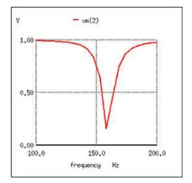
parallel resonant bandstop filter Notch frequency = LC resonant frequency (159.15 Hz)
