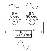
Compared to DC circuit analysis, this is very strange indeed. Note that it's possible to obtain voltmeter indications of 6 and 8 volts, respectively, across the two AC voltage sources, yet only read 10 volts for a total voltage!
