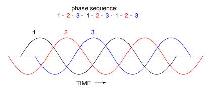
With the three fundamental waveforms equally shifted across the time axis of the graph, it is easy to see how they would cancel each other to give a resultant current of zero in the neutral conductor. Let's consider, though, what a 3rd harmonic waveform for phase 1 would look like superimposed on the graph:
