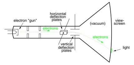
If we allow one AC signal to deflect the beam up and down (connect that AC voltage source to the "vertical" deflection plates) and another AC signal to deflect the beam left and right (using the other pair of deflection plates), patterns will be produced on the screen of the CRT indicative of the *ratio* of these two AC frequencies. These patterns are called *Lissajous figures* and are a common means of comparative frequency measurement in electronics.
