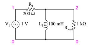
The inductor's impedance decreases with decreasing frequency. This low impedance in parallel tends to short out low-frequency signals from getting to the load resistor. As a consequence, most of the voltage gets dropped across series resistor  $R_1$ .
