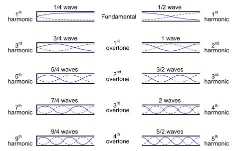
The actual frequencies (measured in Hertz) for any of these harmonics or overtones depends on the physical length of the tube and the waves' propagation velocity, which is the speed of sound in air.
