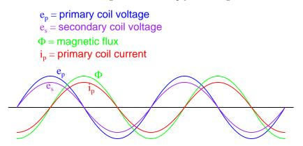
This effect is called *mutual inductance*: the induction of a voltage in one coil in response to a change in current in the other coil. Like normal (self-) inductance, it is measured in the unit of Henrys, but unlike normal inductance it is symbolized by the capital letter "M" rather than the
