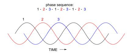
However, if we *reverse* the rotation of the alternator's shaft (turn it counter-clockwise), the magnet will pass by the pole pairs in the opposite sequence. Instead of 1-2-3, we'll have 3-2-1. Now, winding 2's waveform will be *leading*  $120^{\circ}$  ahead of 1 instead of lagging, and 3 will be another  $120^{\circ}$  ahead of 2:
