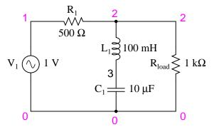
When the series LC combination reaches resonance, its very low impedance shorts out the signal, dropping it across resistor  $R_1$  and preventing its passage on to the load.
