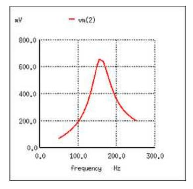
parallel resonant bandpass filter Load voltage peaks at resonant frequency (159.15 Hz)
