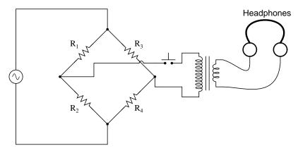
Listening to the headphones as one or more of the resistor "arms" of the bridge is adjusted, a condition of balance will be realized when the headphones fail to produce "clicks" (or tones, if the bridge's power source frequency is within audio range) as the switch is actuated.
