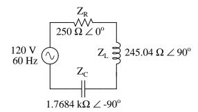
Now, with all quantities of opposition to electric current expressed in a common, complex number format (as impedances, and not as resistances or reactances), they can be handled in the same way as plain resistances in a DC circuit. This is an ideal time to draw up an analysis table for this circuit and insert all the "given" figures (total voltage, and the impedances of the resistor, inductor, and capacitor).
