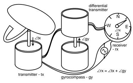
$\angle antenna-N = \angle antenna + \angle gyro$
