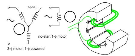
The single coil of a single phase induction motor does not produce a rotating magnetic field, but a pulsating field reaching maximum intensity at  $0^{\circ}$  and  $180^{\circ}$  electrically.
