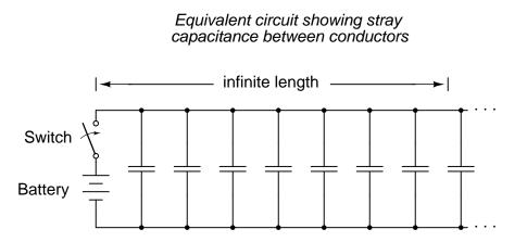
Voltage applied between two conductors creates an electric field between those conductors. Energy is stored in this electric field, and this storage of energy results in an opposition to change in voltage. The reaction of a capacitance against changes in voltage is described by the equation i = C(de/dt), which tells us that current will be drawn proportional to the voltage's rate of change over time. Thus, when the switch is closed, the capacitance between conductors will react against
