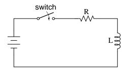
The idea of this circuit is simple: to "charge" the inductor when the switch is closed. The rate of inductor charging will be set by the ratio L/R, which is the time constant of the circuit in seconds. However, if you were to build such a circuit, you might find unexpected oscillations (AC) of voltage across the inductor when the switch is closed. Why is this? There's no capacitor in the circuit, so how can we have resonant oscillation with just an inductor, resistor, and battery?
