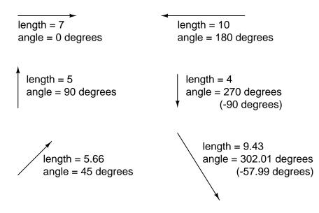
Like distances and directions on a map, there must be some common frame of reference for angle figures to have any meaning. In this case, directly right is considered to be  $0^{\circ}$ , and angles are counted in a positive direction going counter-clockwise:
