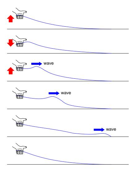
This is analogous to a long transmission line with internal loss: the signal steadily grows weaker as it propagates down the line's length, never reflecting back to the source. However, if the far end of the rope is secured to a solid object at a point prior to the incident wave's total dissipation, a second wave will be reflected back to your hand:
