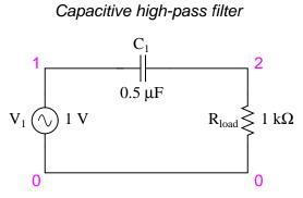
The capacitor's impedance increases with decreasing frequency. This high impedance in series tends to block low-frequency signals from getting to load.
