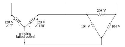
With a  $\Delta$ -connected load, two of the resistances suffer reduced voltage while one remains at the original line voltage, 208. A Y-connected load suffers an even worse fate with the same winding failure in a Y-connected source:
