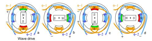
Conceptually, the simplest drive is *wave drive* as illustrated above. The rotation sequence left to right is positive  $\phi$ -1 points rotor north pole up, (+)  $\phi$ -2 points rotor north right, negative  $\phi$ -1 attracts rotor north down, (-)  $\phi$ -2 points rotor left. The wave drive waveforms below show that only one coil is energized at a time. While simple, this does not produce as much torque as other drive techniques.
