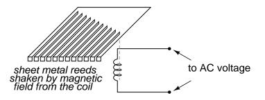
The user of this meter views the ends of all those unequal length reeds as they are collectively shaken at the frequency of the applied AC voltage to the coil. The one closest in resonant frequency to the applied AC will vibrate the most, looking something like this:
