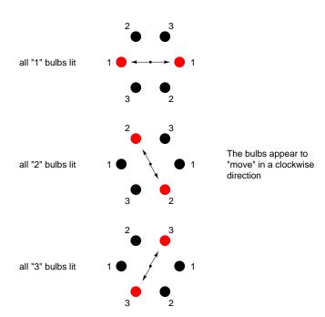
Now the lights appear to be "moving" in a clockwise direction because they are arranged around a circle instead of a straight line. It should come as no surprise that the appearance of motion will reverse if the phase sequence of the bulbs is reversed.
