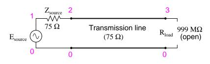
Transmission line v1 1 0 ac 1 sin rsource 1 2 75 t1 2 0 3 0 z0=75 td=1u rload 3 0 999meg .ac lin 101 1m 1meg \* Using "Nutmeg" program to plot analysis .end
