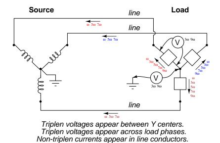
In summary, removal of the neutral conductor leads to a "hot" center-point on the load "Y", and also to harmonic load phase voltages of equal magnitude, all comprised of triplen frequencies. In the previous simulation where we had a 4-wire, Y-connected system, the undesirable effect from harmonics was excessive neutral *current*, but at least each phase of the load received voltage nearly free of harmonics.
