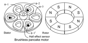
The 3- $\phi$  pancake motor above has 6-stator poles and 8-rotor poles. The rotor is a flat ferrite ring magnetized with eight axially magnetized alternating poles. We do not show that the rotor is capped by a mild steel plate for mounting to the bearing in the middle of the stator. The steel plate also helps complete the magnetic circuit. The stator poles are also mounted atop a steel plate,
