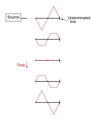
Standing waves are quite abundant in the physical world. Consider a string or rope, shaken at one end, and tied down at the other (only one half-cycle of hand motion shown, moving downward):
