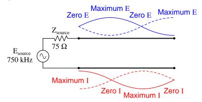
When the supply frequency sweeps up to 1 MHz, a full standing wave exists on the transmission line. At this point, the source-end of the line experiences the same voltage and current amplitudes as the load-end: full voltage and zero current. In essence, the source "sees" an open circuit at the point where it connects to the transmission line.
