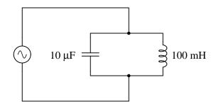
In the above circuit, we have a 10  $\mu$ F capacitor and a 100 mH inductor. Since we know the equations for determining the reactance of each at a given frequency, and we're looking for that point where the two reactances are equal to each other, we can set the two reactance formulae equal to each other and solve for frequency algebraically:
