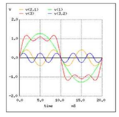
The most noticeable change here is how the crests of the wave have flattened even more. There are more several dips and crests at each end of the wave, but those dips and crests are smaller in amplitude than they were before. Watch again as we add the next odd harmonic waveform to the mix:
