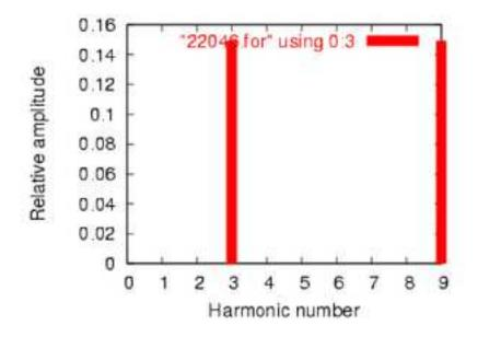
This is a balanced Y-Y power system, each phase identical to the single-phase AC system simulated earlier. Consequently, it should come as no surprise that the Fourier analysis for line current in one phase of the 3-phase system is nearly identical to the Fourier analysis for line current in the single-phase system: a fundamental (60 Hz) line current of 0.1198 amps, and odd harmonic currents of approximately 50 mA each.
