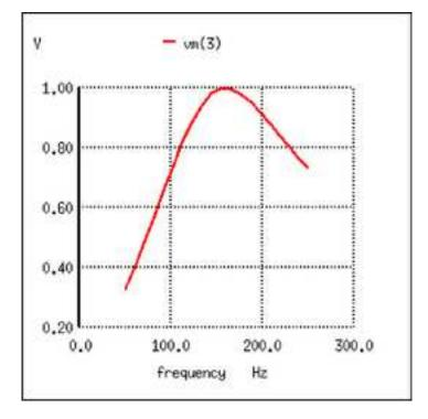
series resonant bandpass filter Load voltage peaks at resonant frequency (159.15 Hz)
