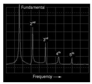
The distinction between a waveform having even harmonics versus no even harmonics resides in the difference between a triangle waveshape and a sawtooth waveshape. That difference is *symmetry* above and below the horizontal centerline of the wave. A waveform that is symmetrical above and below its centerline (the shape on both sides mirror each other precisely) will contain *no* evennumbered harmonics.
