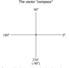
Rectangular form, on the other hand, is where a complex number is denoted by its respective horizontal and vertical components. In essence, the angled vector is taken to be the hypotenuse of a right triangle, described by the lengths of the adjacent and opposite sides. Rather than describing a vector's length and direction by denoting magnitude and angle, it is described in terms of "how far left/right" and "how far up/down."
