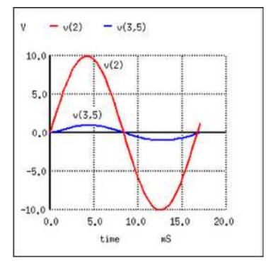
In going from primary, V(2), to secondary, V(3,5), the voltage was stepped down by a factor of ten, above, and the current was stepped up by a factor of 10 below. Both current and voltage waveforms are in phase in going from primary to secondary, below.
