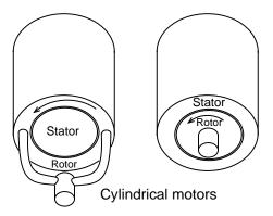
The most usual construction, cylindrical, can take on two forms, above. The most common cylindrical style is with the rotor on the inside, above right. This style motor is used in hard disk drives. It is also possible the put the rotor on the outside surrounding the stator. Such is the case with brushless DC fan motors, sans the shaft. This style of construction may be short and fat. However, the direction of the magnetic flux is radial with respect to the rotational axis.
