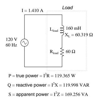
These three types of power - true, reactive, and apparent - relate to one another in trigonometric form. We call this the *power triangle*:
