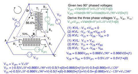
Scott-T transformer 2- $\phi$  to 3- $\phi$  conversion equations
