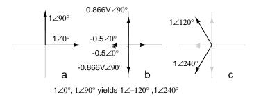
Above we graphically show the 2- $\phi$  vectors at (a). At (b) the vectors are scaled by transformers T1 and T2 to 0.5 and 0.866 respectively. At (c)  $1 \angle 120^{\circ} = -0.5 \angle 0^{\circ} + 0.866 \angle 90^{\circ}$ , and  $1 \angle 240^{\circ} = -0.5 \angle 0^{\circ} - 0.866 \angle 90^{\circ}$ .
