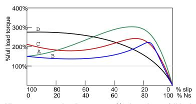
All motors, except class D, operate at %5 slip or less at full load.
