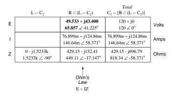
A quick double-check of our work at this point would be to see whether or not the voltage drops across  $C_1$  and the series-parallel combination of  $R//(L--C_2)$  indeed add up to the total. According to Kirchhoff's Voltage Law, they should!
