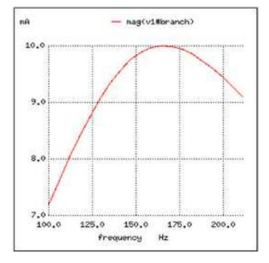
Note that the peak of the current graph has not changed from the earlier series LC circuit (the one with the 1  $\Omega$  token resistance in it), even though the resistance is now 100 times greater. The only thing that has changed is the "sharpness" of the curve. Obviously, this circuit does not resonate as strongly as one with less series resistance (it is said to be "less selective"), but at least it has the same natural frequency!
