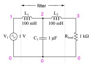
The inductors should block any high frequencies, while the capacitor should short out any high frequencies as well, both working together to allow only low frequency signals to reach the load.
