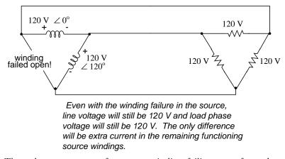
The only consequence of a source winding failing open for a  $\Delta$ -connected source is increased phase current in the remaining windings. Compare this fault tolerance with a Y-connected system suffering an open source winding:
