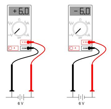
The mathematical sign of a digital DC voltmeter's display has meaning only in the context of its test lead connections. Consider the use of a DC voltmeter in determining whether or not two DC voltage sources are aiding or opposing each other, assuming that both sources are unlabeled as to their polarities. Using the voltmeter to measure across the first source:
