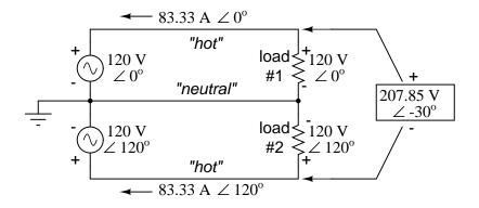
Since each voltage source is 120 volts, and each load resistor is connected directly in parallel with its respective source, the voltage across each load *must* be 120 volts as well. Given load currents of 83.33 amps, each load must still be dissipating 10 kilowatts of power. However, voltage between the two "hot" wires is not 240 volts ( $120 \angle 0^{\circ} - 120 \angle 180^{\circ}$ ) because the phase difference between the two sources is not 180°. Instead, the voltage is:
