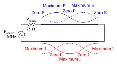
However, if the signal frequency is such that the line resonates at 1/4 wavelength or some multiple thereof, the source will "see" the exact opposite of the termination impedance. That is, if the line is open-circuited, the source will "see" a short-circuit at the point where it connects to the line; and if the line is short-circuited, the source will "see" an open circuit:
