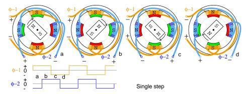
Single step bipolar drive is shown above. The step angle is the same as for wave drive. Unipolar drive (not shown) would require a pair of unipolar waveforms for each of the above bipolar waveforms applied to the ends of a center tapped winding.
