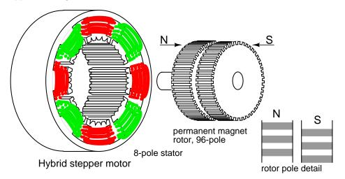
Note that the 48-teeth on one rotor section are offset by half a pitch from the other. See rotor pole detail above. This rotor tooth offset is also shown below. Due to this offset, the rotor effectively has 96 interleaved poles of opposite polarity. This offset allows for rotation in 1/96 th of a revolution steps by reversing the field polarity of one phase. Two phase windings are common as shown above and below. There could be as many as five phases.
