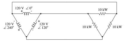
With each load resistance receiving 120 volts from its respective phase winding at the source, the current in each phase of this circuit will be 83.33 amps:
