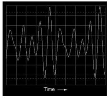
The oscilloscope display (time-domain) shows a waveform with many more peaks and valleys than before, a direct result of the mixing of these three frequencies. As you will notice, some of these peaks are higher than the peaks of the original single-pitch waveform, while others are lower. This is a result of the three different waveforms alternately reinforcing and canceling each other as their respective phase shifts change in time.
