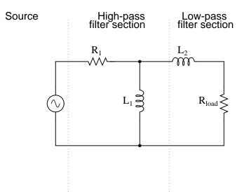
The fact that the high-pass section comes "first" in this design instead of the low-pass section makes no difference in its overall operation. It will still filter out all frequencies too high or too low.
