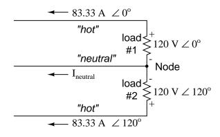
$\begin{aligned} -I_{load\#1} - I_{load\#2} - I_{neutral} &= 0 \\ -I_{neutral} &= I_{load\#1} + I_{load\#2} \\ I_{neutral} &= -I_{load\#1} - I_{load\#2} \\ I_{neutral} &= - (83.33 \text{ A} \angle 0^{\circ}) - (83.33 \text{ A} \angle 120^{\circ}) \\ I_{neutral} &= 83.33 \text{ A} \angle 240^{\circ} \text{ or } 83.33 \text{ A} \angle -120^{\circ} \end{aligned}$
