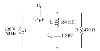
The first order of business, as usual, is to determine values of impedance (Z) for all components based on the frequency of the AC power source. To do this, we need to first determine values of reactance (X) for all inductors and capacitors, then convert reactance (X) and resistance (R) figures into proper impedance (Z) form:
