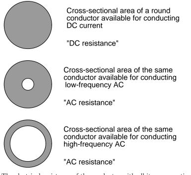
The electrical resistance of the conductor with all its cross-sectional area in use is known as the "DC resistance," the "AC resistance" of the same conductor referring to a higher figure resulting
