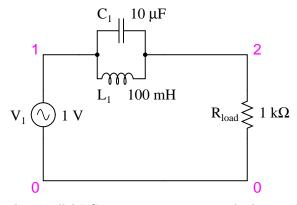
The parallel LC components present a high impedance at resonant frequency, thereby blocking the signal from the load at that frequency. Conversely, it passes signals to the load at any other frequencies.
