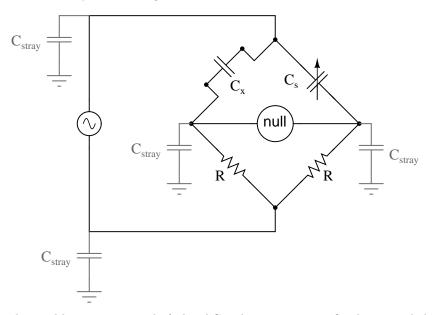
The problem is worsened if the AC voltage source is firmly grounded at one end, the total stray impedance for leakage currents made far less and any leakage currents through these stray capacitances made greater as a result:
