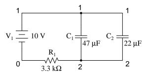
For DC analysis, the initial conditions of any reactive component (C or L) must be specified (voltage for capacitors, current for inductors). This is provided by the last data field of each capacitor card (ic=0). To perform a DC analysis, the .tran ("transient") analysis option must be specified, with the first data field specifying time increment in seconds, the second specifying total analysis timespan in seconds, and the "uic" telling it to "use initial conditions" when analyzing.
