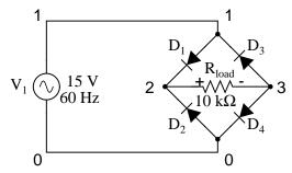
Diodes, like all semiconductor components in SPICE, must be modeled so that SPICE knows all the nitty-gritty details of how they're supposed to work. Fortunately, SPICE comes with a few generic models, and the diode is the most basic. Notice the .model card which simply specifies "d" as the generic diode model for mod1. Again, since we're plotting the waveforms here, we need to specify all parameters of the AC source in a single card and print/plot all values using the .tran option.
