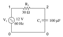
The .ac card specifies the points of ac analysis from 60Hz to 60Hz, at a single point. This card, of course, is a bit more useful for multi-frequency analysis, where a range of frequencies can be analyzed in steps. The .print card outputs the AC voltage between nodes 1 and 2, and the AC voltage between node 2 and ground.
