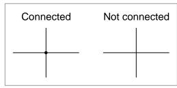
Older electrical schematics showed connecting wires crossing, while non-connecting wires "jumped" over each other with little half-circle marks. Newer electrical schematics show connecting wires joining with a dot, while non-connecting wires cross with no dot. However, some people still use the older convention of connecting wires crossing with no dot, which may create confusion.
