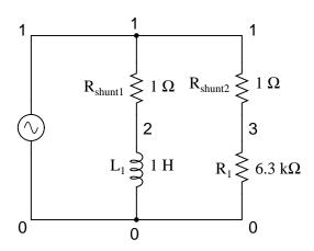
The currents through each leg are indicated by the voltage drops across each respective shunt resistor (1 amp = 1 volt through 1  $\Omega$ ), output by the v(1,2) and v(1,3) terms of the .print card. The phase of the currents through each leg are indicated by the phase of the voltage drops across each respective shunt resistor, output by the vp(1,2) and vp(1,3) terms in the .print card.
