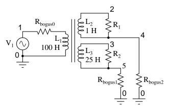
SPICE understands transformers as a set of mutually coupled inductors. Thus, to simulate a transformer in SPICE, you must specify the primary and secondary windings as separate inductors, then instruct SPICE to link them together with a "k" card specifying the coupling constant. For ideal transformer simulation, the coupling constant would be unity (1). However, SPICE can't handle this value, so we use something like 0.999 as the coupling factor.
