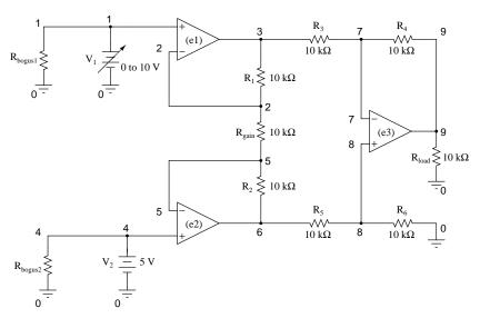
Note the very high-resistance  $R_{bogus1}$  and  $R_{bogus2}$  resistors in the netlist (not shown in schematic for brevity) across each input voltage source, to keep SPICE from thinking  $V_1$  and  $V_2$  were open-circuited, just like the other op-amp circuit examples.
