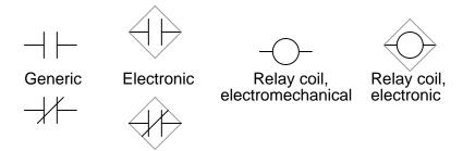
Relays, electronic schematic notation style
