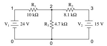
Without a .dc card and a .print or .plot card, the output for this netlist will only display voltages for nodes 1, 2, and 3 (with reference to node 0, of course).
