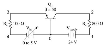
This analysis sweeps the input voltage (Vin) from 0 to 5 volts in 0.1 volt increments, then prints out the voltage between the collector and emitter leads of the transistor v(2,3). The transistor (Q1) is an NPN with a forward Beta of 50.
