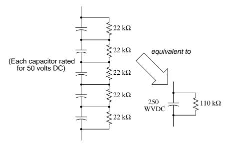
Bear in mind that the total capacitance for this five-capacitor network will be 1/5, or 20%, of each capacitor's value. Also, to ensure even charging of capacitors in the network, be sure all capacitor values (in  $\mu$ F) and all resistor values are identical.
