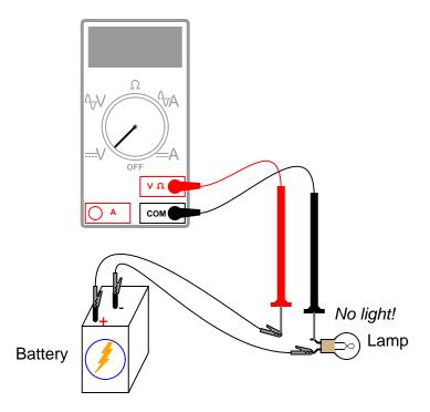
What voltages measure the same as before? What voltages are different since introducing the break? How much voltage is manifest, or *dropped* across the break? What is the *polarity* of the voltage drop across the break, as indicated by the meter?
