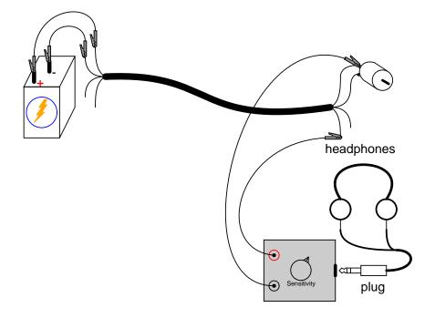
The noise voltage detected here is due to stray capacitance between adjacent cable conductors creating an AC current "path" between the wires. Remember that no current actually goes through a capacitance, but the alternate charging and discharging action of a capacitance, whether it be intentional or unintentional, provides alternating current a pathway of sorts.
