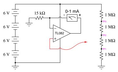
This alteration in the power supply increases the voltages at TP1, TP2, and TP3 to 6, 12, and 18 volts, respectively. With a 15 k $\Omega$  range resistor and a 1 mA meter movement, measuring 18 volts will gently "peg" the meter, but you should be able to measure the 6 and 12 volt test points just fine.
