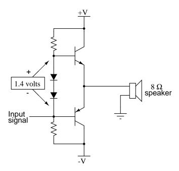
The two series-connected diodes will drop approximately 1.4 volts, equivalent to the combined  $V_{be}$  forward voltage drops of the two transistors, resulting in a scenario where each transistor is just on the verge of turning on when the input signal is zero volts, eliminating the 1.4 volt "dead" signal zone that existed before.
