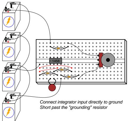
As soon as the "grounding" resistor is shorted with a jumper wire, the op-amp's output voltage will start to change, or drift. Ideally, this should not happen, because the integrator circuit still
