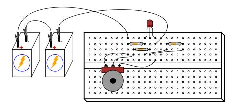
Although this different method of feedback accomplishes the same goal of increased stability by diminishing gain, the two feedback circuits will not behave identically. Note the range of possible output voltages with each feedback scheme (the low and high voltage values obtained with a full sweep of the input voltage potentiometer), and how this differs between the two circuits.
