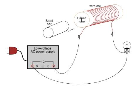
Wrap hundreds of turns of magnet wire around the paper tube. Connect this home-made inductor in series with an AC power supply and lamp to form a circuit. When the tube is empty, the lamp should glow brightly. When the steel bar is inserted in the tube, the lamp dims from increased inductance (L) and consequently increased inductive reactance  $(X_L)$ .
