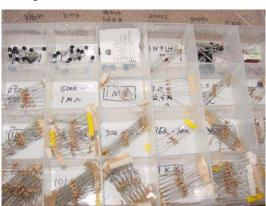
In this view of one of my component boxes, you can see plenty of 1/8 watt resistors, transistors, diodes, and even a few 8-pin integrated circuits ("chips"). Labels for each compartment were made with a permanent ink marker.
