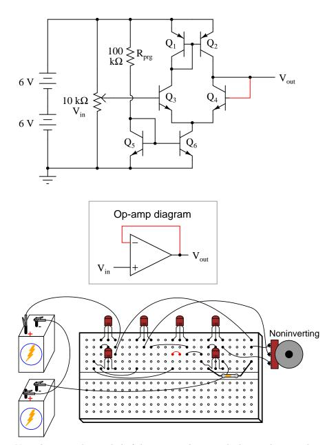
Note the triangular symbol of the op-amp shown in the lower schematic diagram. The inverting and noninverting inputs are designated with (-) and (+) symbols, respectively, with the output terminal at the right apex. The feedback wire connecting output to inverting input is shown in red in the above diagrams.
