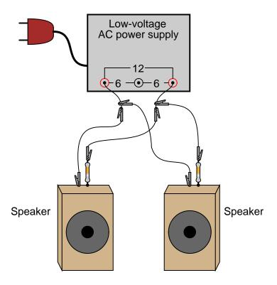
Connect each speaker to the low-voltage AC power supply through a 220  $\Omega$  resistor. The resistor limits the amount of power delivered to each speaker by the power supply. A low-pitched, 60-Hertz tone should be heard from the speakers. If the tone sounds too loud, use higher-value resistors.
