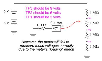
Try using the meter movement and 15 k $\Omega$  resistor as shown to measure these three voltages. Does the meter read falsely high or falsely low? Why do you think this is?
