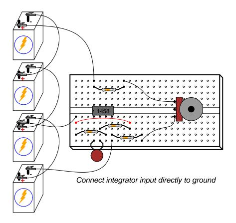
Applying exactly zero voltage to the input of an integrator circuit should, ideally, cause the output voltage rate-of-change to be zero. When you make this change to the circuit, you should notice the output voltage remaining at a constant level or changing very slowly.
