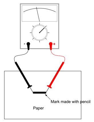
Move the probe tips closer together on the black mark and note the change in resistance value. Does it increase or decrease with decreased probe spacing? If the results are inconsistent, you need to redraw the mark with more and heavier pencil strokes, so that it is consistent in its density. What does this teach you about resistance versus length of a conductive material?
