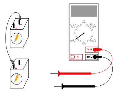
Connecting components in *series* means to connect them in-line with each other, so that there is but a single path for electrons to flow through them all. If you connect batteries so that the positive of one connects to the negative of the other, you will find that their respective voltages add. Measure the voltage across each battery individually as they are connected, then measure the total voltage across them both, like this:
