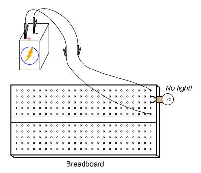
Here there is no "shorting" wire present on the breadboard, yet there is a short circuit, and the lamp refuses to light. Based on your understanding of breadboard hole connections, can you determine where the "short" is in this circuit?
