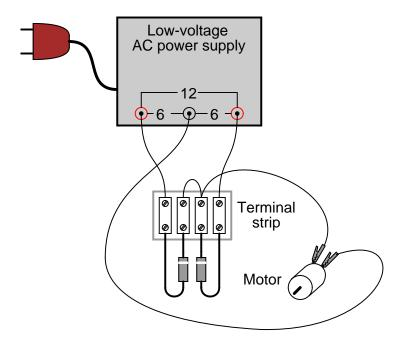
This rectifier circuit is called *full-wave* because it makes use of the entire waveform, both positive and negative half-cycles, of the AC source voltage in powering the DC load. As a result, there is less "ripple" voltage seen at the load. The RMS (Root-Mean-Square) value of the rectifier's output is also greater for this circuit than for the half-wave rectifier.
