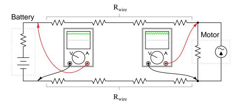
Use the audio detector to measure "noise" voltage directly across the battery. Since the AC noise is produced in this circuit by pulsating voltage drops along stray resistances, the less resistance we measure across, the less noise voltage we should detect:
