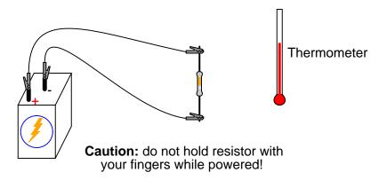
Measure each resistor's resistance with your ohmmeter, noting the exact values on a piece of paper for later reference.
