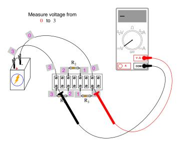
Using the voltmeter to "step" around the circuit in this manner yields three positive voltage figures and one negative:
