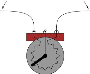
Build the circuit as shown in the schematic and illustration, using just two terminals on the potentiometer, and see how motor speed may be controlled by adjusting shaft position. Experiment with different terminal connections on the potentiometer, noting the changes in motor speed control. If your potentiometer has a high resistance (as measured between the two outer terminals), the motor might not move at all until the wiper is brought very close to the connected outer terminal.
