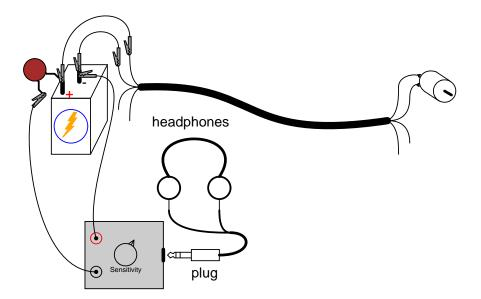
You may also measure noise voltage dropped along either of the telephone cable conductors supplying power to the motor, by connecting the audio detector between both ends of a single cable conductor. The noise detected here originates from current pulses through the resistance of the wire:
