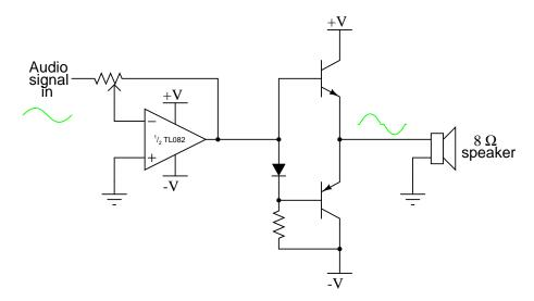
Since the voltage drop of a single diode will always be less than the combined voltage drops of the two transistors' base-emitter junctions, the transistors can never turn on simultaneously, thereby preventing class AB operation. Next, to help get rid of the remaining crossover distortion, the feedback signal of the op-amp is taken from the output terminal of the amplifier (the transistors' emitter terminals) like this:
