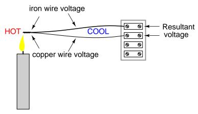
Thermocouples are widely used as temperature-sensing devices because the mathematical relationship between temperature difference and resultant voltage is both repeatable and fairly linear. By measuring voltage, it is possible to infer temperature. Different ranges of temperature measurement are possible by selecting different metal pairs to be joined together.
