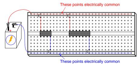
With so many of these integrated circuits having "reset," "enable," and "disable" terminals needing to be maintained in a "high" or "low" state, not to mention the  $V_{DD}$  (or  $V_{CC}$ ) and ground power terminals which require connection to the power supply, having both terminals of the power supply readily available for connection at any point along the board's length is very useful.
