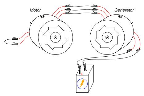
Spin the generator shaft while watching the motor shaft's rotation. Try reversing any two of the three-phase line connections between the two units and spin the generator again. What is different this time?
