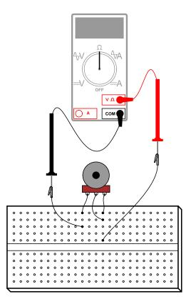
Suppose we wanted to elevate the lower end of this resistance range so that we had an adjustable range from 10 k $\Omega$  to 20 k $\Omega$  with a full sweep of the potentiometer's adjustment. This could be easily accomplished by adding a 10 k $\Omega$  resistor in *series* with the potentiometer. Add one to the circuit as shown and re-measure total resistance while adjusting the potentiometer:
