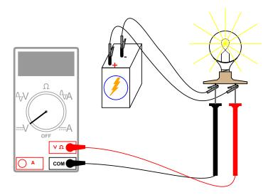
The voltmeter should register a voltage lower than the usual voltage of the battery. If you use your voltmeter to read the voltage directly at the battery terminals, you will measure a low voltage there as well. Why is this? The large current drawn by the high-power lamp causes the voltage at the battery terminals to "sag" or "droop," due to voltage dropped across resistance internal to the battery.
