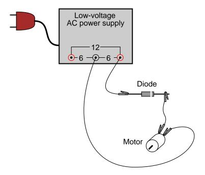
Connect the motor to the low-voltage AC power supply through the rectifying diode as shown. The diode only allows current to pass through during one half-cycle of a full positive-and-negative cycle of power supply voltage, eliminating one half-cycle from ever reaching the motor. As a result, the motor only "sees" current in one direction, albeit a *pulsating* current, allowing it to spin in one direction.
