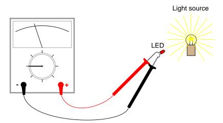
Batteries develop electrical voltage through chemical reactions. When a battery "dies," it has exhausted its original store of chemical "fuel." The LED, however, does not rely on an internal "fuel" to generate voltage; rather, it *converts* optical energy into electrical energy. So long as there is light to illuminate the LED, it will produce voltage.
