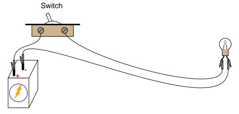
Build a one-battery, one-switch, one-lamp circuit as shown in the schematic diagram and in the illustration. This circuit is most impressive when the wires are *long*, as it shows how the switch is able to control circuit current no matter how physically large the circuit may be.
