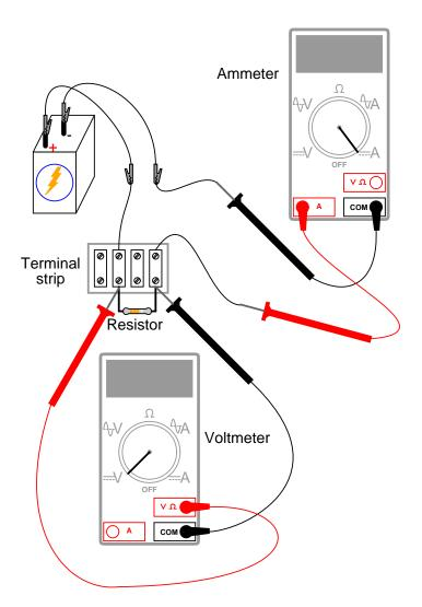
Select a resistor from the assortment, and measure its resistance with your multimeter set to the appropriate resistance range. Be sure not to hold the resistor terminals when measuring resistance, or else your hand-to-hand body resistance will influence the measurement! Record this resistance value for future use.
