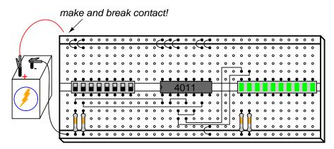
When a latch circuit such as this is powered up into its "latched" state, the gates race against each other for control. Given the "low" inputs, both gates try to output "high" signals. If one of the gates reaches its "high" output state before the other, that "high" state will be fed back to the other gate's input to force its output "low," and the race is won by the faster gate.
