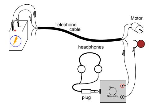
Connect the motor to the battery using two of the telephone cable's four conductors. The motor should run, as expected. Now, connect the audio signal detector across the motor terminals, with the 0.047  $\mu$ F capacitor in series, like this:
