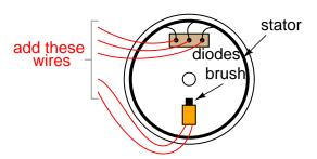
I recommend that you solder ring-lug terminals to your wires, and attach them underneath the terminal nuts along with the stator wire ends, so that each diode block terminal is securing two ring lugs.
