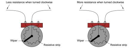
Be careful, though, that you don't use the two outer terminals, as this will result in *no change* in resistance as the potentiometer shaft is turned. In other words, it will no longer function as a variable resistance:
