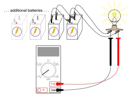
There should also be a noticeable difference in light intensity as the voltage "sag" is improved. Try measuring the current of one battery and comparing it to the total current (light bulb current). Shown here is the easiest way to measure single-battery current:
