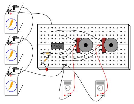
Comparator circuits are widely used to compare physical measurements, provided those physical variables can be translated into voltage signals. For instance, if a small generator were attached to an anemometer wheel to produce a voltage proportional to wind speed, that wind speed signal could be compared with a "set-point" voltage and compared by an op-amp to drive a high wind speed alarm:
