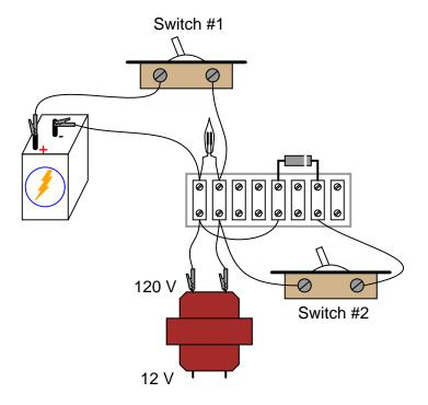
When assembling the circuit, be very careful of the diode's orientation. The cathode end of the diode (the end marked with a single band) must face the positive (+) side of the battery. The diode should be reverse-biased and nonconducting with switch #1 in the "on" position. Use the high-voltage (120 V) winding of the transformer for the inductor coil. The primary winding of a step-down transformer has more inductance than the secondary winding, and will give a greater lamp-flashing effect.
