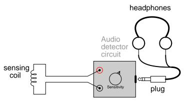
Using the audio detector circuit explained earlier to detect AC voltage in the audio frequencies, a coil of wire may serve as sensor of AC magnetic fields. The voltages produced by the coil will be quite small, so it is advisable to adjust the detector's sensitivity control to "maximum."
