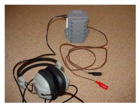
As you can see, I built my detector using scrap parts (household electrical switch/receptacle box for the enclosure, section of brown lamp cord for the test leads). Even some of the internal components were salvaged from scrap (the step-down transformer and headphone jack were taken from an old radio, purchased in non-working condition from a thrift store). The entire thing,
