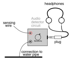
"Ground" one lead of the detector to a metal object in contact with the earth (dirt). Most any water pipe or faucet in a house will suffice. Take the other lead and hold it close to an electrical appliance or lamp fixture. **Do not try to make contact with the appliance or with any conductors within!** Any AC electric fields produced by the appliance will be heard in the headphones as a buzzing tone.
