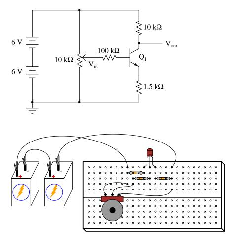
Repeat the same voltage measurement and recording exercise with the 1.5 k $\Omega$  resistor installed, calculating the new (reduced) voltage gain. Try altering the transistor's temperature again and noting the output voltage for a steady input voltage. Does it change more or less than without the 1.5 k $\Omega$  resistor?
