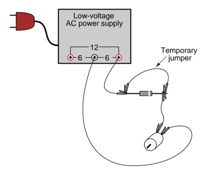
As you can see, permanent-magnet "DC" motors do not function well on alternating current. Remove the temporary jumper wire and reverse the diode's orientation in the circuit. Note the effect on the motor.
