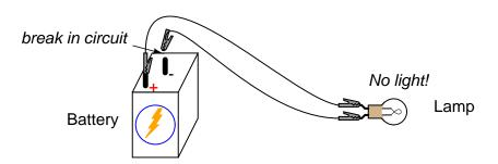
Using your multimeter set to the appropriate "DC volt" range, measure voltage across the battery, across the lamp, and across each jumper wire. Familiarize yourself with the normal voltages in a functioning circuit.
