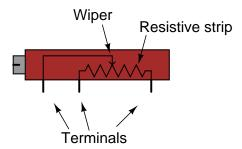
It should be noted that not all linear potentiometers have the same pin assignments. On some, the middle pin is the wiper.
