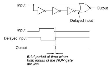
The single NOR gate and three inverter gates create this effect by exploiting the propagation delay time of multiple, cascaded gates. In this experiment, I use three NOR gates with paralleled inputs to create three inverters, thus using all four NOR gates of a 4001 integrated circuit:
