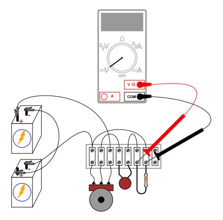
Measure voltage between the potentiometer's wiper terminal and the "ground" point shown in the schematic diagram (the negative terminal of the lower 6-volt battery). This is the input voltage for the circuit, and you can see how it smoothly varies between zero and 12 volts as the potentiometer control is turned full-range. Since the potentiometer is used here as a voltage divider, this behavior should be unsurprising to you.
