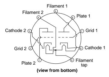
You will notice on the amplifier schematic that both triode elements inside the 12AX7's glass envelope are being used, in parallel: plate connected to plate, grid connected to grid, and cathode connected to cathode. This is done to maximize power output from the tube, but it is not necessary for demonstrating basic operation. You may use just one of the triodes, for simplicity, if you wish.
