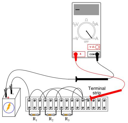
Note both the magnitude and the sign of the current as indicated by the ammeter. Add this figure (algebraically) to the three resistor currents. What do you notice about the result that is similar to the Kirchhoff's Voltage Law experiment? Kirchhoff's Current Law is to currents "summing" at a point (node) in a circuit, just as Kirchhoff's Voltage Law is to voltages adding in a series loop: in both cases, the algebraic sum is equal to zero.
