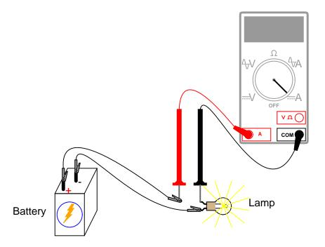
Current is the measure of the rate of electron "flow" in a circuit. It is measured in the unit of the Ampere, simply called "Amp," (A).
