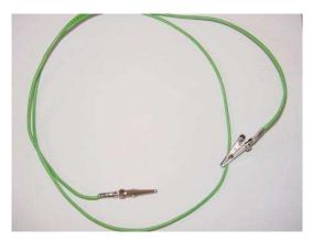
The home-made jumper wires with large, uninsulated (bare metal) alligator clips are okay to use so long as care is taken to avoid any unintentional contact between the bare clips and any other wires or components. For use in crowded breadboard circuits, jumper wires with insulated (rubber-covered) clips like the jumper shown from Radio Shack are much preferred.
