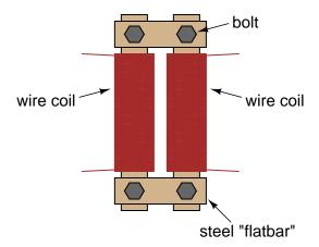
Wrap two, equal-length bars of steel with a thin layer of electrically-insulating tape. Wrap several hundred turns of magnet wire around these two bars. You may make these windings with an equal or unequal number of turns, depending on whether or not you want the transformer to be able to "step" voltage up or down. I recommend equal turns to begin with, then experiment later with coils of unequal turn count.
