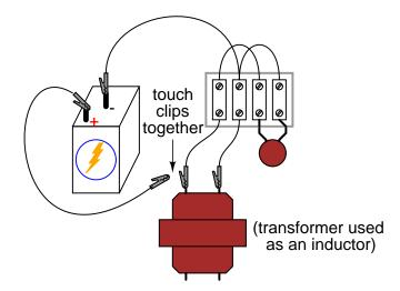
If an inductor and a capacitor are connected in parallel with each other, and then briefly energized by connection to a DC voltage source, oscillations will ensue as energy is exchanged from the capacitor to inductor and vice versa. These oscillations may be viewed with an oscilloscope connected in parallel with the inductor/capacitor circuit. Parallel inductor/capacitor circuits are commonly known as *tank circuits*.
