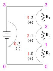
These figures, algebraically added ("algebraically" = respecting the signs of the numbers), should equal zero. This is the fundamental principle of Kirchhoff's Voltage Law: that the algebraic sum of all voltage drops in a "loop" add to zero.
