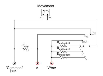
$\ensuremath{^{\text{"}}} R_{\text{multiplier}}\ensuremath{^{\text{"}}}$  resistors are actually rheostat networks
