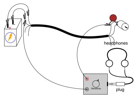
Now that we have established how AC noise is created and distributed in this circuit, let's explore how it is *coupled* to adjacent wires in the cable. Use the audio detector to measure voltage between one of the motor terminals and one of the unused wires in the telephone cable. The 0.047  $\mu$ F capacitor is not needed in this exercise, because there is no DC voltage between these points for the detector to detect anyway:
