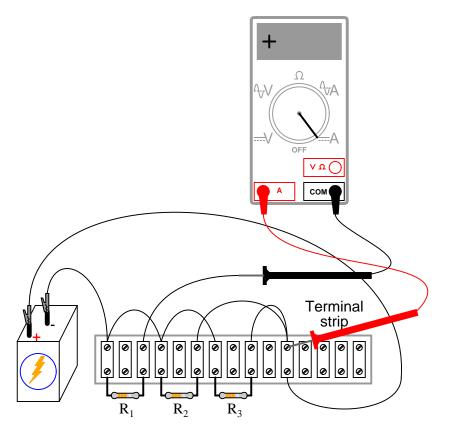
Measure current for each of the three resistors, comparing with the current figures calculated previously. With the digital ammeter connected as shown, all three indications should be positive, not negative.
