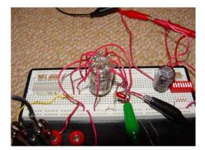
One benefit of mounting the tube in this position is ease of pin identification, since most "pin connection diagrams" for tubes are shown from a bottom view:
