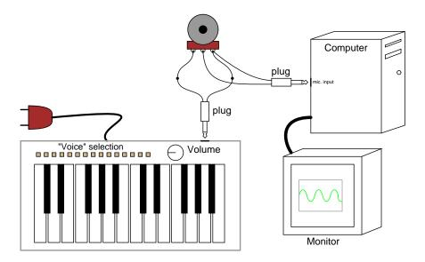
The Winscope program comes with another feature other than the typical "time-domain" oscilloscope display: "frequency-domain" display, which plots amplitude (vertical) over frequency (horizontal). An oscilloscope's "time-domain" display plots amplitude (vertical) over time (horizontal), which is fine for displaying waveshape. However, when it is desirable to see the harmonic constituency of a complex wave, a frequency-domain plot is the best tool.
