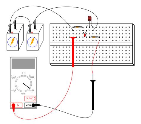
You may have to select the most sensitive current range on the meter to measure this small flow. After measuring this *controlling* current, try measuring the LED's current (the *controlled* current) and compare magnitudes. Don't be surprised if you find a ratio in excess of 200 (the controlled current 200 times as great as the controlling current)!
