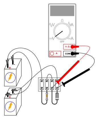
Connect three, then four 6-volt batteries together in series, forming an 18 volt and 24 volt power source, respectively. Measure and record the diode's and resistor's voltage drops for each new power supply voltage. What do you notice about the diode's voltage drop for these four different source voltages? Do you see how the diode voltage never exceeds a level of 12 volts? What do you notice about the resistor's voltage drop for these four different source voltage levels?
