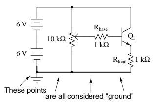
For example, if I were to speak of voltage at the base of the transistor  $(V_B)$ , I would mean the voltage measured between the transistor's base terminal and the negative side of the power supply (ground), with the red probe touching the base terminal and the black probe touching ground. Normally, it is nonsense to speak of voltage at a single point, but having an implicit reference point for voltage measurements makes such statements meaningful:
