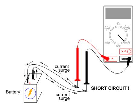
Ammeters are generally protected from excessive current by means of a small *fuse* located inside the meter housing. If the ammeter is accidently connected across a substantial voltage source, the resultant surge in current will "blow" the fuse and render the meter incapable of measuring current until the fuse is replaced. **Be very careful to avoid this scenario!**
