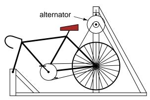
The rear wheel drives the generator sheave with a *long* v-belt. This belt also supports the rear of the bicycle, maintaining a constant tension when a rider is pedaling the bicycle. The generator hangs from a steel support structure (I used welded 2-inch square tubing, but a frame could be made out of lumber). Not only is this machine practical, but it is reliable enough to be used as an exercise machine, and it is inexpensive to make:
