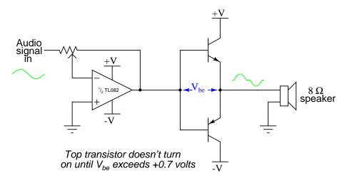
Bottom transistor doesn't turn on until  $V_{be}$  drops below -0.7 volts
