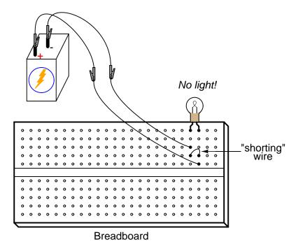
Here is an example of an accidental short circuit of the type typically made by students unfamiliar with breadboard usage:
