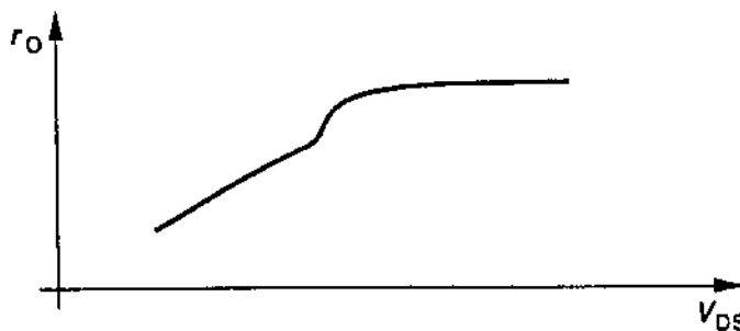
Figure 16.14 Kink in output resistance in Level 3 model.
