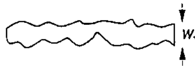
Figure 18.2 Excessive width variation in a narrow poly line.
