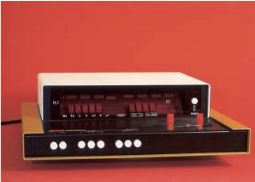
FIGURE 8–47 Digital bridge used for precisely measuring resistance, inductance, and capacitance.
