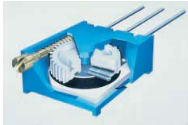
(b) Internal view of variable resistor.
