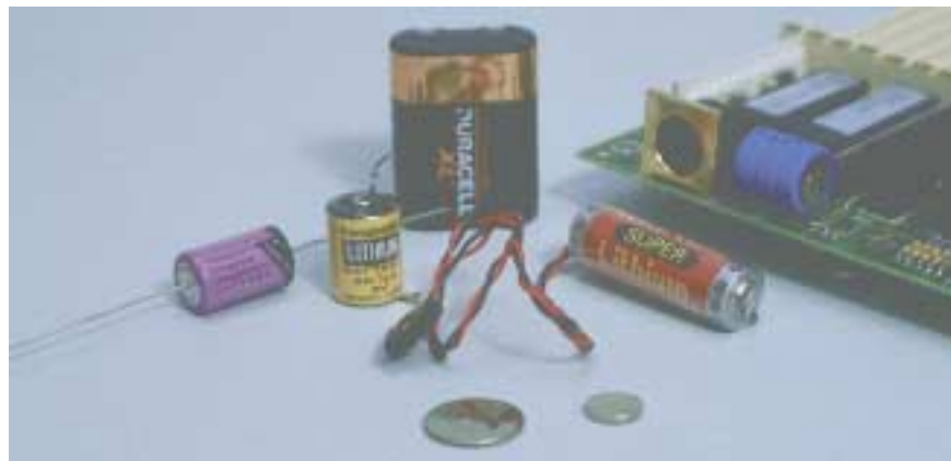
FIGURE 2-13 An assortment of lithium batteries. The battery on the computer motherboard is for memory backup.
