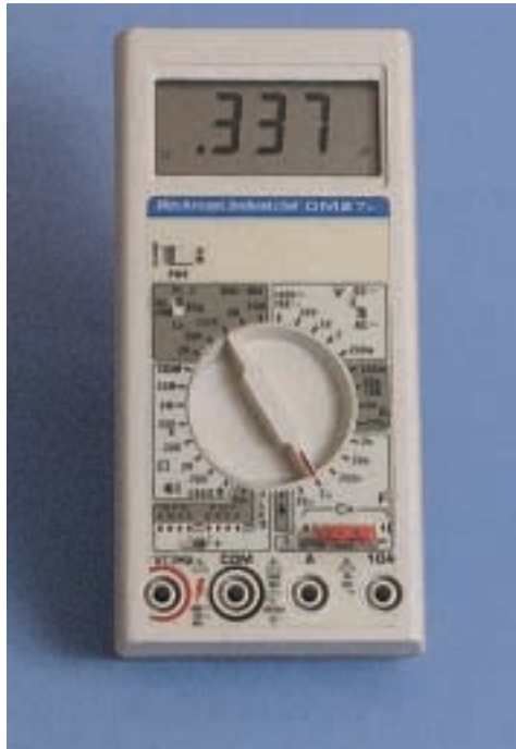
FIGURE 15–69 A DMM. While all DMMs measure voltage, current, and resistance, this one also measures frequency.
