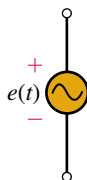
FIGURE 15–3 Symbol for a sinusoidal voltage source. Lowercase letter e is used to indicate that the voltage varies with time.
