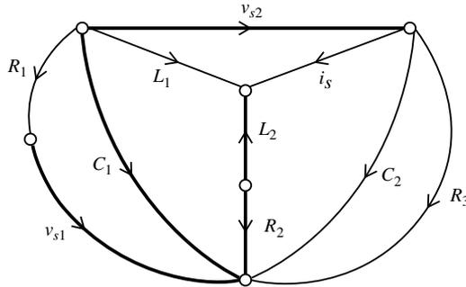
FIGURE 10.6 The directed graph associated with the circuit of Figure 10.5.
