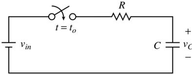
FIGURE 10.1 A simple RC circuit.
