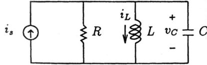
FIGURE 10.7 A parallel RLC circuit.
