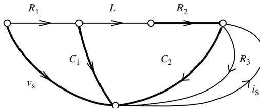
FIGURE 10.4 The directed graph associated with the circuit of Figure 10.3.
