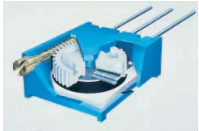
(b) Internal view of variable resistor.
