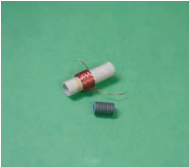
FIGURE 13–19 A variable inductor with its ferrite core removed for viewing.
