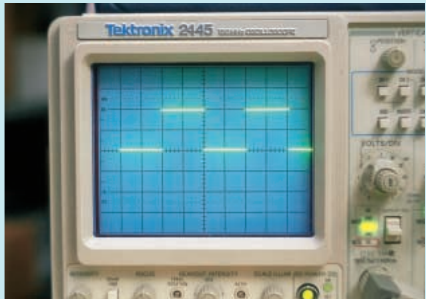
FIGURE 15-16 The concepts of frequency and period apply to nonsinusoidal waveforms.
