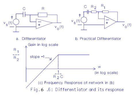
A circuit that works well as a differentiator under ideal conditions is shown in Fig. 6.6a. For this circuit, the transfer function is:
