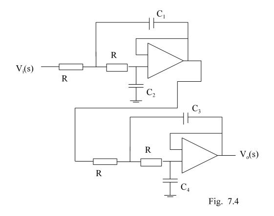
The transfer function for the above circuit is:
