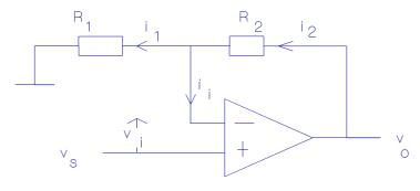
Fig.2.1: NON-INVERTING AMPLIFIER
