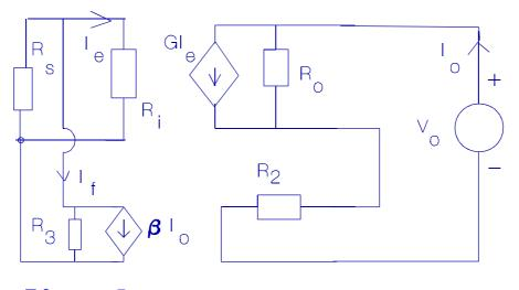
Fig.5.5:-Finding Output Resistance
