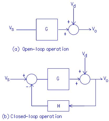
Fig.3.4 : Effect of feedback on distortion
