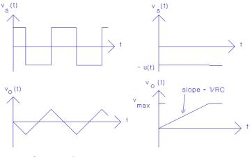
Fig. 6 .2: Waveforms for Integrator
