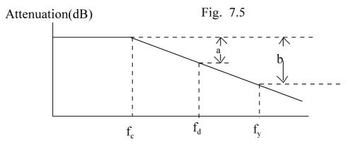
Using Bode Plot to determine attenuation at any frequency
