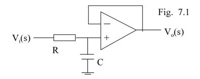
For the circuit in Fig. 7.1, the transfer function is  $H(s) = \frac{1}{sRC+1}$  (7.3)
