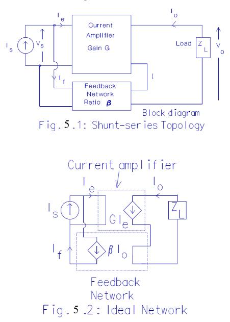
The ideal network with this topology can be represented by an equivalent circuit as shown in Fig. 5.2. This topology is the dual of series-shunt topology considered in the previous section. This topology uses a current amplifier in the forward path.
