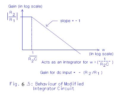
At frequencies above the corner frequency, the transfer function is:
