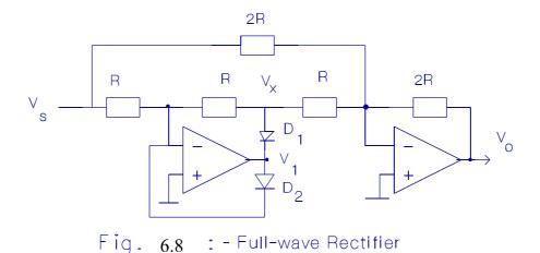
Let  $V_s$  be negative. The inverting input terminal of first opamp tends to be negative and its output becomes positive. Then  $V_1 = 0.7 \text{ V}$ , the diode drop and  $V_x = 0 \text{ V}$ . Now  $D_2$  conducts and  $D_1$  is reverse-biased. Under these conditions,  $V_o = -V_s$ . Hence we have that  $V_o = |V_s|$ . If diodes  $D_1$  and  $D_2$  are reverse-connected,  $V_o = -|V_s|$ .
