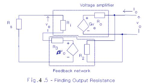
An ideal voltage amplifier has zero output resistance. In practice, it has a small and finite output resistance, which is denoted as  $R_o$  in Fig. 4.2. The output resistance is the resistance of the circuit seen by the load. That is, we can replace the load resistance by a voltage source. The resistance as seen by this source with the input source  $V_s$  removed is usually defined as the output resistance. By definition, output resistance  $R_y$  is:
