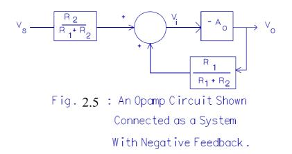
For the block diagram in Fig. 2.5, we get the ratio  $V_o/V_s$  as
