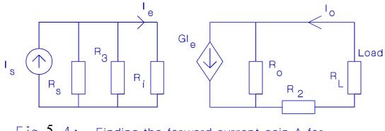
Fig.5.4: - Finding the forward current gain A for Shunt-series Topology
