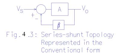
The circuit in Fig. 4.2 can be reduced to the block diagram shown in Fig. 4.3. From Fig.4.3, the closed-loop gain T is expressed to be:
