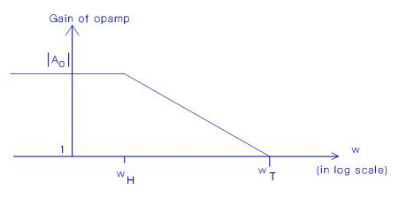
Fig. 1.3: Change in gain of Opamp with Frequency
