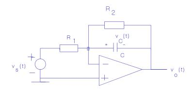
Fig. 6.4: Modified Integrator Circuit
