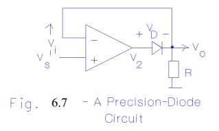
Figure 6.7 shows the circuit of a precision diode. When  $V_s$  is positive,
