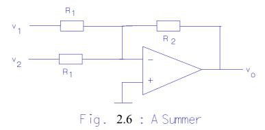
$$v_o = -\frac{R_2}{R_1} (v_1 + v_2)$$
