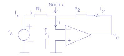
Fig. 2.4 : An Inverting Amplifier
