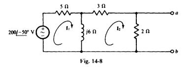
If the voltage source is replaced by a short circuit, the impedance  $Z_{1h}$  at terminals a and b is, by circuit reduction.
