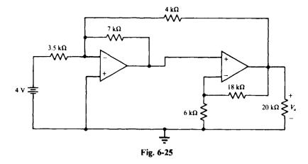
Although nodal analysis can be applied, it is simpler to view this circuit as a summer cascaded with a noninverting amplifier. The summer has two inputs,  $V_o$  and 4 V. Consequently, through use of the summer and noninverting voltage formulas,
