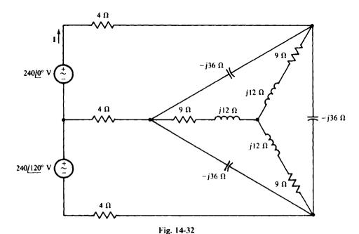
As the circuit stands, a considerable number of mesh or nodal equations are required to find I. But the circuit, which has a  $\Delta$  and a Y, can be reduced easily to just two meshes by using  $\Delta$ -Y transformations. Although these transformations do not always lessen the work required, they do here because they are so simple as a result of the common impedances of the Y branches and also of the  $\Delta$  branches.
