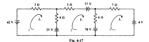
The self-resistances are  $3+4=7\Omega$  for mesh 1,  $4+5+6=15\Omega$  for mesh 2, and 6+7=13  $\Omega$  for mesh 3. The mutual resistances are 4  $\Omega$  for meshes 1 and 2, 6  $\Omega$  for meshes 2 and 3, and 0  $\Omega$  for meshes 1 and 3. The aiding source voltages are 42 + 25 = 67 V for mesh 1, -25 - 57 - 70 =-152 V for mesh 2, and 70 + 4 = 74 V for mesh 3. So, the mesh equations are
