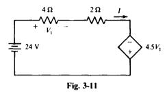
3.25 In the circuit of Fig. 3-11, determine the resistance "seen" by the independent voltage source.
