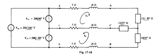
Notice in Fig. 17-18 the use of lowercase letters at the source terminals to distinguish them from the load terminals, as is necessary because of the line impedances.
