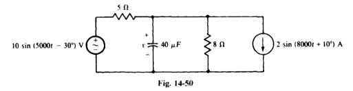
14.56 Find the average power dissipated in the 5- $\Omega$  resistor of the circuit shown in Fig. 14-50.
