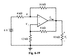
In Fig. 6-19, observe the lack of polarity references for  $V_{-}$  and  $V_{+}$ . Polarity references are not essential because these voltages are always referenced positive with respect to ground. Likewise the polarity reference for  $V_{0}$  could have been omitted.
