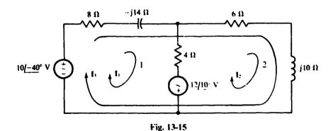
Placing the two mesh equations together shows the symmetry of coefficients (here - 4) about the principal diagonal as a result of the common mutual impedance.
