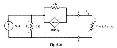
The Thévenin equivalent can be obtained by determining any two of  $V_{\rm Th}$ ,  $R_{\rm Th}$ , and  $I_{\rm SC}$ . By inspection, it appears that the two easiest to determine are  $V_{\rm Th}$  and  $R_{\rm Th}$ .
