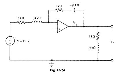
Because this circuit has the same configuration as the inverter op-amp circuit of Fig. 6-4, the same formula applies, with the R's replaced by Z's. The feedback impedance is  $Z_f = 6 - j8 \text{ k}\Omega$  and the input impedance is  $Z_i = 3 + j4 \text{ k}\Omega$ . Therefore, with the impedances expressed in kilohms,
