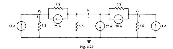
nodes 1 and 3. The currents flowing into the nodes from current sources are 42 + 25 = 67 A for node 1, -25 - 57 - 70 = -152 A for node 2, and 70 + 4 = 74 A for node 3. So, the nodal equations are
