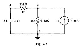
In this circuit file, observe the use of suffix letters in the value field to designate powers of 10. The 2E3 for the V1 statement could as well be 2K. Following is a complete listing of PSpice suffix letters and scale factors.
