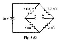
5.53 What will be the reading of a zero-resistance ammeter connected across terminals a and b of the bridge circuit shown in Fig. 5-53? Assume that the ammeter is connected to have an upscale reading. What will be the reading if a 1-k $\Omega$  resistor is in series with the ammeter?
