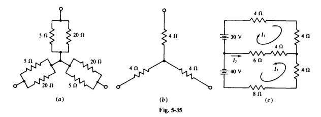
resistors of the two Y's are in parallel, as shown in Fig. 5-35a. The two Y's can be reduced to the single Y shown in Fig. 5-35b, in which each Y resistance is  $5\parallel 20=4\Omega$ . With this Y replacing the  $\Delta$ -Y combination, the circuit is as shown in Fig. 5-35c.
