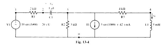
Observe that the resistor, inductor, and capacitor statements are essentially the same as for the other types of analyses, except that no initial conditions are specified in the inductor and capacitor statements. If the circuit had contained a dependent source, the corresponding statement would have been the same also.
