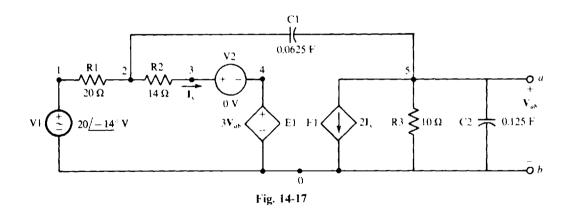
Obtaining  $\mathbf{Z}_{1h}$  directly requires deactivating the independent voltage source, which in turn requires changing the node 1 specification of resistor R1 to node 0. Also, a current source of 1/0. A can be applied at the a-b terminals with the current directed into node a. Then, the voltage across this source has the same numerical value as  $\mathbf{Z}_{1h}$ . Following is the modified circuit file along with the source voltage from the output file.
