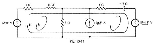
For the second loop, the self-impedance is  $3+j4+4-j6=7-j2\Omega$ , of which  $3+j4\Omega$  is mutual with loop 1. The 2/65-A current flowing through the components of  $4-j6\Omega$  produces a voltage drop of  $(4-j6)(2/65^\circ)=14.4/8.69$  V that has the same effect as the voltage from an opposing voltage source. In addition, the voltage sources have a net aiding voltage of  $6/30^\circ - 8/-15^\circ = 5.67/117^\circ$  V. The resulting loop 2 equation is
