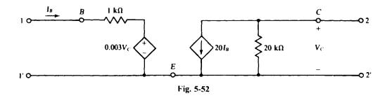
5.51 Find the output resistance at terminals 2 and 2' of the transistor circuit shown in Fig. 5-52 if a source with a  $500-\Omega$  internal resistance is connected to terminals 1 and 1'.
