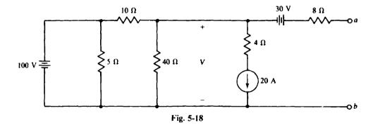
The Thévenin or open-circuit voltage, positive at terminal a, is the indicated V plus the 30 V of the 30-V source. The 8- $\Omega$  resistor has no effect on this voltage because there is zero current flow through it as a result of the open circuit. With zero current there is zero voltage. V can be found from a single nodal equation:
