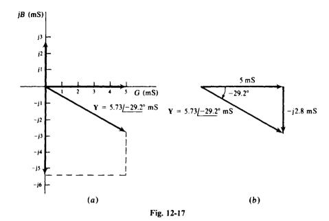
12.31 A 100- $\Omega$  resistor, a 1-mH inductor, and a 0.1- $\mu$ F capacitor are in parallel. Find the total admittances in polar form at radian frequencies of (a) 50 krad/s, (b) 100 krad/s, and (c)
