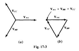
In general, three sinusoids have a sum of zero if they have the same frequency and peak value but are phase-displaced by 120. This is true regardless of what, if anything, that the sinusoids correspond to. In particular, it is true for currents.
