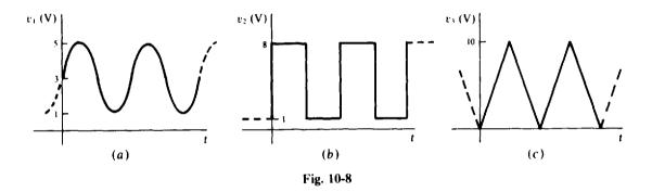
The cycle of the waveform shown in Fig. 10-8c beginning at t = 0 s is a triangle with a height of 10 and a base of T. The area under the curve for this one cycle is, from the triangular area formula of one-half the height times the base,  $0.5 \times 10 \times T = 5T$ . And so the average value is 5T T = 5 V.
