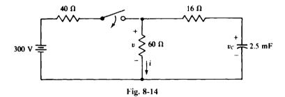
All that are needed for the v and i formulas are  $v_c(0+)$ ,  $v_c(\infty)$ , i(0+),  $i(\infty)$ , and  $\tau = R_{Th}C$ . Of course,  $v_c(0+) = 100 \text{ V}$  because the capacitor voltage cannot jump. The voltage  $v_c(\infty)$  is the same as the voltage across the 60- $\Omega$  resistor a long time after the switch closes, because at this time the capacitor acts like an open circuit. So, by voltage division,
