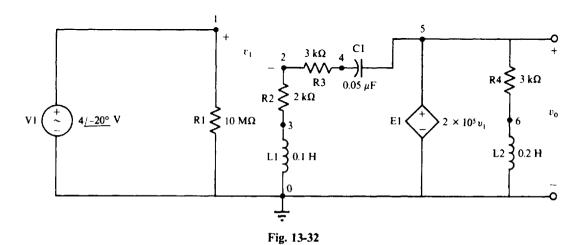
Following is the circuit file. The specified frequency, 1591.55 Hz, is equal to the source frequency of 10 000 rad/s divided by  $2\pi$ . Also shown is the output obtained when this circuit file is run with PSpice. The answer of  $V(5) = 9.121/-57.87^{\circ} V$  is the phasor for
