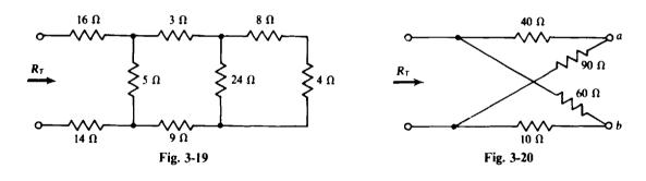
(a) With terminals a and b open, the 40- and 90- $\Omega$  resistors are in series, as are the 60- and 10- $\Omega$  resistors. The two series combinations are in parallel; so
