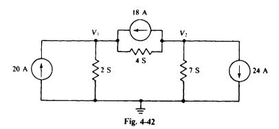
4.55 Double the currents from the current sources in the circuit shown in Fig. 4-42 and redetermine the node voltages. Compare them with the original node voltages.
