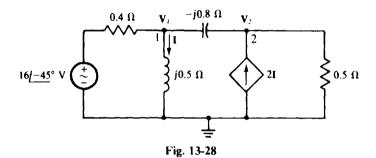
used to find  $V_1$ , and then I will be found from  $V_1$ . For nodal analysis, the voltage source and series resistor are preferably transformed to a current source with parallel resistor. The current source has a current of  $(16/-45^\circ)/0.4 = 40/-45^\circ$  A directed into node 1, and the parallel resistor has a resistance of 0.4  $\Omega$ . The self-admittances are
