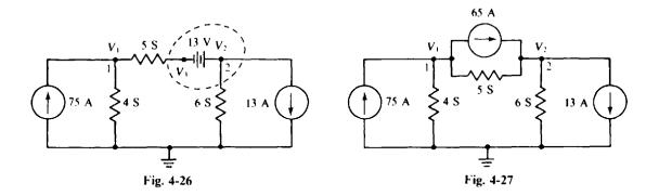
One analysis approach is to transform the voltage source and series resistor to a current source and parallel resistor, as shown in the circuit of Fig. 4-27.
