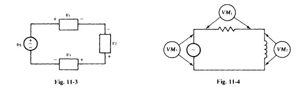
11.16 In the circuit shown in Fig. 11-4, voltmeters  $VM_1$  and  $VM_2$  have readings of 40 and 30 V, respectively. Find the reading of voltmeter  $VM_3$ .
