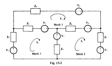
where  $I_1Z_1$ ,  $(I_1 - I_3)Z_2$ , and  $(I_1 - I_2)Z_3$  are the voltage drops across the impedances  $Z_1$ ,  $Z_2$ , and  $Z_3$ . Of course,  $V_1 + V_2 - V_3$  is the sum of the voltage rises from voltage sources in mesh 1. As a memory aid, a source voltage is added if it "aids" current flow—that is, if the principal current has a direction out of the positive terminal of the source. Otherwise, the source voltage is subtracted.
