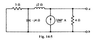
The Thévenin impedance  $\mathbf{Z}_{Th}$  is the impedance at terminals a and b with the current source replaced by an open circuit. By circuit reduction,
