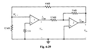
Observe that op amp 1 has no negative feedback and so is probably in saturation, and it is saturated at 14 V because of the 5 V applied to the *noninverting* input terminal. Assume this is so. Then this 14 V is an input to the circuit portion containing op amp 2, which is an inverter. Consequently,  $V_{20} = -(3/12)(14) = -3.5 \text{ V}$ . And, by voltage division,
