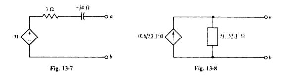
source. Therefore, the parallel impedance is  $3 - j4 = 5/(-53.1) \Omega$ , and the source current directed toward node a is
