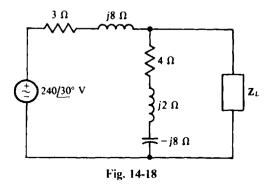
The Thévenin equivalent of the source circuit at the load terminals is needed. By voltage division,
