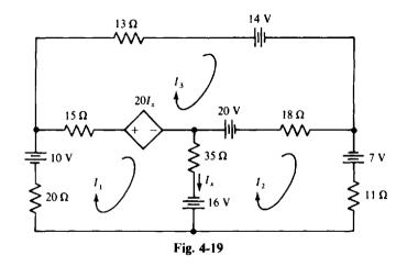
equations using the self- and mutual-resistance approach, and then add the dependent source expressions to the pertinent equations. The result of doing that here is
