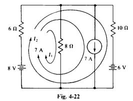
solved for. Also, only one loop current should flow through the 7-A source so that this loop current is known, making it unnecessary to apply KVL to the corresponding loop. There are other ways of selecting the loop current paths to satisfy these conditions.
