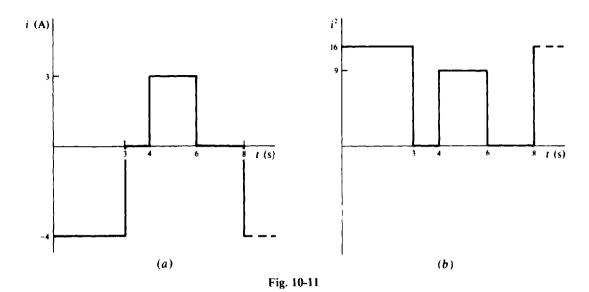
The first step is to square the wave, which has a period of 8 s. The squared wave is shown in Fig. 10-11b. The next step is to find the average of the squared wave, which can be found by dividing the area by the period: [16(3) + 9(6 - 4)] = 8.25. The last step is to find the square root of this average:  $I_{ctt} = 8.25 = 2.87 \text{ A}$ .
