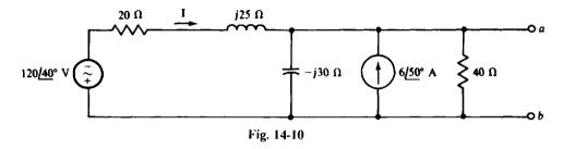
When the voltage source is replaced by a short circuit and the current source by an open circuit, the admittance at terminals a and b is
