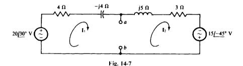
The Thévenin impedance  $\mathbf{Z}_{Th}$  can be found easily by replacing the voltage sources with short circuits and finding the impedances at terminals a and b. Since the short circuit places the right- and left-hand halves of the circuit in parallel.
