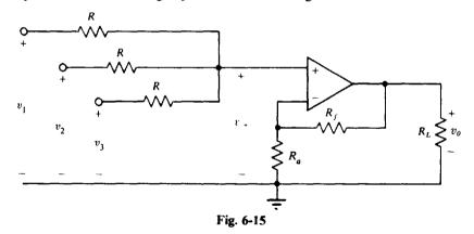
Clearly, in terms of  $v_+$ , this circuit is a noninverting amplifier. So,
