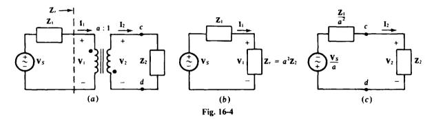
the usual manner. Then if the secondary winding voltage and current are also of interest, they can be obtained from the primary winding voltage and current.
