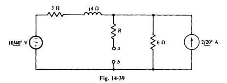
14.36 Find  $I_N$  and  $Z_{Th}$  for the Norton equivalent of the circuit shown in Fig. 14-39 for  $R = 2 \Omega$ .
