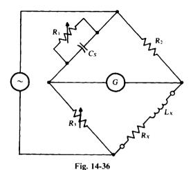
First, general formulas will be derived for  $R_X$  and  $L_X$  in terms of the other bridge components. Then, values will be substituted into these formulas to find  $R_X$  and  $L_X$  for the specified bridge. From a comparison of Figs. 14-3 and 14-36,  $\mathbf{Z}_2 = R_2$ ,  $\mathbf{Z}_3 = R_3$ ,  $\mathbf{Z}_X = R_X + j\omega L_X$ , and
