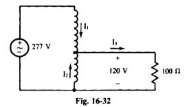
The resistor current is obviously  $I_3 = 120/100 = 1.2$  A. And the resistor receives  $120 \times 1.2 = 144$  VA. Since this is also the voltamperes supplied by the source, then  $277I_1 = 144$  and  $I_1 = 144/277 = 0.52$  A. Last, from KCL applied at the transformer winding tap,  $I_2 = I_3 - I_1 = 1.2 - 0.52 = 0.68$  A. Scalar addition can be used here since all three currents are in phase.
