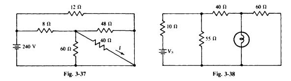
3.86 In the circuit shown in Fig. 3-38 there is a 120-V, 60-W light bulb. What must be the supply voltage  $V_s$  for the light bulb to operate under rated conditions?
