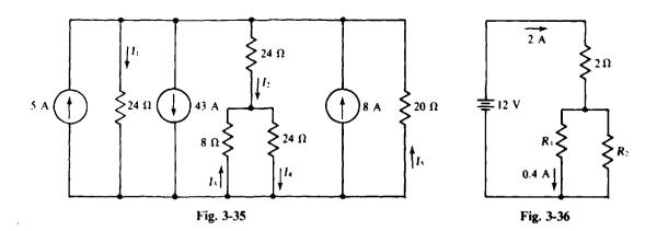
3.81 Find  $R_1$  and  $R_2$  for the circuit shown in Fig. 3-36.
