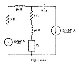
14.52 In the circuit shown in Fig. 14-47, move the  $-j8-\Omega$  impedance from in series with the current source to in parallel with it. Find the  $Z_L$  that absorbs maximum average power and find this power.
