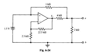
By inspection, the part of the circuit comprising the op amp and the 2.5-k $\Omega$  and 22.5-k $\Omega$  resistors is a noninverting amplifier. Consequently,
