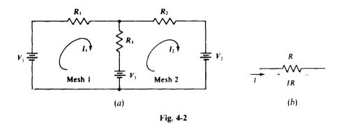
$I_1R_1$  and  $(I_1 - I_2)R_3$ , respectively, the latter because the current through  $R_3$  in the direction of  $I_1$  is  $I_1 - I_2$ . The total voltage rise from voltage sources is  $V_1 - V_3$ , in which  $V_3$  has a negative sign because it is a voltage drop. So, the mesh equation for mesh 1 is
