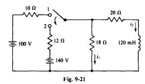
9.52 In the circuit shown in Fig. 9-21, the switch is thrown at t = 0 s to position 2 from position 1 where it has been a long time. Find the indicated currents at t = 0 + s and also at a long time later.
