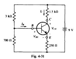
Perhaps the best way to find  $V_{CE}$  is to first find  $I_B$  and  $I_C$ , and from them the voltage drops across the 1.5-k $\Omega$  and 250- $\Omega$  resistors. Then, use KVL on the right-hand mesh and obtain  $V_{CE}$  from 9 V minus these two drops.
