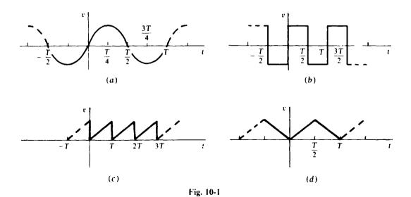
In these definitions, notice the terms wave and waveform. They do not refer to the same thing. A wave is a varying voltage or current, but a waveform is a graph of such a voltage or current. Often, however, these terms are used interchangeably...
