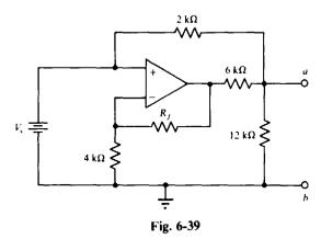
**6.46** Repeat Prob. 6.45 for  $V_s = 5 \text{ V}$  and  $R_f = 6 \text{ k}\Omega$ .
