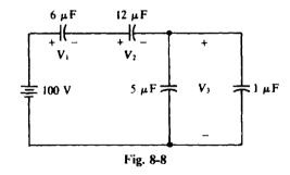
At the end opposite the source, the two parallel capacitors have an equivalent capacitance of  $5 + 1 = 6 \mu F$ . With this reduction, the capacitors are in series, making
