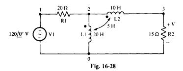
Figure 16-28 shows the PSpice circuit corresponding to the phasor-domain circuit of Fig. 16-27. The inductance values are based on a frequency of  $\omega = 1 \text{ rad/s}$ , which is selected for convenience. The coefficient of coupling needed for the circuit file is  $k = M/\sqrt{L_1L_2} = 5\sqrt{20 \times 10} = 0.353553$ .
