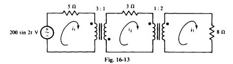
A good procedure is to find  $i_1$  using reflected resistances, then find  $i_2$  from  $i_1$ , and last find  $i_3$  from  $i_2$ . The 8  $\Omega$  reflects into the middle circuit as  $-8/2^2 = 2 \Omega$ , making a total resistance of  $-2 + 3 = 5 \Omega$  in the middle circuit. This  $5 \Omega$  reflects into the source circuit as  $-3^2(5) = 45 \Omega$ . Consequently,
