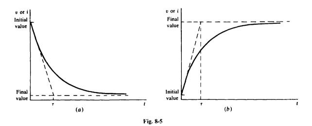
for all time greater than zero (t > 0 s). In these equations, v(0+) and i(0+) are initial values immediately after switching;  $v(\infty)$  and  $i(\infty)$  are final values; e = 2.718, the base of natural logarithms; and  $\tau$  is the time constant of the circuit of interest. These equations apply to all voltages and currents in a linear, RC, single-capacitor circuit in which the independent sources, if any, are all dc.
