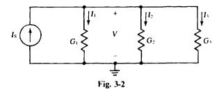
From this result it should be evident that, in general, the total conductance of parallel-connected resistors (parallel resistors) equals the sum of the individual conductances:
