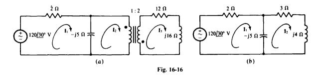
The 12- $\Omega$  resistance and the j16- $\Omega$  inductive impedance reflect into the primary circuit as a  $(1/2)^2(12) = 3-\Omega$  resistance and a series  $(1/2)^2(j16) = j4-\Omega$  inductive impedance in parallel with the  $-j5-\Omega$  capacitive impedance, as shown in Fig. 16-16b. The impedance of the parallel combination is
