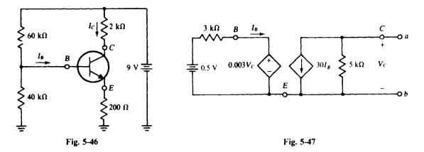
5.44 Find the Thévenin equivalent of the transistor circuit shown in Fig. 5-47. Reference  $V_{Th}$  positive toward terminal a.
