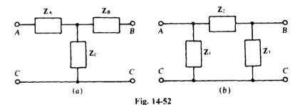
14.60 Transform the Π shown in Fig. 14-52*b* to the T in Fig. 14-52*a* for (a)  $\mathbf{Z}_1 = \mathbf{Z}_2 = \mathbf{Z}_3 = 36/-24$  Ω, and (b)  $\mathbf{Z}_1 = 15/-24$  Ω,  $\mathbf{Z}_2 = 14 - j20$  Ω,  $\mathbf{Z}_3 = 10 + j16$  Ω.
