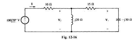
The current can be found by dividing the voltage by the total impedance, and this impedance can be found by combining impedances starting at the end of the circuit opposite the source. There, the series resistor and capacitor have a combined impedance of 15 - j30 = 33.5/-63.4  $\Omega$ . This can be combined in parallel fashion with the  $j20 \Omega$  of the parallel inductor:
