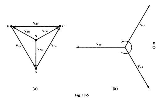
In a similar manner it can be shown for a balanced circuit that the line current phasor subscripts correspond to the phase sequence order in the same way as explained for the voltage phasor subscripts. Also, the same is true for either the first or the second subscripts of the phase current phasors for a balanced  $\Delta$  load. (A balanced  $\Delta$  load has three equal impedances.)
