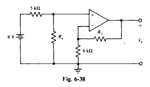
Assume for the op-amp circuit of Fig. 6-38 that  $R_a = 10 \text{ k}\Omega$  and that the op-amp saturation voltages are  $V_a = \pm 13 \text{ V}$ . Determine the range of resistances of  $R_f$  that will result in linear operation.
