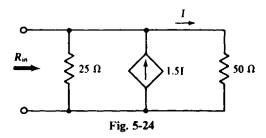
Since this circuit has a dependent source but no independent sources, the approach to finding the input resistance is to apply a source at the input. Then the input resistance is equal to the input voltage divided by the input current. A good source to apply is a 1-A current, as shown in Fig. 5-25.
