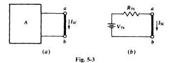
From  $V_{\text{Th}} = I_{\text{SC}}R_{\text{Th}}$ , it is evident that the Thévenin equivalent can be obtained by determining any two of the quantities  $V_{\text{Th}}$ ,  $I_{\text{SC}}$ , and  $R_{\text{Th}}$ . Common sense dictates that the two used should be the two that are the easiest to determine.
