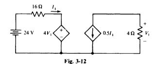
From KVL applied to the left-hand half of the circuit,  $16I_1 + 4V_1 = 24$ . And for the right-hand half of the circuit, Ohm's law gives
