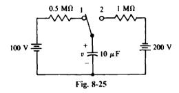
8.67 After a long time in position 2, the switch in the circuit shown in Fig. 8-25 is thrown at t = 0 s to position 1 for 4 s, after which it is returned to position 2. Find t for  $t \ge 0$  s.
