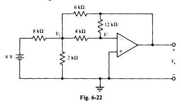
Since  $V_{-} = 0$  V, the node-voltage equations at the  $V_{1}$  and inverting-input terminal nodes are
