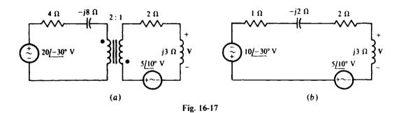
original impedance, and the voltage of the reflected voltage source is 1/a times the original voltage. Also, the polarity of the reflected voltage source is reversed because the dots are located at opposite ends of the windings. The result is shown in Fig. 16-17b. By voltage division,
