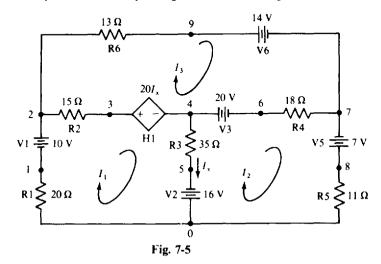
Since PSpice does not provide a power output except for the total power produced by independent voltage sources, the power absorbed by the dependent source must be calculated by hand after PSpice is used to obtain the voltage across the dependent source and the current flowing into the positive terminal of this source.
