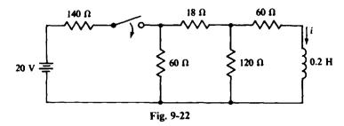
9.57 Assume that the switch in the circuit shown in Fig. 9-22 has been closed a long time. Find i as a function of time after the switch opens at t = 0 s.
