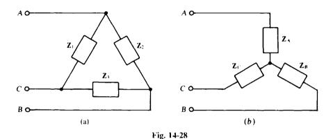
(a) Because all three  $\Delta$  impedances are the same, all three Y impedances are the same and each is equal to one-third of the common  $\Delta$  impedance:
