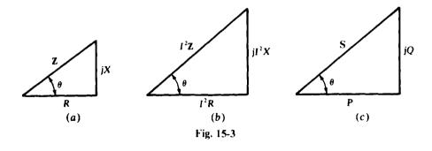
The length of the hypotenuse |S| = S, is called the *apparent power*. Its name comes from the fact that it is equal to the product of the input rms voltage and current:
