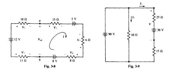
Since the 90-V source is across the  $10-\Omega$  resistor,  $I_1 = 90/10 = 9$  A. Around the outside loop in a clockwise direction, the voltage drop across the two resistors is  $(25 + 15)I_2 = 40I_2$ . This is equal to the sum of the voltage rises across the voltage sources in this outside loop:
