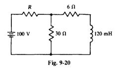
9.47 Find the time constant of the circuit shown in Fig. 9-20 for  $R = 90 \Omega$ .
