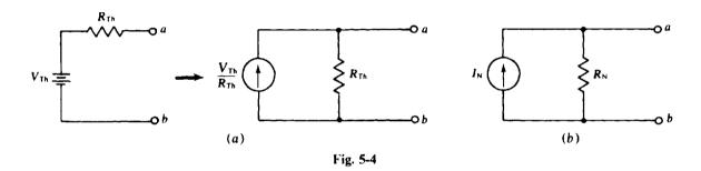
equal to the Norton current  $I_N$ . Often in circuit diagrams, the notation  $I_{SC}$  is used for the source current instead of  $I_N$ . Also, often  $R_{Th}$  is used for the resistance instead of  $R_N$ .
