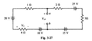
3.61 Use voltage division to find the voltage  $V_4$  in the circuit shown in Fig. 3-27.
