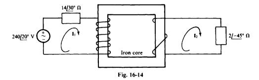
Because the primary has 6 turns and the secondary has 2 turns, the turns ratio is a = 6/2 = 3 and so the impedance reflected into the primary circuit is  $3^2(2/-45) = 18/-45 \Omega$ . Thus,
