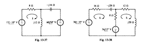
13.37 Find the mesh currents in the circuit shown in Fig. 13-38.
