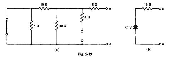
The fact that neither the 5- $\Omega$  nor the 4- $\Omega$  resistor has an effect on  $V_{Th}$  and  $R_{Th}$  leads to the generalization that resistors in parallel with ideal voltage sources, and resistors in series with ideal current sources, have no effect on voltages and currents elsewhere in a circuit.
