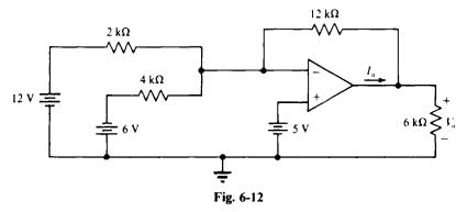
Because of the zero voltage drop across the op-amp input terminals, the voltage with respect to ground at the inverting input terminal is the same 5 V that is at the noninverting input terminal. With this voltage known, the voltage  $V_o$  can be determined from summing the currents flowing into the inverting input terminal:
