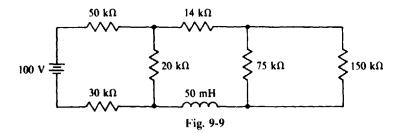
The time constant is  $LR_{Th}$ , where  $R_{Th}$  is the Thévenin resistance of the circuit at the inductor terminals. For this circuit.
