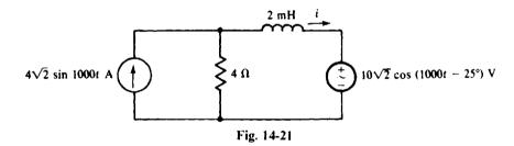
It is necessary to construct the corresponding phasor-domain circuit, as shown in Fig. 14-22. The current I can be considered to have a component I' from the current source and a component I' from the voltage source such that I = I' + I''. The component I' can be found by using current division after replacing the voltage source with a short circuit:
