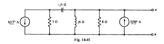
14.40 What resistor will draw a 2-A rms current when connected across terminals a and b of the circuit shown in Fig. 14-41?
