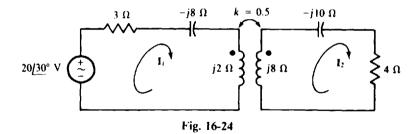
Before mesh equations can be written, the magnitude  $\omega M$  of  $j\omega M$  must be determined. From multiplying both sides of M=k,  $L_1L_2$  by  $\omega$ ,
