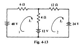
The self-resistance of mesh 1 is  $6 + 4 = 10 \Omega$ , the mutual resistance with mesh 2 is  $4 \Omega$ , and the sum of the source voltage rises in the direction of  $I_1$  is 40 - 12 = 28 V. So, the mesh 1 KVL equation is  $10I_1 - 4I_2 = 28$ .
