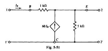
5.49 Find the output resistance at terminals 2 and 2' of the transistor circuit shown in Fig. 5-51 if a source with a 1-k $\Omega$  internal resistance is connected to terminals 1 and 1'. In finding the output resistance remember to replace the source by its internal resistance.
