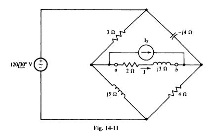
are the load impedances. With this done,  $Z_{Th}$  can be found after replacing the voltage source with a short circuit. This short circuit places the 3- $\Omega$  and j5- $\Omega$  impedances in parallel and also the  $-j4-\Omega$  and 4- $\Omega$  impedances in parallel. Since these two parallel arrangements are in series between terminals a and b.
