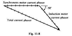
11.20 A synchronous motor draws a 9-A current from a 240-V, 60-Hz source. A parallel induction motor draws 8 A. If the synchronous motor current leads the applied voltage by 20°, and if the induction motor current lags this voltage by 30°, what is the total current drawn from the source? Find this current graphically and algebraically.
