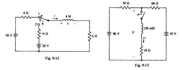
9.27 For the circuit shown in Fig. 9-13, find i for  $t \ge 0$  s if the switch is closed at t = 0 s after being open for a long time.
