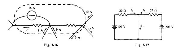
From KCL applied at the top middle node,  $I_3 = I_1 + I_2 = 5 - 8 = -3$  A. Of course the negative sign in the answer means that 3 A actually flows up through the short circuit, opposite the direction of the  $I_3$  current reference arrow.
