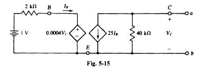
A good approach is to first find  $I_{SC}$ , which is the Norton current  $I_N$ ; next find  $V_{OC}$ , which is the Thévenin voltage  $V_{Th}$ ; and then take their ratio to obtain the Norton resistance  $R_N$ , which is the same as  $R_{Th}$ .
