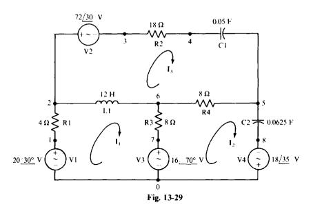
In the circuit file the frequency must be specified in hertz, which for 1 rad s is  $-1.2\pi = 0.159 155$  Hz. The circuit file corresponding to the PSpice circuit of Fig. 13-29 is as follows:
