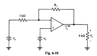
(a) Since for  $V_b = 0 \text{ V}$  the circuit is an inverter, the inverter voltage-gain formula can be used to obtain  $V_a$ .
