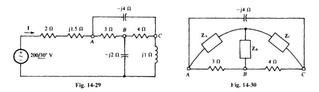
Extending between nodes A, B, and C there is a  $\Delta$ , as shown in Fig. 14-30, that can be transformed to the shown Y, with the result that the entire circuit becomes series-parallel and so can be reduced by combining impedances. The denominator of each  $\Delta$ -to-Y transformation formula is  $3 + 4 - j4 = 7 - j4 = 8.062/-29.7 \ \Omega$ . And by these formulas,
