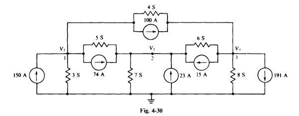
The self-conductances are 3+4+5=12 S for node 1, 5+6+7=18 S for node 2, and 6+4+8=18 S for node 3. The mutual conductances are 5 S for nodes 1 and 2, 6 S for nodes 2 and 3, and 4 S for nodes 1 and 3. The currents into the nodes from current sources are 150-100-74=-24 A for node 1, 74+15+23=112 A for node 2, and 100-191-15=-106 A for node 3. So, the nodal equations are
