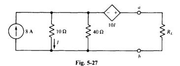
For maximum power transfer,  $R_L = R_{Th}$  and  $P_{max} = V_{Th}^2/(4R_{Th})$ . So, it is necessary to obtain the Thévenin equivalent of the portion of the circuit to the left of the a and b terminals.
