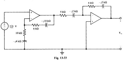
Since the first op-amp circuit has the configuration of a noninverting amplifier, and the second has that of an inverter, the pertinent formulas from Chap. 6 apply, with the R's replaced by Z's. So, with the impedances expressed in kilohms,
