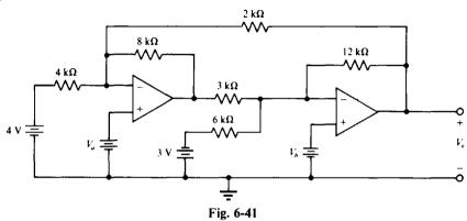
**6.50** Repeat Prob. 6.49 for  $V_a = 3 \text{ V}$  and  $V_b = 2 \text{ V}$ .
