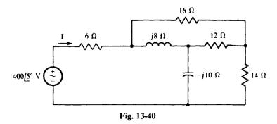
13.41 Use loop analysis to find the current flowing down through the capacitor in the circuit shown in Fig. 13-40.
