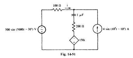
14.58 Find the average power absorbed by the  $200-\Omega$  resistor in the circuit shown in Fig. 14-51.
