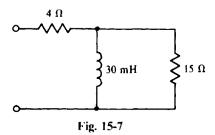
Because a circuit is specified, the power factor and capacitor are probably easier to find using impedance and admittance instead of powers. The power factor is the cosine of the impedance angle. Since the reactance of the inductor is  $-2\pi(60)(0.03) = 11.3 \Omega$ , the impedance of the circuit is
