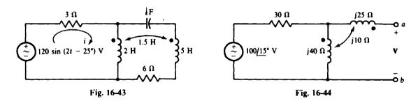
16.82 Find V in the circuit of Fig. 16-44. Then switch the dot on one winding and find V again.
