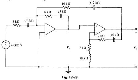
The first op-amp circuit can be considered to be similar to a summer with one input of 4/30 V and the other of  $V_o$ . Then the output  $V_a$  is
