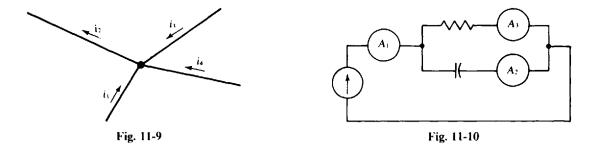
11.40 In the circuit shown in Fig. 11-10, ammeters  $A_1$  and  $A_2$  have readings of 4 and 3 A, respectively. What is the reading of ammeter  $A_3$ ?
