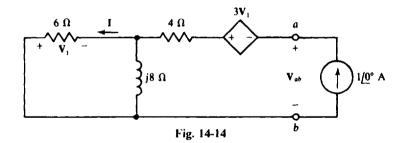
the circuit is different. The voltage  $V_1$  can be found from the current I flowing through the 6- $\Omega$  resistor across which  $V_1$  is taken. Since the 6- and  $j8-\Omega$  impedances are in parallel, and since 1/0 A from the current source flows into this parallel arrangement, I is, by current division,
