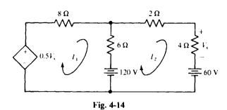
A good first step is to solve for the controlling quantity  $V_x$  in terms of the mesh current  $I_2$ . Clearly,  $V_x = 4I_2$ , and consequently the voltage of the dependent source is  $0.5V_x = 0.5(4I_2) = 2I_2$ . Then, the application of KVL to the meshes gives
