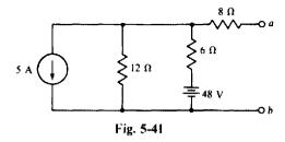
5.38 In the circuit shown in Fig. 5-41, change the 5-A current source to a 7-A current source, the  $12-\Omega$  resistor to an  $18-\Omega$  resistor, and the 48-V source to a 96-V source. Then find the Norton equivalent circuit with the current arrow directed toward terminal a.
