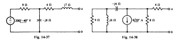
14.34 Find  $I_N$  and  $Z_{Th}$  for the Norton equivalent of the circuit shown in Fig. 14-38.
