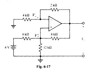
By nodal analysis at the noninverting input terminal,
