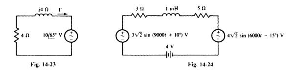
14.22 Although superposition does not usually apply to power calculations, it does apply to the calculation of average power absorbed when all sources are sinusoids of different frequencies. (A dc source can be considered to be a sinusoidal source of zero frequency.) Use this fact to find the average power absorbed by the 5- $\Omega$  resistor in the circuit shown in Fig. 14-24.
