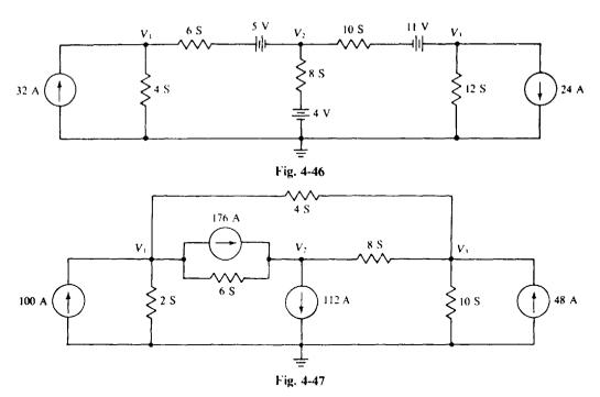
4.63 Repeat Prob. 4.62 with the three current-source changes of 176 to 108 A, 112 to 110 A, and 48 to 66 A.
