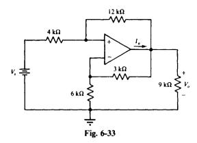
6.34 For the op-amp circuit of Fig. 6-33, find the range of  $V_s$  for linear operation if the op-amp saturation voltages are  $V_o = \pm 14 \text{ V}$ .
