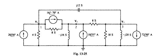
The self-admittances are 4+8+j12=12+j12 S for node 1, 8-j16+8=16-j16 S for node 2, and 8+18-j20+j12=26-j8 S for node 3. The mutual admittances are 8 S for nodes 1 and 2, j12 S for nodes 1 and 3, and 8 S for nodes 2 and 3. The currents flowing into the nodes from current sources are  $20/30^{\circ}-16/-70^{\circ}=27.7/64.7^{\circ}$  A for node 1,  $16/-70^{\circ}+18/35^{\circ}=20.8/-13.1^{\circ}$  A for node 2, and  $-72/30^{\circ}$  A for node 3. So, the nodal equations are
