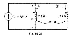
The mutual voltage terms have the same signs as the self-induced voltage terms because both current reference directions are into dotted ends. Upon rearrangement and simplification, these equations become
