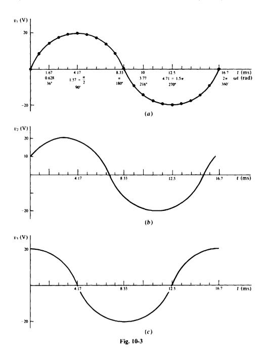
States. The period is T = 1/60 = 16.7 ms. A cycle of this voltage can be plotted by substituting, into 20 sin 377t, different times for t from the time interval of t = 0 s to t = 16.7 ms. Figure 10-3a shows the results of evaluating this sine wave at 21 different times and drawing a smooth curve through the plotted points. For comparison purposes, all three abscissa units seconds, radians, and degrees are shown.
