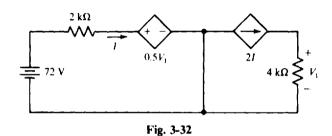
3.67 Calculate  $V_1$  in the circuit of Fig. 3-32.
