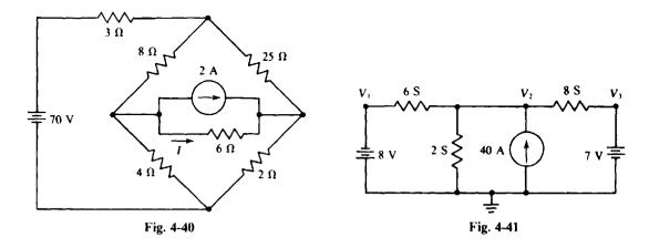
4.53 Obtain the node voltages in the circuit shown in Fig. 4-41.
