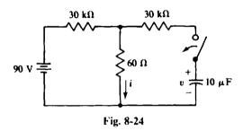
**8.65** Repeat Prob. 8.64 for v(0+) = 20 V and for the 60-k $\Omega$  resistor replaced by a 70-k $\Omega$  resistor.
