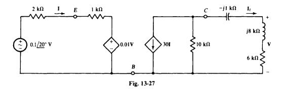
In the right-hand section of the circuit, the current  $I_L$  is, by current division,
