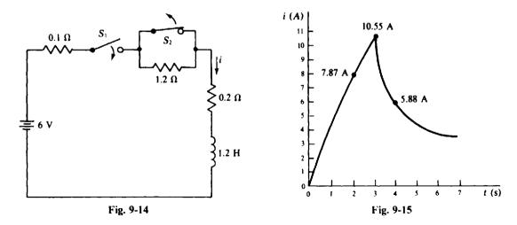
the current or time constant because this resistor is shorted by switch  $S_2$ . So, for the first three seconds,  $i = 20 - 20e^{-t/4}$  A, and from this,  $i(2) = 20 - 20e^{-2/4} = 7.87$  A.
