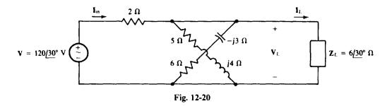
The current I<sub>in</sub> can be found from the source voltage divided by the input impedance Z<sub>in</sub>, which equals the  $2\Omega$  of the series resistor plus the total impedance of the three branches to the right of this resistor. Since these branches extend between the same two nodes, they are in parallel and have a total admittance Y that is the sum of the individual admittances:
