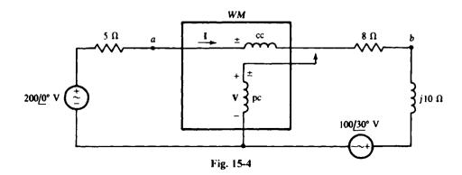
The wattmeter reading is equal to  $VI\cos\theta$ , where V is the rms voltage across the potential coil, I is the rms current flowing through the current coil, and  $\theta$  is the phase angle difference of the corresponding voltage and current phasors when they are referenced as shown with respect to the  $\pm$  markings of the wattmeter coils. These three quantities must be found to determine the wattmeter reading.
