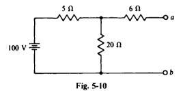
A good approach is to use Thévenin's theorem to simplify the circuit to the Thévenin equivalent of a  $V_{Th}$  voltage source in series with an  $R_{Th}$  resistor. Then the load resistor R is in series with these, and Ohm's law can be used to find R:
