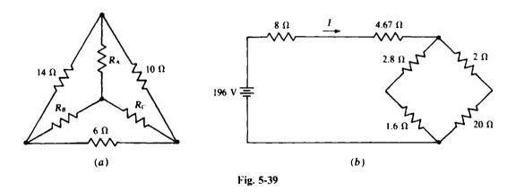
5.33 In the circuit shown in Fig. 5-38, what resistor R replacing the 20- $\Omega$  resistor causes the bridge to be balanced? Also, what is I then?
