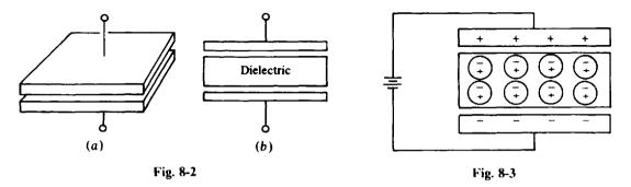
A voltage source connected to a capacitor, as shown in Fig. 8-3, causes the capacitor to become charged. Electrons from the top plate are attracted to the positive terminal of the source, and they pass through the source to the negative terminal where they are repelled to the bottom plate. Because each electron lost by the top plate is gained by the bottom plate, the magnitude of charge O is the same on
