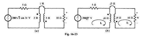
The first step is the construction of the phasor-domain circuit shown in Fig. 16-23b. Next, the mesh equations are written:
