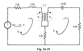
Because the 5- $\Omega$  resistor directly couples both halves of the circuit, the reflection approach cannot be used. However, two mesh equations can be written, and then these equations augmented with the voltage and current transformer equations to obtain four equations in terms of four unknowns:
