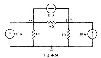
The self-conductance of node 1 is 6 + 4 = 10 S. The conductance mutual with node 2 is 6 S, and the sum of the currents into node 1 from current sources is 57 - 15 = 42 A. So, the node 1 KCL equation is  $10V_1 - 6V_2 = 42$ .
