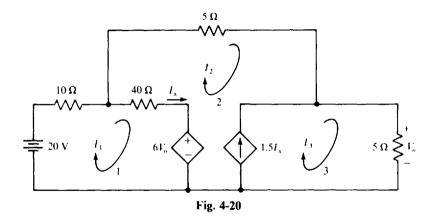
As always for a circuit containing dependent sources, a good first step is to solve for the dependent source controlling quantities in terms of the quantities being solved for, which are mesh currents here. Obviously,  $I_x = I_1 - I_2$  and  $V_0 = 5I_3$ . So, the dependent current source provides a current of  $1.5I_x = 1.5(I_1 - I_2)$  and the dependent voltage source provides a voltage of  $6V_0 = 6(5I_3) = 30I_3$ .
