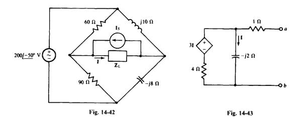
14.43 Find the output impedance of the circuit shown in Fig. 14-43.
