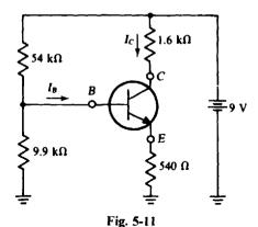
One way to find the base current is to break the circuit at the base lead and determine the Thévenin equivalent of the bias circuit. For this approach it helps to consider the 9-V source to be two 9-V sources, one of which is connected to the 1.6-k $\Omega$  collector resistor and the other of which is connected to the 54-k $\Omega$  bias resistor. Then the bias circuit appears as illustrated in Fig. 5-12a. From it, the voltage  $V_{Th}$  is, by voltage division.
