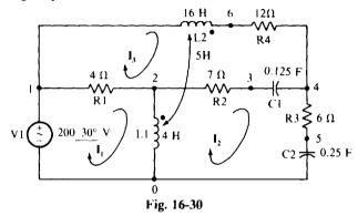
Figure 16-30 shows the PSpice circuit corresponding to the phasor-domain circuit of Fig. 16-29 of Prob. 16.40. As usual, the inductances and capacitances are based on the frequency  $\omega = 1$  rad s. The coefficient of coupling needed for the circuit file is  $k = M \sqrt{L_1 L_2} = 5 \sqrt{4 \times 16} = 0.625$ .
