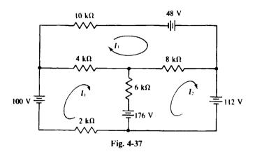
4.43 Double the voltages of the voltage sources in the circuit shown in Fig. 4-37 and redetermine the mesh currents. Compare them with the original mesh currents.
