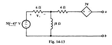
Because of the series arm with dependent source connected to terminal a,  $V_{Th}$  is easier to find than  $I_N$ . This voltage is equal to the sum of the voltage drops across the  $j8-\Omega$  impedance and the  $3V_1$  dependent voltage source. (Of course, the  $4-\Omega$  resistor has a 0-V drop.) It is usually best to first solve for the controlling quantity, which here is the voltage  $V_1$  across the  $6-\Omega$  resistor. By voltage division,
