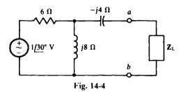
The Thévenin impedance  $\mathbf{Z}_{Th}$  is the impedance at terminals a and b with the load impedance removed and the voltage source replaced by a short circuit. From combining impedances.
