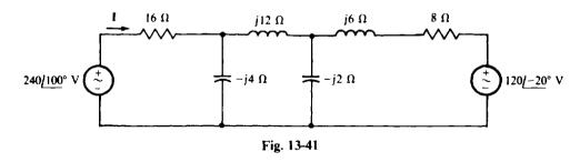
13.43 For the circuit shown in Fig. 13-41, use loop analysis to find the current flowing down through the capacitor that has the reactance of  $-j2 \Omega$ .
