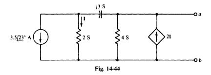
14.46 In the circuit shown in Fig. 14-44, reverse the I reference direction—have it up instead of down—and find Is and Z<sub>1b</sub> for the Norton equivalent circuit.
