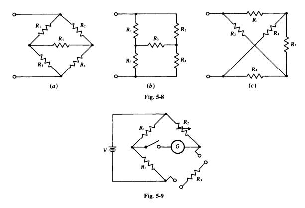
For a resistance measurement, the resistance  $R_2$  of the variable resistor is adjusted until the galvanometer needle does not deflect when the switch in the center branch is closed. This lack of deflection is the result of zero voltage across the galvanometer, and this means that, even with the switch open, the voltage across  $R_1$  equals that across  $R_2$ , and the voltage across  $R_3$  equals that across  $R_X$ . In this condition the bridge is said to be balanced. By voltage division,
