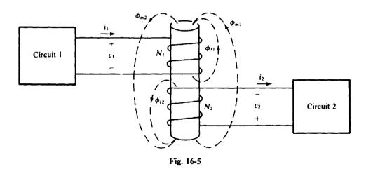
Figure 16-5 shows two circuits coupled by an air-core transformer. Current  $i_1$  produces a mutual flux  $\phi_{m1}$  and a leakage flux  $\phi_{l1}$ , and current  $i_2$  produces a mutual flux  $\phi_{m2}$  and leakage flux  $\phi_{l2}$ . As mentioned, a mutual flux couples both windings, but a leakage flux couples only one winding.
