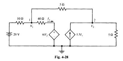
The controlling current  $I_x$  expressed in terms of node voltages is  $I_x = (V_1 - 6V_2)/40$ . So, the dependent current source provides a current of  $1.5I_x = 1.5(V_1 - 6V_2)/40$ . Applying KCL to nodes 1 and 2 produces
