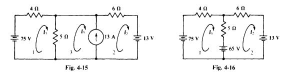
One analysis approach is to transform the 13-A current source and parallel 5- $\Omega$  resistor into a voltage source, as shown in the circuit of Fig. 4-16.
