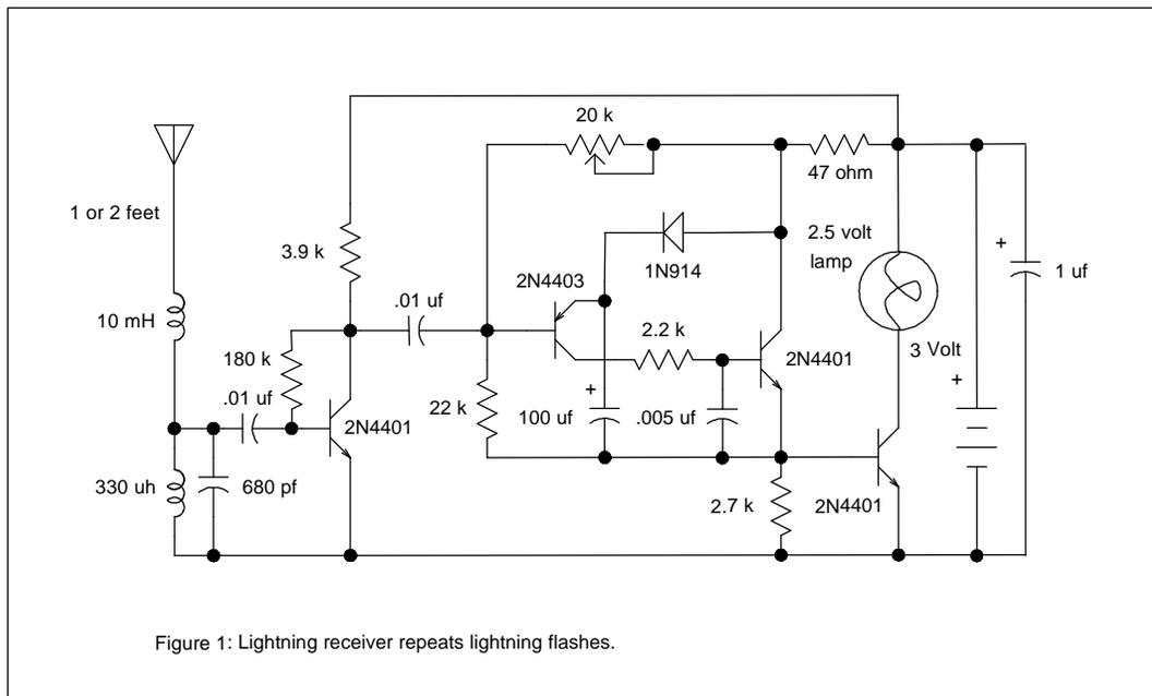
Figure 1: Lightning receiver repeats lightning flashes.
