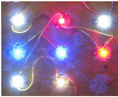
Fig. 4. Realized lamp module with one warm white, three neutral white; one blue, one royal blue one red and one deep red LEDs.
