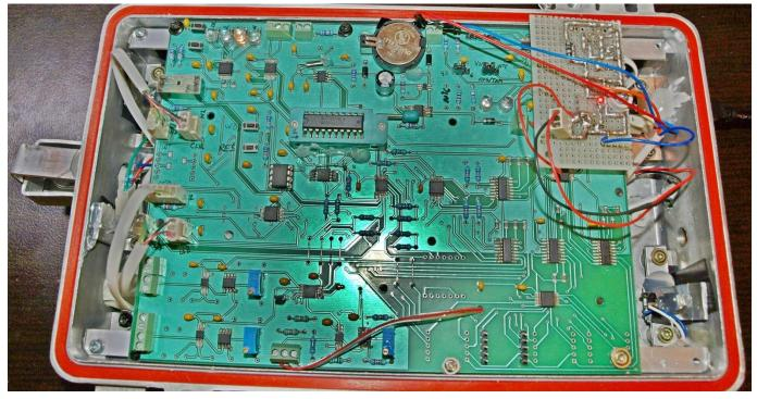
Fig. 1 – Evaluation board of the Adaptive Weather Station
