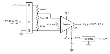
Figure 60. ±10-V, 4-mA to 20-mA PLC Input
