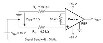
Figure 59. Example Application with G = 10 V/V and 1-V Differential Voltage
