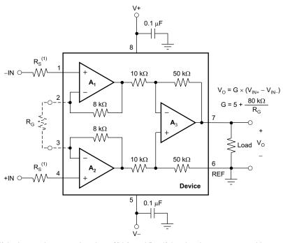
(1) This resistor is optional if the input voltage remains above  $[(V-)-2\ V]$  or if the signal source current drive capability is limited to less than 3.5 mA. See the *Input Protection* section for more details.
