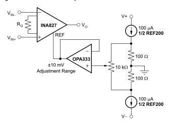
Figure 55. Optional Trimming of Output Offset Voltage
