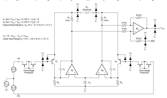
Figure 56. INA827 Simplified Circuit Diagram
