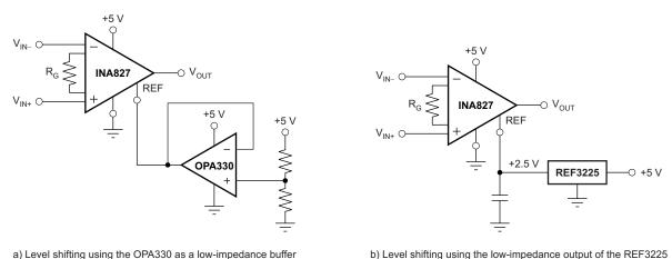
Figure 58. Options for Low-Impedance Level Shifting
