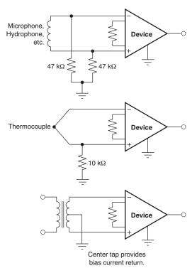
Figure 57. Providing an Input Common-Mode Current Path
