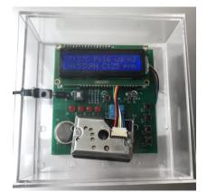
Fig. 6. The portable sensory box for monitoring of air pollution.
