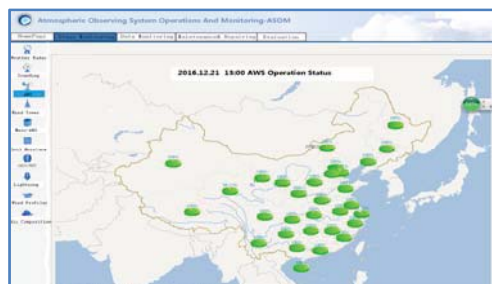
Fig.2 all surface weather stations running status monitoring from ASOM ( All provincial AWSs hourly status real-time monitoring display, Round cakes and data represent each province's normal AWSs, abnormal AWSs and fault AWSs ration Statistics
