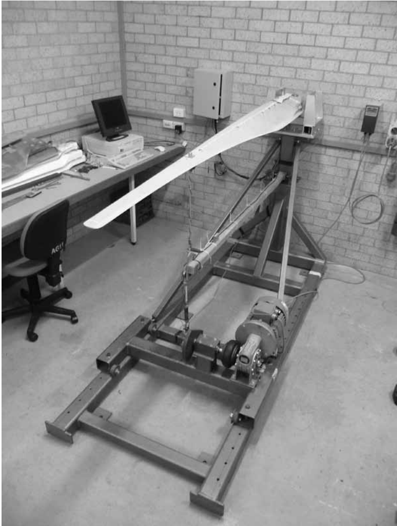
13.9 Fatigue test rig with 2.5 m blade. The safety cage has been removed to show blade driven by the hinged arm in the middle of the photo. Strain gauges and their electrical connections can be seen on the pressure (upper) surface.
