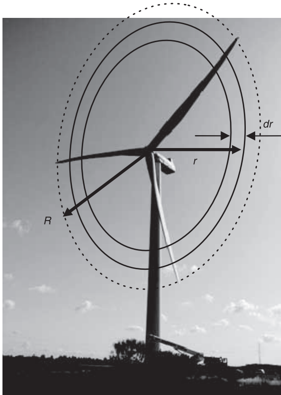
6.4 Sketch of the division of a wind turbine rotor into annular elements (Photo by Christian Bak: NM80 at Tjæreborg Enge, Denmark).
