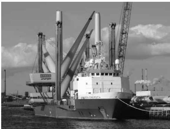
18.4 Examples of external cranes for replacement of large components; jack-up barge ODIN (top) and crane ship Sea Energy (bottom).
