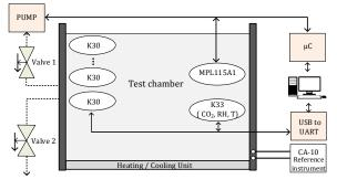
Fig. 1. Experimental set-up
