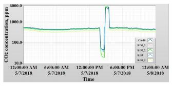
Fig. 3. 24 hours of measurements of carbon dioxide mixing ratios from two K30 NDIR sensors and the CA-10  $CO_2$  Analyzer
