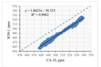
Fig. 4. Calibration function of K30-1 Sensor vs CA-10  $CO_2$ Analyzer
