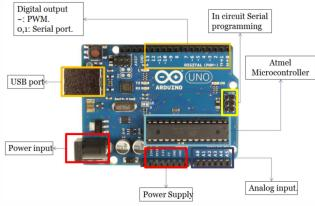
Fig. 1: Arduino UNO Board
