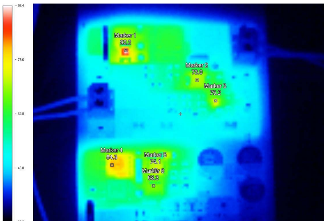
Fig. 12. Thermography image of the experimentally examined converters.
