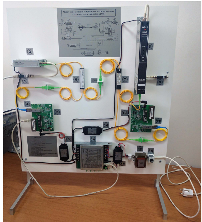
Fig. 6. Overall view of the implemented practical model for management, monitoring and research of passive optical network
