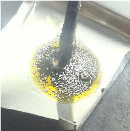
Fig. 4. Stage of solder paste melting with original flux in large crucible.
