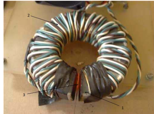
Fig. 1. Induction coil for heating in a magnetic circuit.
