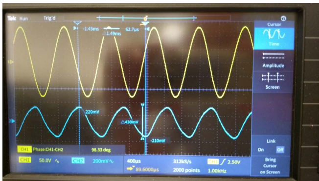
Fig.7. Oscillograms measured with the setup presented on Fig 6; upper line - U_D , lower line - U_R
