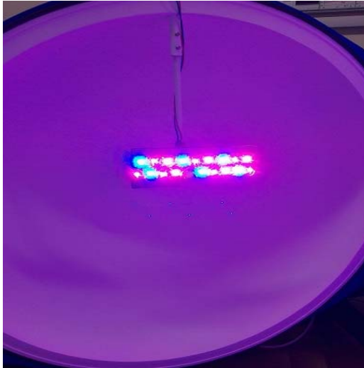
Fig. 5. Experimental LED module in the integrating sphere.
