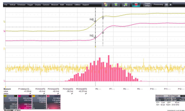
Fig. 6. Backplane clock 100MHz signal skew.
