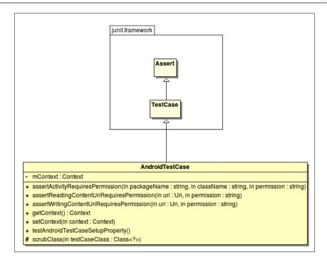
Use this class when you need access to an Activity Context like Resources, databases, or files in the filesystem. Context is stored as a field in this class conveniently named mContext and can be used inside the tests if needed. The getContext() method can be used too.
