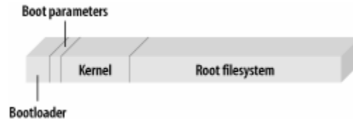
Figure 2-5. Typical solid state storage device layout
