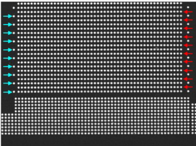
Figure 3: Both n^+ diffusion contacts of odd rows (indicated by blue arrows) and p^+ contacts of even rows (indicated by red arrows) could not be distinguished by contrast difference using FIB PVC.
