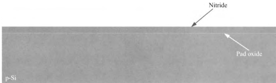
Figure 7.29 STI film stack. Silicon nitride deposited by LPCVD at approximately 800 °C.
