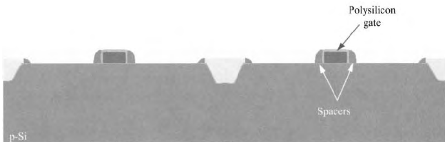
Figure 7.55 Dry, anisotropic, end-pointed reactive ion etch of spacer nitride yielding gate sidewall spacers.
