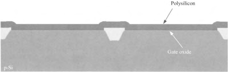
Figure 7.47 Polysilicon deposition via LPCVD at approximately 550 °C. Note that the polysilicon deposition must occur immediately following gate oxidation.
