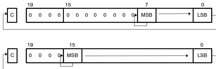
Figure 4-40. Rotate Right Arithmetically RRA.B and RRA.W
