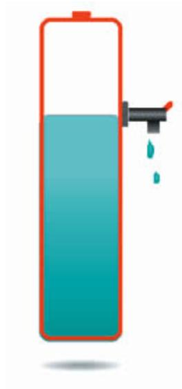
**Figure 6-5: Illustration of equipment with high cut-off voltage.**
