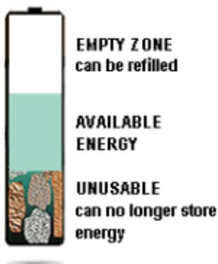
**Figure 6-1: Battery charge capacity.**
