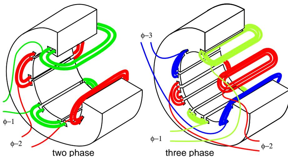
Above, the windings for both a two-phase motor and a three-phase motor have been installed in the stator slots. The coils are wound on an external fixture, then worked into the slots. Insulation wedged between the coil periphery and the slot protects against abrasion.
