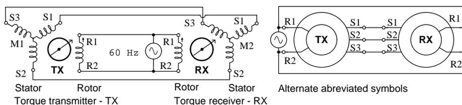
Synchro stators are wound with 3-phase windings brought out to external terminals. The single rotor winding of a torque transmitter or receiver is brought out by brushed slip rings. Synchro transmitters and receivers are electrically identical. However, a synchro receiver has inertial damping built in. A synchro torque transmitter may be substituted for a torque receiver.
