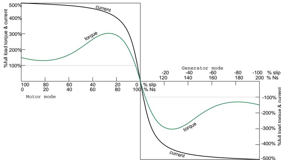
Such an *induction generator* must be excited by a "live" source of 50 or 60 Hz power. No power can be generated in the event of a power company power failure. This type of alternator appears to be unsuited as a standby power source. As an auxiliary power wind turbine generator, it has the advantage of not requiring an automatic power failure disconnect switch to protect repair crews.
