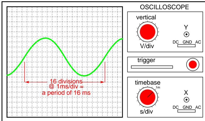
$$\text{Frequency} = \frac{1}{\text{period}} = \frac{1}{16 \text{ ms}} = 62.5 \text{ Hz}$$
