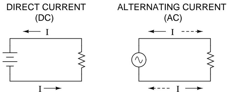
Whereas the familiar battery symbol is used as a generic symbol for any DC voltage source, the circle with the wavy line inside is the generic symbol for any AC voltage source.
