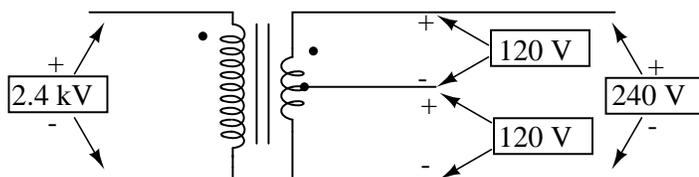
If the AC power comes directly from a generator (alternator), the coils can be similarly center-tapped for the same effect. The extra expense to include a center-tap connection in a transformer or alternator winding is minimal.
