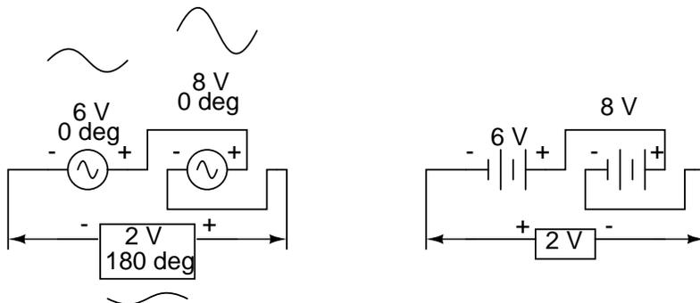
Note how the polarities appear to be opposed to each other now, due to the reversal of wire connections on the 8 volt source. Since both sources are described as having equal phase angles ( $0^\circ$ ), they truly are opposed to one another, and the overall effect is the same as the former scenario with "additive" polarities and differing phase angles: a total voltage of only 2 volts.
