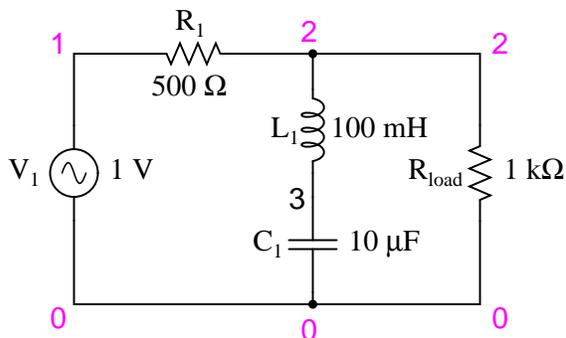
When the series LC combination reaches resonance, its very low impedance shorts out the signal, dropping it across resistor  $R_1$  and preventing its passage on to the load.
