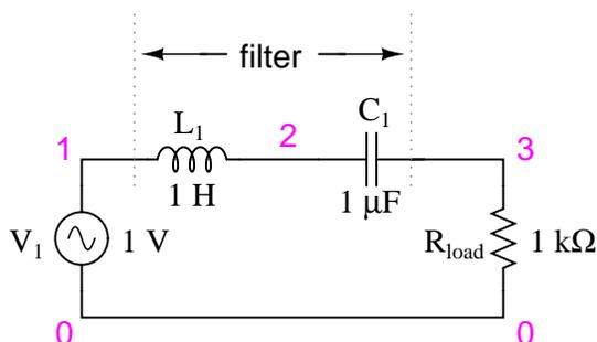
Series LC components pass signal at resonance, and block signals of any other frequencies from getting to the load.
