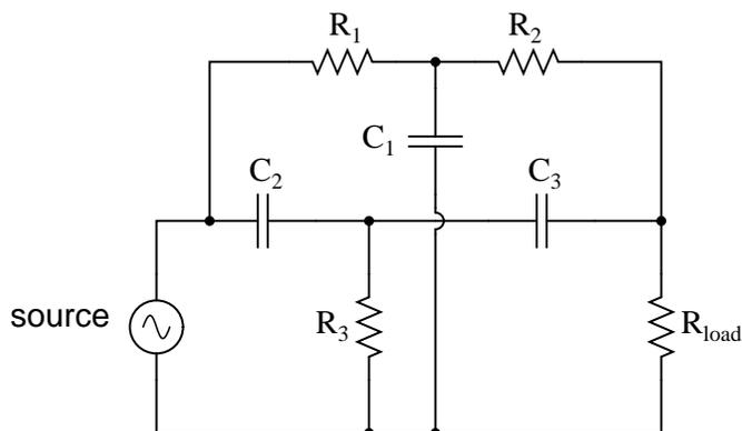
The low-pass filter section is comprised of  $R_1$ ,  $R_2$ , and  $C_1$  in a "T" configuration. The high-pass filter section is comprised of  $C_2$ ,  $C_3$ , and  $R_3$  in a "T" configuration as well. Together, this arrangement is commonly known as a "Twin-T" filter, giving sharp response when the component values are chosen in the following ratios:
