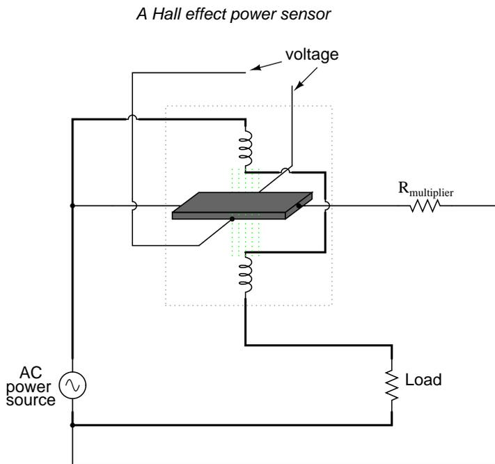
Not only will the output voltage of the Hall effect device be the representation of instantaneous power at any point in time, but it will also be a DC signal! This is because the Hall voltage polarity is dependent upon *both* the polarity of the magnetic field and the direction of current through the conductor. If both current direction and magnetic field polarity reverses – as it would ever half-cycle of the AC power – the output voltage polarity will stay the same.
