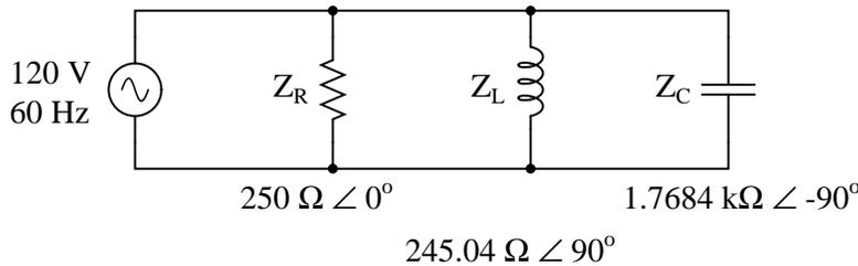
With all component values expressed as impedances ( $Z$ ), we can set up an analysis table and proceed as in the last example problem, except this time following the rules of parallel circuits instead of series:
