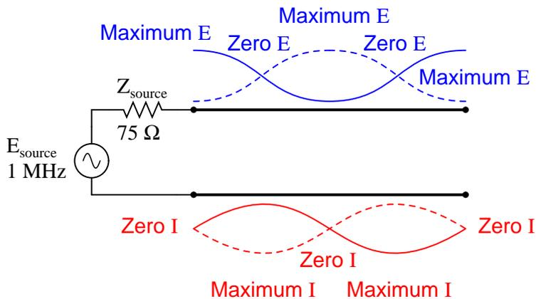
In a similar fashion, a short-circuited transmission line generates standing waves, although the node and antinode assignments for voltage and current are reversed: at the shorted end of the line, there will be zero voltage (node) and maximum current (antinode). What follows is the SPICE simulation and illustrations of what happens at all the interesting frequencies: 0 Hz, 250 kHz, 500 kHz, 750 kHz, and 1 MHz. The short-circuit jumper is simulated by a  $1\ \mu\Omega$  load impedance:
