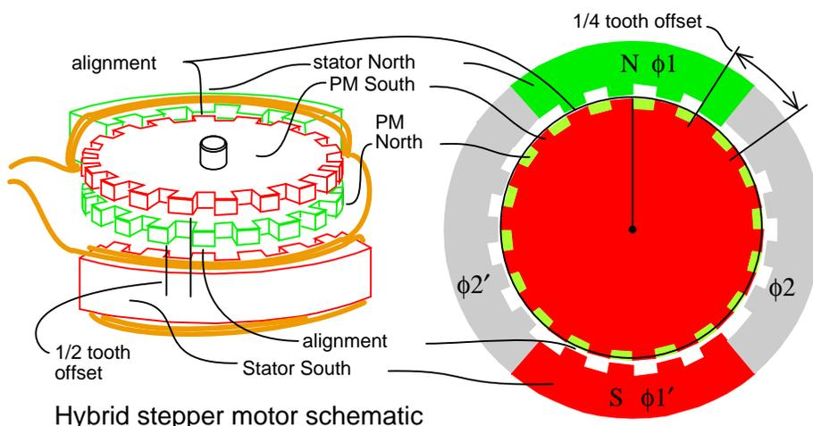
Hybrid stepper motor schematic
