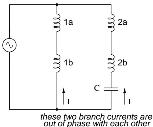
That phase shift creates magnetic fields from coils 2a and 2b that are equally out of step with the fields from coils 1a and 1b. The result is a set of magnetic fields with a definite phase rotation. It is this phase rotation that pulls the rotating magnet around in a definite direction.
