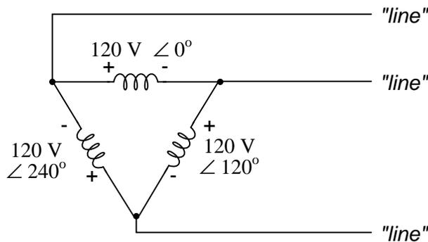
At first glance it seems as though three voltage sources like this would create a short-circuit, electrons flowing around the triangle with nothing but the internal impedance of the windings to hold them back. Due to the phase angles of these three voltage sources, however, this is not the case.
