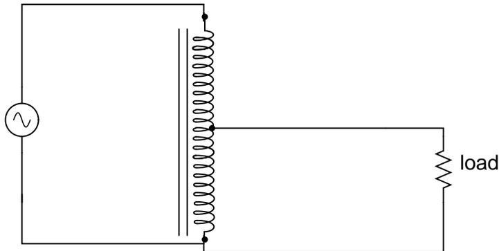
Autotransformers find popular use in applications requiring a slight boost or reduction in voltage to a load. The alternative with a normal (isolated) transformer would be to either have just the right primary/secondary winding ratio made for the job or use a step-down configuration with the secondary winding connected in series-aiding ("boosting") or series-opposing ("bucking") fashion. Primary, secondary, and load voltages are given to illustrate how this would work.
