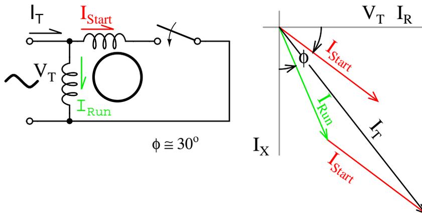
This motor has more starting torque than a shaded pole motor (next section), but not as much as a two phase motor built from the same parts. The current density in the auxiliary winding is so high during starting that the consequent rapid temperature rise precludes frequent restarting or slow starting loads.
