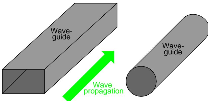
Waveguides are practical only for signals of extremely high frequency, where the wavelength approaches the cross-sectional dimensions of the waveguide. Below such frequencies, waveguides are useless as electrical transmission lines.
