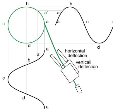
Above we illustrate that the two  $90^\circ$  phase shifted sine waves are applied to oscilloscope deflection plates which are at right angles in space. If this were not the case, a one dimensional line would display. The combination of  $90^\circ$  phased sine waves and right angle deflection, results in a two dimensional pattern— a circle. This circle is traced out by a counterclockwise rotating spot.
