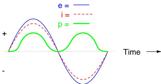
Note that the waveform for power is always positive, never negative for this resistive circuit. This means that power is always being dissipated by the resistive load, and never returned to the source as it is with reactive loads. If the source were a mechanical generator, it would take 240 watts worth of mechanical energy (about 1/3 horsepower) to turn the shaft.
