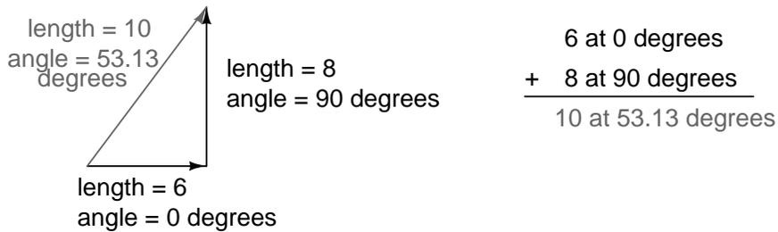
If two AC voltages –  $90^\circ$  out of phase – are added together by being connected in series, their voltage magnitudes do not directly add or subtract as with scalar voltages in DC. Instead, these voltage quantities are complex quantities, and just like the above vectors, which add up in a trigonometric fashion, a 6 volt source at  $0^\circ$  added to an 8 volt source at  $90^\circ$  results in 10 volts at a phase angle of  $53.13^\circ$ :
