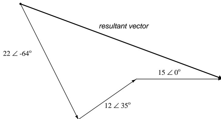
In order to determine what the resultant vector's magnitude and angle are without resorting to graphic images, we can convert each one of these polar-form complex numbers into rectangular form and add. Remember, we're *adding* these figures together because the polarity marks for the three voltage sources are oriented in an additive manner:
