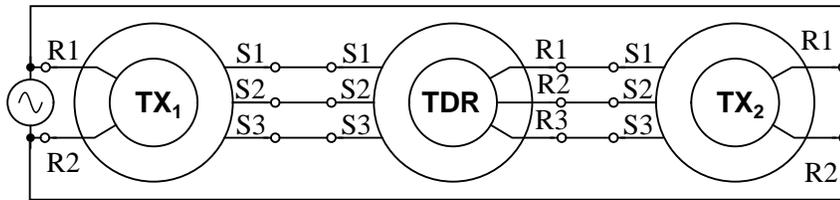
TDR subtraction:  $\angle TDR = \angle TX_1 - \angle TX_2$
