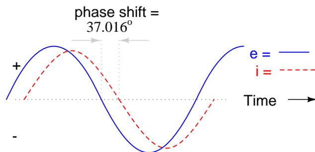
For the resistor and the inductor, the phase relationships between voltage and current haven't changed. Voltage across the resistor is in phase ( $0^\circ$  shift) with the current through it; and the voltage across the inductor is  $+90^\circ$  out of phase with the current going through it. We can verify this mathematically:
