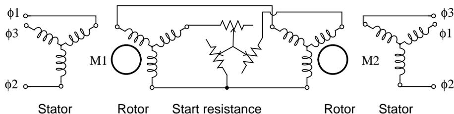
The rotors may be stationary. If one rotor is moved through an angle  $\theta$ , the other selsyn shaft will move through an angle  $\theta$ . If drag is applied to one selsyn, this will be felt when attempting to rotate the other shaft. While multi-horsepower (multi-kilowatt) selsyns exist, the main application is small units of a few watts for instrumentation applications— remote position indication.
