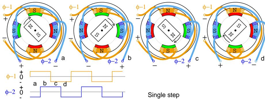
Single step bipolar drive is shown above. The step angle is the same as for wave drive. Unipolar drive (not shown) would require a pair of unipolar waveforms for each of the above bipolar waveforms applied to the ends of a center tapped winding.
