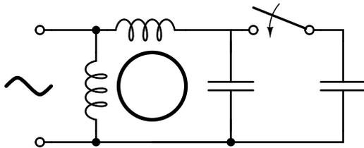
A motor starting capacitor may be a double-anode non-polar electrolytic capacitor which could be two + to + (or - to -) series connected polarized electrolytic capacitors. Such AC rated electrolytic capacitors have such high losses that they can only be used for intermittent duty (1 second on, 60 seconds off) like motor starting. A capacitor for motor running must not be of electrolytic construction, but a lower loss polymer type.
