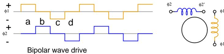
The above waveforms are bipolar because both polarities, (+) and (-) are required to drive the stepper. The coil magnetic field reverses because the current was reversed. Below, the waveforms are of only positive polarity.
