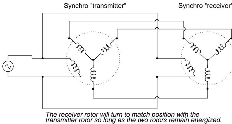
Such "transmitter/receiver" pairs have been used on ships to relay rudder position, or to relay navigational gyro position over fairly long distances. The only difference between the "transmitter" and the "receiver" is which one gets turned by an outside force. The "receiver" can just as easily be used as the "transmitter" by forcing its shaft to turn and letting the synchro on the left match position.
