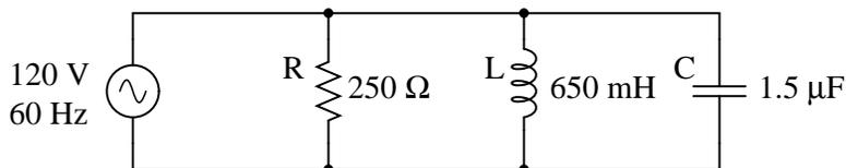
The fact that these components are connected in parallel instead of series now has absolutely no effect on their individual impedances. So long as the power supply is the same frequency as before, the inductive and capacitive reactances will not have changed at all:
