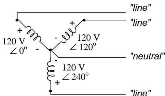
The three conductors leading away from the voltage sources (windings) toward a load are typically called *lines*, while the windings themselves are typically called *phases*. In a Y-connected system, there may or may not be a neutral wire attached at the junction point in the middle, although it certainly helps alleviate potential problems should one element of a three-phase load fail open, as discussed earlier:
