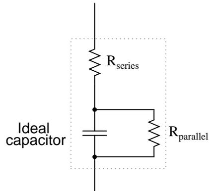
Fortunately, these stray resistances are usually of modest impact (low series resistance and high parallel resistance), much less significant than the stray resistances present in an average inductor.
