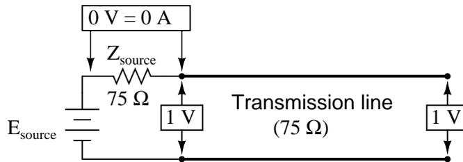
At 250 kHz, we see zero voltage and maximum current at the source-end of the transmission line, yet still full voltage at the load-end:
