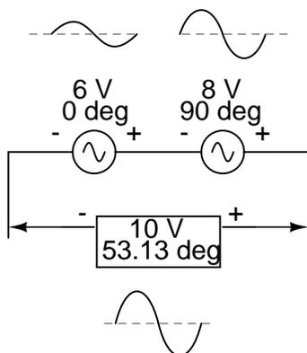
Compared to DC circuit analysis, this is very strange indeed. Note that it's possible to obtain voltmeter indications of 6 and 8 volts, respectively, across the two AC voltage sources, yet only read 10 volts for a total voltage!
