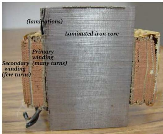
This is a step-down transformer, as evidenced by the high turn count of the primary winding and the low turn count of the secondary. As a step-down unit, this transformer converts high-voltage, low-current power into low-voltage, high-current power. The larger-gauge wire used in the secondary
