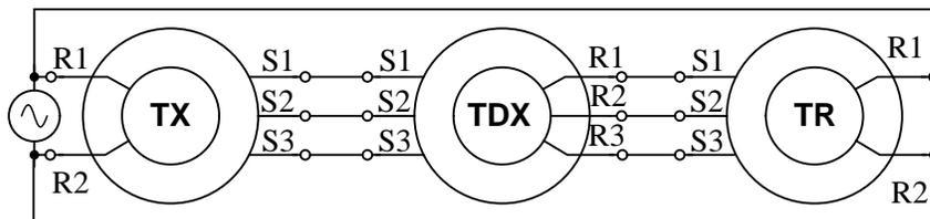
TDX subtraction:  $\angle_{\text{TX}} - \angle_{\text{TDX}} = \angle_{\text{TR}}$
