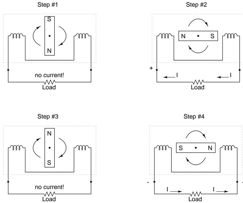
Notice how the polarity of the voltage across the wire coils reverses as the opposite poles of the rotating magnet pass by. Connected to a load, this reversing voltage polarity will create a reversing current direction in the circuit. The faster the alternator's shaft is turned, the faster the magnet will spin, resulting in an alternating voltage and current that switches directions more often in a given amount of time.
