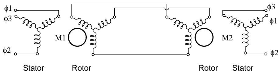
Instrumentation selsyns have no use for starting resistors. They are not intended to be self rotating. Since the rotors are not shorted out nor resistor loaded, no starting torque is developed. However, manual rotation of one shaft will produce an unbalance in the rotor currents until the parallel unit's shaft follows. Though we show three phase rotors above, a single phase rotor is sufficient as shown below. Note that a common source of three phase power is applied to both stators above.
