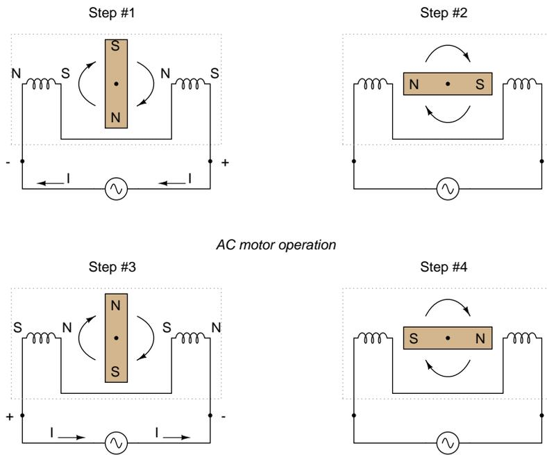
If the rotating magnet is able to keep up with the frequency of the alternating current energizing the electromagnet windings (coils), it will continue to be pulled around clockwise. However, clockwise is not the only valid direction for this motor's shaft to spin. It could just as easily be powered in a counter-clockwise direction by the same AC voltage waveform:
