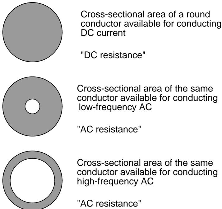
The electrical resistance of the conductor with all its cross-sectional area in use is known as the "DC resistance," the "AC resistance" of the same conductor referring to a higher figure resulting
