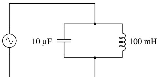
In the above circuit, we have a 10  $\mu\text{F}$  capacitor and a 100 mH inductor. Since we know the equations for determining the reactance of each at a given frequency, and we're looking for that point where the two reactances are equal to each other, we can set the two reactance formulae equal to each other and solve for frequency algebraically:
