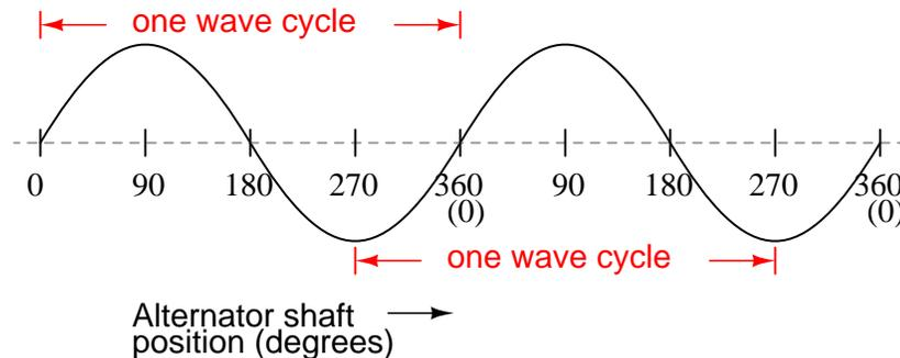
Since the horizontal axis of this graph can mark the passage of time as well as shaft position in degrees, the dimension marked for one cycle is often measured in a unit of time, most often seconds or fractions of a second. When expressed as a measurement, this is often called the *period* of a wave. The period of a wave in degrees is *always* 360, but the amount of time one period occupies depends on the rate voltage oscillates back and forth.
