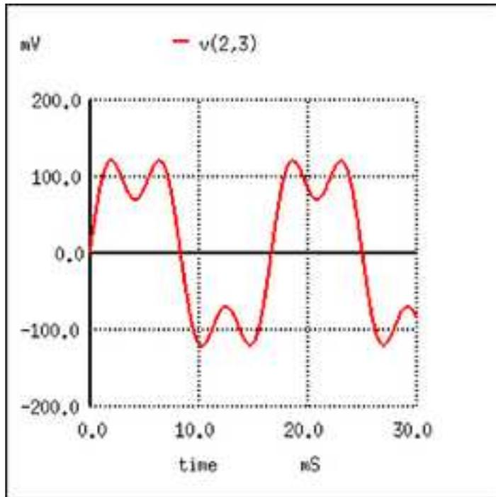
fourier components of transient response v(2,3)
