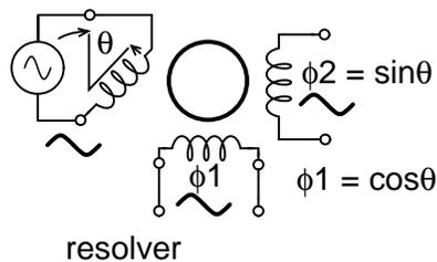
For example, a black-box within a radar encodes the distance to a target as a sine wave proportional voltage  $V$ , with the bearing angle as a shaft angle. Convert to X and Y co-ordinates. The sine wave is fed to the rotor of a resolver. The bearing angle shaft is coupled to the resolver shaft. The coordinates (X, Y) are available on the resolver stator coils:
