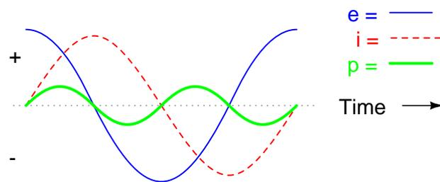
Note that the power alternates equally between cycles of positive and negative. This means that power is being alternately absorbed from and returned to the source. If the source were a mechanical generator, it would take (practically) no net mechanical energy to turn the shaft, because no power would be used by the load. The generator shaft would be easy to spin, and the inductor would not become warm as a resistor would.
