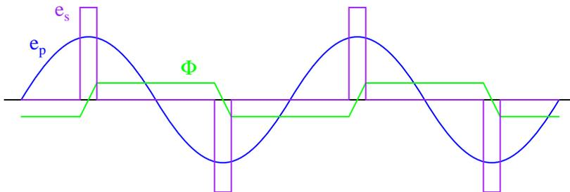
Another cause of abnormal transformer core saturation is operation at frequencies lower than normal. For example, if a power transformer designed to operate at 60 Hz is forced to operate at 50 Hz instead, the flux must reach greater peak levels than before in order to produce the same opposing voltage needed to balance against the source voltage. This is true even if the source voltage is the same as before.
