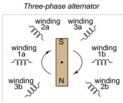
Together, the six "pole" windings of a three-phase alternator are connected to comprise three winding pairs, each pair producing AC voltage with a phase angle  $120^\circ$  shifted from either of the other two winding pairs. The interconnections between pairs of windings (as shown for the single-phase alternator: the jumper wire between windings 1a and 1b) have been omitted from the three-phase alternator drawing for simplicity.
