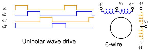
The above waveforms are unipolar because only one polarity is required. This simplifies the drive electronics. There are twice as many waveforms because a pair of (+) waves is required to produce an alternating magnetic field by application to opposite ends of a center tapped coil. The motor requires alternating magnetic fields. These may be produced by either unipolar or bipolar waves. However, motor coils must have center taps for unipolar drive.
