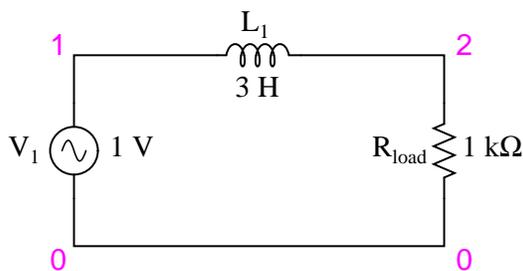
The inductor's impedance increases with increasing frequency. This high impedance in series tends to block high-frequency signals from getting to the load. This can be demonstrated with a SPICE analysis:
