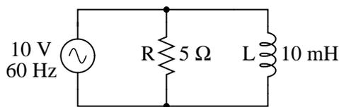
Because the power source has the same frequency as the series example circuit, and the resistor and inductor both have the same values of resistance and inductance, respectively, they must also have the same values of impedance. So, we can begin our analysis table with the same "given" values:
