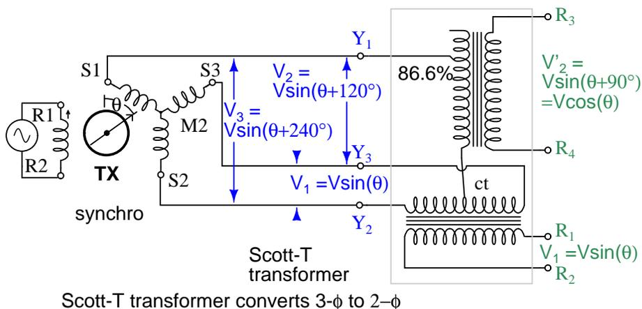
It is possible to derive resolver-like quadrature angular components from a synchro transmitter by using a *Scott-T* transformer. The three TX outputs, 3-phases, are processed by a *Scott-T* transformer into a pair of quadrature components. See the chapter 9 for details.
