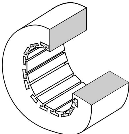
The stator laminations are thin insulated rings with slots punched from sheets of electrical grade steel. A stack of these is secured by end screws, which may also hold the end housings.
