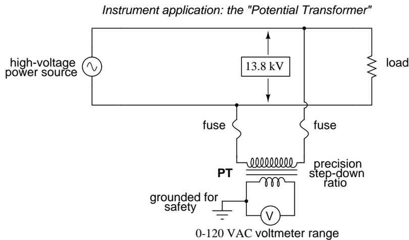
Now the voltmeter reads a precise fraction, or ratio, of the actual system voltage, its scale set to read as though it were measuring the voltage directly. The transformer keeps the instrument voltage at a safe level and electrically isolates it from the power system, so there is no direct connection between the power lines and the instrument or instrument wiring. When used in this capacity, the transformer is called a *Potential Transformer*, or simply *PT*.
