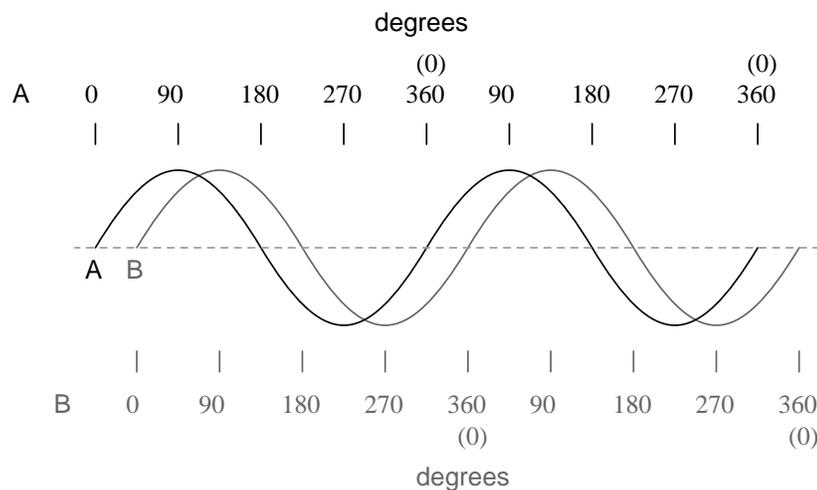
The shift between these two waveforms is about 45 degrees, the "A" wave being ahead of the "B" wave. A sampling of different phase shifts is given in the following graphs to better illustrate this concept:
