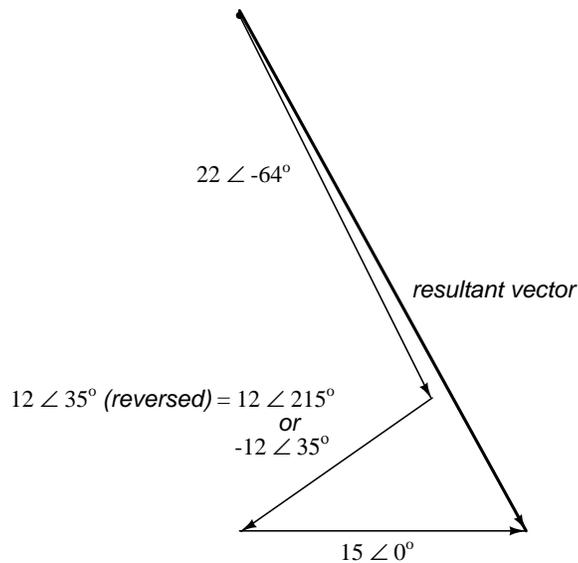
The connection reversal on the 12 volt supply can be represented in two different ways in polar form: by an addition of  $180^\circ$  to its vector angle (making it 12 volts  $\angle 215^\circ$ ), or a reversal of sign on the magnitude (making it -12 volts  $\angle 35^\circ$ ). Either way, conversion to rectangular form yields the same result:
