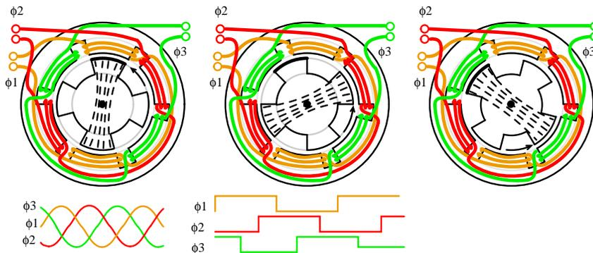
While the variable reluctance motor is simple, even more so than an induction motor, it is difficult to control. Electronic control solves this problem and makes it practical to drive the motor well above and below the power line frequency. A variable reluctance motor driven by a *servo*, an electronic feedback system, controls torque and speed, minimizing ripple torque.
