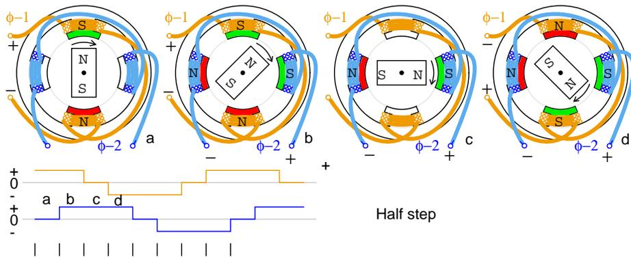
Half step drive is a combination of wave drive and full step drive with one winding energized, followed by both windings energized, yielding twice as many steps. The unipolar waveforms for half step drive are shown above. The rotor can align with the field poles as for wave drive and between the poles as for full step drive.
