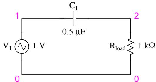
The capacitor's impedance increases with decreasing frequency. This high impedance in series tends to block low-frequency signals from getting to load.
