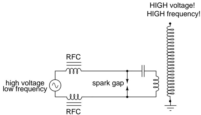
The purpose of the high-voltage, low-frequency AC power source is to "charge" the primary tank circuit. When the spark gap fires, its low impedance acts to complete the capacitor/primary coil tank circuit, allowing it to oscillate at its resonant frequency. The "RFC" inductors are "Radio Frequency Chokes," which act as high impedances to prevent the AC source from interfering with the oscillating tank circuit.
