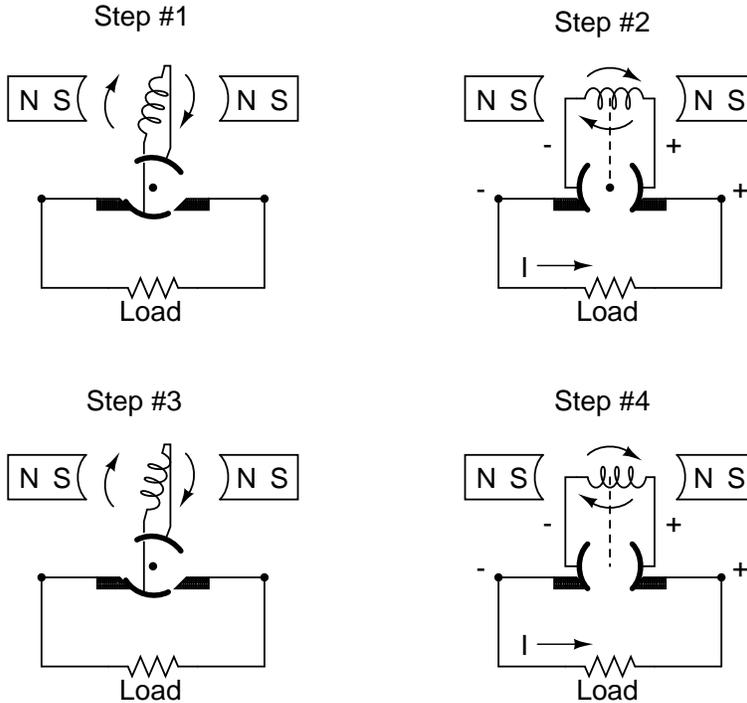
The generator shown above will produce two pulses of voltage per revolution of the shaft, both pulses in the same direction (polarity). In order for a DC generator to produce *constant* voltage, rather than brief pulses of voltage once every 1/2 revolution, there are multiple sets of coils making intermittent contact with the brushes. The diagram shown above is a bit more simplified than what you would see in real life.
