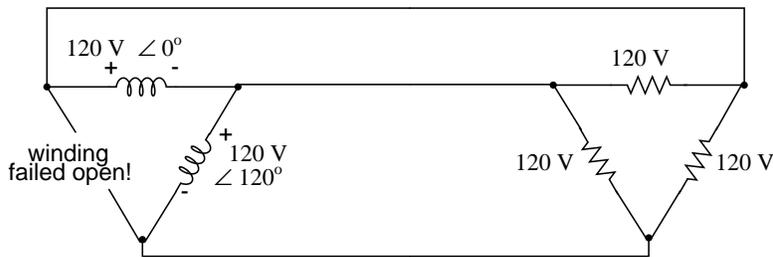
*Even with the winding failure in the source, line voltage will still be 120 V and load phase voltage will still be 120 V. The only difference will be extra current in the remaining functioning source windings.*
