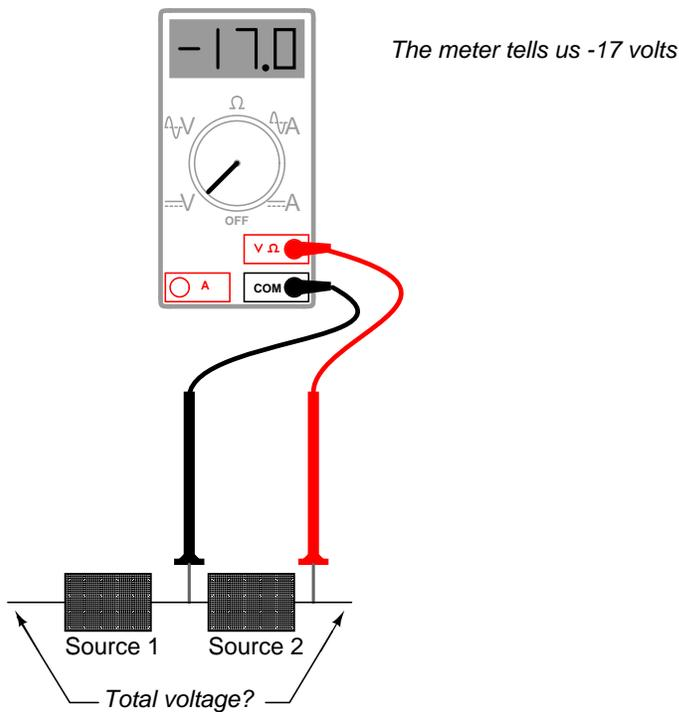
This second voltmeter reading, however, is a *negative* (-) 17 volts, which tells us that the black test lead is actually touching the positive side of voltage source #2, while the red test lead is actually touching the negative. Thus, we know that source #2 is a battery facing in the *opposite* direction:
