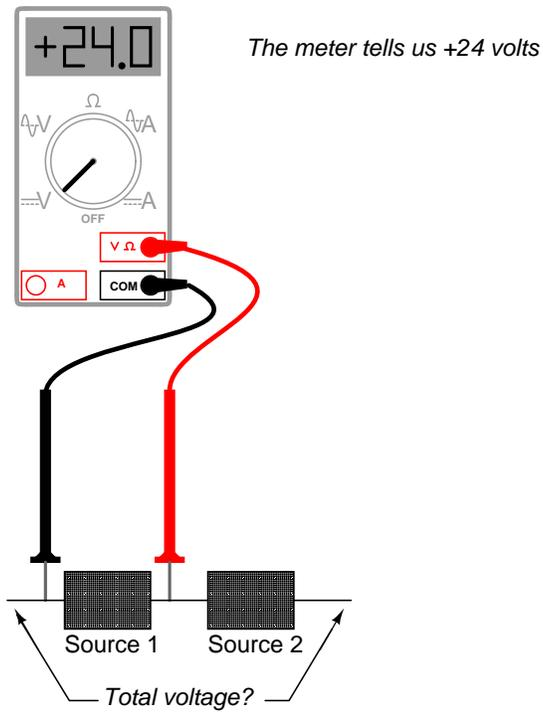
This first measurement of +24 across the left-hand voltage source tells us that the black lead of the meter really is touching the negative side of voltage source #1, and the red lead of the meter really is touching the positive. Thus, we know source #1 is a battery facing in this orientation:
