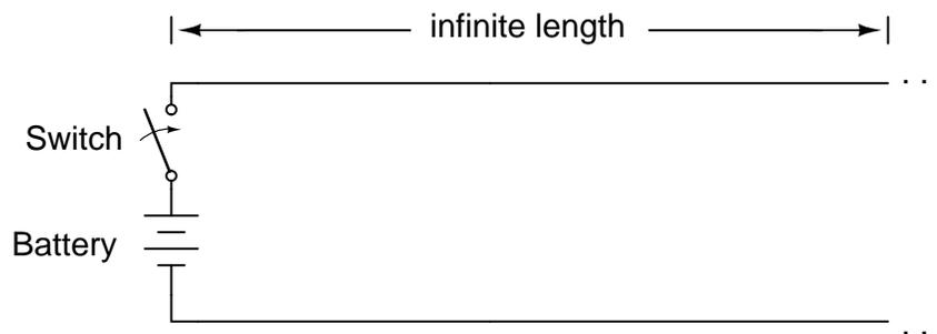
Despite being able to avoid wire resistance through the use of superconductors in this "thought experiment," we cannot eliminate capacitance along the wires' lengths. *Any* pair of conductors separated by an insulating medium creates capacitance between those conductors:
