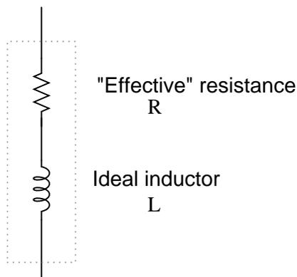
It is worthy to note that the skin effect and radiation losses apply just as well to straight lengths of wire in an AC circuit as they do a coiled wire. Usually their combined effect is too small to notice, but at radio frequencies they can be quite large. A radio transmitter antenna, for example, is designed with the express purpose of dissipating the greatest amount of energy in the form of electromagnetic radiation.
