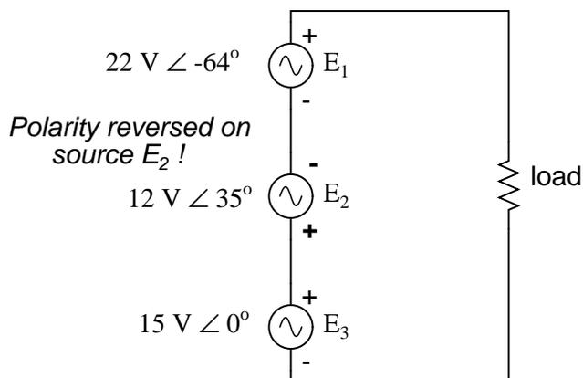
Note how the 12 volt supply's phase angle is still referred to as  $35^\circ$ , even though the leads have been reversed. Remember that the phase angle of any voltage drop is stated in reference to its noted polarity. Even though the angle is still written as  $35^\circ$ , the vector will be drawn  $180^\circ$  opposite of what it was before:
