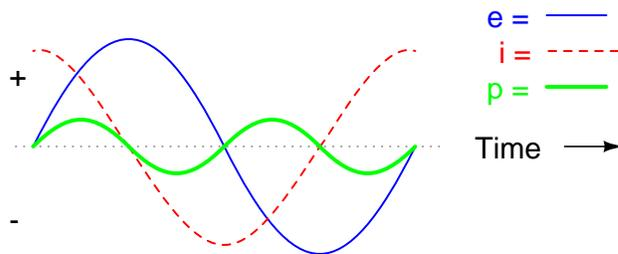
As with the simple inductor circuit, the 90 degree phase shift between voltage and current results in a power wave that alternates equally between positive and negative. This means that a capacitor does not dissipate power as it reacts against changes in voltage; it merely absorbs and releases power, alternately.
