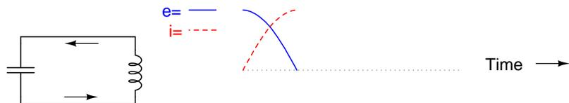
capacitor fully discharged: zero voltage
