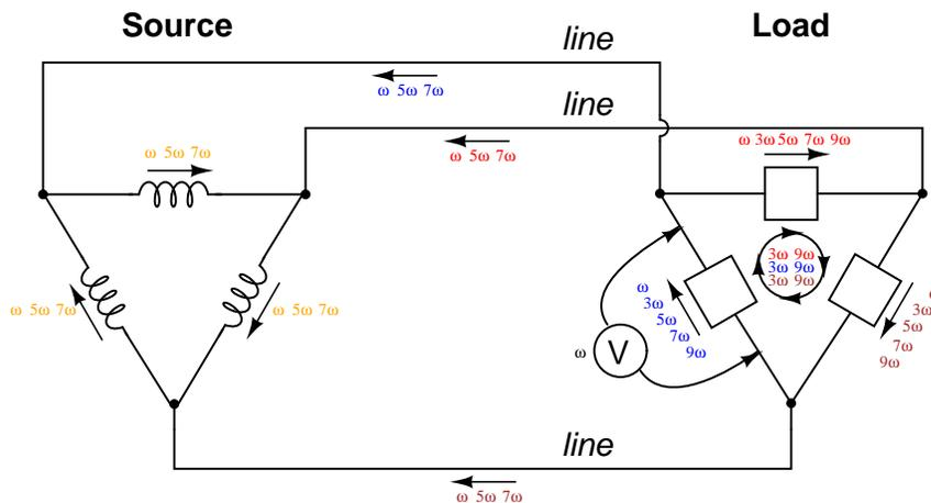
*Load phases receive undistorted sine-wave voltage.
