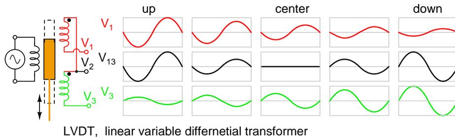
LVDT, linear variable differential transformer
