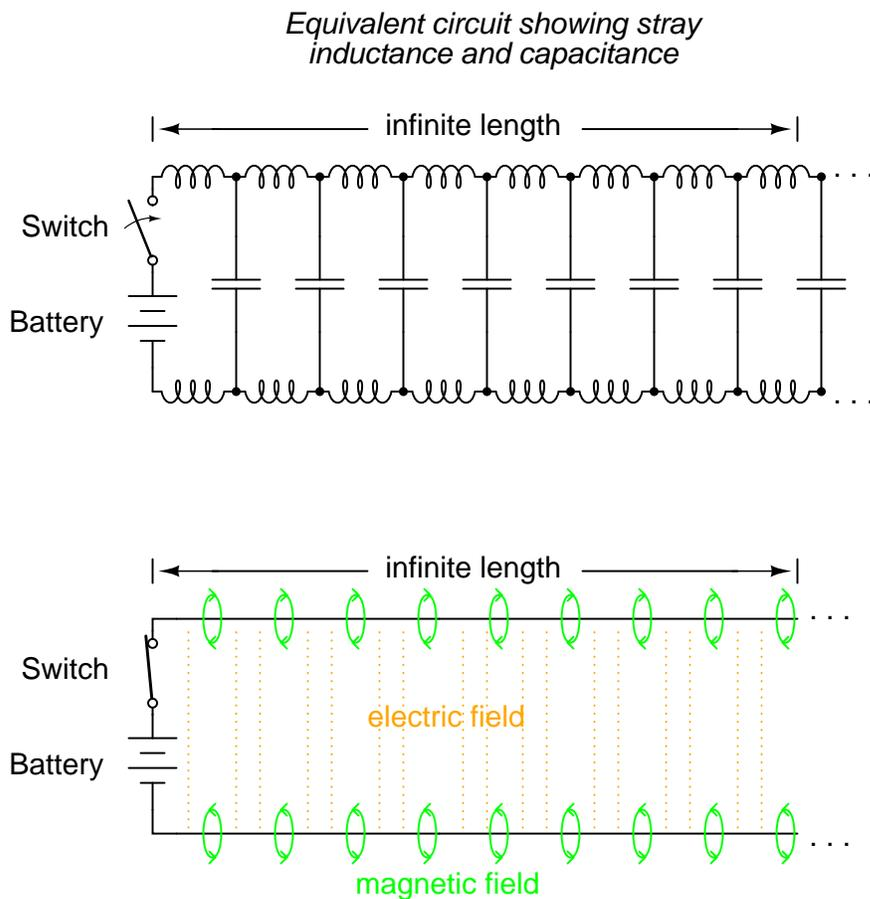
Because the electrons in the two wires transfer motion to and from each other at nearly the speed of light, the "wave front" of voltage and current change will propagate down the length of the wires at that same velocity, resulting in the distributed capacitance and inductance progressively charging to full voltage and current, respectively, like this:
