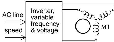
Conversely, the drive frequency may be increased to increase the synchronous speed of the motor. However, the voltage needs to be increased to overcome increasing reactance to keep current up to a normal value and maintain torque. The above inverter approximates sinewaves to the motor with pulse width modulation outputs. This is a chopped waveform which is either on or off, high or low, the percentage of "on" time corresponds to the instantaneous sine wave voltage.
