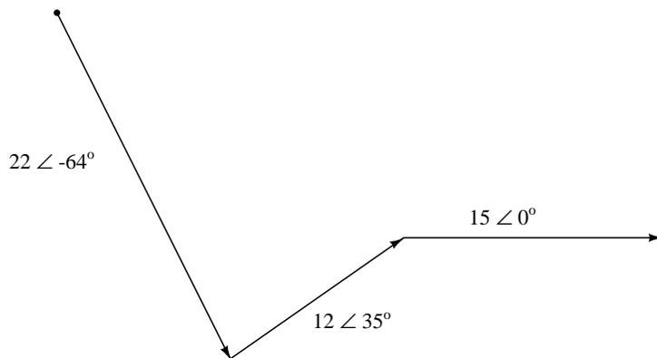
The sum of these vectors will be a resultant vector originating at the starting point for the 22 volt vector (dot at upper-left of diagram) and terminating at the ending point for the 15 volt vector (arrow tip at the middle-right of the diagram):
