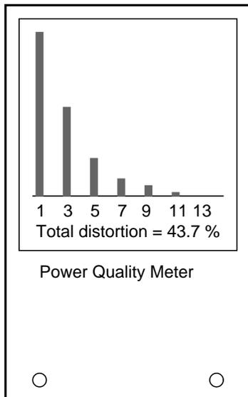
Each number on the horizontal scale of this meter represents a harmonic of the fundamental frequency. For American power systems, the "1" represents 60 Hz (the 1st harmonic, or *fundamental*), the "3" for 180 Hz (the 3rd harmonic), the "5" for 300 Hz (the 5th harmonic), and so on. The black rectangles represent the relative magnitudes of each of these harmonic components in the measured AC voltage. A pure, 60 Hz sine wave would show only a tall black bar over the "1" with no black
