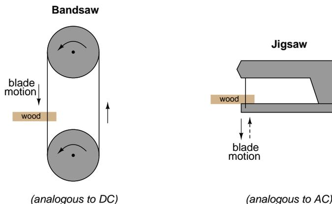
The problem of trying to describe the changing quantities of AC voltage or current in a single, aggregate measurement is also present in this saw analogy: how might we express the speed of a jigsaw blade? A bandsaw blade moves with a constant speed, similar to the way DC voltage pushes
