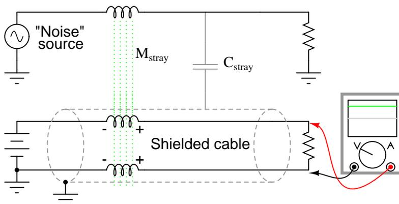
The grounded cable shield – a wire braid or metal foil wrapped around the two insulated conductors – isolates both conductors from electrostatic (capacitive) coupling by blocking any external
