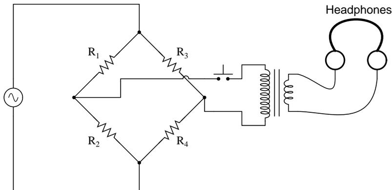
Listening to the headphones as one or more of the resistor "arms" of the bridge is adjusted, a condition of balance will be realized when the headphones fail to produce "clicks" (or tones, if the bridge's power source frequency is within audio range) as the switch is actuated.
