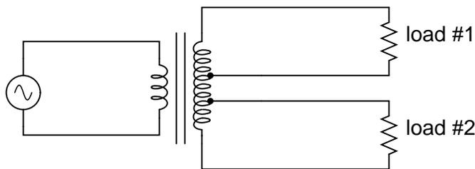
A tap is nothing more than a wire connection made at some point on a winding between the very ends. Not surprisingly, the winding turn/voltage magnitude relationship of a normal transformer holds true for all tapped segments of windings. This fact can be exploited to produce a transformer capable of multiple ratios:
