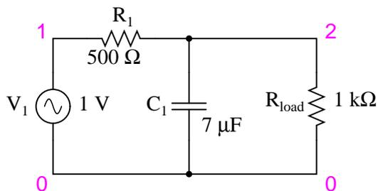
The capacitor's impedance decreases with increasing frequency. This low impedance in parallel with the load resistance tends to short out high-frequency signals, dropping most of the voltage across series resistor  $R_1$ .
