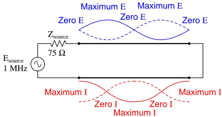
However, if the signal frequency is such that the line resonates at  $1/4$  wavelength or some multiple thereof, the source will "see" the exact opposite of the termination impedance. That is, if the line is open-circuited, the source will "see" a short-circuit at the point where it connects to the line; and if the line is short-circuited, the source will "see" an open circuit:
