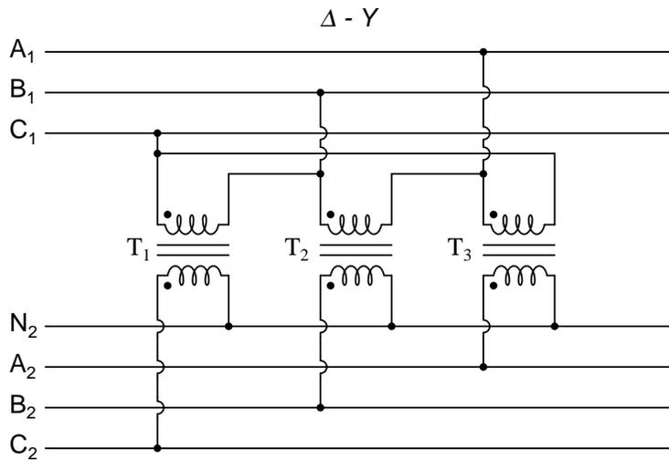
Such a configuration would allow for the provision of multiple voltages (line-to-line or line-to-neutral) in the second power system, from a source power system having no neutral.
