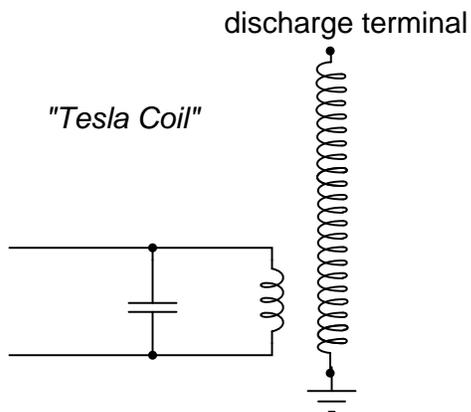
The capacitor, in conjunction with the transformer's primary winding, forms a tank circuit. The secondary winding is wound in close proximity to the primary, usually around the same nonmagnetic form. Several options exist for "exciting" the primary circuit, the simplest being a high-voltage, low-frequency AC source and spark gap:
