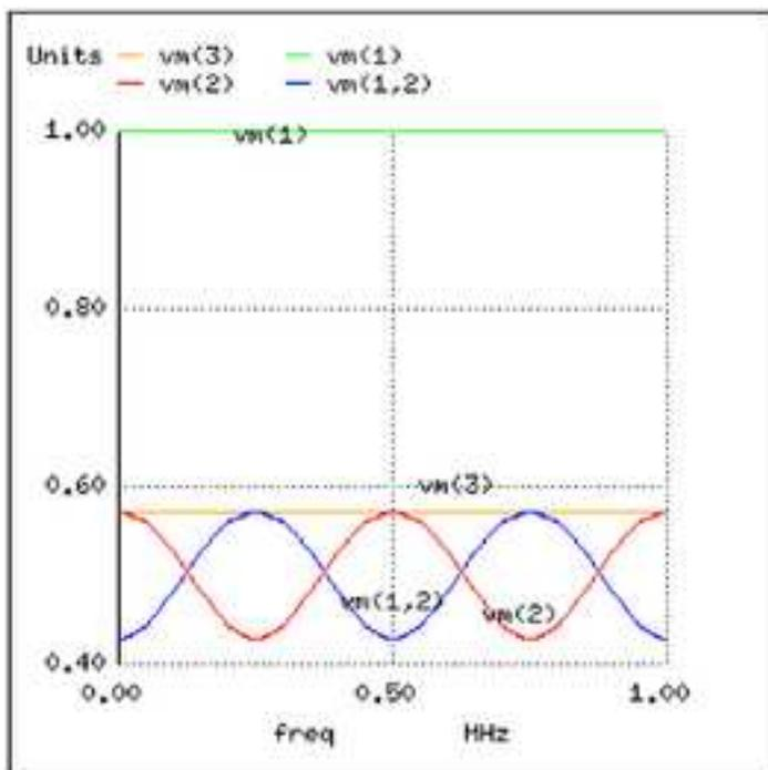
If we run another SPICE analysis, this time printing numerical results rather than plotting them, we can discover exactly what is happening at all the interesting frequencies (DC, 250 kHz, 500 kHz, 750 kHz, and 1 MHz):
