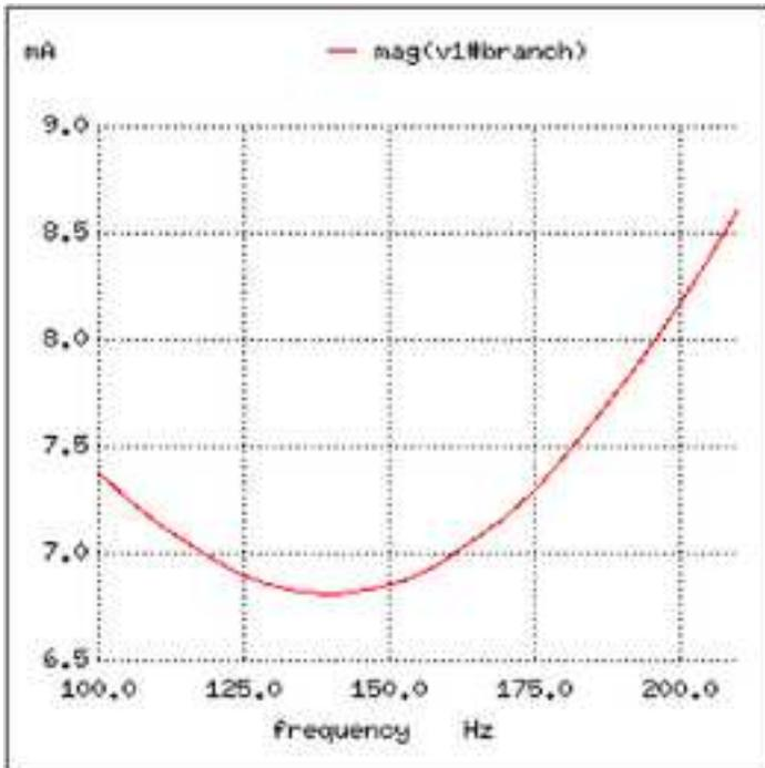
Minimum current at 136.8 Hz instead of 159.2 Hz!
