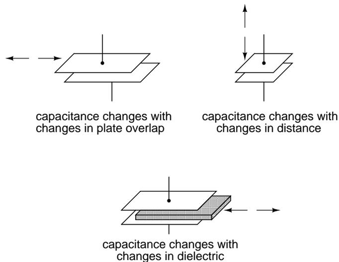
Transducers with greater sensitivity and immunity to changes in other variables can be obtained by way of differential design, much like the concept behind the LVDT (Linear Variable *Differential* Transformer). Here are a few examples of differential capacitive transducers:
