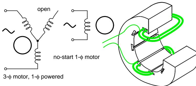
The single coil of a single phase induction motor does not produce a rotating magnetic field, but a pulsating field reaching maximum intensity at  $0^\circ$  and  $180^\circ$  electrically.
