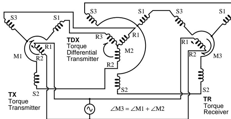
A shipboard radar antenna coupled to a synchro transmitter encodes the antenna angle with respect to ship's bow. It is desired to display the antenna position with respect to true north. We need to add the ships heading from a gyrocompass to the bow-relative antenna position to display antenna angle with respect to true north.  $\angle_{\text{antenna}} + \angle_{\text{gyro}}$
