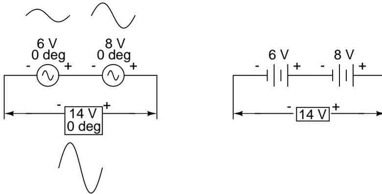
Please note the (+) and (-) polarity marks next to the leads of the two AC sources. Even though we know AC doesn't have "polarity" in the same sense that DC does, these marks are essential to knowing how to reference the given phase angles of the voltages. This will become more apparent in the next example.
