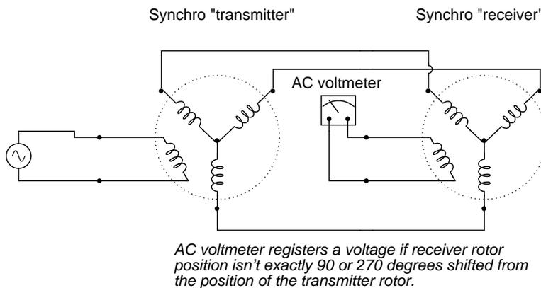
This can be thought of almost as a sort of bridge circuit that achieves balance only if the receiver shaft is brought to one of two (matching) positions with the transmitter shaft.
