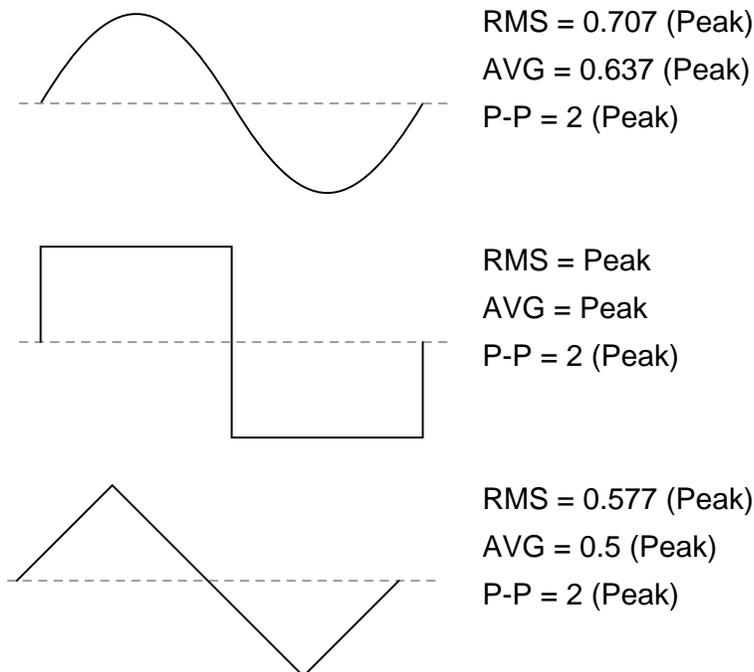
In addition to RMS, average, peak (crest), and peak-to-peak measures of an AC waveform, there
