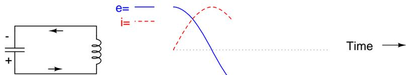
capacitor charging: voltage increasing (in opposite polarity)
