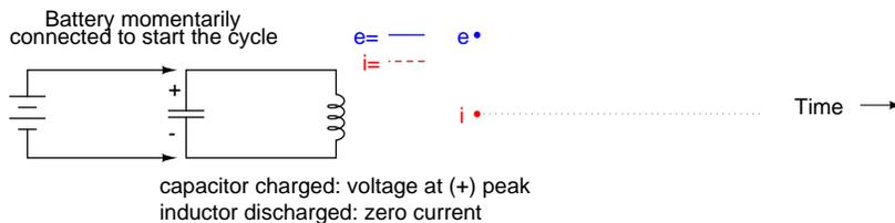
The capacitor will begin to discharge, its voltage decreasing. Meanwhile, the inductor will begin to build up a "charge" in the form of a magnetic field as current increases in the circuit:
