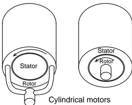
The most usual construction, cylindrical, can take on two forms, above. The most common cylindrical style is with the rotor on the inside, above right. This style motor is used in hard disk drives. It is also possible to put the rotor on the outside surrounding the stator. Such is the case with brushless DC fan motors, sans the shaft. This style of construction may be short and fat. However, the direction of the magnetic flux is radial with respect to the rotational axis.
