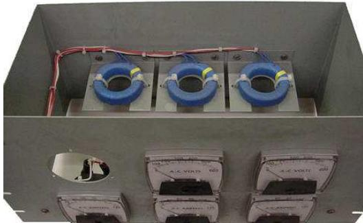
Because of the expense (and often large size) of instrument transformers, they are not used to scale AC meters for any applications other than high voltage and high current. For scaling a milliamp or microamp movement to a range of 120 volts or 5 amps, normal precision resistors (multipliers and shunts) are used, just as with DC.
