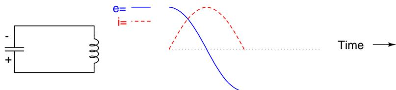
capacitor fully charged: voltage at (-) peak
