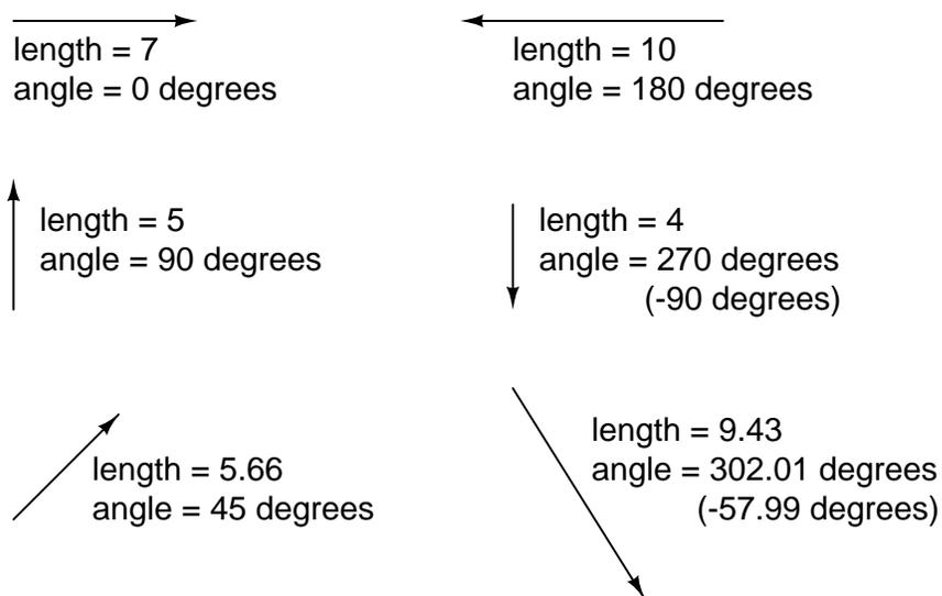
Like distances and directions on a map, there must be some common frame of reference for angle figures to have any meaning. In this case, directly right is considered to be  $0^\circ$ , and angles are counted in a positive direction going counter-clockwise:
