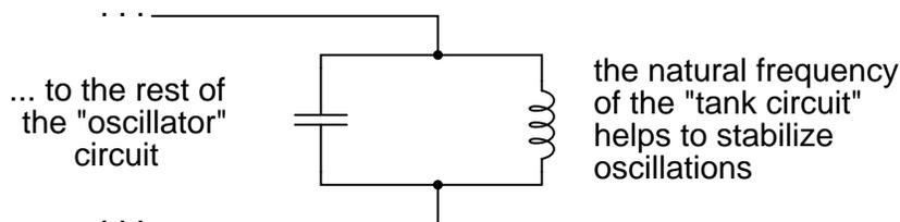
Another use for resonance is in applications where the effects of greatly increased or decreased impedance at a particular frequency is desired. A resonant circuit can be used to "block" (present high impedance toward) a frequency or range of frequencies, thus acting as a sort of frequency "filter" to strain certain frequencies out of a mix of others. In fact, these particular circuits are called *filters*, and their design constitutes a discipline of study all by itself:
