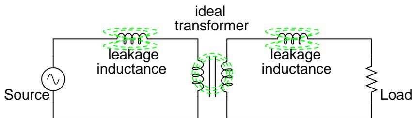
If we change the transformer design to have better magnetic coupling between the primary and secondary coils, the figures for voltage between primary and secondary windings will be much closer to equality again:
