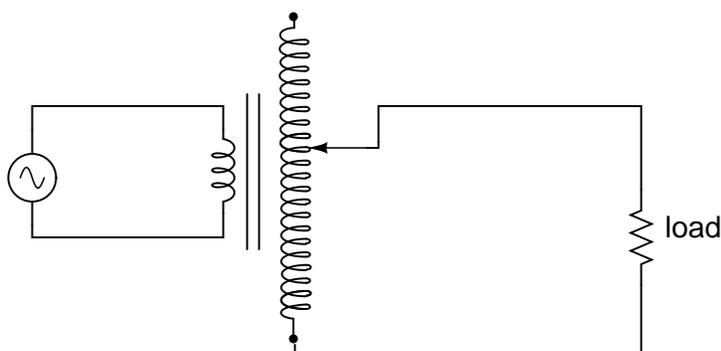
One consumer application of the variable transformer is in speed controls for model train sets, especially the train sets of the 1950's and 1960's. These transformers were essentially step-down units, the highest voltage obtainable from the secondary winding being substantially less than the primary voltage of 110 to 120 volts AC. The variable-sweep contact provided a simple means of voltage control with little wasted power, much more efficient than control using a variable resistor!
