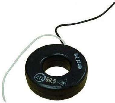
Some CTs are made to hinge open, allowing insertion around a power conductor without disturbing the conductor at all. The industry standard secondary current for a CT is a range of 0 to 5 amps AC. Like PTs, CTs can be made with custom winding ratios to fit almost any application. Because their "full load" secondary current is 5 amps, CT ratios are usually described in terms of full-load primary amps to 5 amps, like this:
