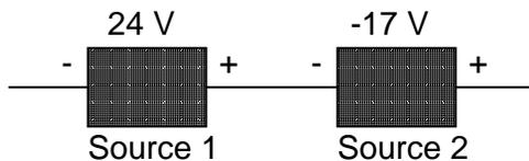
According to this diagram, the polarity marks (which indicate meter test lead placement) indicate
