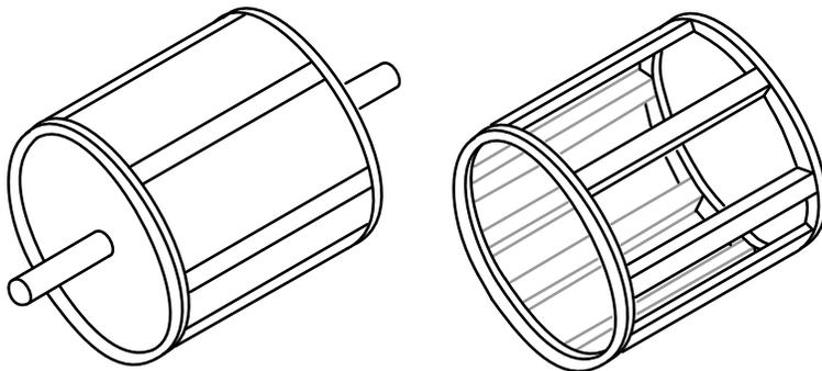
The squirrel cage conductors may be skewed, twisted, with respect to the shaft. The misalignment with the stator slots reduces torque pulsations.
