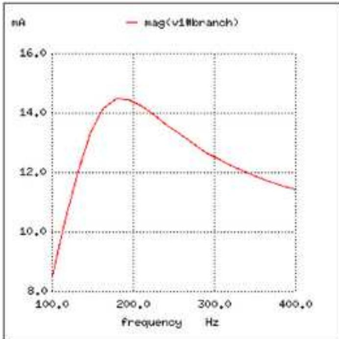
And finally, a series LC circuit with the significant resistance in parallel with the capacitor:
