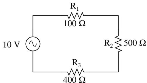
$$R_{\text{total}} = R_1 + R_2 + R_3$$
