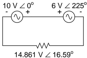
$6\text{ V} \angle 45^\circ$  with negative on the left and positive on the right is exactly the same as  $6\text{ V} \angle 225^\circ$  with positive on the left and negative on the right: the reversal of polarity markings perfectly complements the addition of  $180^\circ$  to the phase angle designation:
