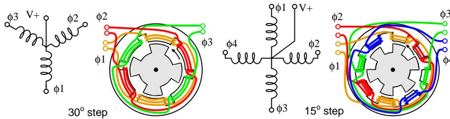
The required stepper drive waveforms for the 3- $\phi$  stepper, above left, can be seen in the "Reluctance motor" section. The drive for a 4- $\phi$  stepper are shown below. Sequentially switching the stator phases produces a rotating magnetic field which the rotor follows. However, due to the lesser number of rotor poles, the rotor moves less than the stator angle for each step. For a variable reluctance stepper motor, the step angle is given by:
