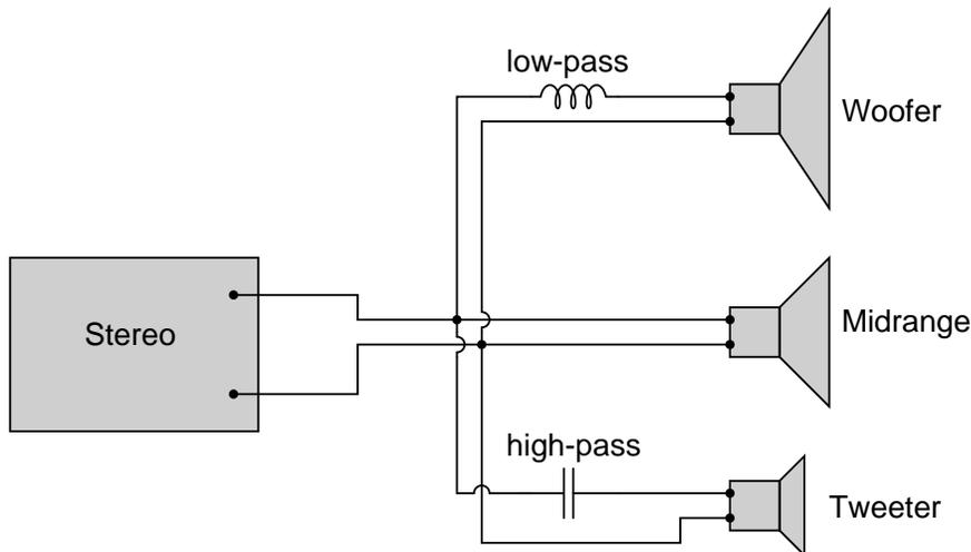
For better performance yet, we might like to have some kind of filter circuit capable of passing frequencies that are between low (bass) and high (treble) to the midrange speaker so that none of the low- or high-frequency signal power is wasted on a speaker incapable of efficiently reproducing those sounds. What we would be looking for is called a *band-pass* filter, which is the topic of the next section.
