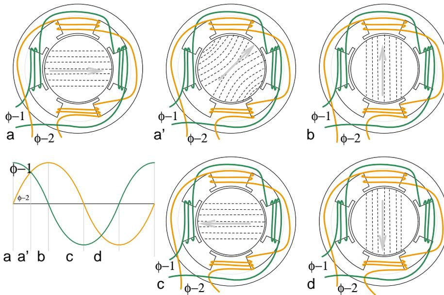
As the  $90^\circ$  phased sinewaves, above left, progress from points (a) through (d), the magnetic field rotates counterclockwise (figures a-d) as follows:
