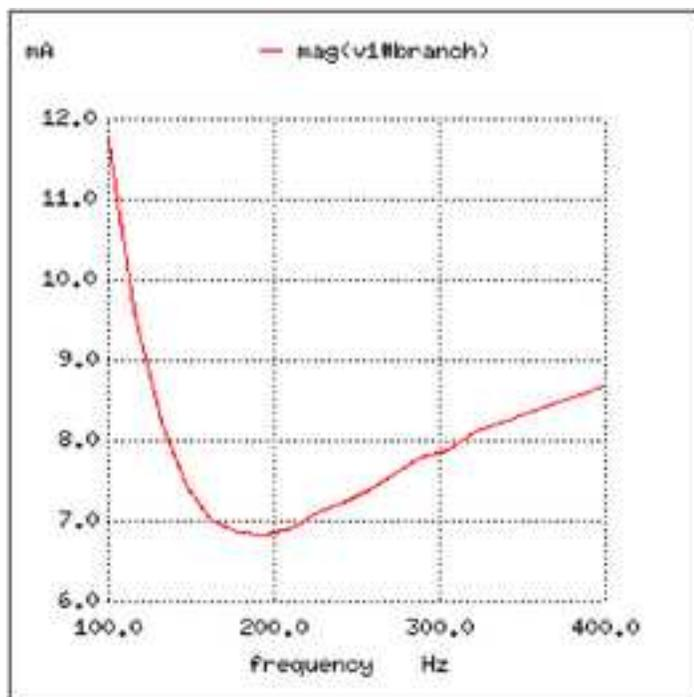
Switching our attention to series LC circuits, we experiment with placing significant resistances in parallel with either L or C. In the following series circuit examples, a  $1\ \Omega$  resistor ( $R_1$ ) is placed in series with the inductor and capacitor to limit total current at resonance. The "extra" resistance inserted to influence resonant frequency effects is the  $100\ \Omega$  resistor,  $R_2$ :
