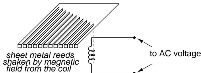
The user of this meter views the ends of all those unequal length reeds as they are collectively shaken at the frequency of the applied AC voltage to the coil. The one closest in resonant frequency to the applied AC will vibrate the most, looking something like this:
