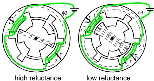
Sequential switching of the stator phases moves the rotor from one position to the next. The magnetic flux seeks the path of least reluctance, the magnetic analog of electric resistance.
