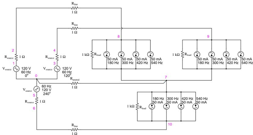
Y-Y source/load 4-wire system with harmonics
