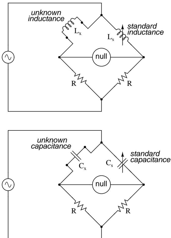
Simple "symmetrical" bridges such as these are so named because they exhibit symmetry (mirror-image similarity) from left to right. The two bridge circuits shown above are balanced by adjusting the calibrated reactive component ( $L_s$  or  $C_s$ ). They are a bit simplified from their real-life counterparts, as practical symmetrical bridge circuits often have a calibrated, variable resistor in series
