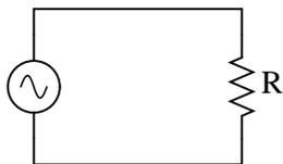
If we were to plot the current and voltage for a very simple AC circuit consisting of a source and a resistor, it would look something like this:
