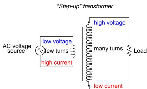
The transformer's ability to step AC voltage up or down with ease gives AC an advantage unmatched by DC in the realm of power distribution. When transmitting electrical power over long distances, it is far more efficient to do so with stepped-up voltages and stepped-down currents (smaller-diameter wire with less resistive power losses), then step the voltage back down and the current back up for industry, business, or consumer use.
