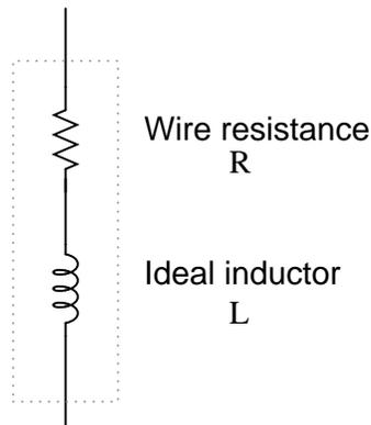
Consequently, the impedance of any real inductor will always be a complex combination of resistance and inductive reactance.
