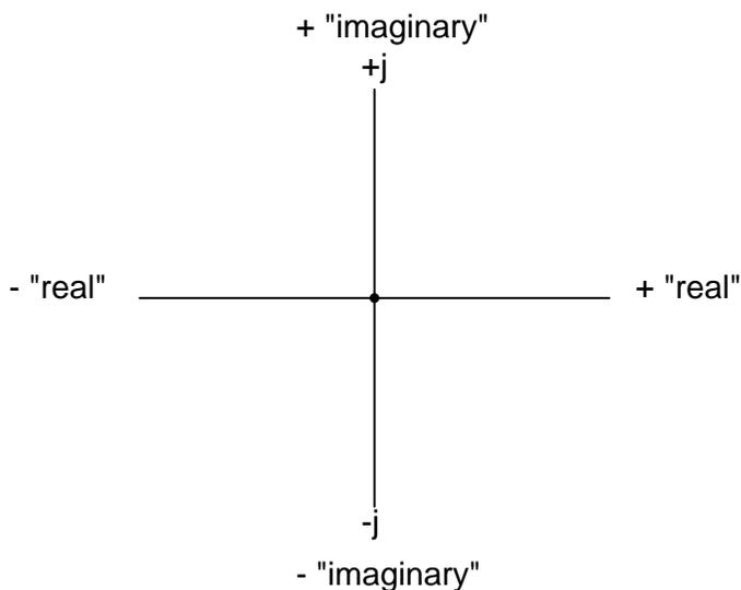
The horizontal component is referred to as the *real* component, since that dimension is compatible with normal, scalar ("real") numbers. The vertical component is referred to as the *imaginary* component, since that dimension lies in a different direction, totally alien to the scale of the real
