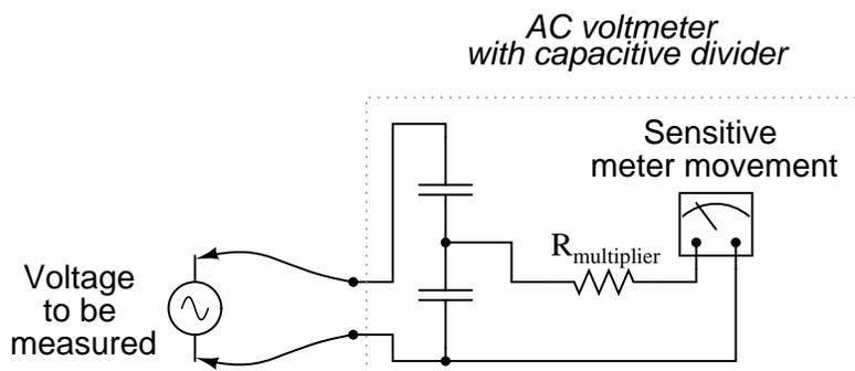
If the meter movement is electrostatic, and thus inherently capacitive in nature, a single "multiplier" capacitor may be connected in series to give it a greater voltage measuring range, just as a series-connected multiplier resistor gives a moving-coil (inherently resistive) meter movement a greater voltage range:
