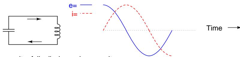
capacitor fully discharged: zero voltage
