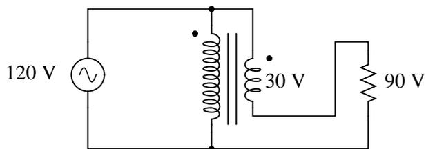
The prime advantage of an autotransformer is that the same boosting or bucking function is obtained with only a single winding, making it cheaper and lighter to manufacture than a regular
