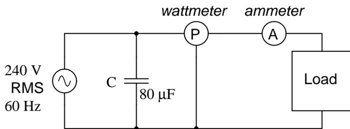
An 80  $\mu\text{F}$  capacitor will have a capacitive reactance of 33.157  $\Omega$ , giving a current of 7.238 amps, and a corresponding reactive power of 1.737 kVAR (for the capacitor *only*). Since the capacitor's current is 180° out of phase from the the load's inductive contribution to current draw, the capacitor's reactive power will directly subtract from the load's reactive power, resulting in:
