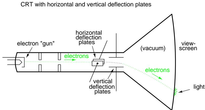
If we allow one AC signal to deflect the beam up and down (connect that AC voltage source to the "vertical" deflection plates) and another AC signal to deflect the beam left and right (using the other pair of deflection plates), patterns will be produced on the screen of the CRT indicative of the *ratio* of these two AC frequencies. These patterns are called *Lissajous figures* and are a common means of comparative frequency measurement in electronics.
