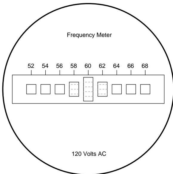
Vibrating reed meters, obviously, are not precision instruments, but they are very simple and therefore easy to manufacture to be rugged. They are often found on small engine-driven generator sets for the purpose of setting engine speed so that the frequency is somewhat close to 60 (50 in Europe) Hertz.
