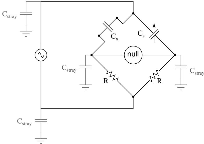
The problem is worsened if the AC voltage source is firmly grounded at one end, the total stray impedance for leakage currents made far less and any leakage currents through these stray capacitances made greater as a result:
