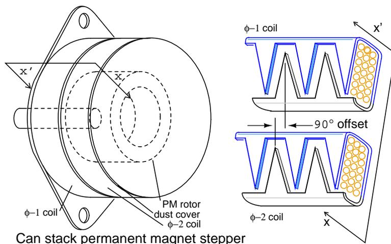
Above is the external package of a can-stack permanent magnet stepper motor.
