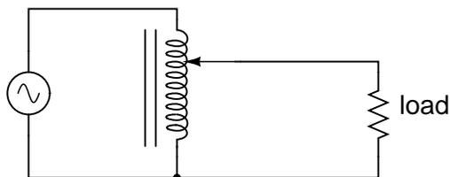
Small variacs for benchtop use are popular pieces of equipment for the electronics experimenter, being able to step household AC voltage down (or sometimes up as well) with a wide, fine range of control by a simple twist of a knob.
