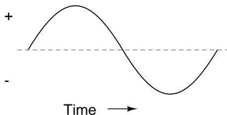
In the voltage plot from an electromechanical alternator, the change from one polarity to the other is a smooth one, the voltage level changing most rapidly at the zero ("crossover") point and most slowly at its peak. If we were to graph the trigonometric function of "sine" over a horizontal range of 0 to 360 degrees, we would find the exact same pattern:
