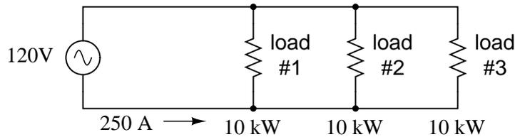
This would necessitate 3/0 gage copper wire (*very* large!), at about 510 pounds per thousand feet, and with a considerable price tag attached. If the distance from source to load was 1000 feet, we would need over a half-ton of copper wire to do the job. On the other hand, we could build a split-phase system with two 15 kW, 120 volt loads:
