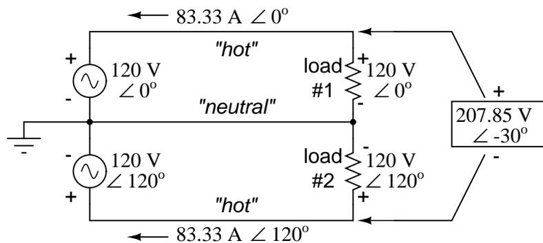
Since each voltage source is 120 volts, and each load resistor is connected directly in parallel with its respective source, the voltage across each load *must* be 120 volts as well. Given load currents of 83.33 amps, each load must still be dissipating 10 kilowatts of power. However, voltage between the two "hot" wires is not 240 volts ( $120 \angle 0^\circ - 120 \angle 180^\circ$ ) because the phase difference between the two sources is not  $180^\circ$ . Instead, the voltage is:
