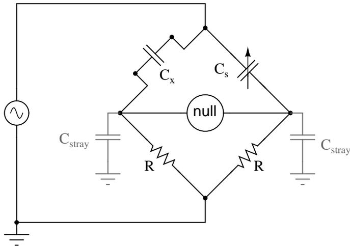
One way of greatly reducing this effect is to keep the null detector at ground potential, so there will be no AC voltage between it and the ground, and thus no current through stray capacitances. However, directly connecting the null detector to ground is not an option, as it would create a *direct* current path for stray currents, which would be worse than any capacitive path. Instead, a special
