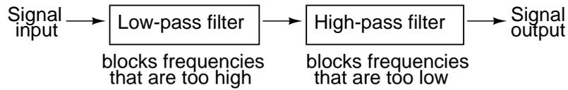
What emerges from the series combination of these two filter circuits is a circuit that will only allow passage of those frequencies that are neither too high nor too low. Using real components, here is what a typical schematic might look like:
