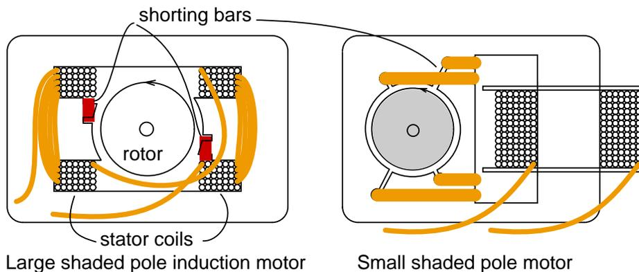
Starting torque is so low that shaded pole motors are only manufactured in smaller sizes, below 50 watts. Low cost and simplicity suit this motor to small fans, air circulators, and other low torque applications. Motor speed can be lowered by switching reactance in series to limit current and torque, or by switching motor coil taps as below
