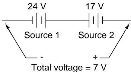
It should be obvious to any experienced student of DC electricity that these two batteries are opposing one another. By definition, opposing voltages *subtract* from one another, so we subtract 17 volts from 24 volts to obtain the total voltage across the two: 7 volts.
