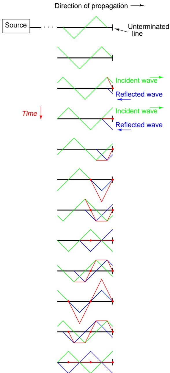
This third, "standing" wave, in fact, represents the only voltage along the line, being the representative sum of incident and reflected voltage waves. It oscillates in instantaneous magnitude, but does not propagate down the cable's length like the incident or reflected waveforms causing it. Note the dots along the line length marking the "zero" points of the standing wave (where the incident
