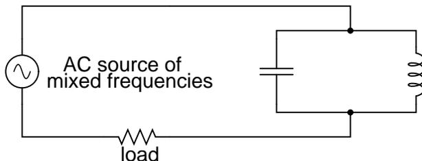
Tank circuit presents a high impedance to a narrow range of frequencies, blocking them from getting to the load
