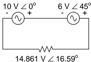
The polarity markings show these two voltage sources aiding each other, so to determine the total voltage across the resistor we must *add* the voltage figures of  $10\text{ V} \angle 0^\circ$  and  $6\text{ V} \angle 45^\circ$  together to obtain  $14.861\text{ V} \angle 16.59^\circ$ . However, it would be perfectly acceptable to represent the 6 volt source as  $6\text{ V} \angle 225^\circ$ , with a reversed set of polarity markings, and still arrive at the same total voltage:
