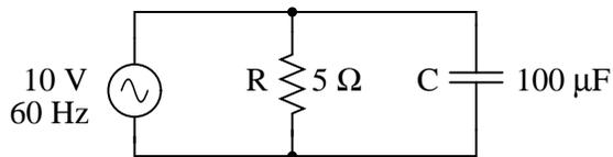
Because the power source has the same frequency as the series example circuit, and the resistor and capacitor both have the same values of resistance and capacitance, respectively, they must also have the same values of impedance. So, we can begin our analysis table with the same "given" values:
