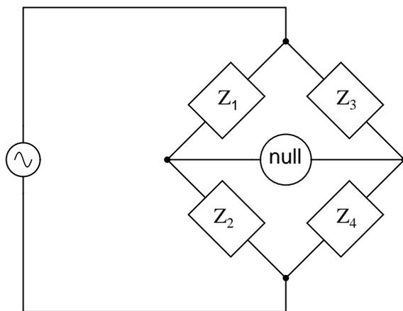
*A box with a "Z" written inside is the symbol for any nonspecific impedance.*
