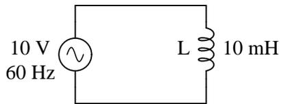
(inductive reactance of 10 mH inductor at 60 Hz)
