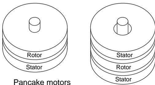
High torque pancake motors may have stator coils on both sides of the rotor as above right. Lower torque applications like floppy disk drive motors suffice with a stator coils on one side of the rotor, above left. The direction of the magnetic flux is axial, that is, parallel to the axis of rotation.
