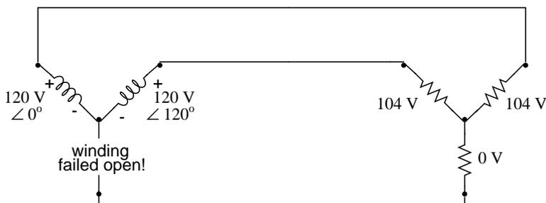
In this case, two load resistances suffer reduced voltage while the third loses supply voltage completely! For this reason,  $\Delta$ -connected sources are preferred for reliability. However, if dual voltages are needed (e.g. 120/208) or preferred for lower line currents, Y-connected systems are the configuration of choice.
