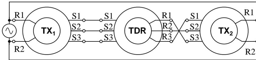
TDR addition:  $\angle TDR = \angle TX_1 + \angle TX_2$
