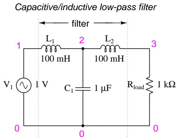
The inductors should block any high frequencies, while the capacitor should short out any high frequencies as well, both working together to allow only low frequency signals to reach the load.
