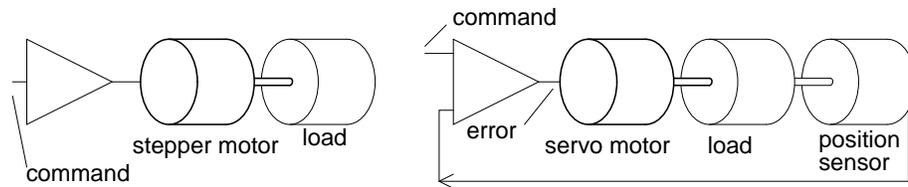
Stepper motor vs servo motor
