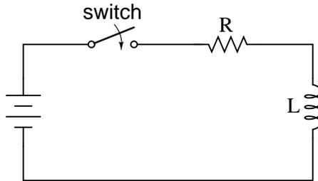
The idea of this circuit is simple: to "charge" the inductor when the switch is closed. The rate of inductor charging will be set by the ratio  $L/R$ , which is the time constant of the circuit in seconds. However, if you were to build such a circuit, you might find unexpected oscillations (AC) of voltage across the inductor when the switch is closed. Why is this? There's no capacitor in the circuit, so how can we have resonant oscillation with just an inductor, resistor, and battery?
