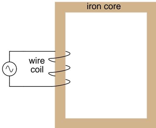
As an inductor, we would expect this iron-core coil to oppose the applied voltage with its inductive reactance, limiting current through the coil as predicted by the equations  $X_L = 2\pi fL$  and  $I = E/X$  (or  $I = E/Z$ ). For the purposes of this example, though, we need to take a more detailed look at the interactions of voltage, current, and magnetic flux in the device.
