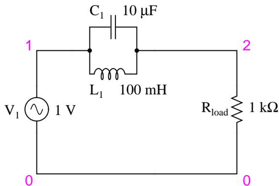
The parallel LC components present a high impedance at resonant frequency, thereby blocking the signal from the load at that frequency. Conversely, it passes signals to the load at any other frequencies.
