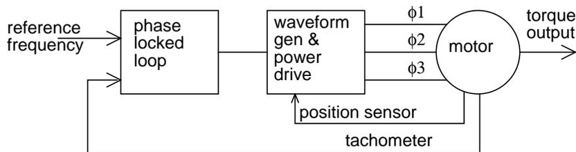
A motor driven by square waves of current, as provided by simple hall effect sensors, is known as a *brushless DC motor*. This type of motor has higher *ripple torque* torque variation through a shaft revolution than a sine wave driven motor. This is not a problem for many applications. Though we are primarily interested in synchronous motors in this section.
