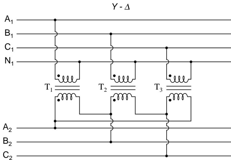
Note how the secondary windings (bottom set) are connected in a chain, the "dot" side of one winding connected to the "non-dot" side of the next, forming the  $\Delta$  loop. At every connection point between pairs of windings, a connection is made to a line of the second power system (A, B, and C).
