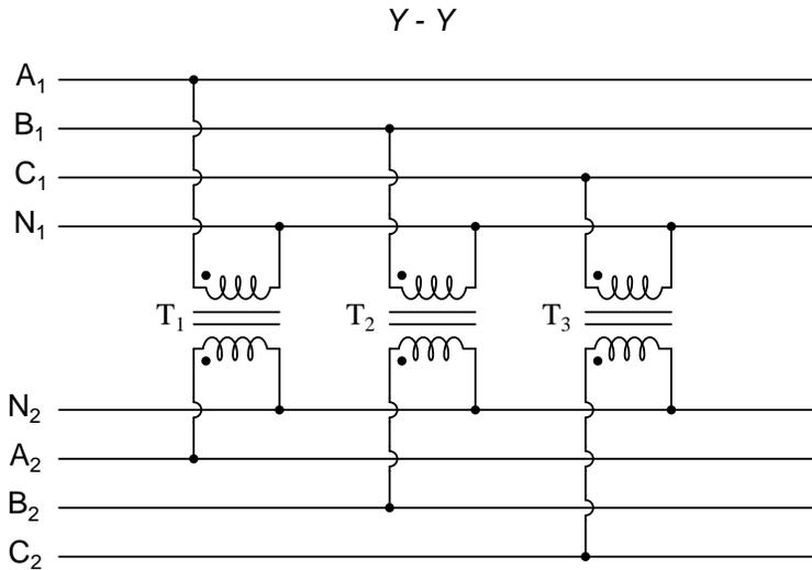
Note how all the winding ends marked with dots are connected to their respective phases A, B, and C, while the non-dot ends are connected together to form the centers of each "Y". Having both primary and secondary winding sets connected in "Y" formations allows for the use of neutral conductors ( $N_1$  and  $N_2$ ) in each power system.
