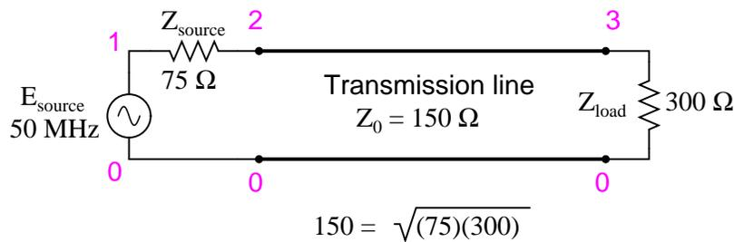
We can specify the cable length in SPICE in terms of time delay from beginning to end. Since the frequency is  $50 \text{ MHz}$ , the signal period will be the reciprocal of that, or  $20$  nano-seconds ( $20 \text{ ns}$ ). One-quarter of that time ( $5 \text{ ns}$ ) will be the time delay of a transmission line one-quarter wavelength long:
