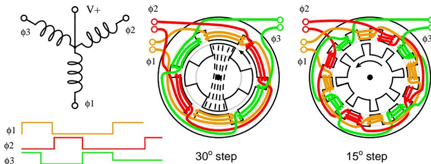
One end of each 3-phase winding of a switched reluctance motor is usually brought out via a common power supply wire, above left. The other coil connections are successively pulled to
