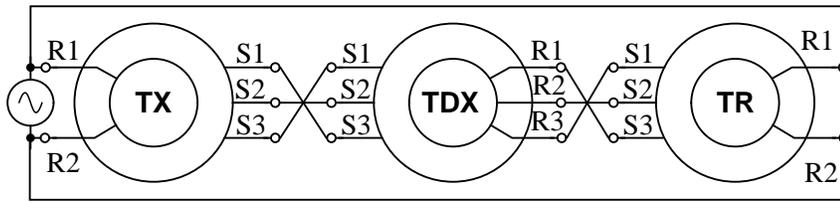
TDX addition:  $\angle TX + \angle TDX = \angle TR$
