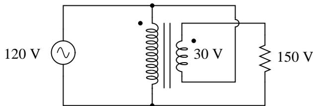
Next, the "bucking" configuration. Here, the secondary coil's polarity is oriented so that its voltage directly subtracts from the primary voltage:
