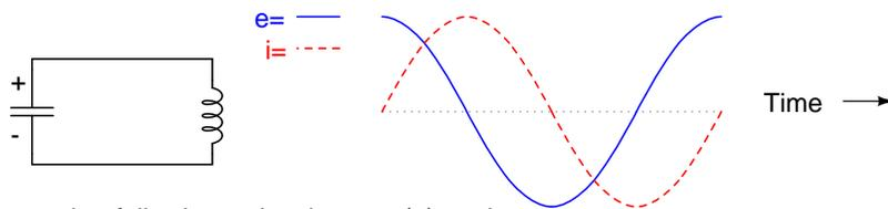
capacitor fully charged: voltage at (+) peak
