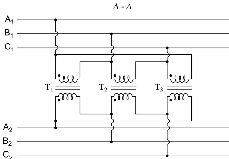
When there is no need for a neutral conductor in the secondary power system,  $\Delta - \Delta$  connection schemes are preferred because of the inherent reliability of the  $\Delta$  configuration.
