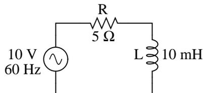
The resistor will offer  $5 \Omega$  of resistance to AC current regardless of frequency, while the inductor will offer  $3.7699 \Omega$  of reactance to AC current at 60 Hz. Because the resistor's resistance is a real
