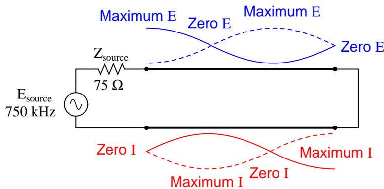
At these frequencies, the transmission line is actually functioning as an *impedance transformer*, transforming an infinite impedance into zero impedance, or vice versa. Of course, this only occurs at resonant points resulting in a standing wave of  $1/4$  cycle (the line's fundamental, resonant frequency) or some odd multiple ( $3/4, 5/4, 7/4, 9/4 \dots$ ), but if the signal frequency is known and unchanging, this phenomenon may be used to match otherwise unmatched impedances to each other.
