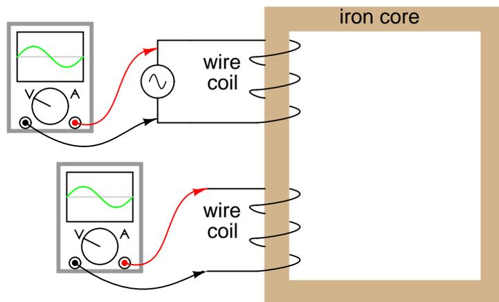
If this secondary coil experiences the same magnetic flux change as the primary (which it should, assuming perfect containment of the magnetic flux through the common core), and has the same number of turns around the core, a voltage of equal magnitude and phase to the applied voltage will be induced along its length. In the following graph, the induced voltage waveform is drawn slightly smaller than the source voltage waveform simply to distinguish one from the other:
