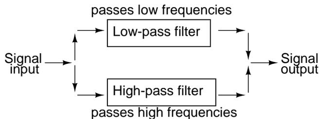
Constructed using two capacitive filter sections, it looks something like this:
