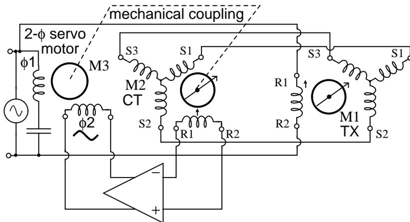
When the control transformer rotor detects a null at  $90^\circ$  to the axis of the stator field, there is no rotor output. Any rotor displacement would produce an AC error voltage proportional to displacement. A *servo* seeks to minimize the error between a commanded and measured variable due
