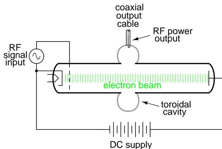
Just as transmission lines are able to function as resonant elements in a circuit, especially when terminated by a short-circuit or an open-circuit, a dead-ended waveguide may also resonate at particular frequencies. When used as such, the device is called a *cavity resonator*. Inductive output tubes use toroid-shaped cavity resonators to maximize the power transfer efficiency between the electron beam and the output cable.
