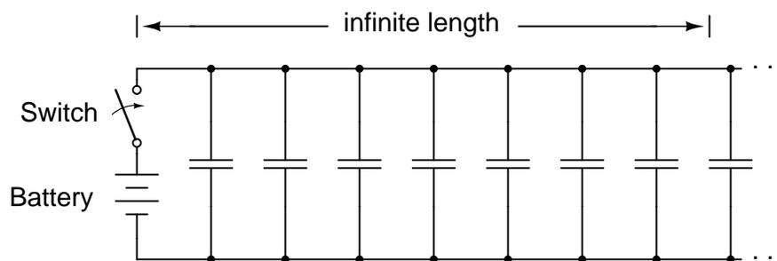
Voltage applied between two conductors creates an electric field between those conductors. Energy is stored in this electric field, and this storage of energy results in an opposition to change in voltage. The reaction of a capacitance against changes in voltage is described by the equation  $i = C(de/dt)$ , which tells us that current will be drawn proportional to the voltage's rate of change over time. Thus, when the switch is closed, the capacitance between conductors will react against
