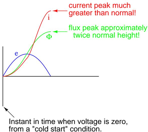
This is the mechanism causing inrush current in a transformer's primary winding when connected to an AC voltage source. As you can see, the magnitude of the inrush current strongly depends on the exact time that electrical connection to the source is made. If the transformer happens to have some residual magnetism in its core at the moment of connection to the source, the inrush could
