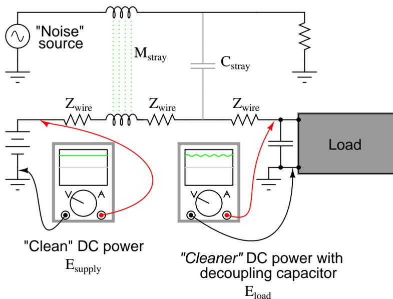
A cursory glance at a crowded printed-circuit board (PCB) will typically reveal decoupling capacitors scattered throughout, usually located as close as possible to the sensitive DC loads. Capacitor size is usually  $0.1 \mu\text{F}$  or more, a minimum amount of capacitance needed to produce a low enough impedance to short out any noise. Greater capacitance will do a better job at filtering noise, but size and economics limit decoupling capacitors to meager values.
