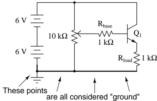
For example, if I were to speak of voltage *at* the base of the transistor ( $V_B$ ), I would mean the voltage measured between the transistor's base terminal and the negative side of the power supply (ground), with the red probe touching the base terminal and the black probe touching ground. Normally, it is nonsense to speak of voltage *at* a single point, but having an implicit reference point for voltage measurements makes such statements meaningful:
