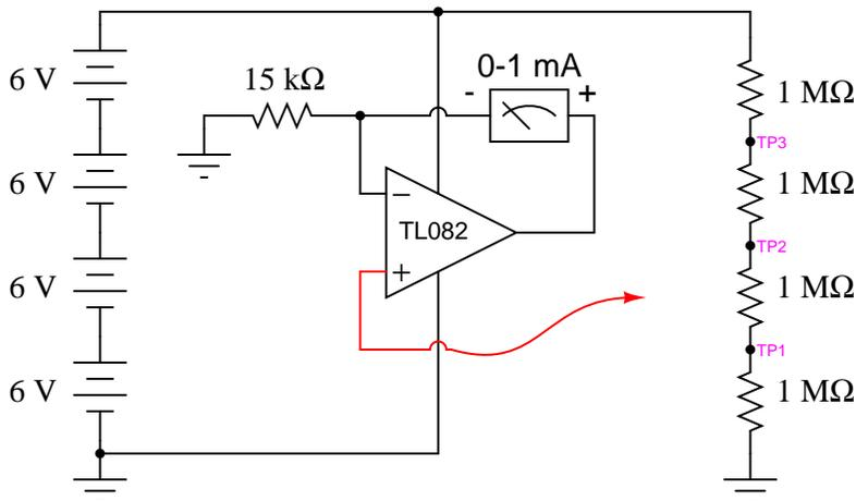
This alteration in the power supply increases the voltages at TP1, TP2, and TP3 to 6, 12, and 18 volts, respectively. With a 15 k $\Omega$  range resistor and a 1 mA meter movement, measuring 18 volts will gently "peg" the meter, but you should be able to measure the 6 and 12 volt test points just fine.
