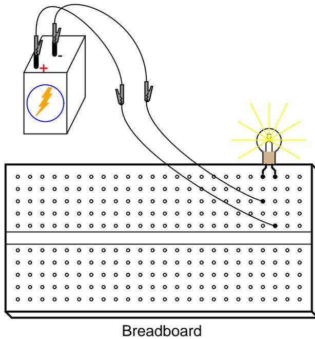
Experiment with different configurations on the breadboard, plugging the lamp into different holes. If you encounter a situation where the lamp refuses to light up and the connecting wires are getting warm, you probably have a situation known as a *short circuit*, where a lower-resistance path than the lamp bypasses current around the lamp, preventing enough voltage from being dropped across the lamp to light it up. Here is an example of a short circuit made on a breadboard:
