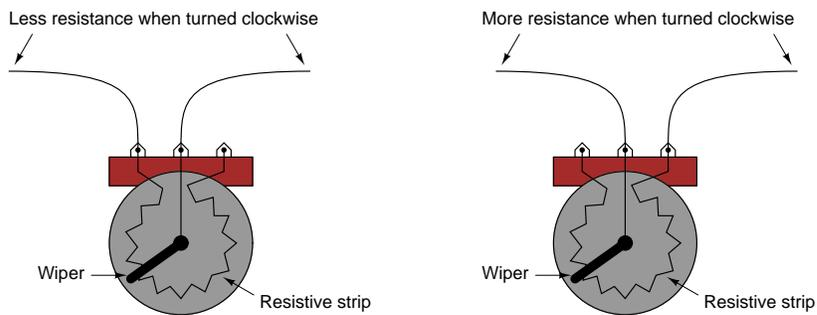
Be careful, though, that you don't use the two outer terminals, as this will result in *no change in resistance* as the potentiometer shaft is turned. In other words, it will no longer function as a *variable* resistance:
