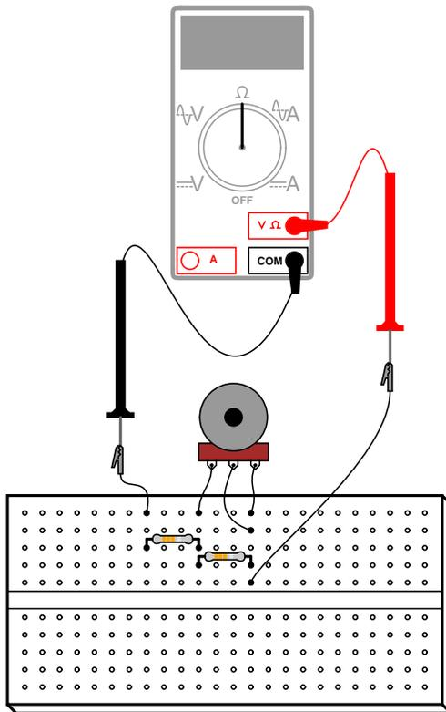
There is nothing we can do to *increase* the span of this rheostat circuit, short of replacing the potentiometer with another of greater total resistance. Adding resistors in parallel can only decrease the span. However, there is no such restriction with calibrating the zero point of this circuit, as it began at  $0 \Omega$  and may be made as great as we wish by adding resistance in series.
