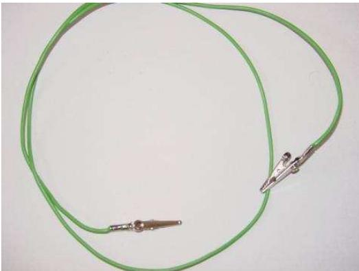
The home-made jumper wires with large, uninsulated (bare metal) alligator clips are okay to use so long as care is taken to avoid any unintentional contact between the bare clips and any other wires or components. For use in crowded breadboard circuits, jumper wires with insulated (rubber-covered) clips like the jumper shown from Radio Shack are much preferred.
