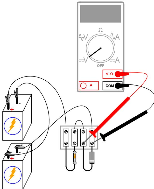
Connect three, then four 6-volt batteries together in series, forming an 18 volt and 24 volt power source, respectively. Measure and record the diode's and resistor's voltage drops for each new power supply voltage. What do you notice about the diode's voltage drop for these four different source voltages? Do you see how the diode voltage never exceeds a level of 12 volts? What do you notice about the resistor's voltage drop for these four different source voltage levels?
