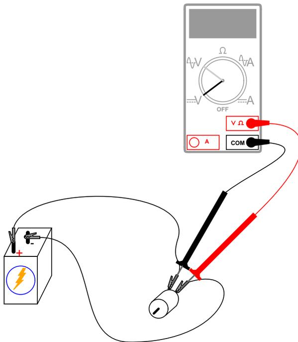
Batteries give very "pure" DC power, and as a result there should be very little AC voltage measured across the motor in this circuit. Whatever AC voltage *is* measured across the motor is due to the motor's pulsating current draw as the brushes make and break contact with the rotating commutator bars. This pulsating current causes pulsating voltages to be dropped across any stray resistances in the circuit, resulting in pulsating voltage "dips" at the motor terminals.
