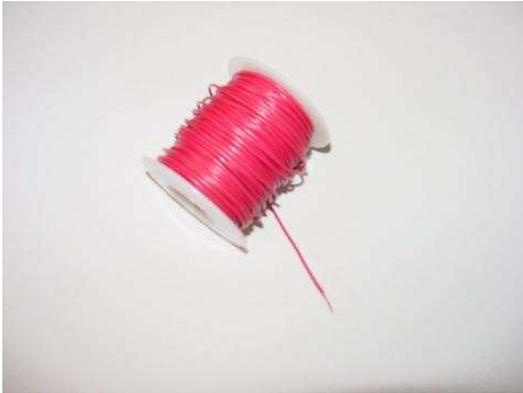
Note how the last 1/4 inch or so of the copper wire protruding from the spool has been "stripped" of its plastic insulation.
