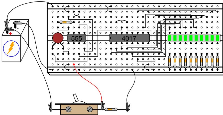
Please note that since we are using the 555 once again to provide a clock signal to the 4017, we must re-connect pin #3 of the 555 chip to pin #14 of the 4017 chip! Also, if you have altered the values of the resistor or capacitor in the 555 timer circuit, you should return to the original 1 MΩ and 0.1 μF components.
