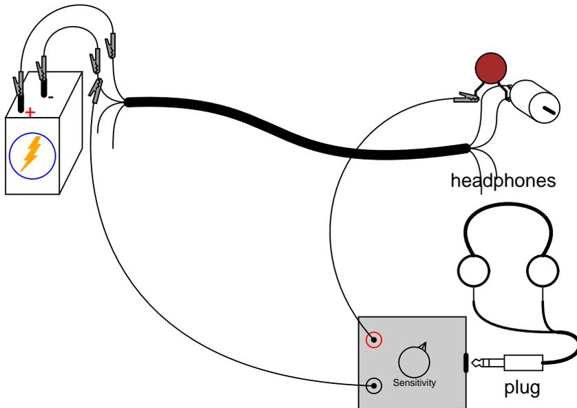
Now that we have established how AC noise is created and distributed in this circuit, let's explore how it is *coupled* to adjacent wires in the cable. Use the audio detector to measure voltage between one of the motor terminals and one of the unused wires in the telephone cable. The  $0.047 \mu\text{F}$  capacitor is not needed in this exercise, because there is no DC voltage between these points for the detector to detect anyway:
