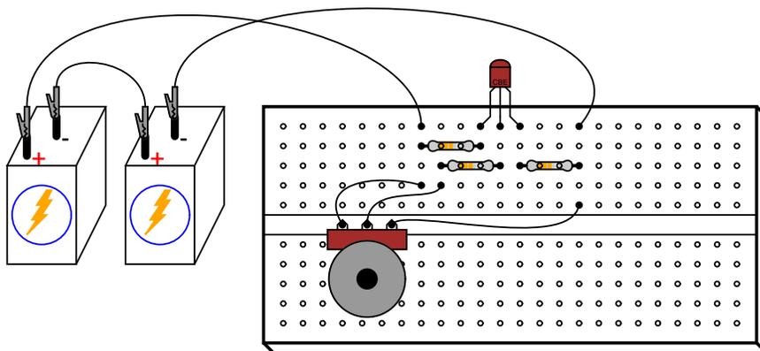
Repeat the same voltage measurement and recording exercise with the 1.5 kΩ resistor installed, calculating the new (reduced) voltage gain. Try altering the transistor's temperature again and noting the output voltage for a steady input voltage. Does it change more or less than without the 1.5 kΩ resistor?
