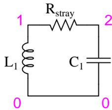
$R_{stray}$  is placed in the circuit to dampen oscillations and produce a more realistic simulation. A lower  $R_{stray}$  value causes longer-lived oscillations because less energy is dissipated. Eliminating this resistor from the circuit results in endless oscillation.
