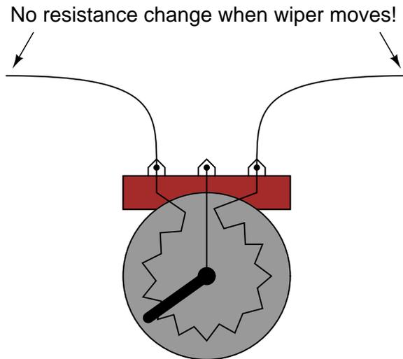
Build the circuit as shown in the schematic and illustration, using just two terminals on the potentiometer, and see how motor speed may be controlled by adjusting shaft position. Experiment with different terminal connections on the potentiometer, noting the changes in motor speed control. If your potentiometer has a high resistance (as measured between the two outer terminals), the motor might not move at all until the wiper is brought very close to the connected outer terminal.
