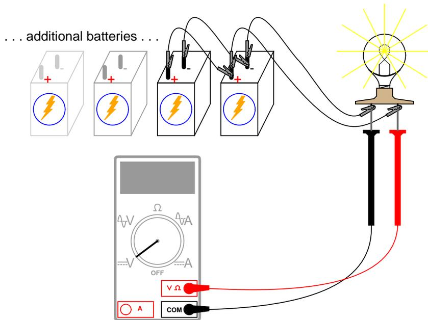
There should also be a noticeable difference in light intensity as the voltage "sag" is improved.
