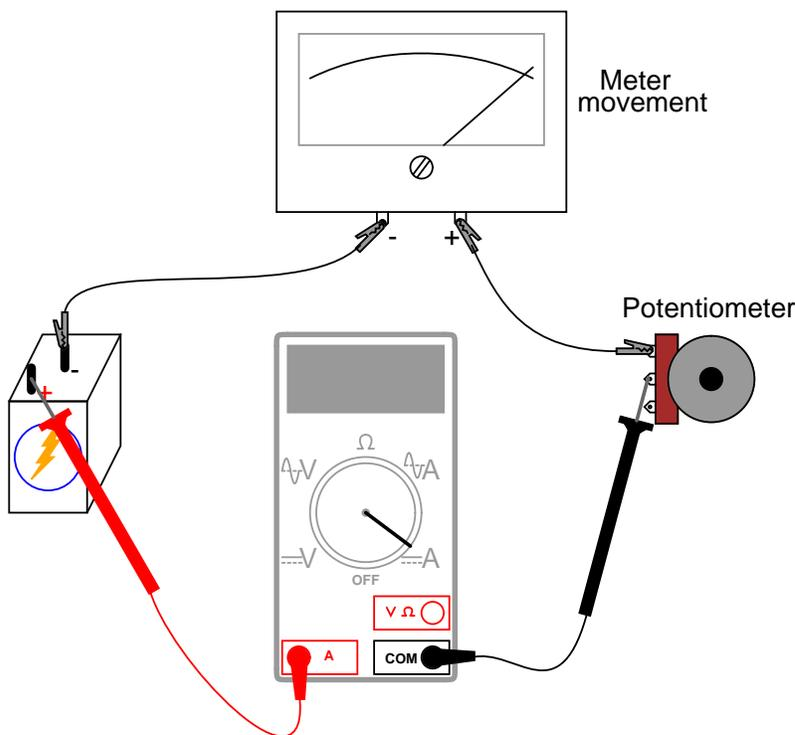
Be very careful not to apply too much current to the meter movement, as movements are very sensitive devices and easily damaged by overcurrent. Most meter movements have full-scale deflection current ratings of 1 mA or less, so choose a potentiometer value high enough to limit current appropriately, and begin testing with the potentiometer turned to maximum resistance. The lower the full-scale current rating of a movement, the more sensitive it is.
