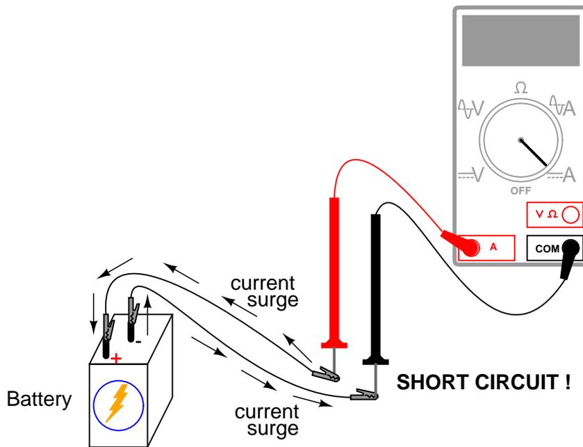
Ammeters are generally protected from excessive current by means of a small *fuse* located inside the meter housing. If the ammeter is accidentally connected across a substantial voltage source, the resultant surge in current will "blow" the fuse and render the meter incapable of measuring current until the fuse is replaced. **Be very careful to avoid this scenario!**
