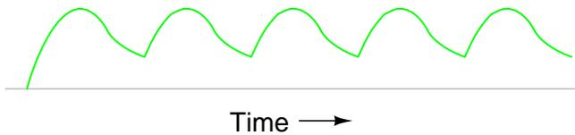
If less ripple is desired under heavy-load conditions, a larger capacitor may be used, or a more complex filter circuit may be built using two capacitors and an inductor:
