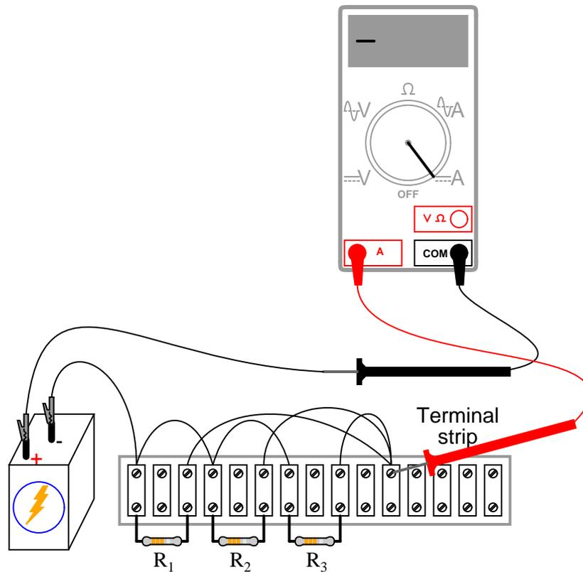
Note both the magnitude and the sign of the current as indicated by the ammeter. Add this figure (algebraically) to the three resistor currents. What do you notice about the result that is similar to the Kirchhoff's Voltage Law experiment? Kirchhoff's Current Law is to currents "summing" at a point (node) in a circuit, just as Kirchhoff's Voltage Law is to voltages adding in a series loop: in both cases, the algebraic sum is equal to zero.
