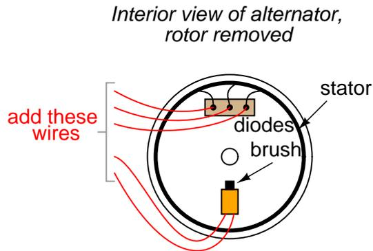
I recommend that you solder ring-lug terminals to your wires, and attach them underneath the terminal nuts along with the stator wire ends, so that each diode block terminal is securing two ring lugs.
