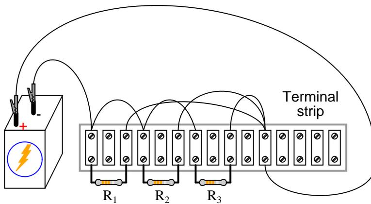
Normally, it is considered improper to secure more than two wires under a single terminal strip screw. In this illustration, I show three wires joining at the top screw of the rightmost lug used on this strip. This is done for the ease of proving a concept (of current *summing* at a circuit node), and does not represent professional assembly technique.
