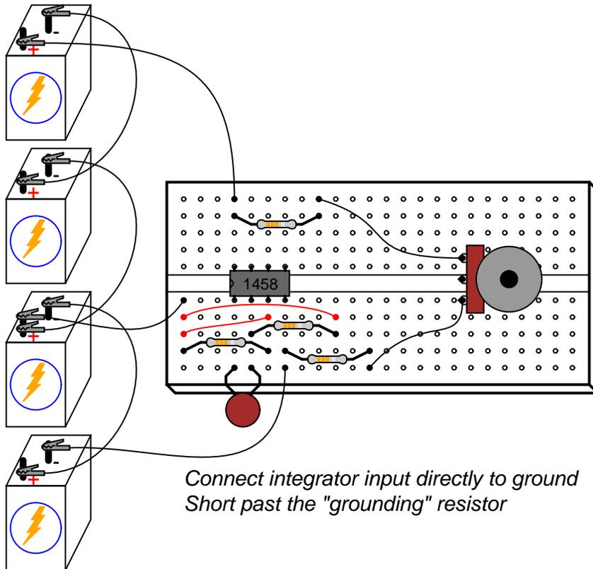
Connect integrator input directly to ground
