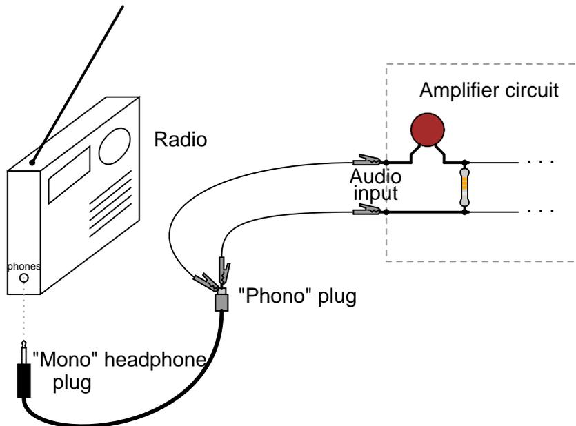
This amplifier circuit also works well in amplifying "line-level" audio signals from high-quality, modular stereo components. It provides a surprising amount of sound power when played through a large speaker, and may be run without heat sinks on the transistors (though you should experiment with it a bit before deciding to forego heat sinks, as the power dissipation varies according to the type of speaker used).
