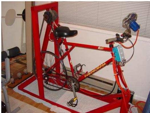
You can see a bank of three 12-volt "RV" light bulbs behind the bicycle unit (in the lower-left corner of the photograph), which I use for a load when riding the bicycle as an exercise machine. A set of three switches is mounted at the front of the bicycle, where I can turn loads on and off while riding.
