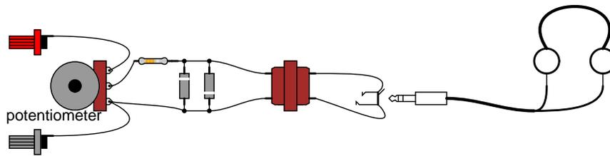
Adjust the 100 k $\Omega$  voltage divider potentiometer to about mid-range when initially sensing a voltage signal of unknown magnitude. If the sound is too loud, turn the potentiometer down and try again. If too soft, turn it up and try again. The detector produces a "click" sound whenever the test leads make or break contact with the voltage source under test. With my cheap headphones, I've been able to detect currents of less than 1/10 of a microamp ( $< 0.1 \mu\text{A}$ ).
