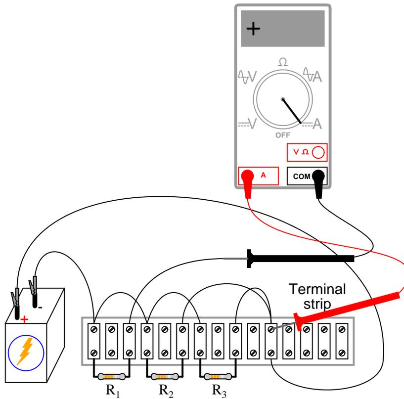
Measure current for each of the three resistors, comparing with the current figures calculated previously. With the digital ammeter connected as shown, all three indications should be positive, not negative.
