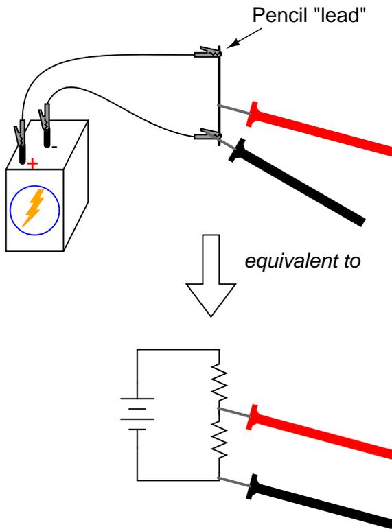
Now, change the voltmeter connection to the circuit so as to measure voltage across the "upper resistor" of the pencil lead, like this:
