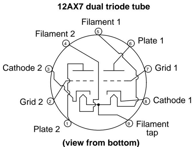
You will notice on the amplifier schematic that both triode elements inside the 12AX7's glass envelope are being used, in parallel: plate connected to plate, grid connected to grid, and cathode connected to cathode. This is done to maximize power output from the tube, but it is not necessary for demonstrating basic operation. You may use just one of the triodes, for simplicity, if you wish.
