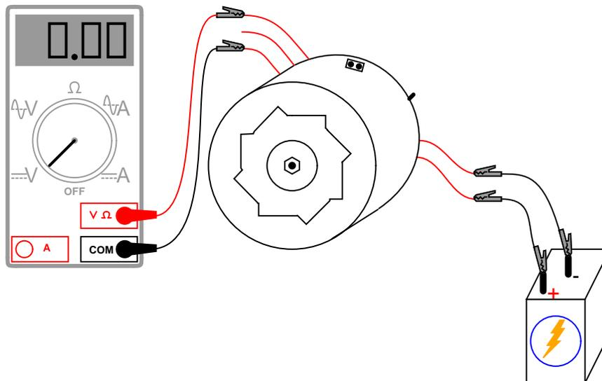
With the multimeter set to the "DC volts" function, *slowly* rotate the alternator shaft. The voltmeter reading should alternate between positive and negative as the shaft it turned: a demonstration of very slow alternating voltage (AC voltage) being generated. If this test is successful, switch the multimeter to the "AC volts" setting and try again. Try spinning the shaft slow and fast, comparing voltmeter readings between the two conditions.
