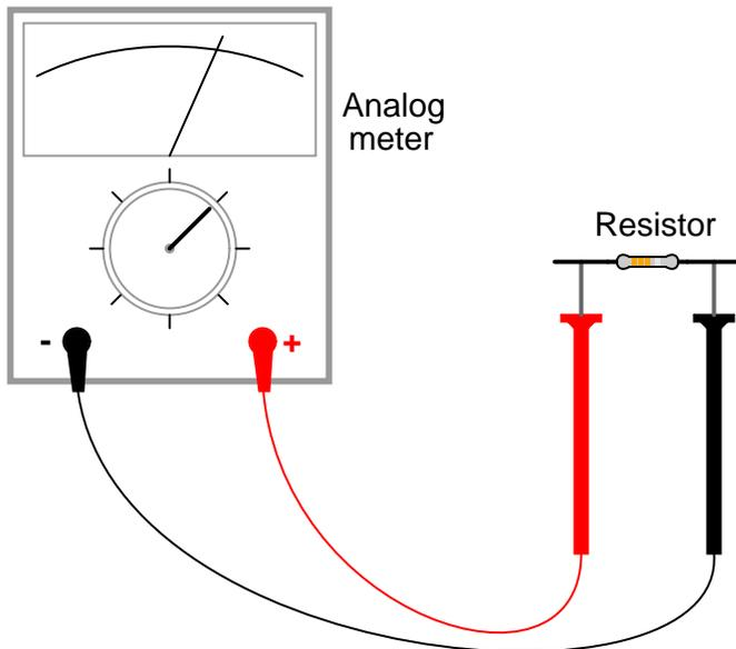
If the needle points very close to zero, you need to select a lower resistance range on the meter, just as you needed to select an appropriate voltage range when reading the voltage of a battery.
