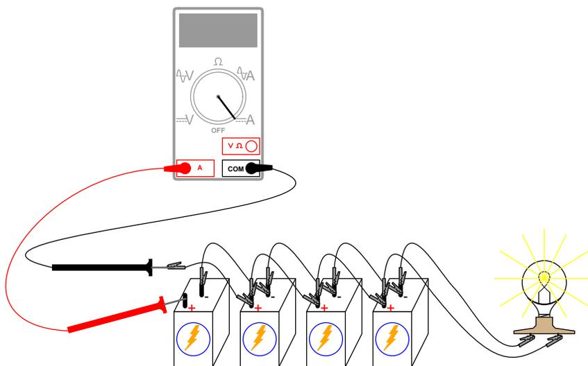
By breaking the circuit for just one battery, and inserting our ammeter within that break, we intercept the current of that one battery and are therefore able to measure it. Measuring total current involves a similar procedure: make a break somewhere in the path that total current must take, then insert the ammeter within than break:
