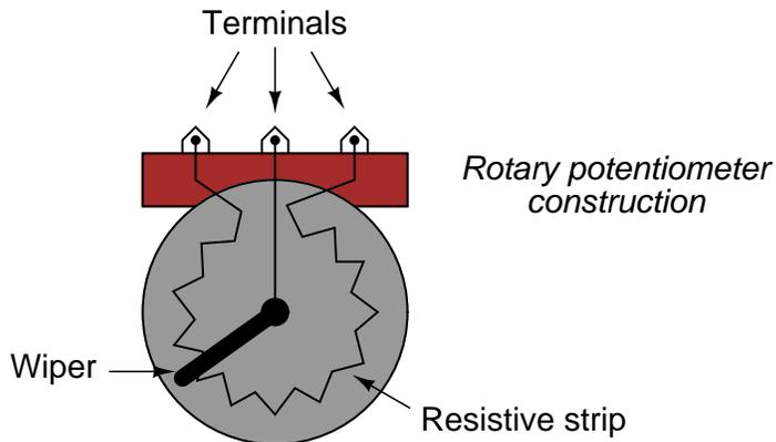
Some rotary potentiometers have a spiral resistive strip, and a wiper that moves axially as it rotates, so as to require multiple turns of the shaft to drive the wiper from one end of the potentiometer's range to the other. Multi-turn potentiometers are used in applications where precise setting is important.
