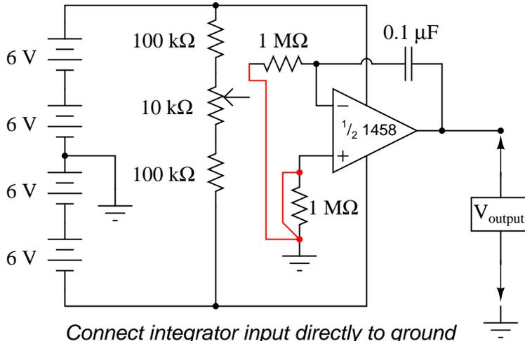
Connect integrator input directly to ground
