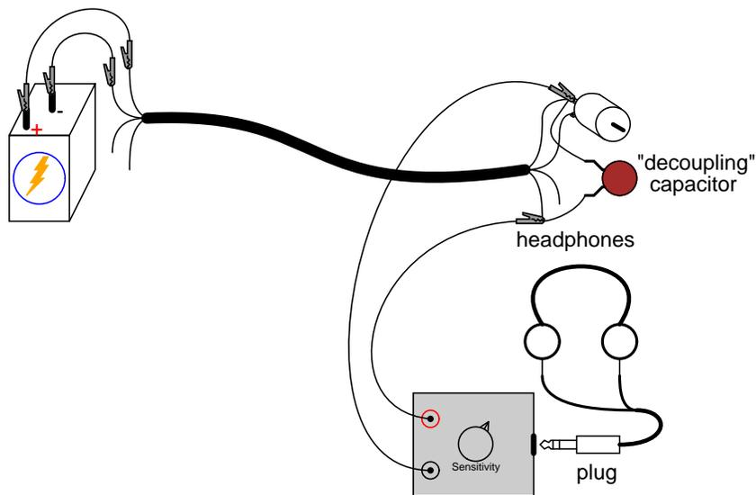
The *decoupling capacitor* acts as a practical short-circuit to any AC noise voltage, while not affecting DC voltage signals between those two points at all. So long as the decoupling capacitor value is significantly larger than the stray "coupling" capacitance between the cable's conductors, the AC noise voltage will be held to a minimum.
