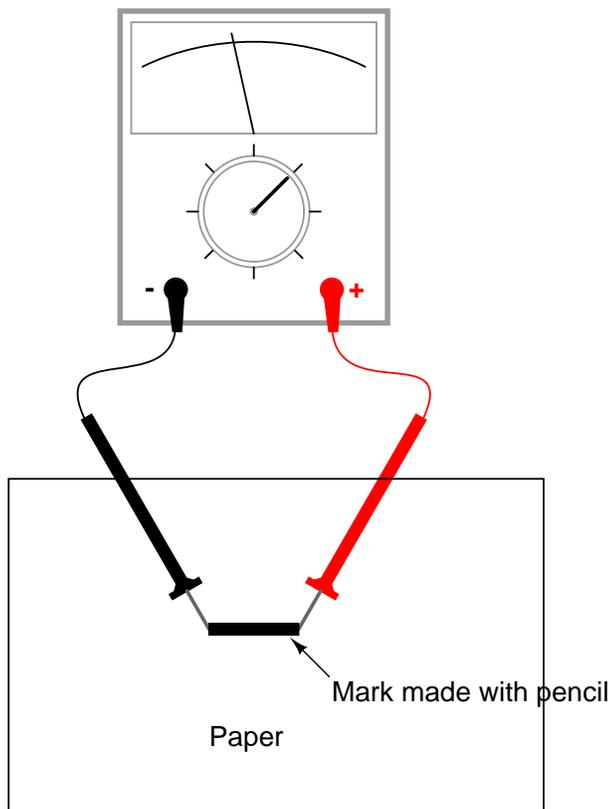
Move the probe tips closer together on the black mark and note the change in resistance value. Does it increase or decrease with decreased probe spacing? If the results are inconsistent, you need to redraw the mark with more and heavier pencil strokes, so that it is consistent in its density. What does this teach you about resistance versus length of a conductive material?
