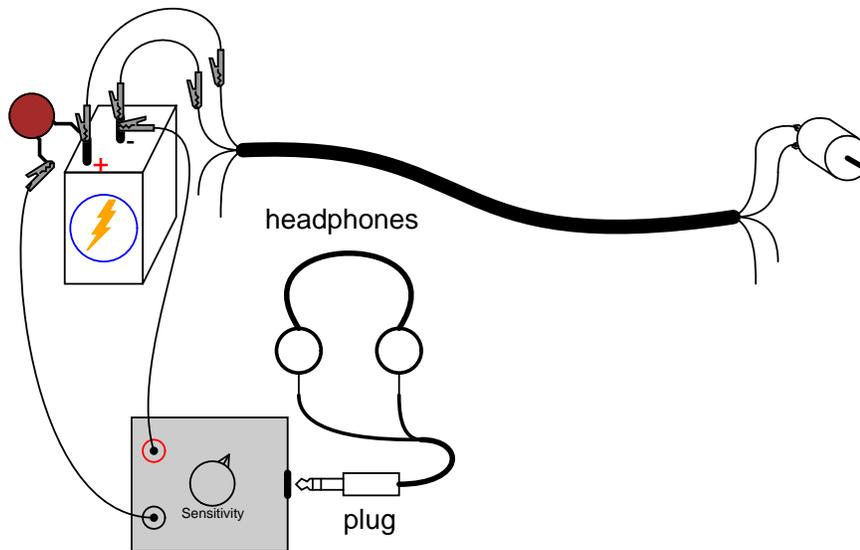
You may also measure noise voltage dropped along either of the telephone cable conductors supplying power to the motor, by connecting the audio detector between both ends of a single cable conductor. The noise detected here originates from current pulses through the resistance of the wire:
