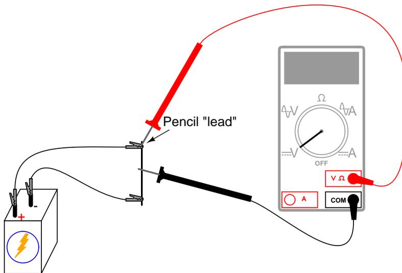
Move the black test probe position along the length of the rod, noting the voltmeter indication. Which position gives the greatest voltage drop for the meter to measure? Does this differ from the previous arrangement? Why?
