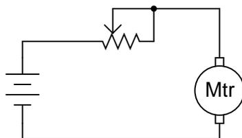
At first, this seems rather pointless, as it has no impact on resistance control. You may verify this fact for yourself by inserting another wire in your circuit and comparing motor behavior before and after the change:
