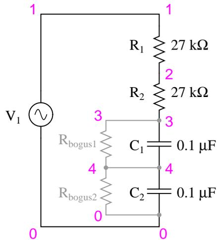
The two large-value resistors  $R_{bogus1}$  and  $R_{bogus2}$  are connected across the capacitors to provide a DC path to ground in order that SPICE will work. This is a "fix" for one of SPICE's quirks, to avoid it from seeing the capacitors as open circuits in its analysis. These two resistors are entirely unnecessary in the real circuit.
