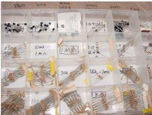
In this view of one of my component boxes, you can see plenty of 1/8 watt resistors, transistors, diodes, and even a few 8-pin integrated circuits ("chips"). Labels for each compartment were made with a permanent ink marker.
