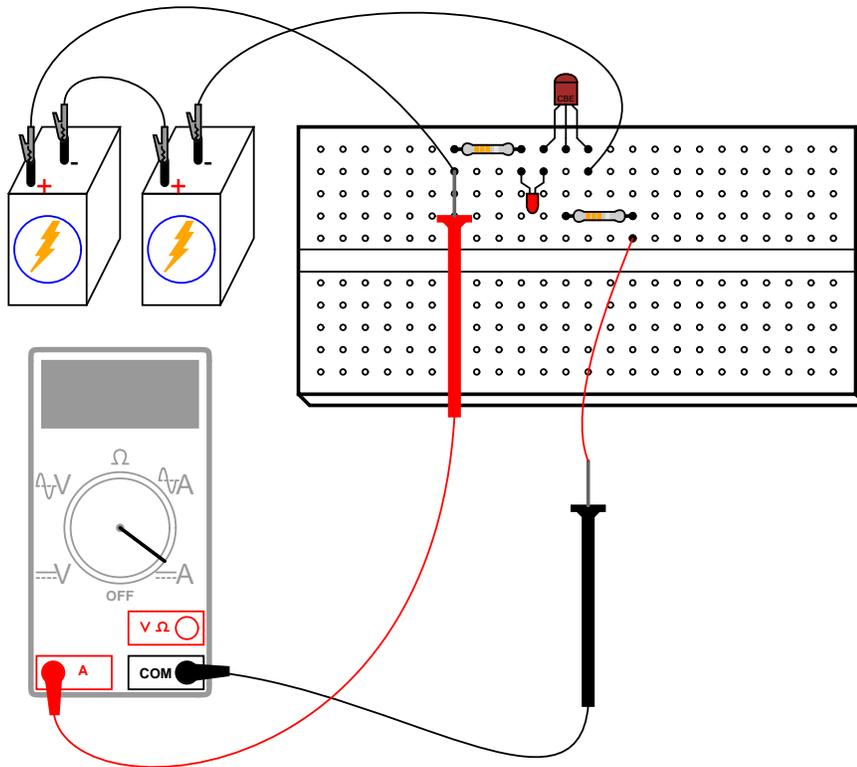
You may have to select the most sensitive current range on the meter to measure this small flow. After measuring this *controlling* current, try measuring the LED's current (the *controlled* current) and compare magnitudes. Don't be surprised if you find a ratio in excess of 200 (the controlled current 200 times as great as the controlling current)!
