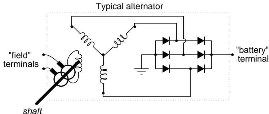
An automotive alternator is a three-phase generator with a built-in rectifier circuit consisting of six diodes. As the sheave (most people call it a "pulley") is rotated by a belt connected to
