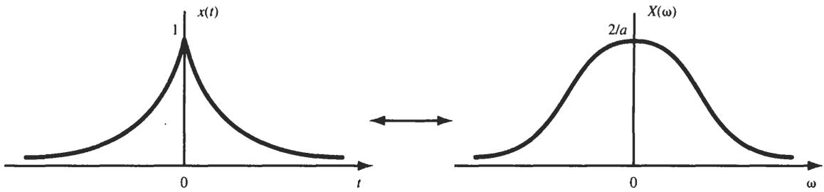
Fig. 5-18  $e^{-a|t|}$  and its Fourier transform.
