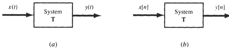
Fig. 1-15 (a) Continuous-time system; (b) discrete-time system.
