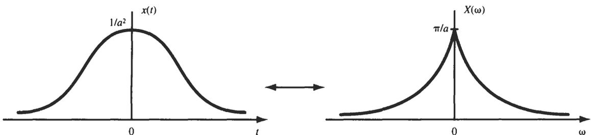
Fig. 5-19  $1/(a^2 + t^2)$  and its Fourier transform.
