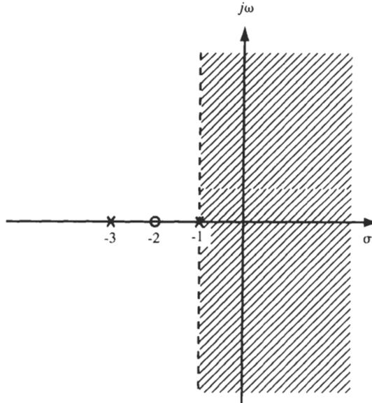
Fig. 3-3  $s$ -plane representation of  $X(s) = (2s + 4)/(s^2 + 4s + 3)$ .
