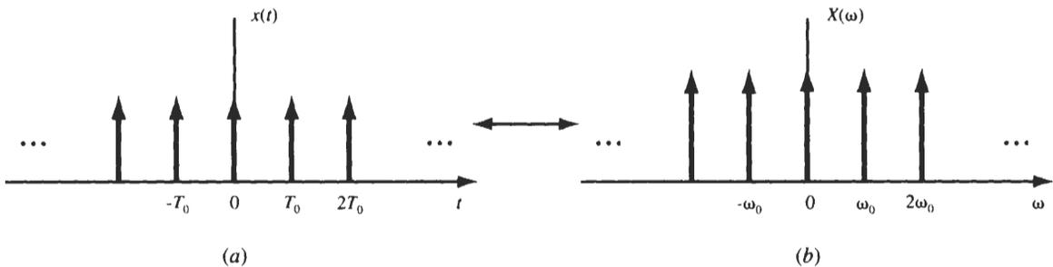
Fig. 5-22 Unit impulse train and its Fourier transform.
