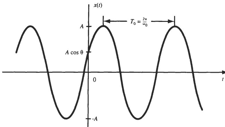
Fig. 1-9 Continuous-time sinusoidal signal.
