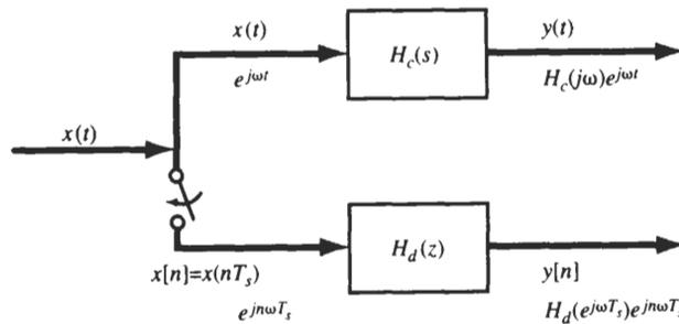
Fig. 6-5 Digital simulation of analog systems.
