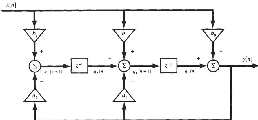
Fig. 7-8 Canonical simulation of the first form.
