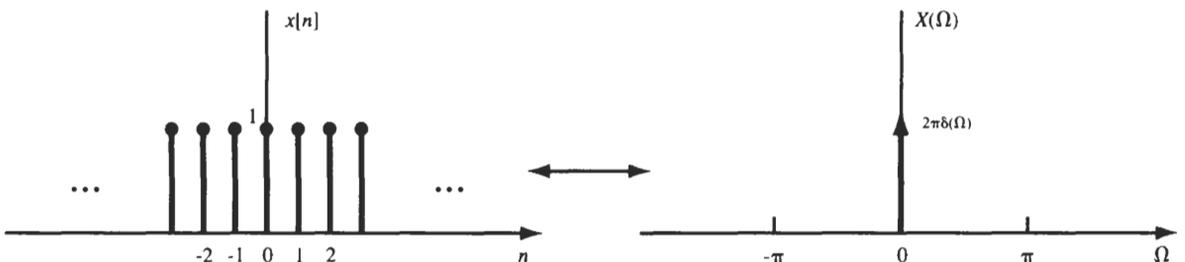
**Fig. 6-14** A constant sequence and its Fourier transform.
