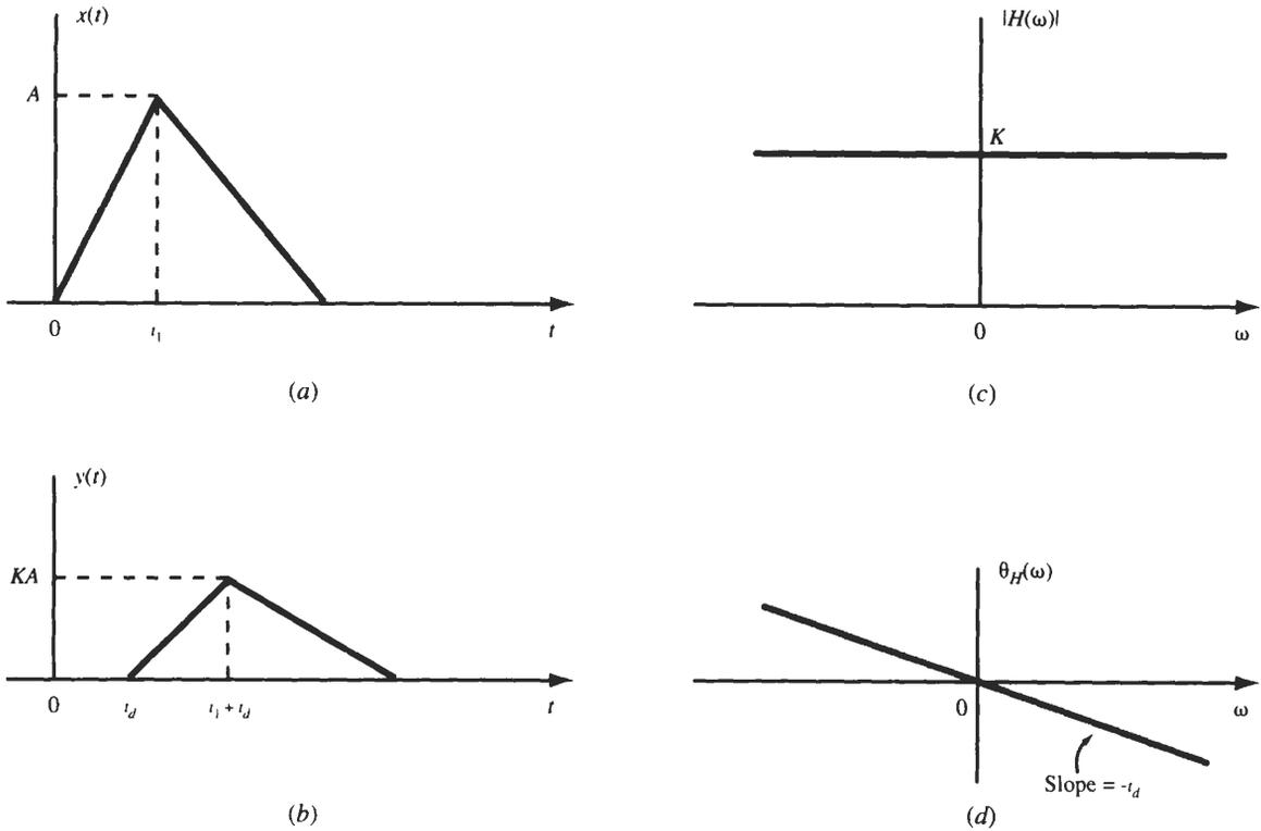
Fig. 5-4 Distortionless transmission.
