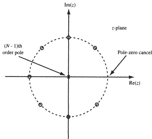
Fig. 4-4 Pole-zero plot with  $N=8$ .
