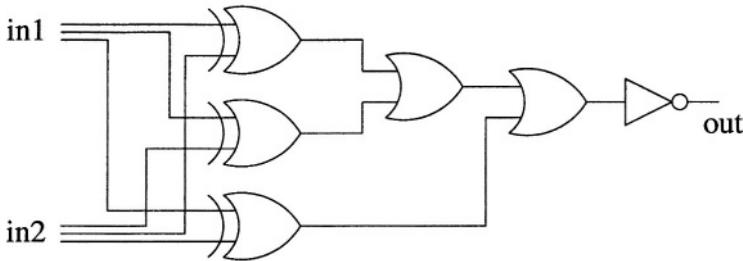
**Fig. 1.6.** Circuit diagram of a 3-bit equality tester
