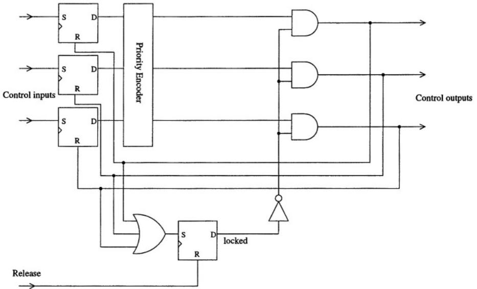
Fig. 5.12. The Design of a Fixed-Priority Synchronous Arbiter
