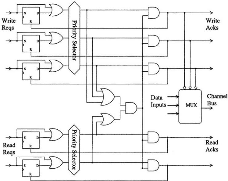
**Fig. 7.4.** A Channel Controller. The synchronous RS flip-flops (R-dominant) are used to latch pending requests (represented as 1-cycle pulses). Static fixed priority selectors are used to arbitrate between multiple requests. The three data-inputs are used by the three writers to put data onto the bus
