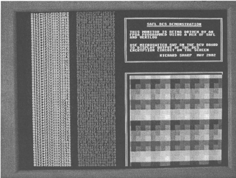
**Fig. 10.10.** A screenshot of the DES circuit displaying its inputs and outputs on a VGA monitor
