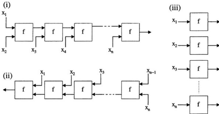
**Fig. 2.5.** The geometrical (circuit-level) interpretation of some  $\mu\text{FP}$  combining forms. (i)  $(/L f) \langle x_1, x_2, \dots, x_n \rangle$ ; (ii)  $(/R f) \langle x_1, x_2, \dots, x_n \rangle$ ; (iii)  $(\alpha f) \langle x_1, x_2, \dots, x_n \rangle$
