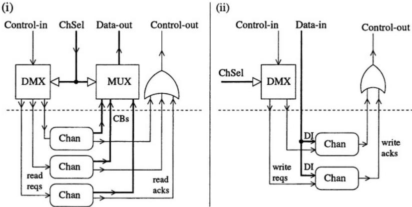
**Fig. 7.5.** (i) A READ node connected to three channels; (ii) A WRITE node connected to two channels. The component marked DMX is a demultiplexer which routes the control signal to one of the three channels depending on the value of its select input (ChSel)
