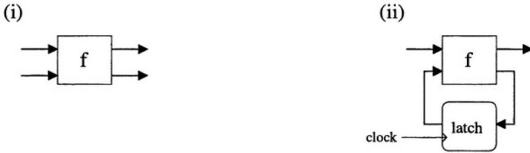
**Fig. 2.6.** The hardware-level realisation of the  $\mu$  combinator— (i) function  $f : \alpha \times \beta \rightarrow \gamma \times \beta$ ; (ii) the effect of applying the  $\mu$  combinator, yielding a function  $\mu f : \alpha \rightarrow \gamma$
