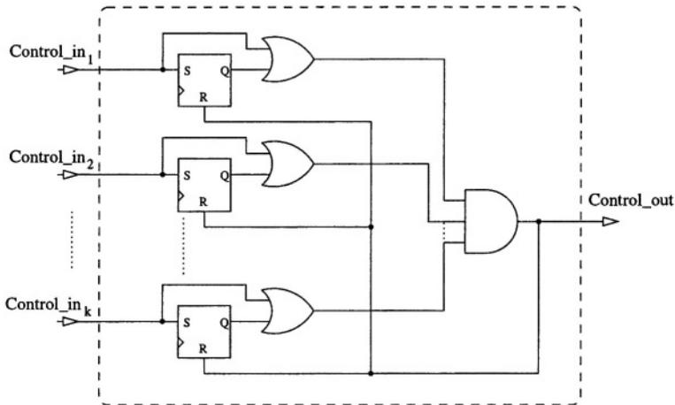
Fig. 5.8. Hardware block corresponding to a CONTROL\_JOIN node
