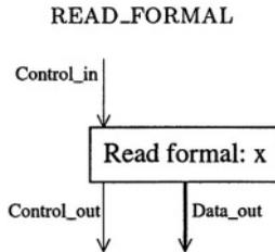
This node propagates control whilst writing the value of the local function's formal parameter,  $x$ , to its data-output. Figure 5.5 shows an example of the `READ_FORMAL` node by translating the body of `fun f(x) = x+3`.
