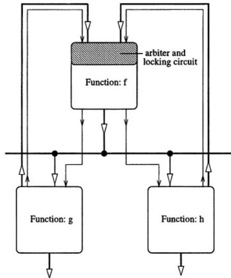
**Fig. 4.4.** A structural diagram of the hardware circuit corresponding to a shared function,  $f$ , called by functions  $g$  and  $h$ . Data buses are shown as thick lines, control wires as thin lines
