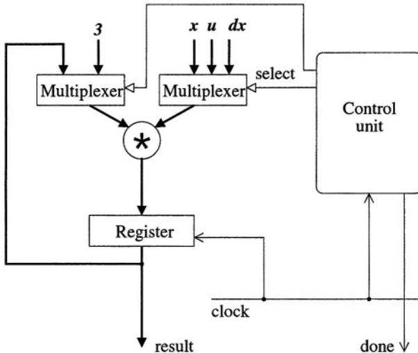
**Fig. 1.1.** A diagrammatic view of a circuit to compute  $3 \cdot x \cdot u \cdot dx$
