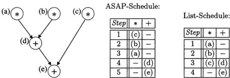
**Fig. 1.10.** (left) the dependencies between operations for an expression of the form  $xy + z$ . Operations are labelled with letters (a)–(e); (centre) an ASAP Schedule of the expression for a single adder and a single multiplier. (right) a List Schedule under the same resource constraints
