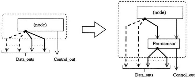
**Fig. 6.2.** We insert permanisors on data-edges using this transformation. The dashed data-edges represent those which do not require permanisors; the solid data-edges represent those which do require permanisors
