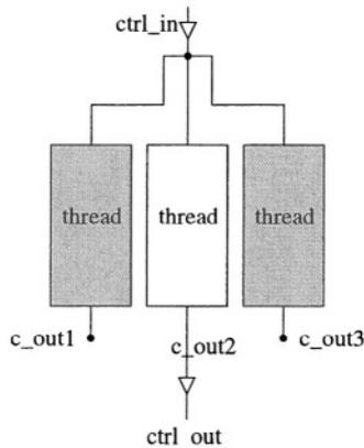
**Fig. 6.7.** A block diagram of a circuit-level implementation of 3 parallel threads. Suppose that our analysis has detected that the “done” control outputs of the 3 threads will be asserted simultaneously. Thus we have no need for a CONTROL\_JOIN NODE. Since signals “c\_out1” and “c\_out3” are no longer connected to anything we can optimise away the control circuitry of the shaded blocks
