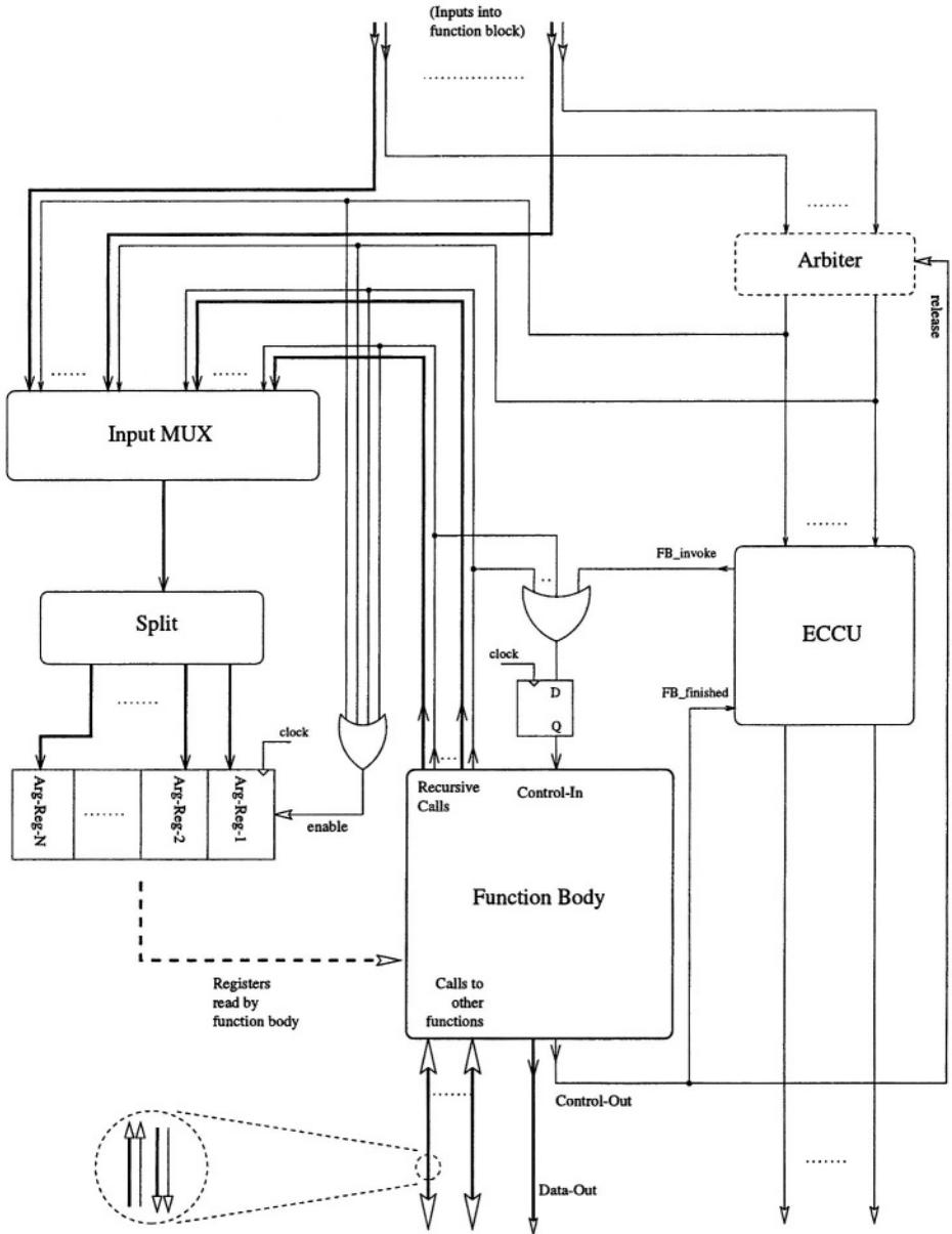
Fig. 5.10. A Block Diagram of a Hardware Functional-Unit
