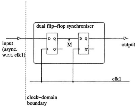
**Fig. 5.14.** A dual flip-flop synchroniser. Potential metastability occurs at the point marked “M”. However, the probability of the synchroniser’s output being in a metastable state is significantly reduced since any metastability is given a whole clock cycle to resolve
