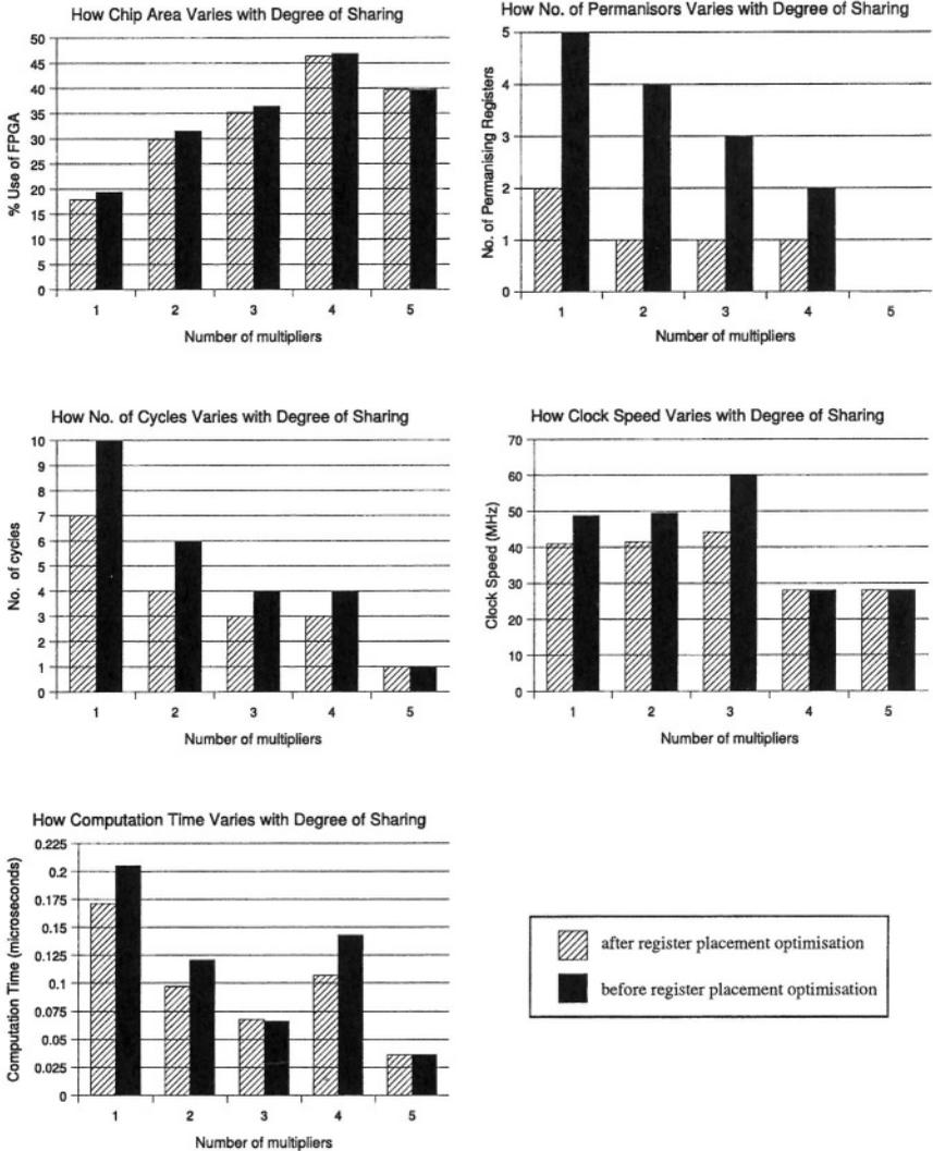
**Fig. 6.8.** How various parameters (area, number of permanisers, number of cycles, clock speeds and computation time) vary as the degree of resource sharing changes
