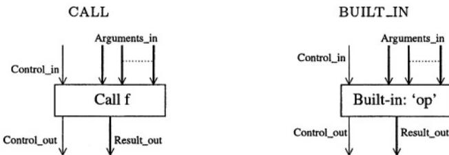
Both these nodes read their data-inputs when control reaches their single control-input, perform their operation and then return their result on the single data-output, propagating control forwards when the operation is complete. (Note that the CALL node is only used to represent non-recursive calls to external functional-units. We have already shown how we use JUMP to represent recursive calls.)
