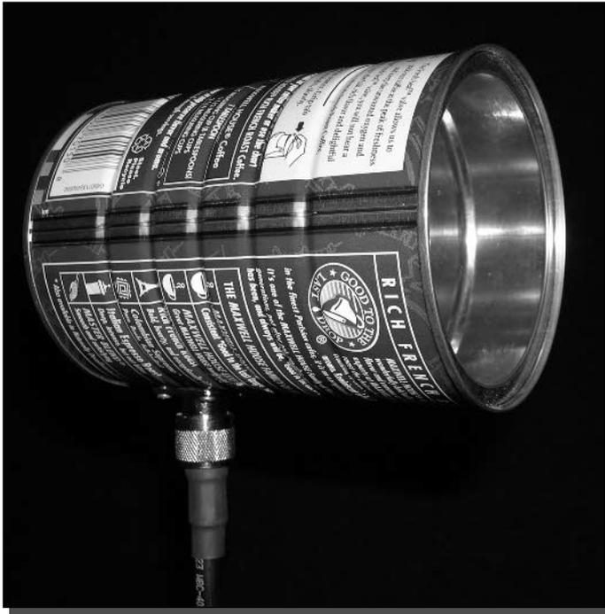
FIGURE 3-2: The tin can waveguide antenna.
