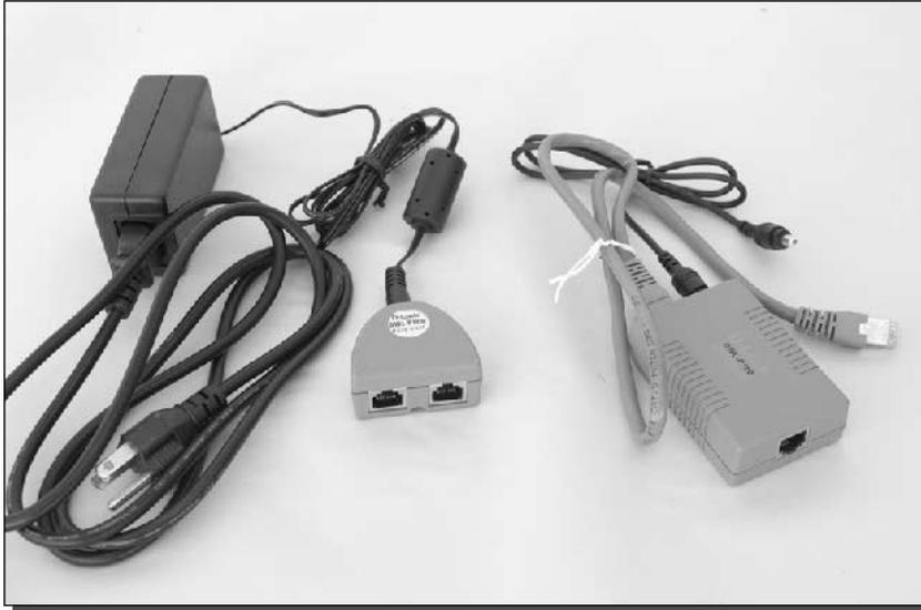
FIGURE 8-5: A Power-over-Ethernet adapter.
