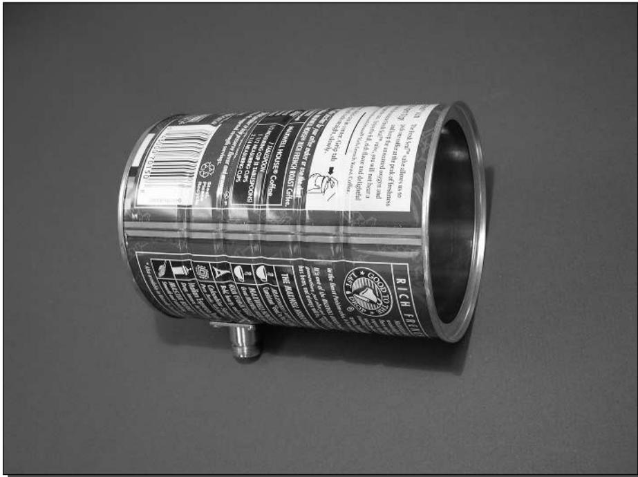
FIGURE 2-11: A waveguide antenna you can build.
