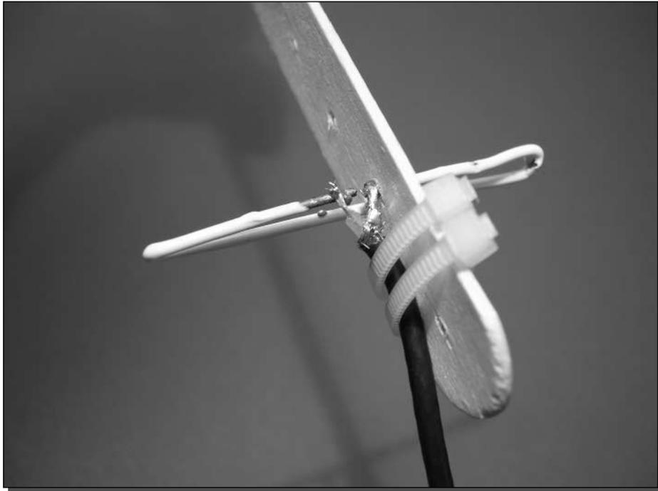
FIGURE 2-20: Cable management on your tiny antenna.
