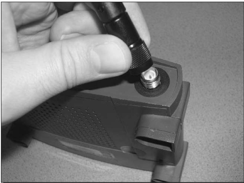
FIGURE 4-12: Removing the original antenna.
