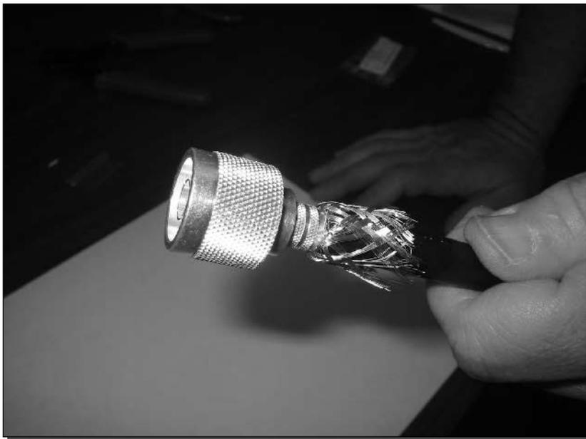
FIGURE 1-22: Connector and pin are in position.
