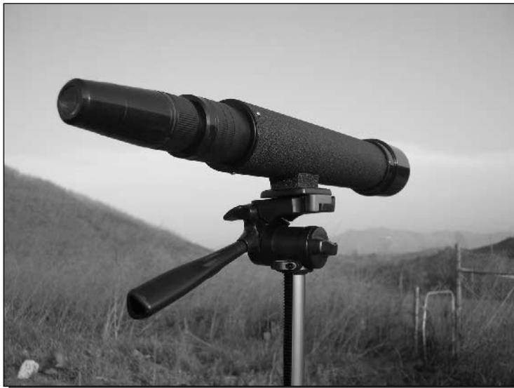
FIGURE 13-4: Spotting scope used to determine direction and angle.
