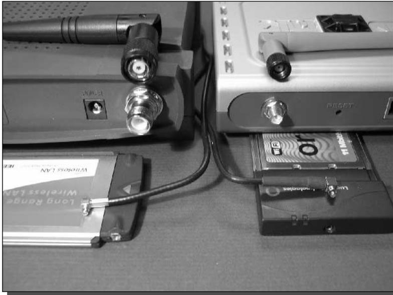
FIGURE 1-27: Various Wi-Fi connector types.
