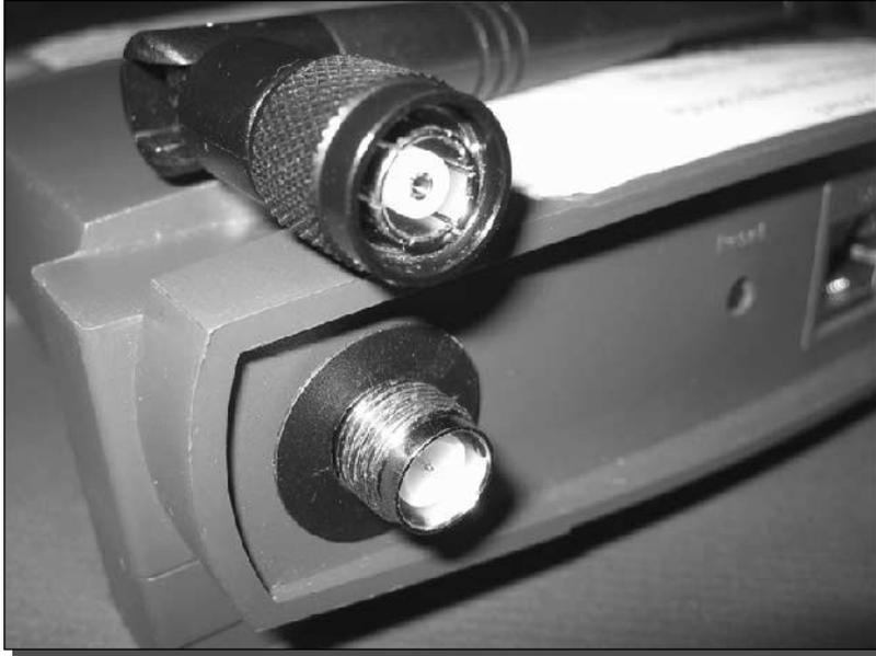
**FIGURE 4-15: Reverse Polarity TNC connectors.**
