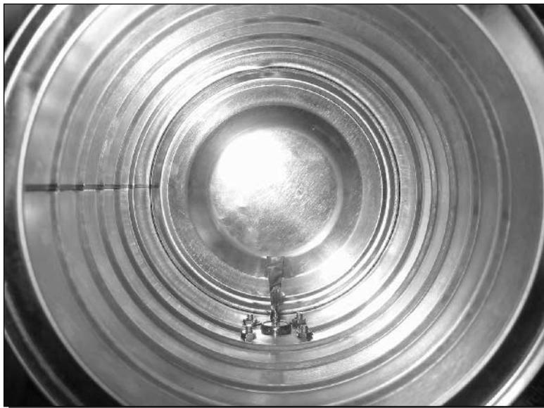
FIGURE 3-18: The mounted N-Connector assembly.
