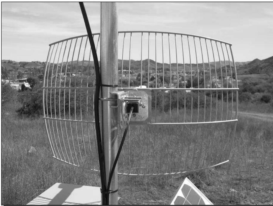
FIGURE 13-5: A parabolic dish antenna.
