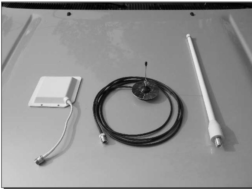
FIGURE 14-14: Antenna options: mid-gain directional, high-gain omni, and mid-gain omni.
