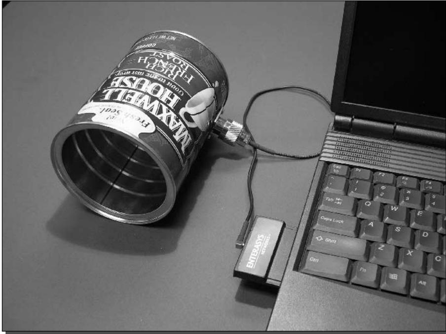
FIGURE 3-19: The completed can antenna hooked up to a laptop.
