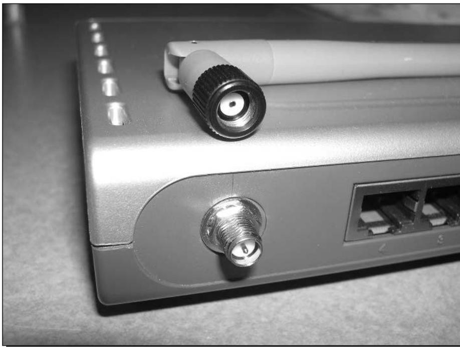
**FIGURE 4-16:** Reverse Polarity SMA connectors.
