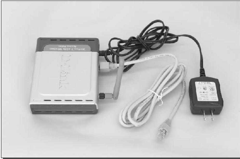
FIGURE 8-4: A wireless access point with detachable antenna and standard accessories.
