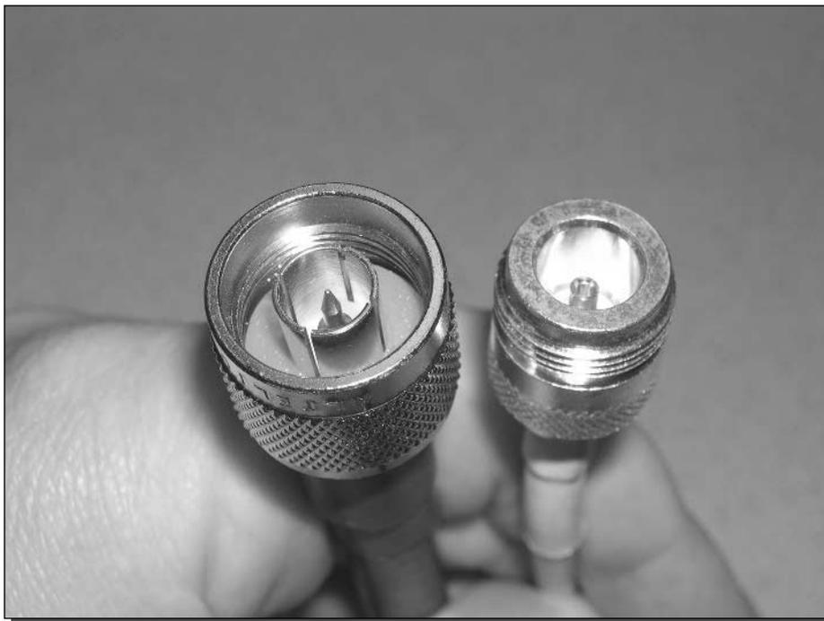
FIGURE 4-14: Standard male connector (left) and standard female connector (right).
