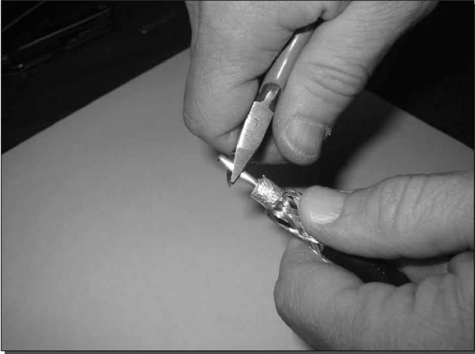
FIGURE 1-18: Clipping the core conductor.
