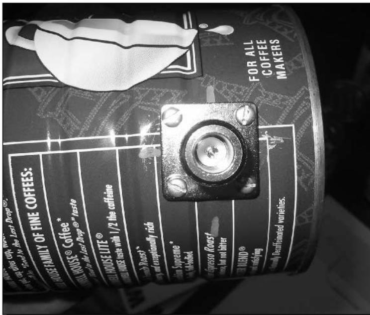
FIGURE 3-17: The connector mounted in the can.
