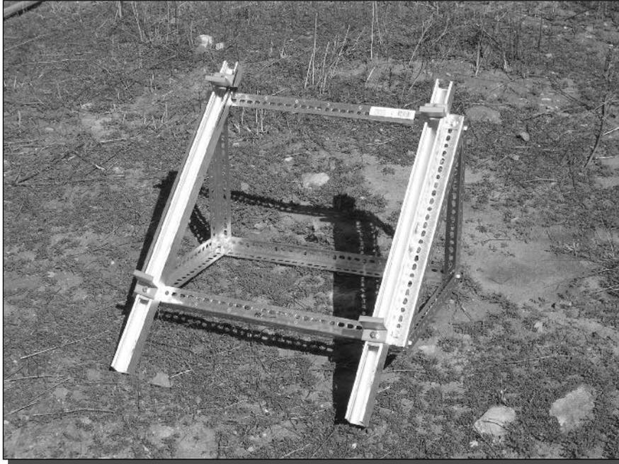
FIGURE 9-18: A solar panel mounting structure built using angle iron.
