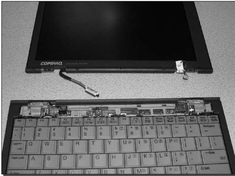
FIGURE 15-10: LCD panel removed.
