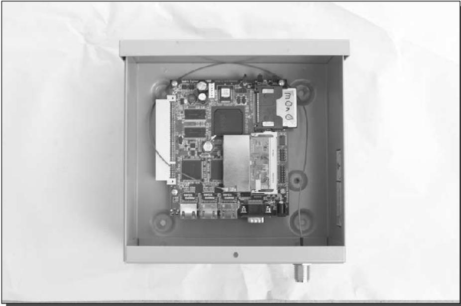
FIGURE 8-25: The Soekris single-board computer configured as a wireless access point.
