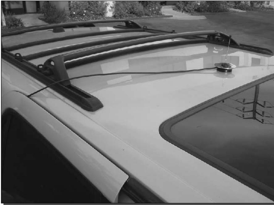
FIGURE 5-14: Magnet mount antenna placement with cable running through doorway.
