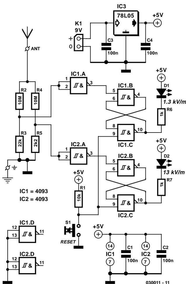
Figure 1. The core of the circuit are two potential dividers and associated flip-flops. LEDs are used to indicate and record the occurrence of two levels of electrical field strength, 1.3 kV/m and 13 kV/m.
