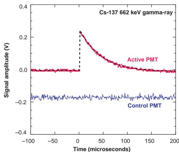
**Fig. 1.** Output signals from the active PMT (top red data points) and control PMT (bottom blue line) for one 662-keV gamma ray emitted by a Cs-137 radioactive source. The control data have been shifted down for clarity. The black dashed line is the detector response function calculated from the preamplifier circuit.
