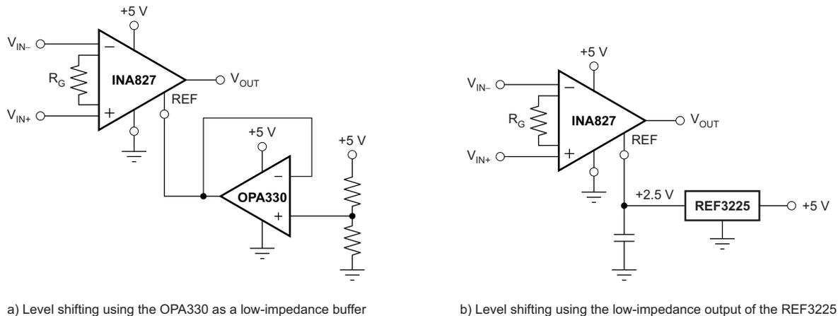
**Figure 58. Options for Low-Impedance Level Shifting**
