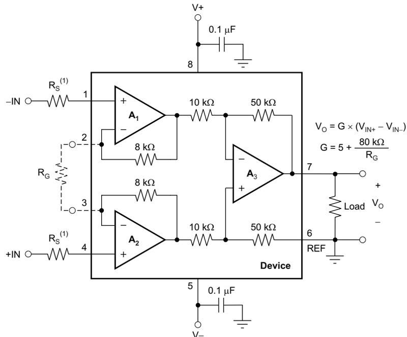
(1) This resistor is optional if the input voltage remains above  $[(V-) - 2 \text{ V}]$  or if the signal source current drive capability is limited to less than 3.5 mA. See the [Input Protection](#) section for more details.
