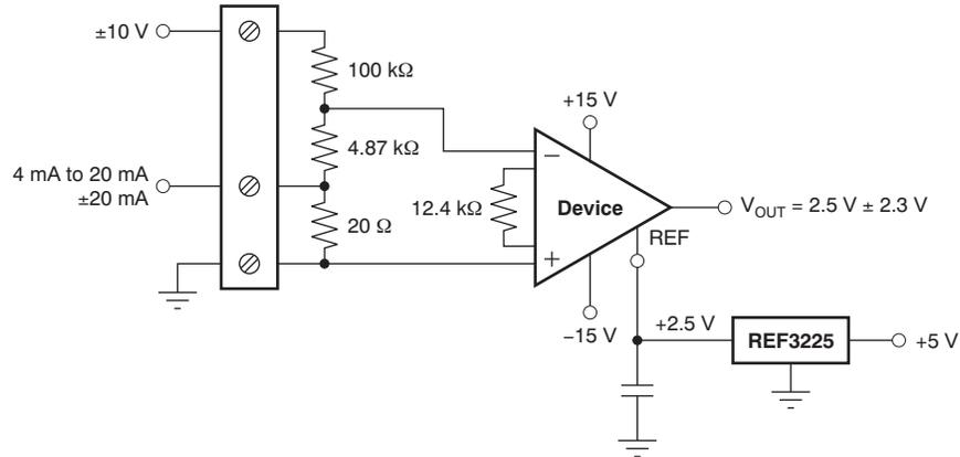
**Figure 60.  $\pm 10\text{-V}$ ,  $4\text{-mA}$  to  $20\text{-mA}$  PLC Input**
