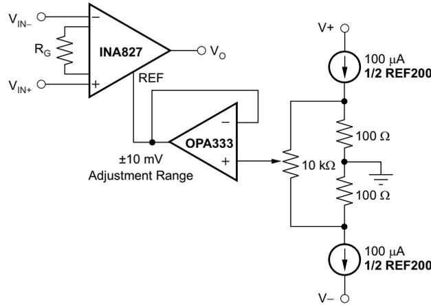
Figure 55. Optional Trimming of Output Offset Voltage
