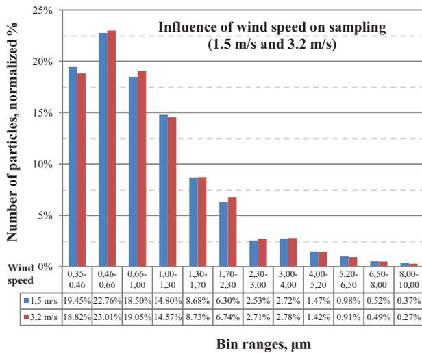
Fig. 7. Influence of wind speed on measured concentrations (with probe)
