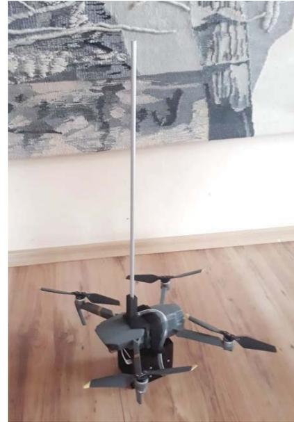
Fig. 2. Quadcopter and integrated gas-sensor system with a probe.
