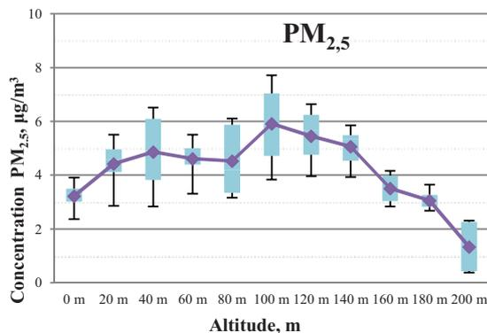
Fig. 4. Boxplot of  $\text{PM}_{2.5}$  concentration changes on 10.5.2019 with altitude increase of 20 m in intervals with a hovering of 40 sec
