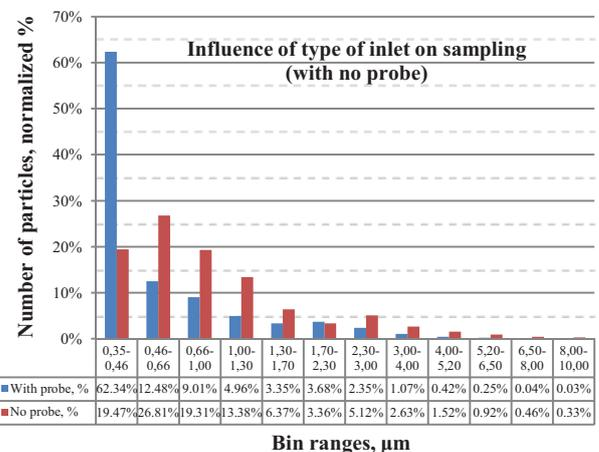
Fig. 6. Influence of type of inlet on measured concentrations
