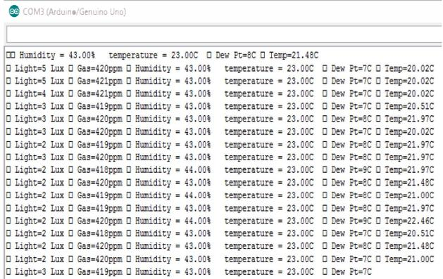
Fig. 6: Serial Monitor Output
