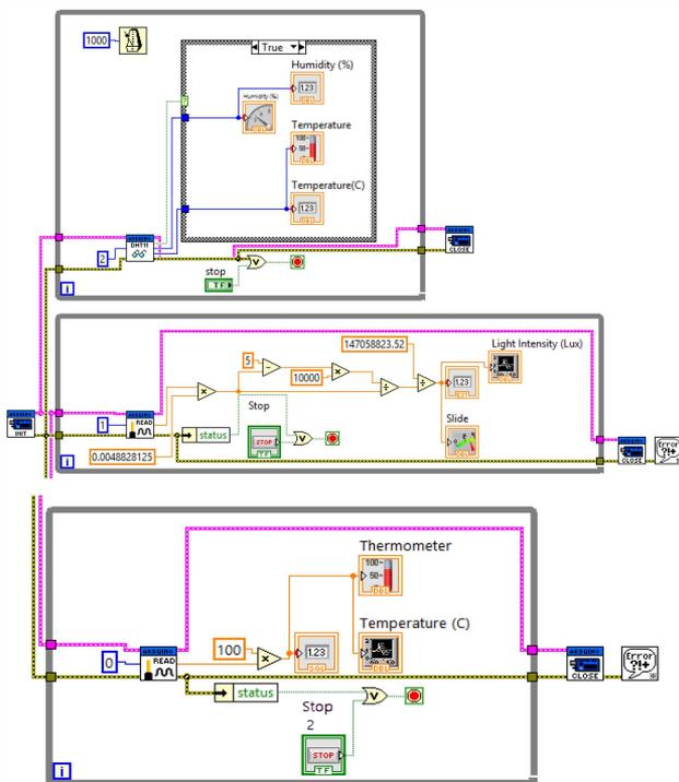
Fig. 5: Combined VI Block Diagram
