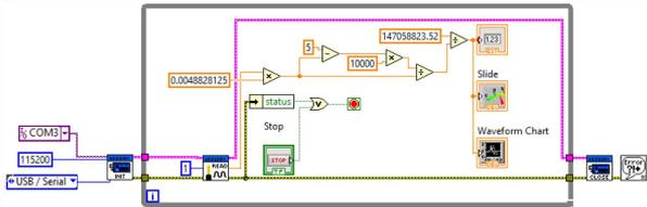
Fig. 4: NORP 12 LDR Light Sensor VI Block Diagram
