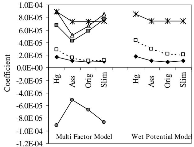
Figure 4 Model coefficients for each sensor type. (diamonds = wet potential C1, circles = dry bulb C2, triangles = wet bulb C3, squares = theoretical wet bulb depression C4, stars = constant B and open squares = standard error of the fit)
