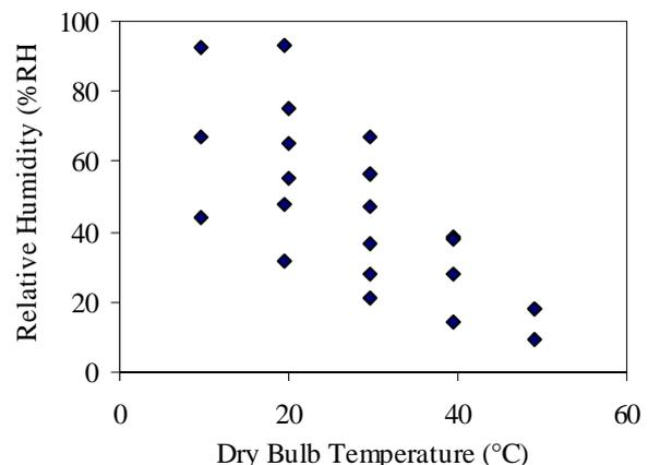
Figure 1 Conditions the wet bulb sensors were tested under.
