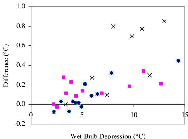
Figure 2 Plot of mean differences between the wet bulb depression measured by RTDs and ordinary thermometers at Melbourne (squares), Esperance (diamonds) and Wagga Wagga (crosses).
