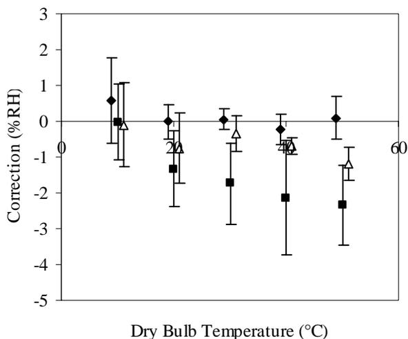
Figure 6 Dry bulb temperature versus the correction the relative humidity for the three models. (squares = theoretical model, triangles = wet potential model, diamonds = multi factor model)
