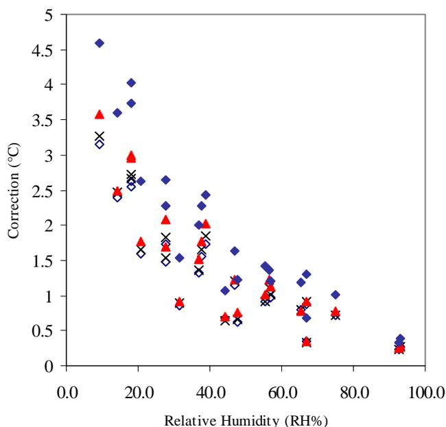
Figure 3 Correction of wet depression to the theoretical wet bulb depression at a given relative humidity. Slim RTD (Open Diamond), Original RTD (Cross), Assman (Triangle) and Ordinary thermometer (Diamond)
