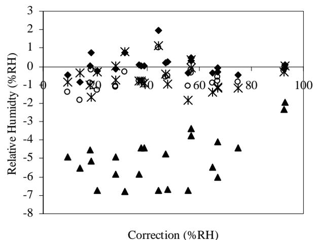
Figure 5 Reference relative humidity versus the correction in relative humidity for the ordinary mercury in glass thermometer (triangles = theoretical model, circles = wet potential model, diamonds = multi factor model and stars = multi factor model without stem correction)
