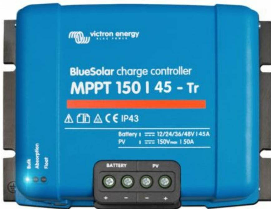
*Above: Victron Energy do a range of solar charge controllers that can work with high voltage solar arrays and reduce the voltage to a lower level for charging batteries. For example, the MPPT 150|45 controller shown above can work with a solar array of up to 150V/50A and can drop the voltage down to either 12, 24, 36 or 48-volts for the battery bank.*
