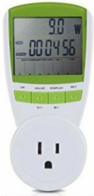
A watt meter, like the example shown above, is a useful tool for measuring the energy requirements of any device that runs on high-voltage AC power from the grid. The watt meter plugs into the wall socket and the appliance plugs into the watt meter. An LCD display on the watt meter then displays the amount of power the device is using. This is the most accurate way of measuring your true power consumption.
