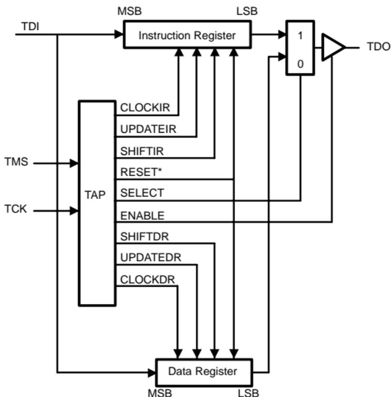
**Figure 3-4. TAP Control Output Interconnect Diagram**
