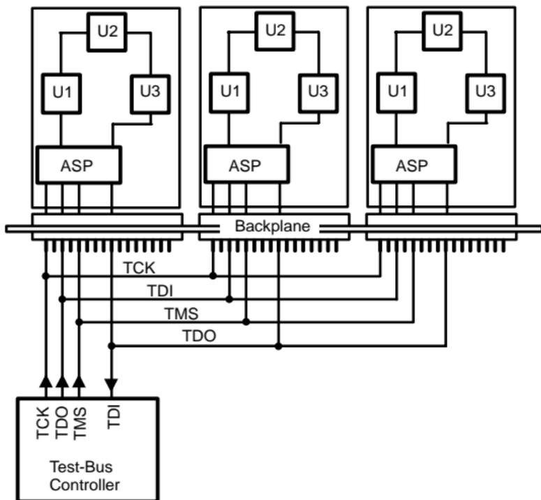
**Figure 7-15. Backplane With ASP-Equipped Boards**
