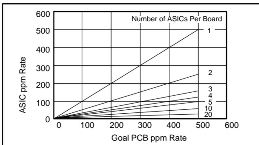
**Figure 4-5. ASIC ppm Versus PCB ppm Rate**
