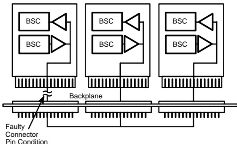
**Figure 7-8. PWB Connector Fault**
