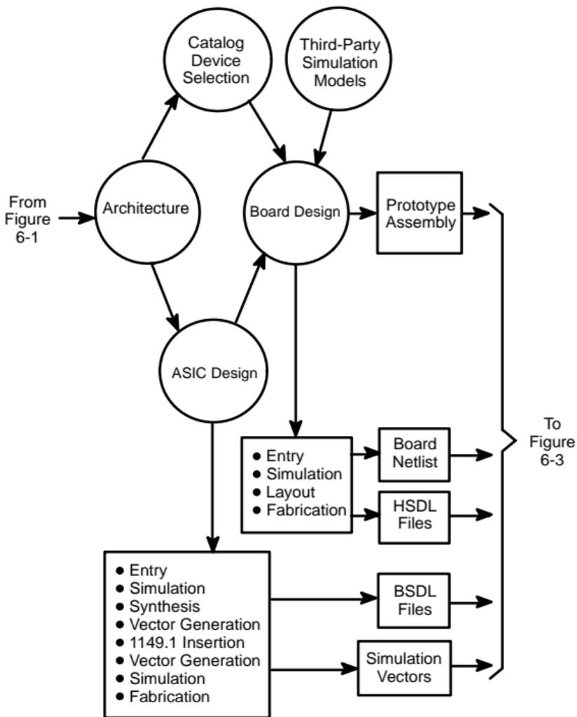
**Figure 6-2. Designing Testability for ASICs and Boards**
