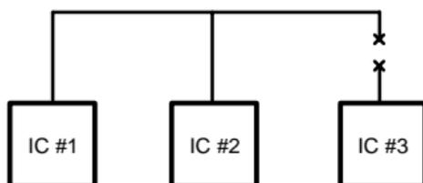
**Figure 7-3. Open-Solder-Joint Condition**
