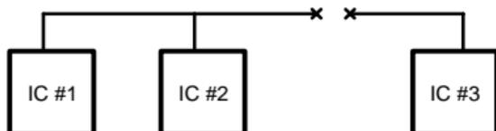
**Figure 7-2. Open-Etch Condition**
