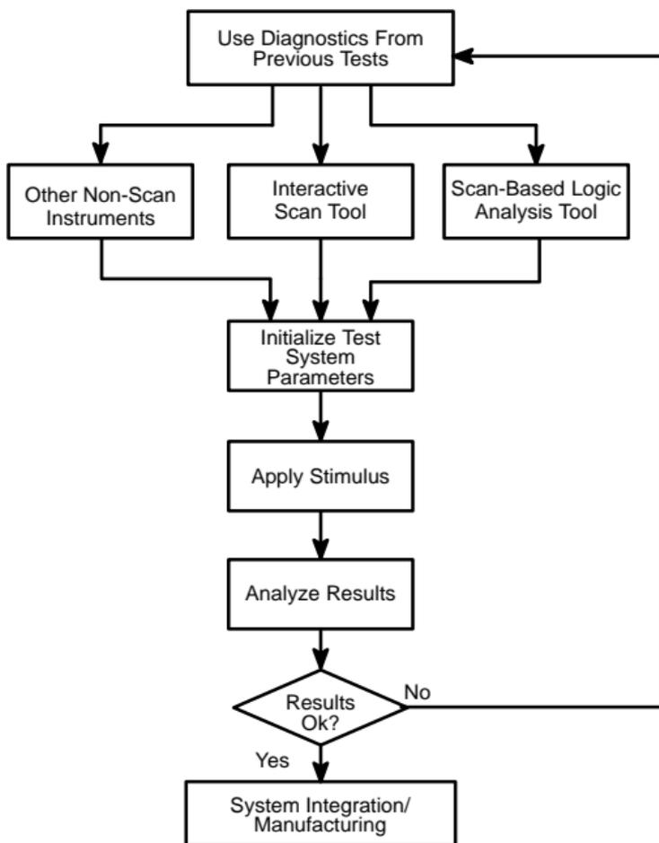
**Figure 7-19. Interactive Verification and Fault Isolation**
