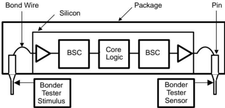
**Figure 7-5. Bond-Wire Testing**
