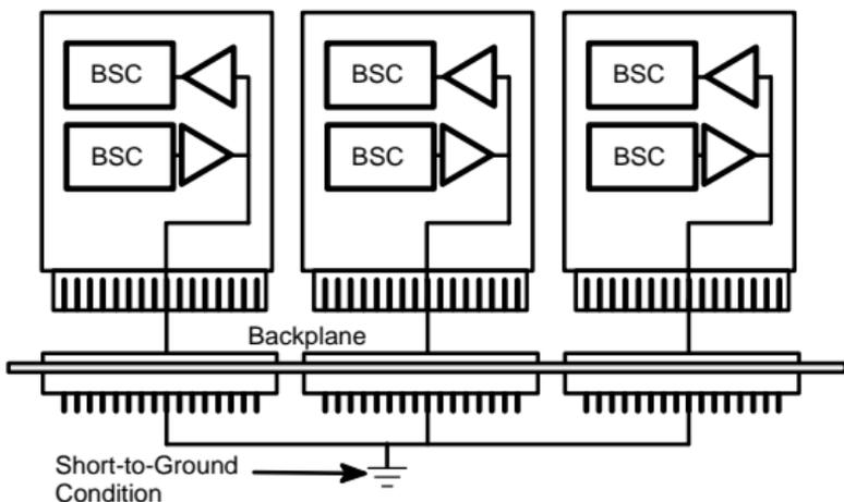
**Figure 7-9. Backplane Short-to-Ground Fault**
