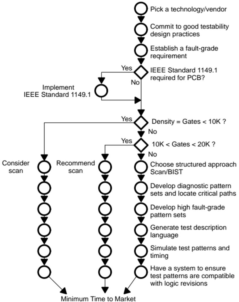
**Figure 4-7. Testability Development Flow**
