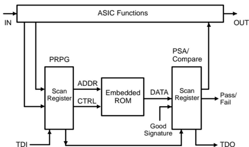
**Figure 7-12. Testing Embedded ROM**
