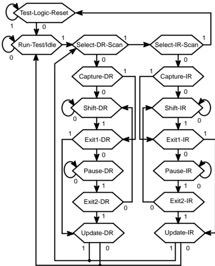
Note: The value shown adjacent to each state transition in this figure represents the signal present at TMS at the rising edge of TCK.
