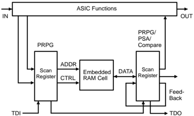
**Figure 7-11. Testing Embedded RAM**
