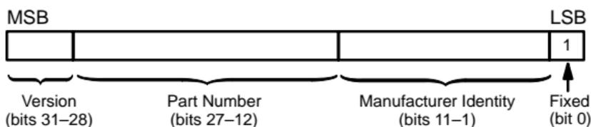
**Figure 3-8. Device Identification Register Structure**
