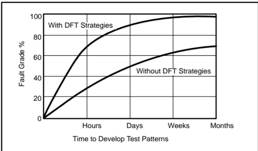
**Figure 4-1. Fault Grade Versus Development Time**
