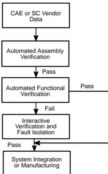
**Figure 7-16. General Boundary-Scan Test**
