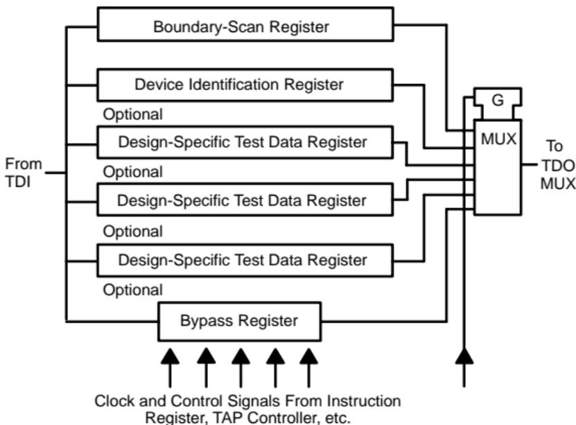
**Figure 3-6. Test Data Register Architecture**
