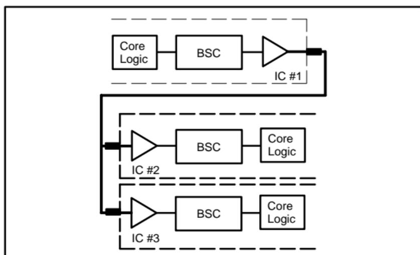
**Figure 7-1. Etch/Interconnect Testing**
