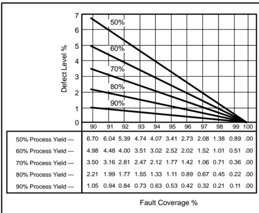
**Figure 4-3. Defect Level Versus Fault Coverage**
