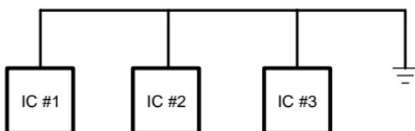
**Figure 7-4. Short-to-Ground Condition**
