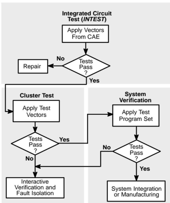
**Figure 7-18. Automated Functional Verification and Fault Detection**
