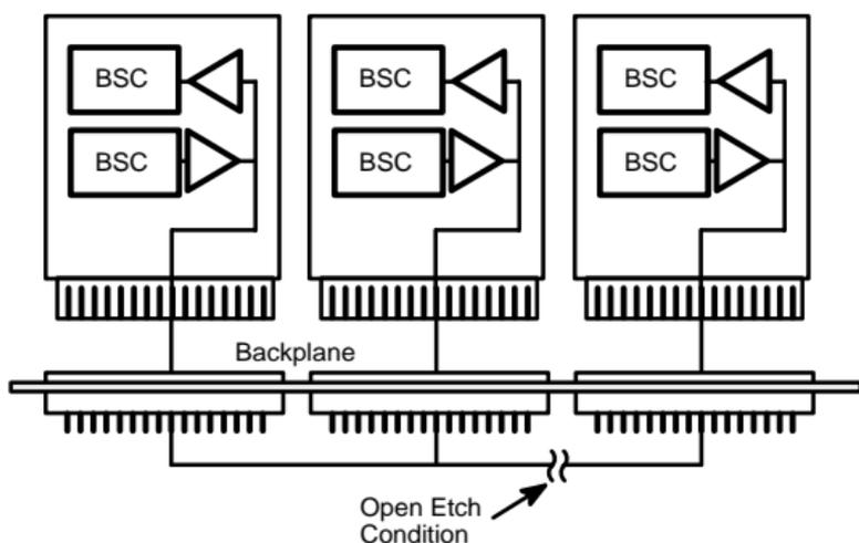
**Figure 7-7. Backplane Open-Circuit Fault**
