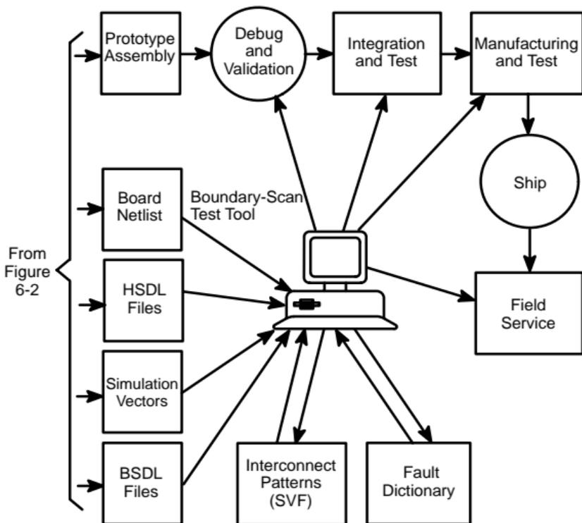
**Figure 6-3. Debug and Verification of a Boundary-Scan Design**
