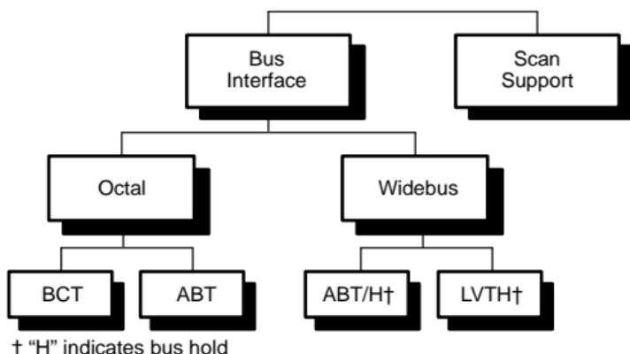
**Figure 8–1. TI's Family of IEEE Std 1149.1 (JTAG) Boundary-Scan Logic**
