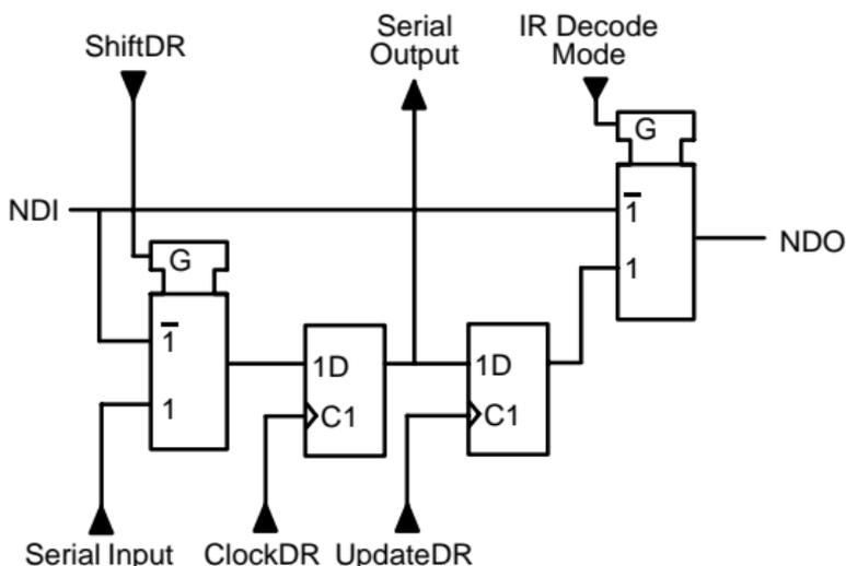
**Figure 3-7. Conceptual View of a Control-and-Observe BSC**
