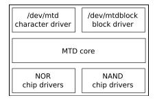
The chip drivers are at the lowest level and interface with flash chips. Only a small number of drivers are needed for NOR flash chips, enough to cover the CFI standard and variations plus a few non-compliant chips, which are now mostly obsolete. For NAND flash, you will need a driver for the NAND flash controller you are using; this is usually supplied as part of the board support package. There are drivers for about 40 of them in the current mainline kernel in the directory drivers/mtd/nand.
