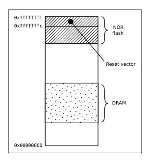
From that point, the bootloader code running in NOR flash memory can initialize the DRAM controller, so that the main memory, the DRAM, becomes available and then it copies itself into the **DRAM**. Once fully operational, the bootloader can load the kernel from flash memory into **DRAM** and transfer control to it.
