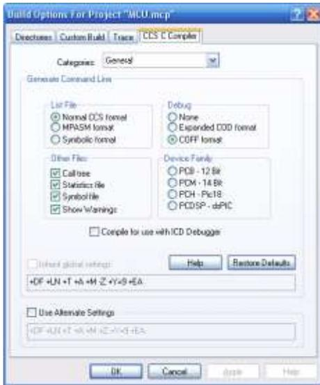
To compile the files in a project and build the project itself, select either the *Project* tab in the menu bar or right-click on the files in the Project window.
