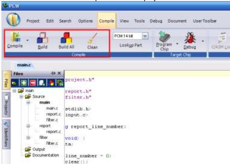
After a file has been compiled, the files used during the compilation will appear under the unit's name in the *Files* pane.
