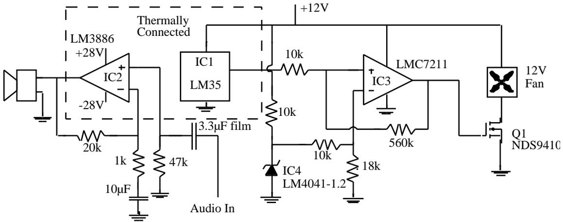
**Figure 5.12.** In this typical monolithic temperature sensor application, sensor IC1 and its leads are attached to 60W audio power amplifier IC2's heat sink. When the heat sink's temperature rises above the 60°C threshold temperature, comparator IC3's output goes high, turning on the cooling fan.
