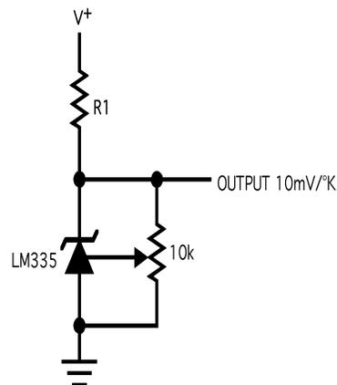
**Figure 3.1. Typical Connection for LM135, LM235, and LM335. Adjust the potentiometer for the correct output voltage at a known temperature (for example 2.982V @ 25°C), to obtain better than  $\pm 1^\circ\text{C}$  accuracy over the -55°C to +150°C temperature range.**
