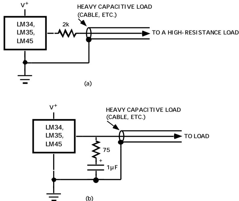
**Figure 4.5. Capacitive drive options. The LM34, LM35, and LM45 can drive large external capacitance if isolated from the load capacitance with a resistor as in (a), or compensated with an R-C network as in (b).**
