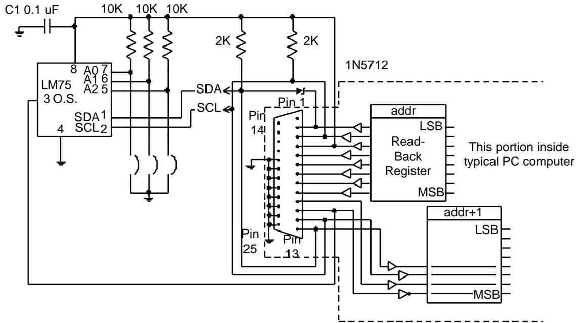
Figure 5.6. PC-Based Temperature Acquisition via the Parallel Printer Port.
