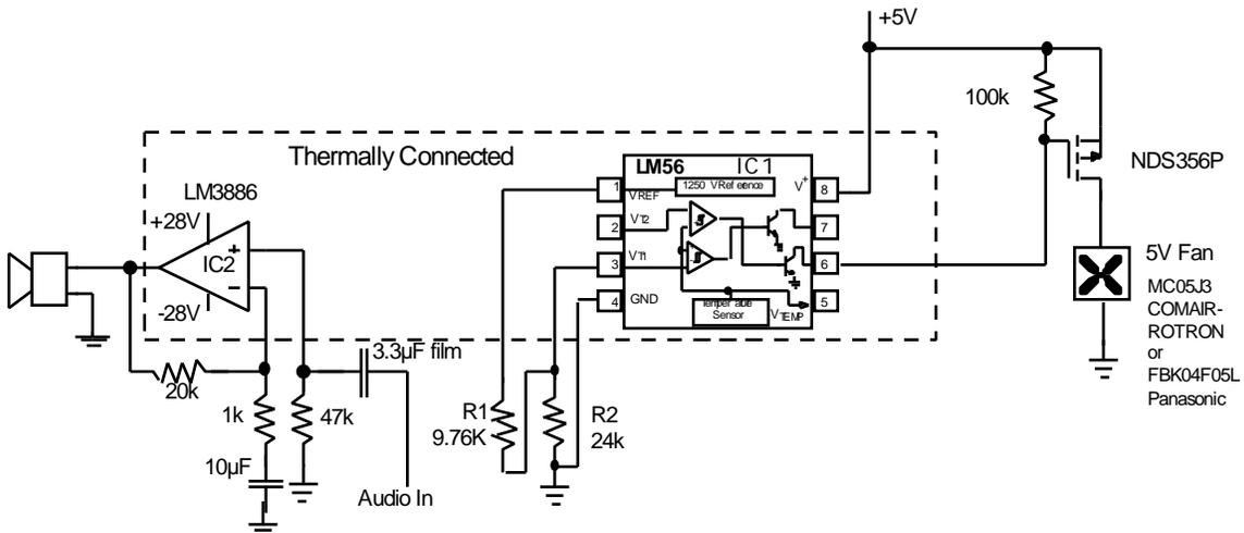
**Figure 5.13.** This circuit's function is similar to that of the circuit above, except that the sensor, comparator, and voltage reference are integrated within the LM56. In this circuit, the fan turns on at 80°C and off at 75°C.
