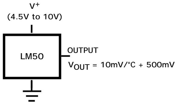
Figure 3.3. LM50 Typical Connection
