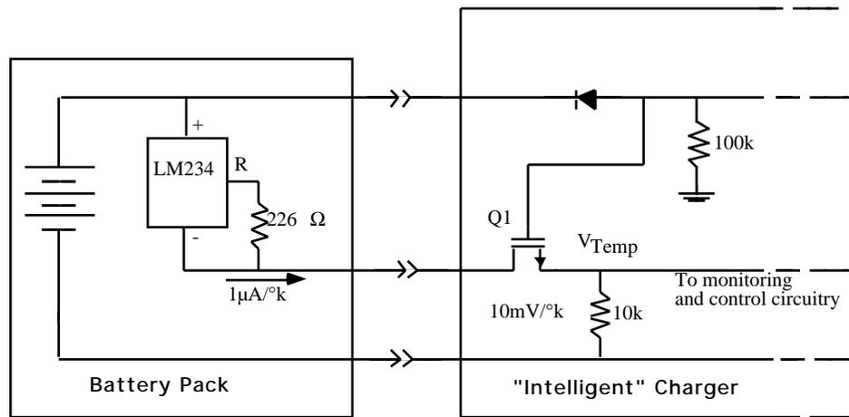
**Figure 5.10.** This battery pack temperature sensor uses no power unless Q1 (located either in the charger, as shown here, or in the “load system”) is turned on. This helps prevent accidental battery discharge.
