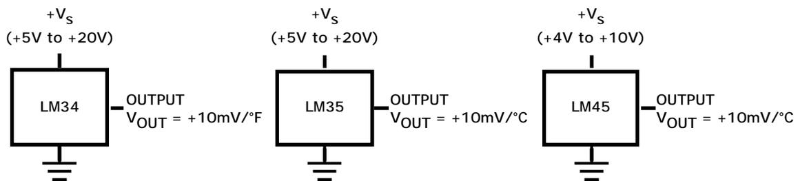
Figure 3.2. LM35, 45, 34 Typical Connections. Each IC is essentially a 3-terminal device (supply, ground, and output), although some are available in packages with more pins.
