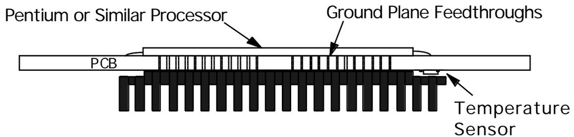
Figure 4.3. Sensor mounted near edge of soldered processor.
