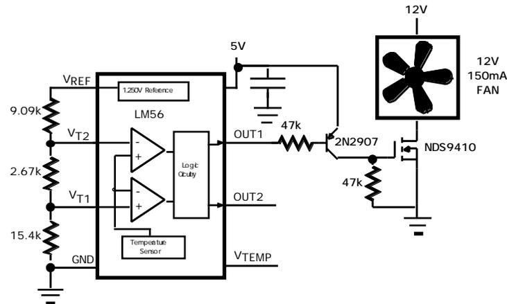
**Figure 5.1.** This circuit turns on a 12V cooling fan when the LM56's temperature exceeds 50°C. OUT2 goes low when the temperature reaches 70°C. The comparator outputs are open collector, so OUT2 will need a pull-up resistor if it is to drive a logic input.
