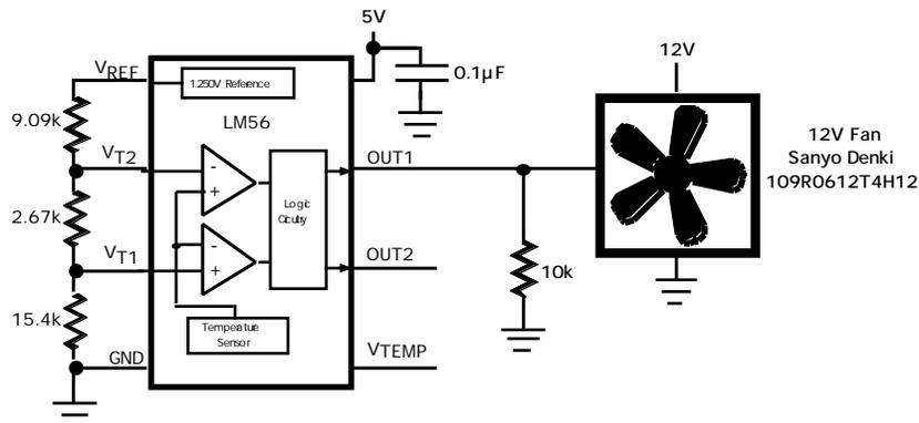
**Figure 5.3.** You can control some fans without adding a power device to the system. This circuit controls a fan's speed by taking a "third lead" low when temperature is high. This increases the fan's speed to provide additional cooling.
