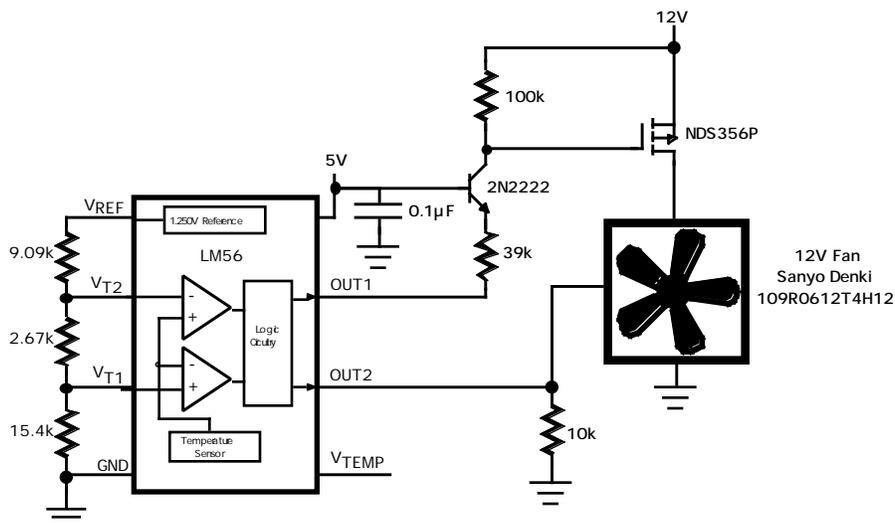
**Figure 5.4.** By combining the two approaches shown in the previous circuits, you can build a fan controller that turns the fan on at one temperature, then increases its speed if temperature rises above a second threshold.
