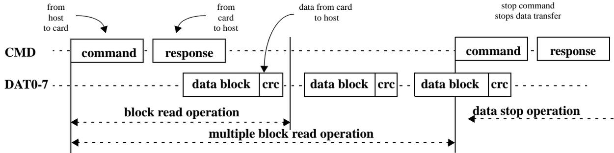
Figure 7 — Multiple-block read operation
