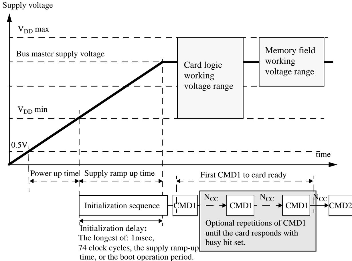
Figure 58 — Power-up diagram
