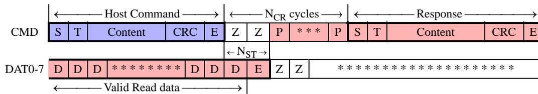
Figure 38 — Stop command timing (CMD12, data transfer mode)
