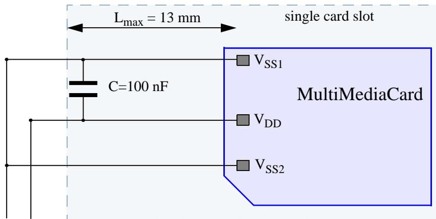
**Figure A.1 — Power supply decoupling**
