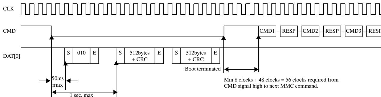
Figure 23 — MultiMediaCard state diagram (boot mode)
