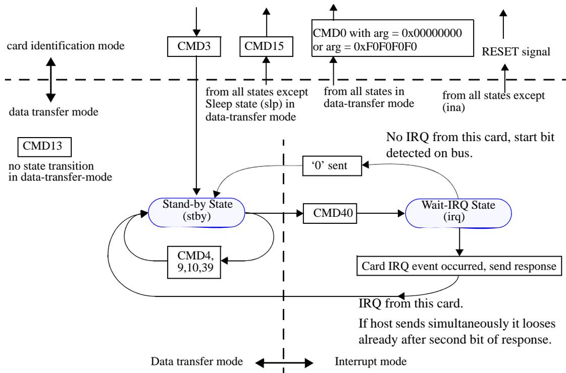
Figure 27 — MultiMediaCard state transition diagram, interrupt mode
