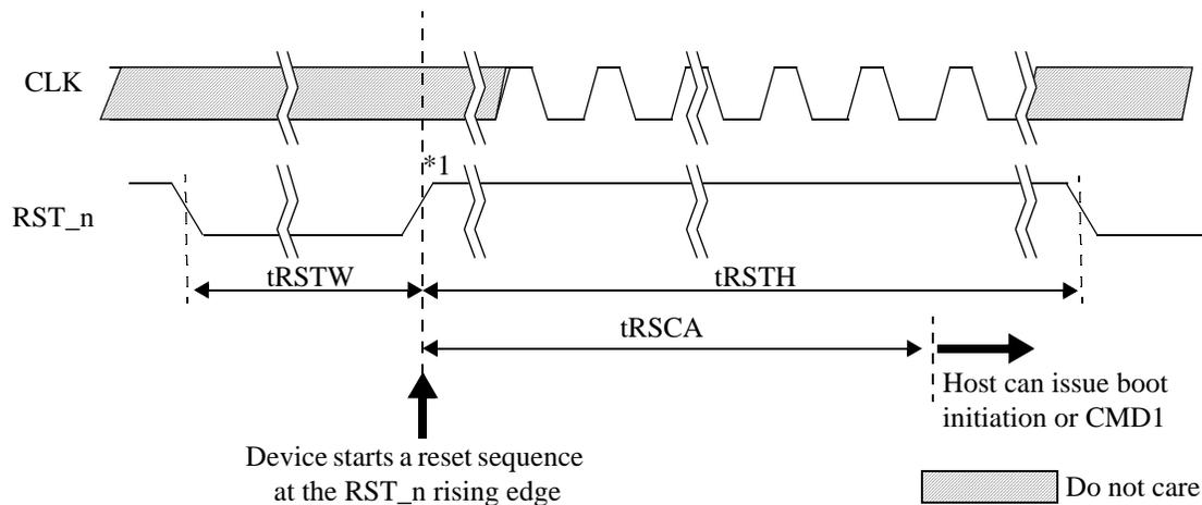
Note1: Device will detect the rising edge of RST\_n signal to trigger internal reset sequence
