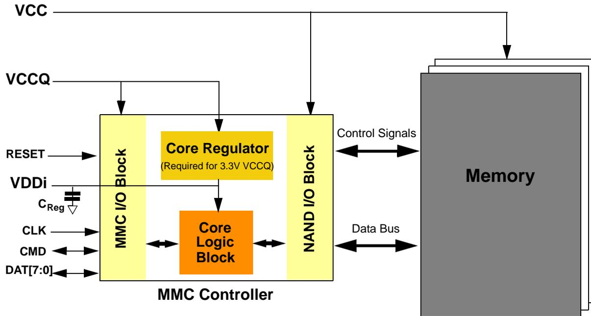
Figure 62 — *e*•MMC internal power diagram
