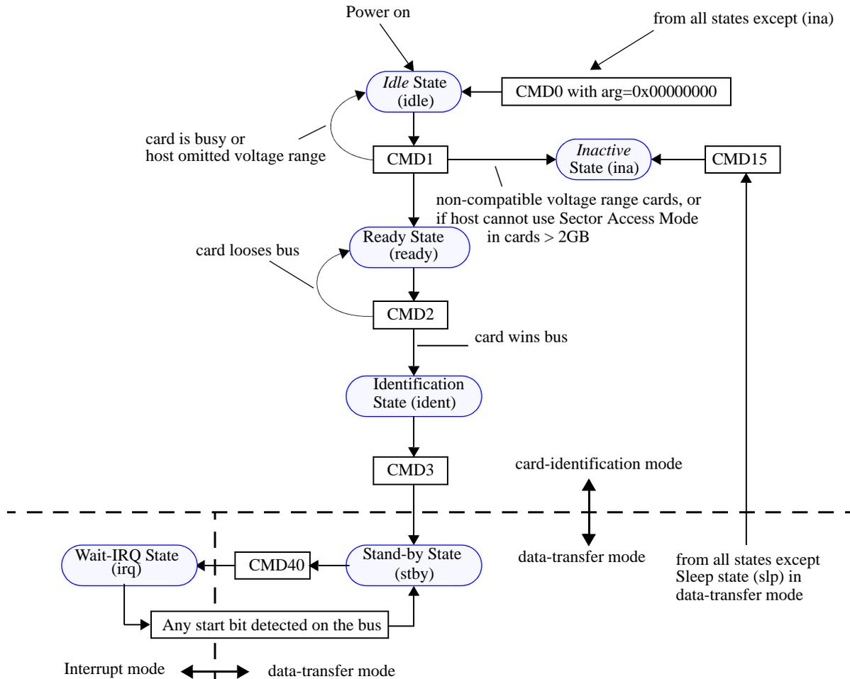
**Figure 26 — MultiMediaCard state diagram (card identification mode)**
