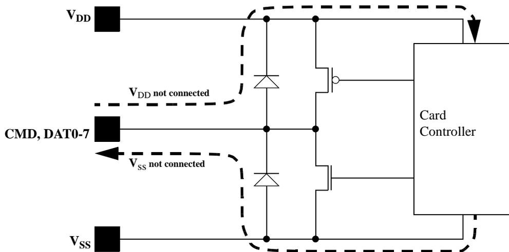
Figure 56 — Improper power supply
