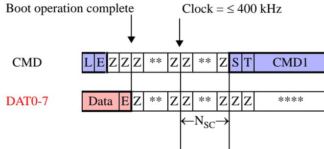
**Figure 48 — Bus mode change timing (push-pull to open-drain)**
