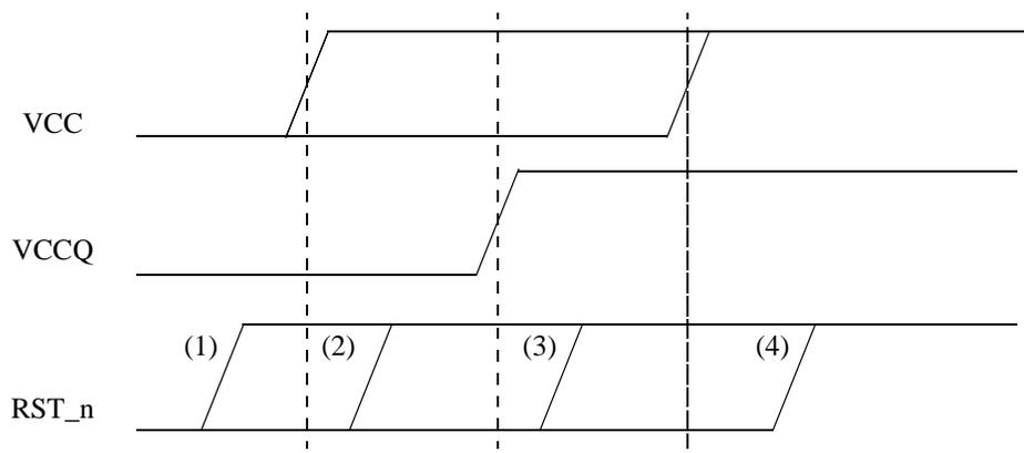
**Figure 21 — RST<sub>n</sub> signal at the power up period**
