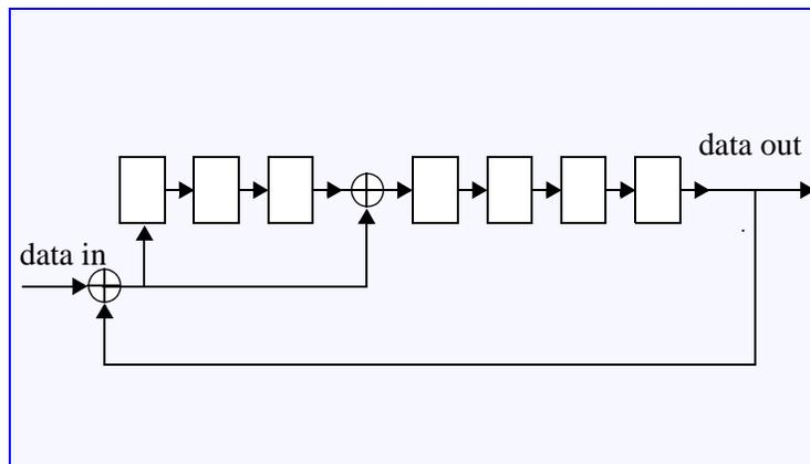
Figure 53 — CRC7 generator/checker
