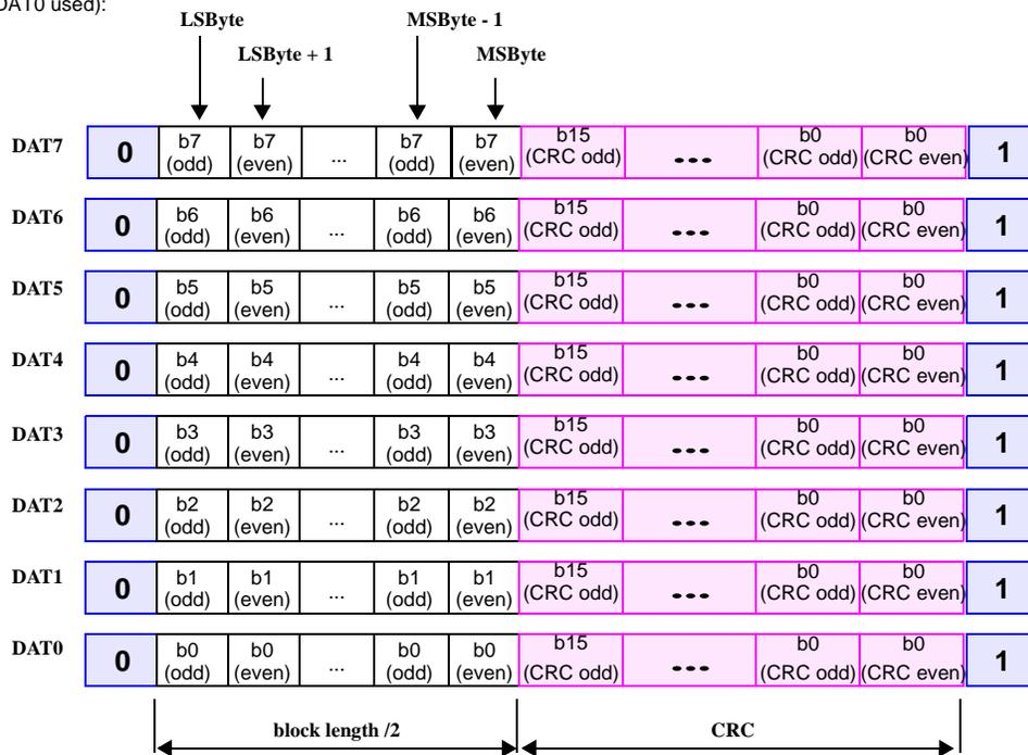
Notice that bytes DATA and the two CRC16 are interleaved. Start and stop bits are full cycle.
