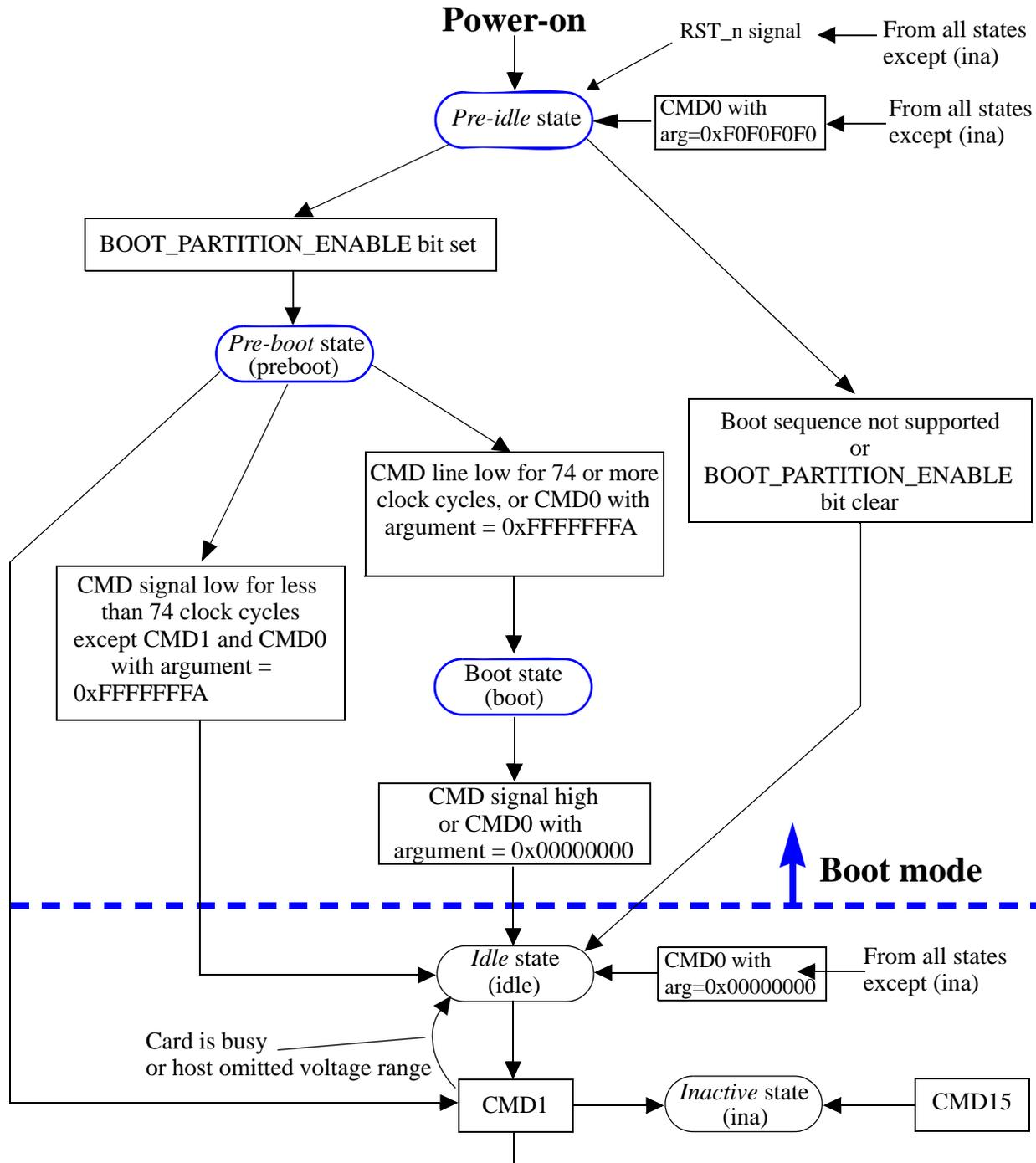
Figure 25 — MultiMediaCard state diagram (boot mode)
