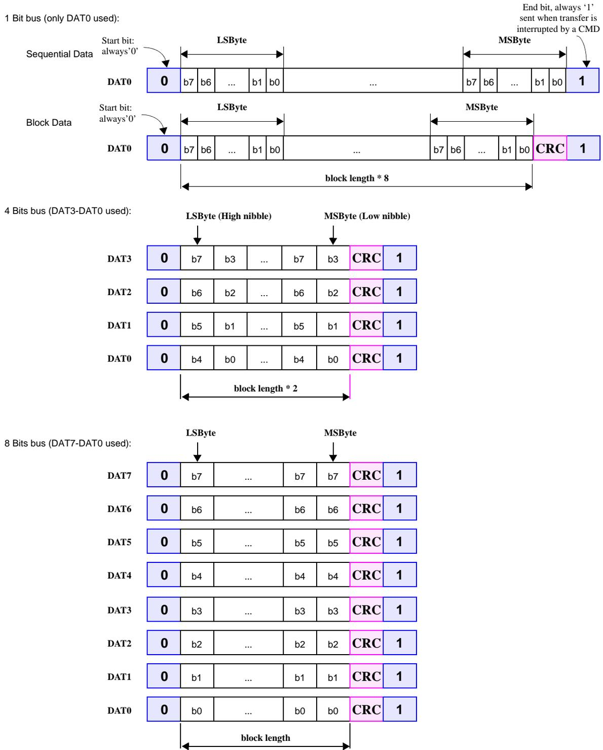
Figure 13 — Data packet format for SDR
