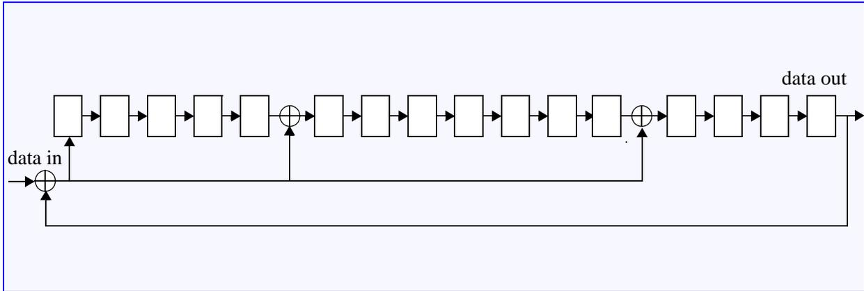
Figure 54 — CRC16 generator/checker
