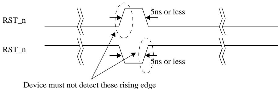
Figure 52 — Noise filtering timing for H/W reset
