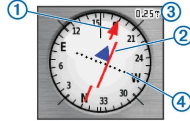
The course pointer ① indicates your relationship to the course line leading to the destination. The course deviation indicator (CDI) ② provides the indication of drift (right or left) from the course. The scale ③ refers to the distance between dots ④ on the course deviation indicator, which tell you how far off course you are.
