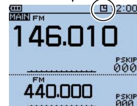
To return to the default setting, push [QUICK]
