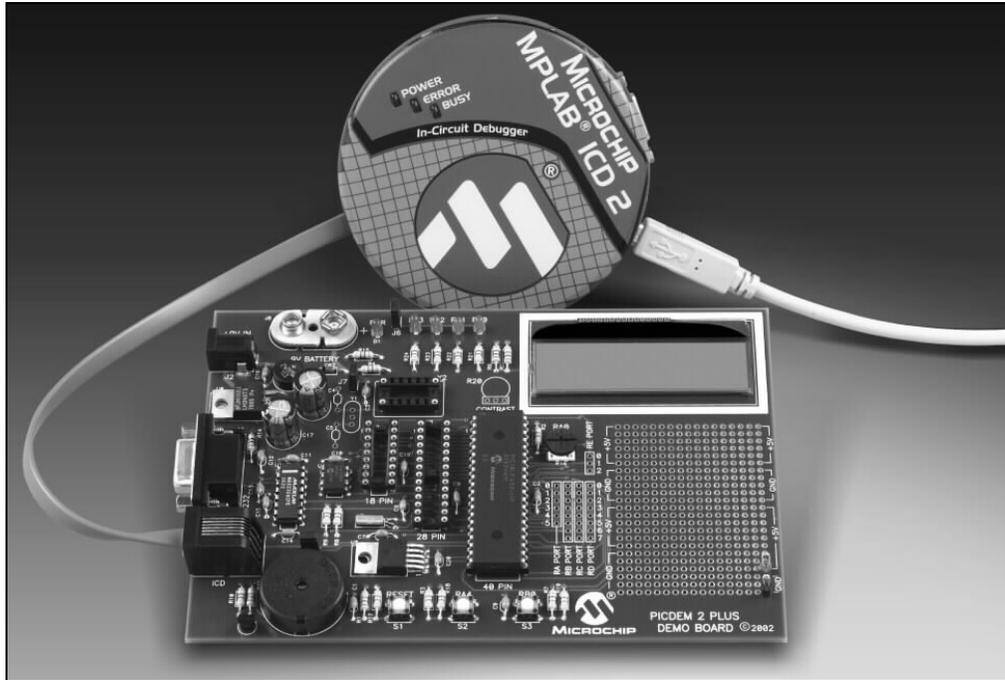
Configure the PICDEM 2 Plus for the desired oscillator as described in Table 2-1. Refer to the ICE/ICD user's guide for any oscillator configuration requirements.
